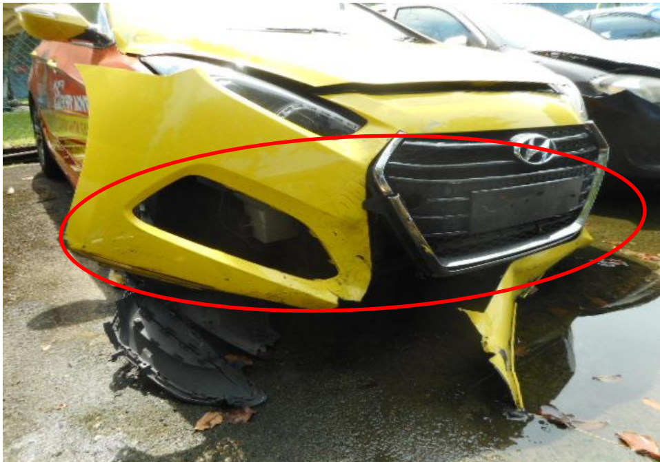
Photo 5 shows a close up view of the Taxi's front portion at the time of my inspection. It appeared to have sustained damage at its front portion. Its front bumper (circled) were damaged at the time of my inspection as a result of the accident.
