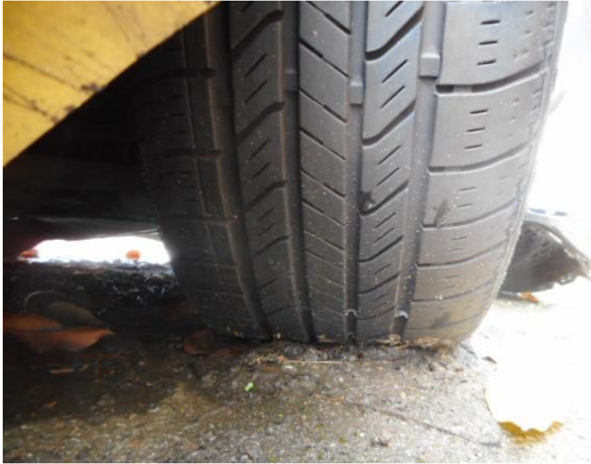
Photo 8 shows the condition of the front right tyre of the Taxi, which was observed to be in serviceable condition with remaining tread depth of approximately 5.1mm. The tyre, which was wrapped around standard steel wheel rim, was also observed to be sufficiently inflated for vehicular operation. There was no tear, cut or burst mark(s) on the outer and the inner sidewalls as well as across the tread of the 4 tyres that were fitted on the Taxi.
