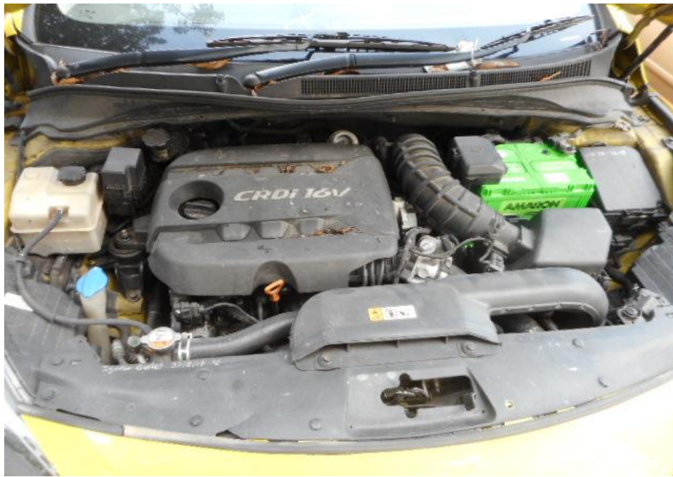
Photo 12 shows a general view of the Taxi's engine compartment, which was accessed by lifting the front cabin of the Taxi. The various parts and components inside the engine compartment were unaffected by the accident. There was also no sign(s) or indication(s) of fresh fluid leakage and/or fluid stain within the engine compartment
