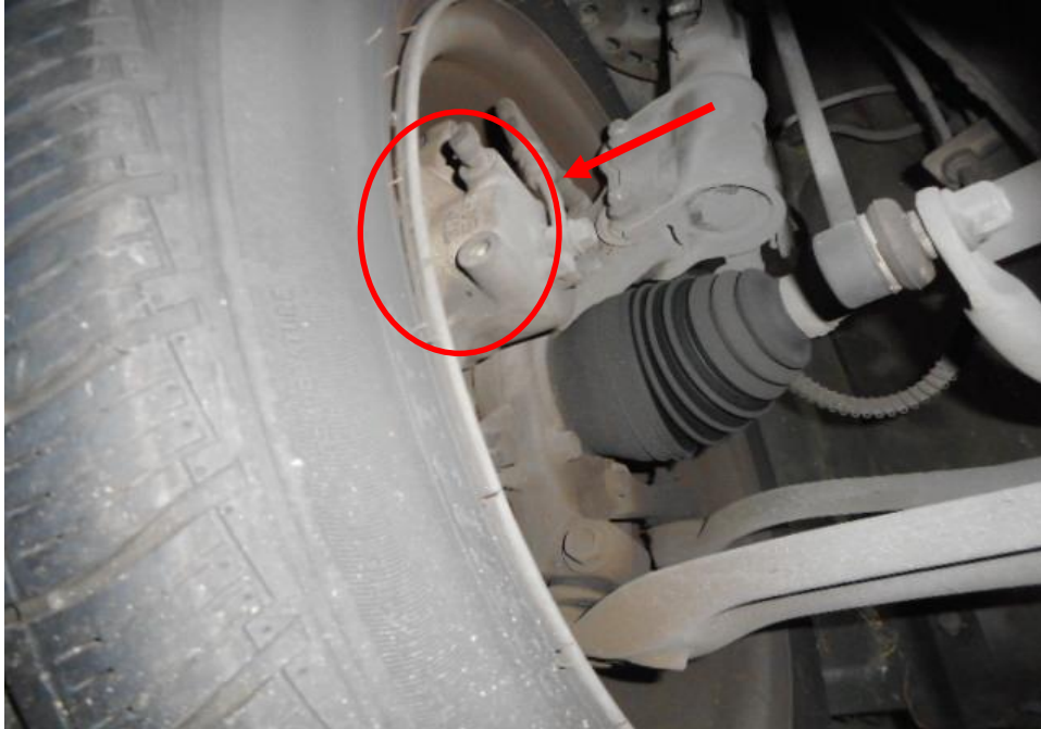
Photo 22 shows the brake hose/pipe (arrowed) at the front right wheel of the Taxi. No leakage of brake fluid was observed. Visual examination of the various components of the braking system like the brake caliper (circled), brake booster, brake pedal etc had revealed all to be intact and without visible damage at the time of accident. There was also no sign of fluid stain(s) observed on the various undercarriage components.
