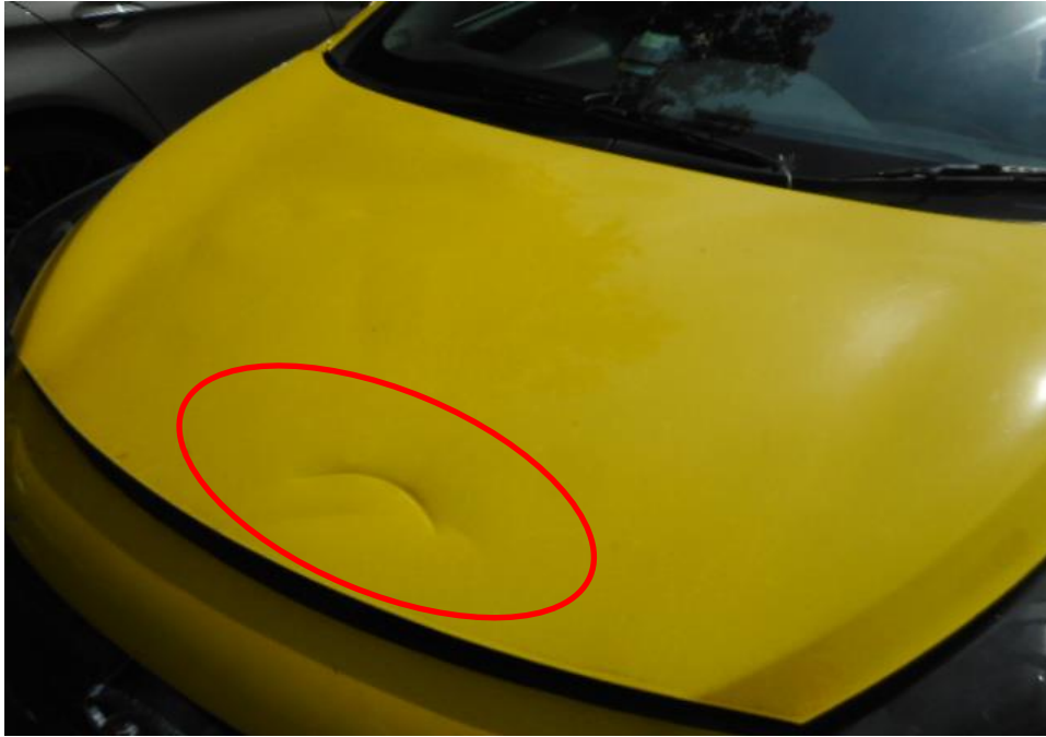
Photo 4 shows a close up view of the Taxi's front portion at the time of my inspection. It appeared to have sustained damage at its front portion. Its front bonnet (circled) were damaged at the time of my inspection as a result of the accident.
