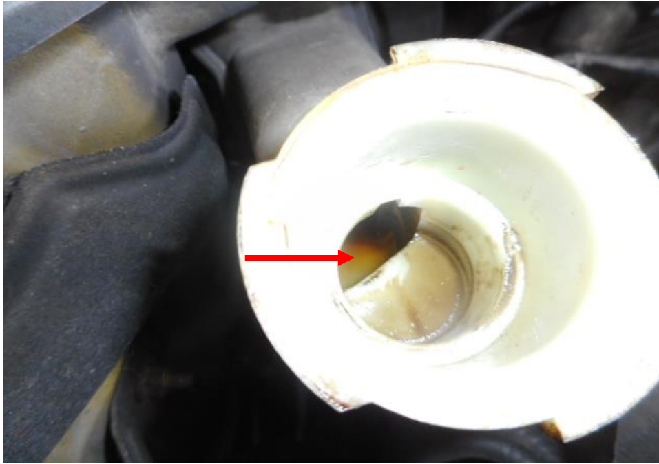
Photo 13 shows the brake fluid reservoir of the Taxi at the time of my inspection. The brake fluid was observed to be of sufficient level (arrowed) and without any visible contamination.
