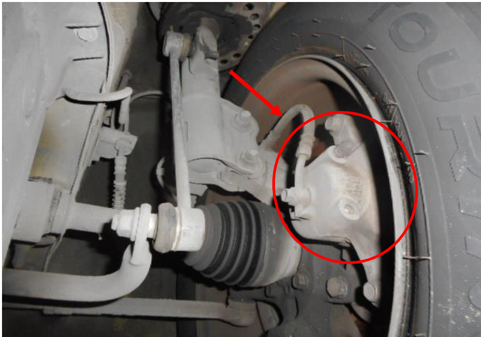
Photo 23 shows the brake hose/pipe (arrowed) at the front left wheel of the Taxi. No leakage of brake fluid was observed. Visual examination of the various components of the braking system like the brake caliper (circled), brake booster, brake pedal etc had revealed all to be intact and without visible damage at the time of accident. There was also no sign of fluid stain(s) observed on the various undercarriage components.
