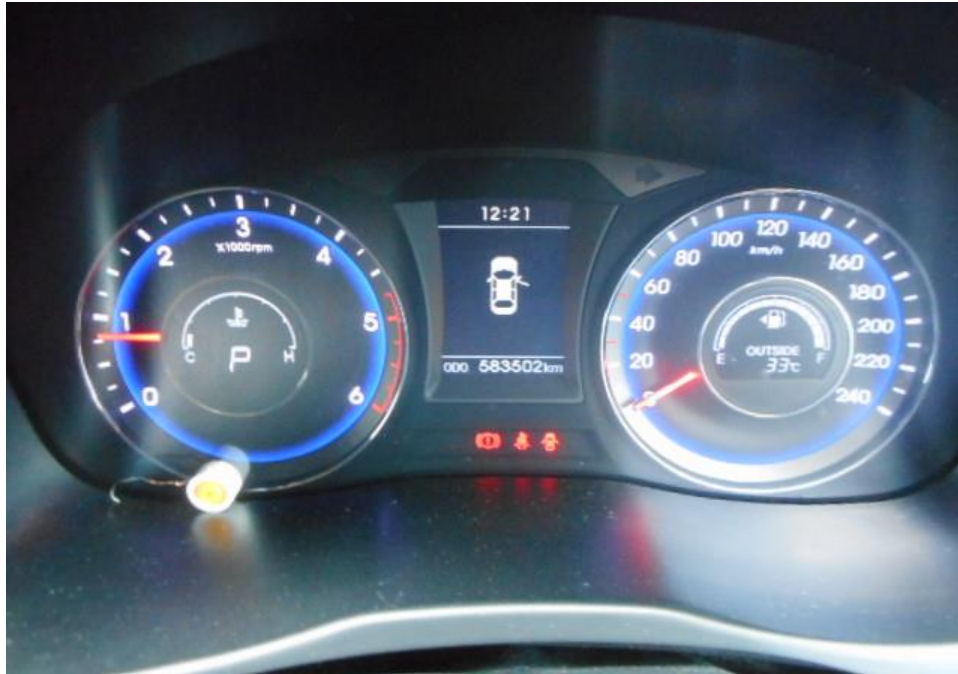
Photo 25 shows no warning lights illuminated on the instrument panel of the Taxi after the engine was cranked. This would suggest that there was no abnormality to the electronic operating system of the Taxi, like the ABS, EPS, SRS, and TC etc.
