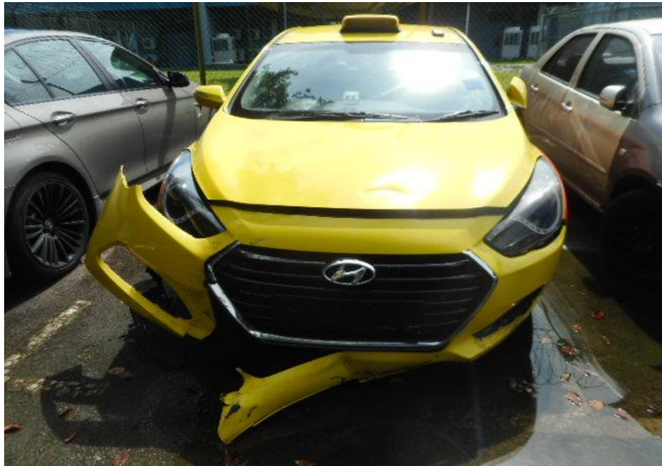
Photo 3 shows a general view of the Taxi's front portion at the time of my inspection. It appeared to have sustained damage at its front portion. Its front bonnet and front bumper were damaged at the time of my inspection as a result of the accident.
