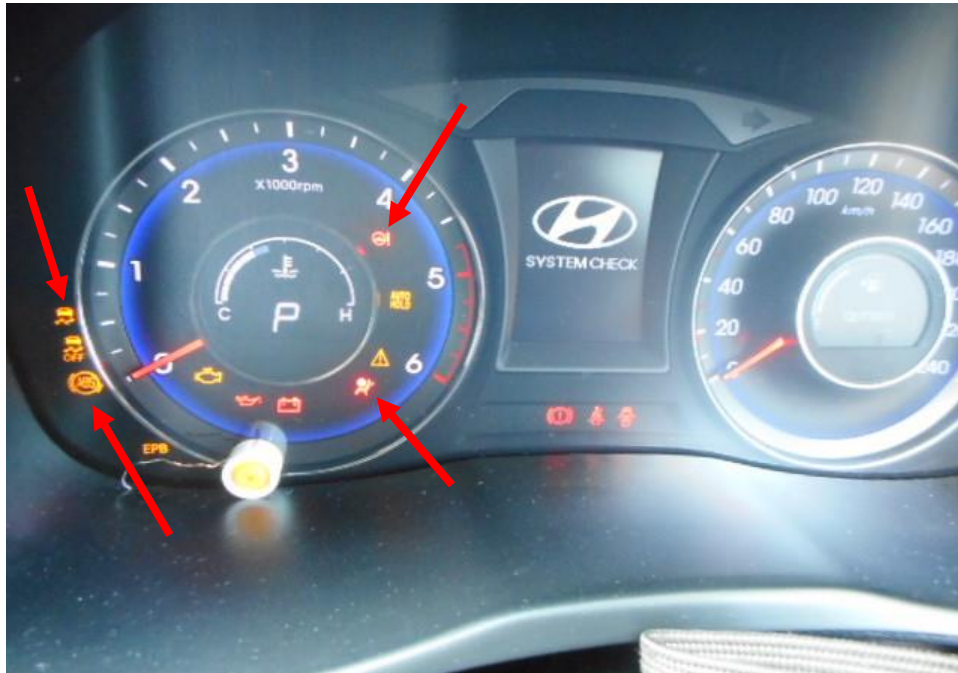
Photo 24 shows the warning light for Anti-Lock Brake System (ABS) and Power Steering System (EPS), Supplemental Restraint System (SRS) and Traction Control (TC) (arrowed) appearing on the instrument panel of the Taxi during the self-test of its various electronic operating systems when its engine was cranked.
