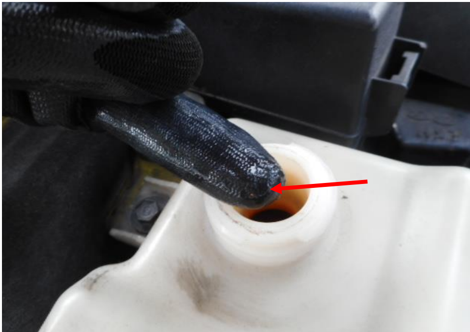
Photo 14 shows the engine coolant reservoir of the Taxi at the time of my inspection. The engine coolant was observed to be of sufficient level (arrowed) and without any visible contamination.
