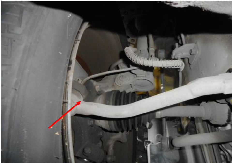
Photo 18 shows the various undercarriage components at the front left wheel of the Taxi, in particular the steering tie rod end (arrowed). The various undercarriage components of the Taxi were all found to be intact without any visible damage. There was also no sign of fluid stain(s) observed on the various undercarriage components.
