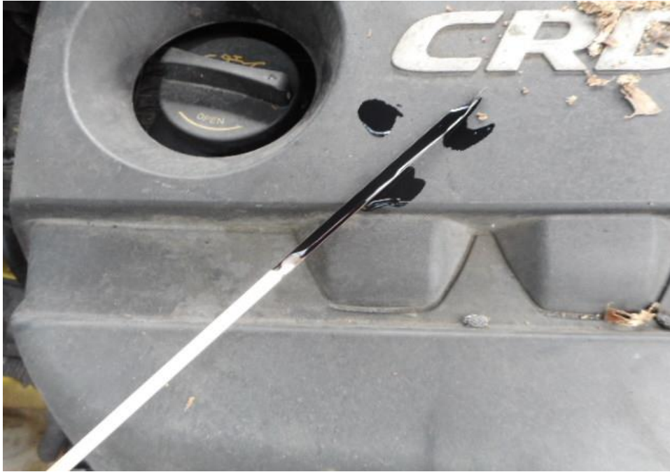
Photo 15 shows the engine oil dip stick of the Taxi at the time of my inspection. The engine oil was observed to be of sufficient level and without any visible contamination.
