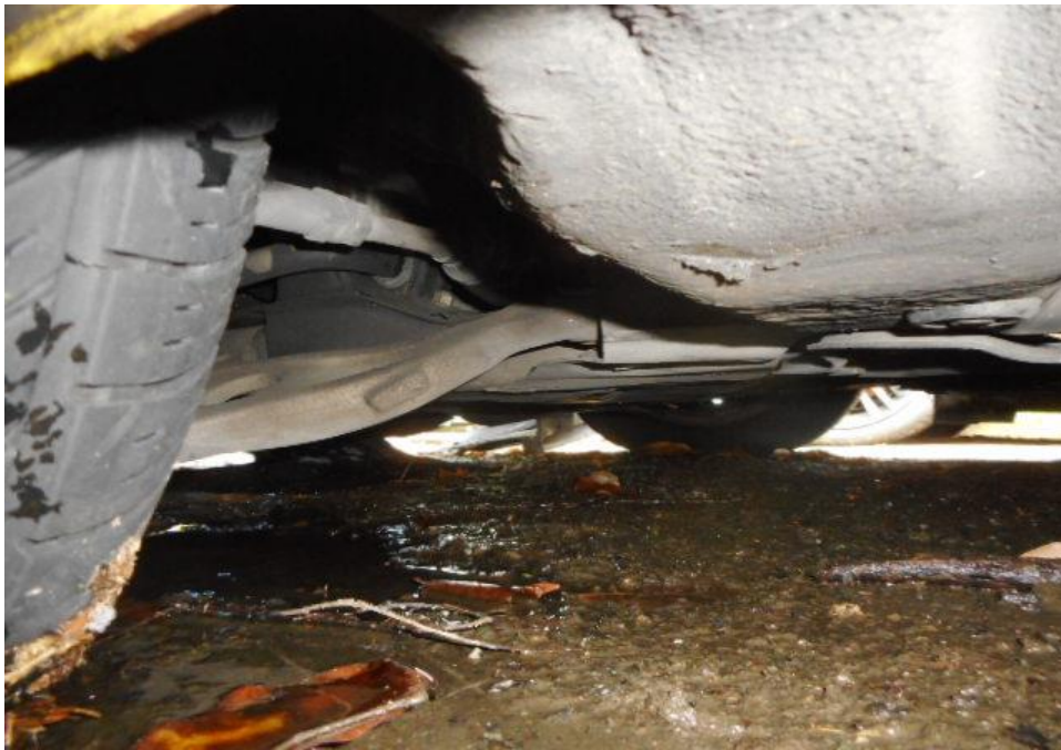
Photo 16 shows the undercarriage of the Taxi, at the area where the engine housing and transmission housing are located. I did not find any sign(s) or indication(s) of fluid leak and/or fluid stain(s) on the underside of the Taxi.
