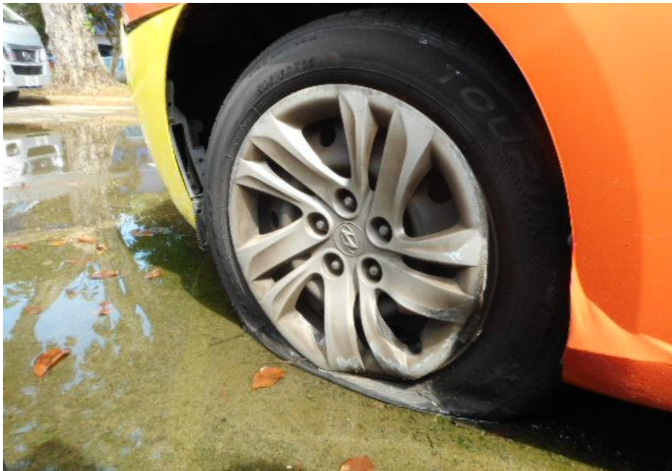
Photo 11 shows the condition of the front left tyre of the Taxi, which were observed to be in serviceable condition with remaining, tread depth of approximately 4.3mm. There was also no tear, cut or burst mark(s) on the outer and the inner sidewalls as well as across the tread of the 4 tyres that were fitted on the Taxi.
