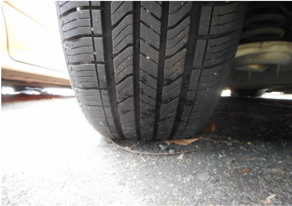
Photo 10 shows the condition of the rear left tyre of the Taxi, which was observed to be in serviceable condition with remaining tread depth of approximately 7.2mm. The tyres, which were wrapped around standard steel wheel rim, were also observed to be sufficiently inflated for vehicular operation.
