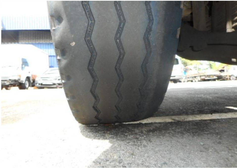
Photo 10 condition of the front left tyre of the Motor Lorry, which was observed to be in serviceable condition with remaining tread depth of approximately 3mm. The tyre, which was wrapped around standard steel wheel rim, was also observed to be sufficiently inflated for vehicular operation.
