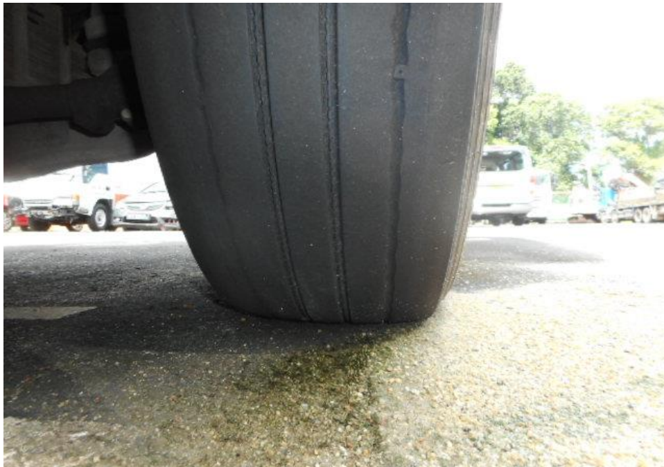
Photo 7 shows the condition of the front right tyre of the Motor Lorry, which was observed to be in serviceable condition with remaining tread depth of approximately 4.5mm. The tyre, which was wrapped around standard steel wheel rim, was also observed to be sufficiently inflated for vehicular operation. There was no tear, cut or burst mark(s) on the outer and the inner sidewalls as well as across the tread of the 10 tyres that were fitted on the Motor Lorry.
