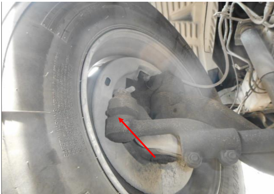
Photo 23 shows the various undercarriage components at the front left wheel of the Motor Lorry, in particular the steering tie rod end (arrowed). The various undercarriage components of the Motor Lorry were all found to be intact without any visible damage. There was also no sign of fluid stain(s) observed on the various undercarriage components.
