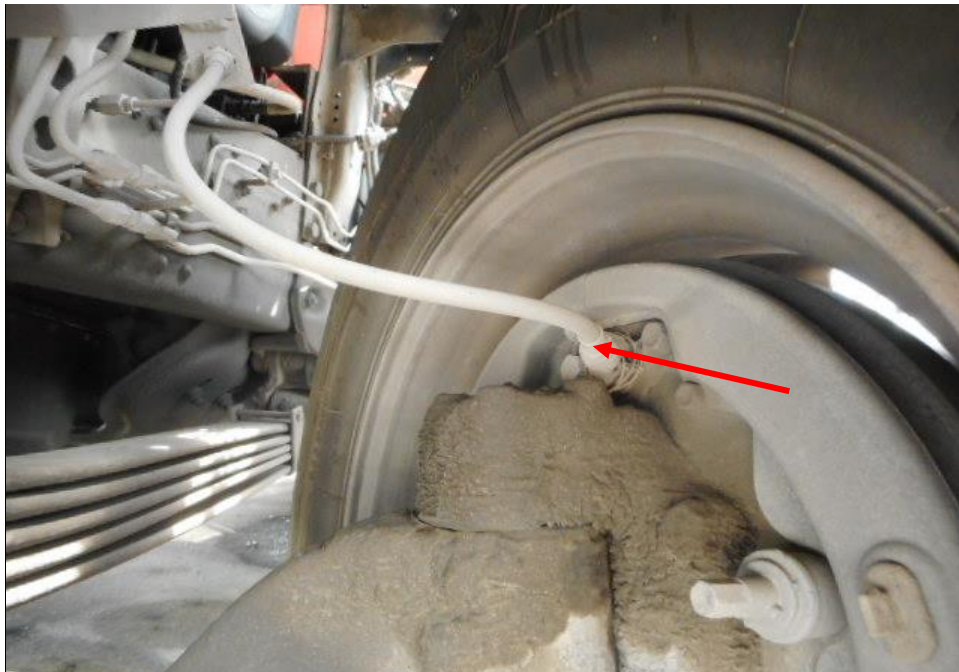
Photo 19 shows the brake pipe (arrowed) at the front right wheel of the Motor Lorry. I did not observe any leakage of brake fluid at the time of my inspection of the Motor Lorry. My static tests of the Motor Lorry's braking system, along with my visual examination of the various mechanical components in the braking system, had indicated that there was no internal leakage of pressure/vacuum and these components were generally in good condition.
