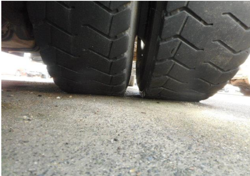
Photo 8 shows the condition of the rear right tyre of the Motor Lorry, which was observed to be in serviceable condition with remaining tread depth of approximately 4.5mm. The tyre, which was wrapped around standard steel wheel rim, was also observed to be sufficiently inflated for vehicular operation.
