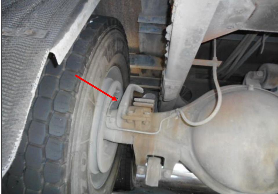
Photo 18 shows the brake pipe (arrowed) at the rear left wheel of the Motor Lorry. I did not observe any leakage of brake fluid at the time of my inspection of the Motor Lorry. My static tests of the Motor Lorry's braking system, along with my visual examination of the various mechanical components in the braking system, had indicated that there was no internal leakage of pressure/vacuum and these components were generally in good condition.
