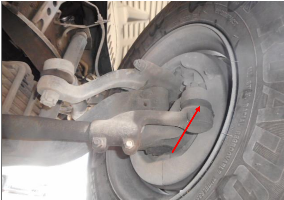
Photo 22 shows the various undercarriage components at the front right wheel of the Motor Lorry, in particular the steering tie rod end (arrowed). The various steering components were all found to be intact, suggesting that the steering system of the Motor Lorry was likely to be in serviceable condition at the material time of accident. There was also no sign of fluid stain(s) observed on the various undercarriage components.
