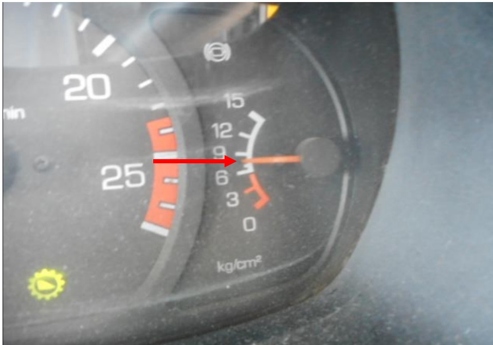
Photo 12 shows the air in the air brake cylinders of the Prime Mover at the time of my inspection. The air in the cylinder was observed to be of sufficient level & serviceable at the time of the accident.
