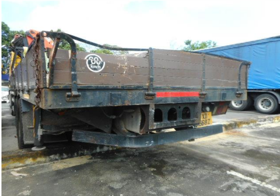
Photo 2 shows a general view of the Motor Lorry's rear body at the time of my inspection. The Motor Lorry was observed to sustained damage at its rear portion. Its rear left brake lamp and rear body panel were damage at the time of my inspection as a result of the accident.
