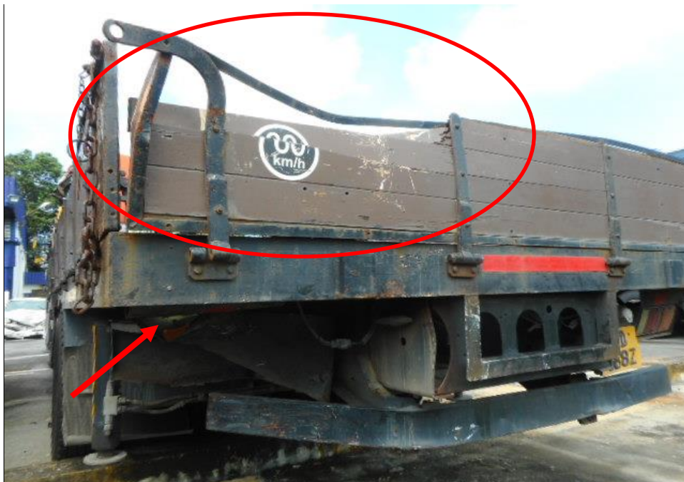
Photo 3 shows a close up view of the Motor Lorry's rear body at the time of my inspection. The Motor Lorry was observed to sustained damage at its rear portion. Its rear right brake lamp (arrowed) and rear body panel (circled) were damage at the time of my inspection as a result of the accident.
