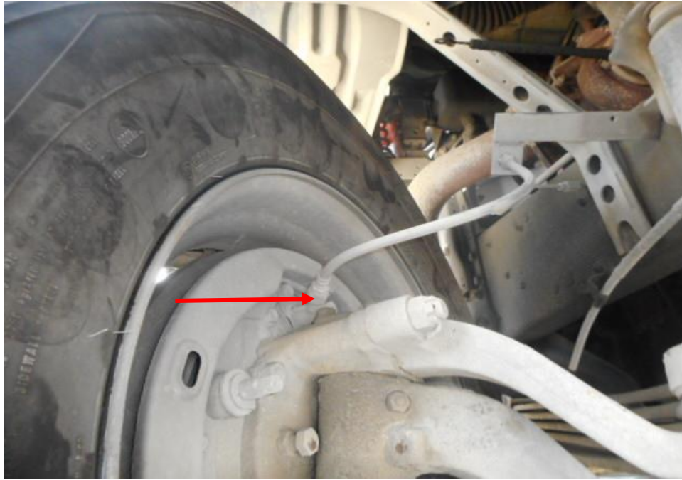
Photo 20 shows the brake pipe (arrowed) at the front left wheel of the Motor Lorry. I did not observe any leakage of brake fluid at the time of my inspection of the Motor Lorry. My visual examination of the various mechanical components in the braking system had indicated that these was no internal leakage of pressure/vacuum and these components were generally in good condition.
