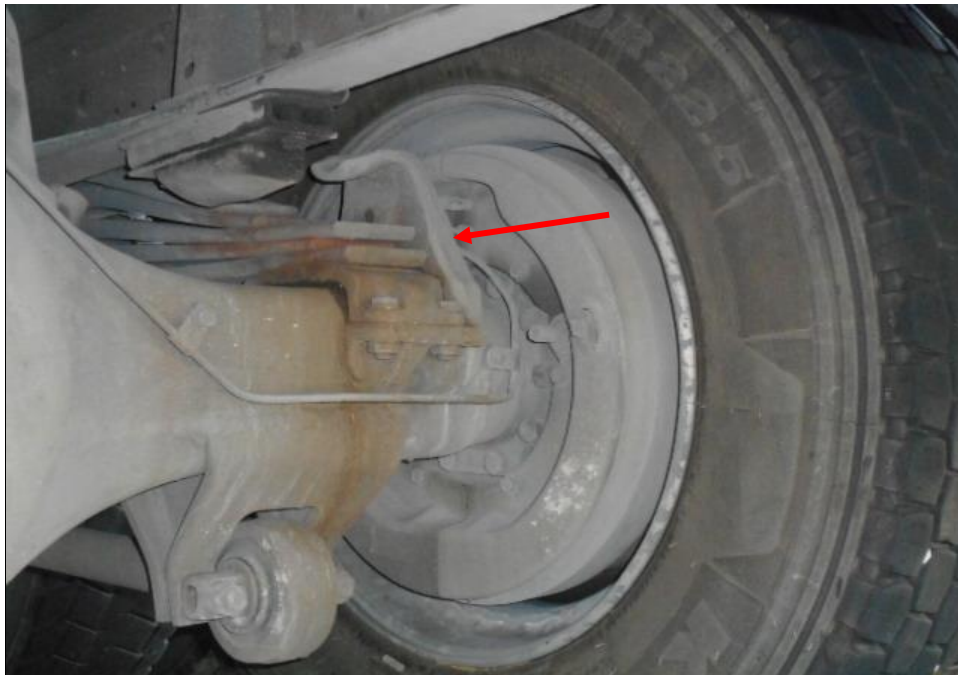
Photo 17 shows the brake pipe (arrowed) at the rear right wheel of the Motor Lorry. I did not observe any leakage of brake fluid at the time of my inspection of the Motor Lorry. My visual examination of the various mechanical components in the braking system, had indicated that these was no internal leakage of pressure/vacuum and these components were generally in good condition.
