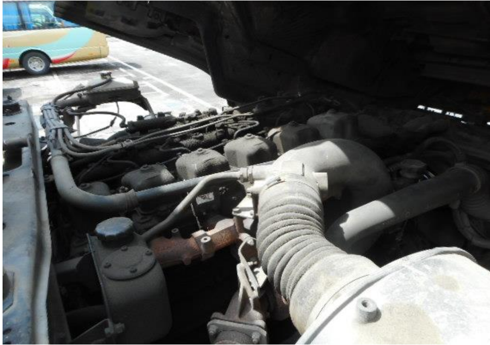
Photo 11 shows a general view of the Motor Lorry's engine compartment, which was accessed by lifting the front cabin of the Motor Lorry. The various parts and components inside the engine compartment were unaffected by the accident. There was also no sign(s) or indication(s) of fresh fluid leakage and/or fluid stain within the engine compartment
