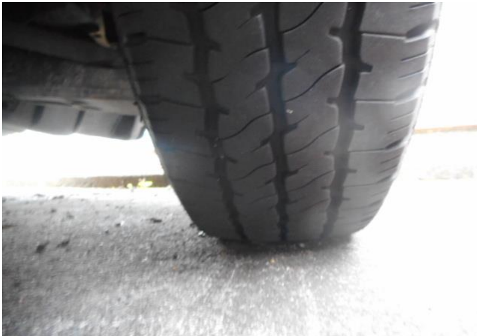
Photo 9 shows the condition of the front right tyre of the Motor Van, which was observed to be in serviceable condition with remaining tread depth of approximately 7.4mm. The tyre, which was wrapped around standard steel wheel rim, was also observed to be sufficiently inflated for vehicular operation. There was no tear, cut or burst mark(s) on the outer and the inner sidewalls as well as across the tread of the 4 tyres that were fitted on the Motor Van.
