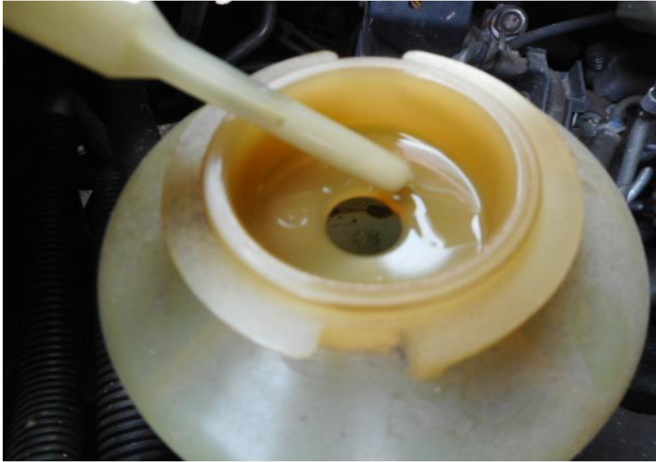
Photo 17 shows the power steering fluid reservoir of the Motor Van at the time of my inspection. The power steering fluid was observed to be of sufficient level and without any visible contamination.
