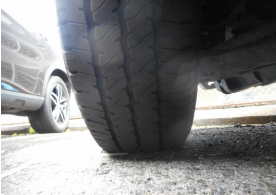
Photo 12 shows the condition of the rear right tyres of the Motor Van, which were observed to be in serviceable condition with remaining, tread depth of approximately 7.2mm. There was also no tear, cut or burst mark(s) on the outer and the inner sidewalls as well as across the tread of the 4 tyres that were fitted on the Motor Van.
