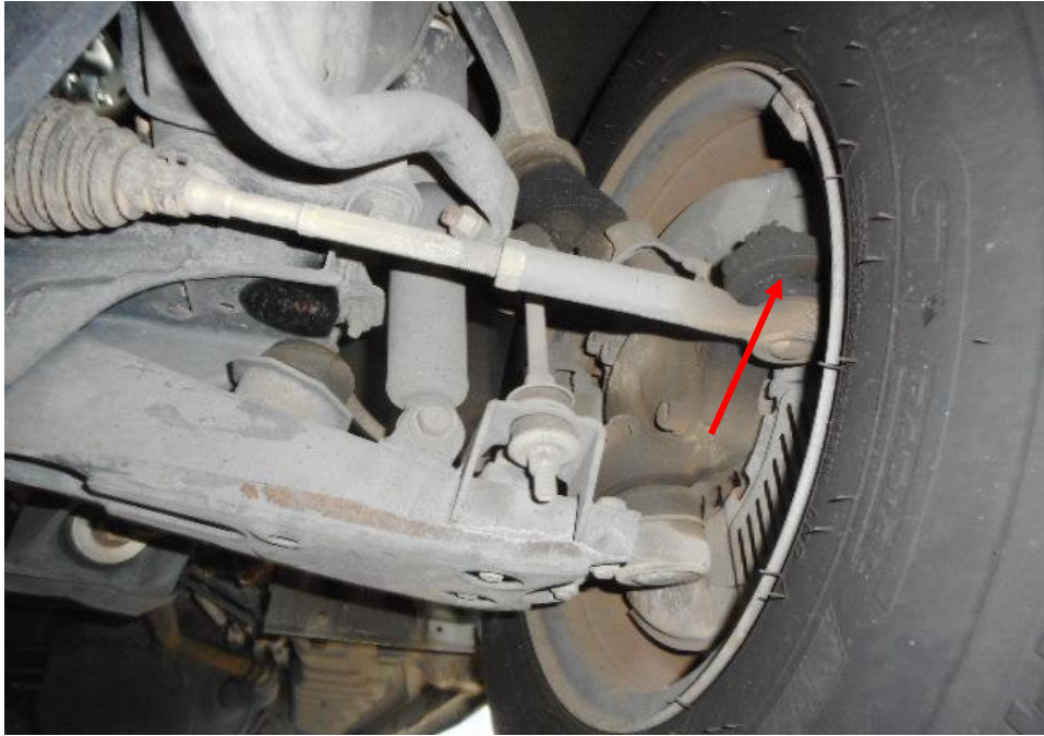
Photo 20 shows the various undercarriage components at the front left wheel of the Motor Van, in particular the steering tie rod end (arrowed). The various undercarriage components of the Motor Van were all found to be intact without any visible damage. There was also no sign of fluid stain(s) observed on the various undercarriage components.
