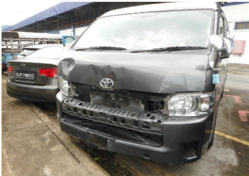
Photo 3 shows a general view of the Motor Van's frontal portion at the time of my inspection. It appeared to have sustained damage at its frontal portion. Its front body panel, front bumper, front bumper reinforcement and its engine radiator were also damage at the time of my inspection.
