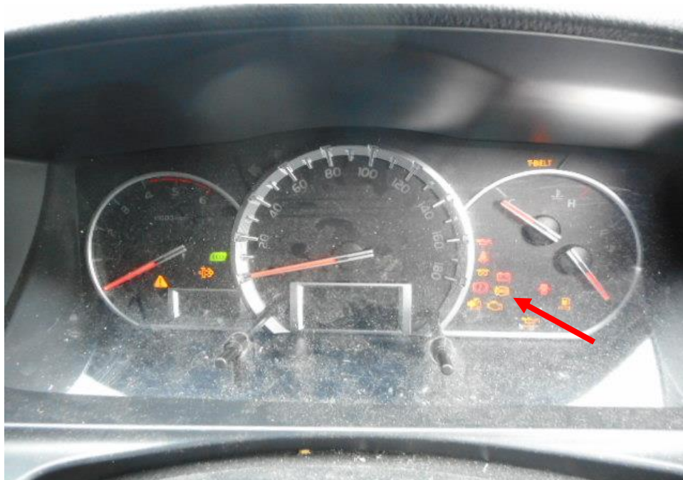
Photo 26 shows the warning light for Anti-Lock Brake System (ABS) (arrowed) appearing on the instrument panel of the Motor Van during the self-test of its various electronic operating systems when its engine was cranked.
