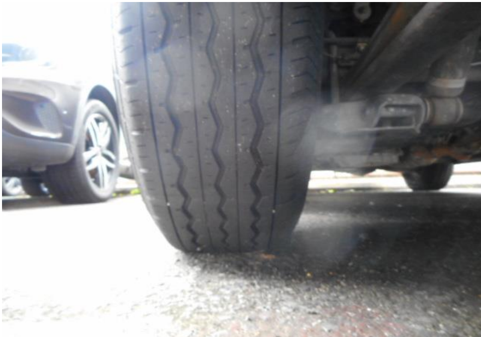
Photo 11 shows the condition of the rear left tyres of the Motor Van, which was observed to be in serviceable condition with remaining tread depth of approximately 4.3mm. The tyres, which were wrapped around standard steel wheel rim, were also observed to be sufficiently inflated for vehicular operation. There was also no damage found on all 4 steel wheel rims of the Motor Van.
