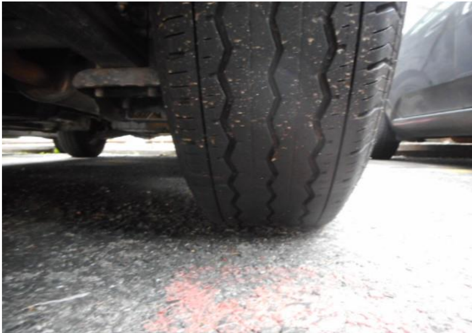
Photo 10 shows the condition of the rear right tyre of the Motor Van, which was observed to be in serviceable condition with remaining tread depth of approximately 3mm. The tyre, which was wrapped around standard steel wheel rim, it was observed to be sufficiently inflated for vehicular operation.
