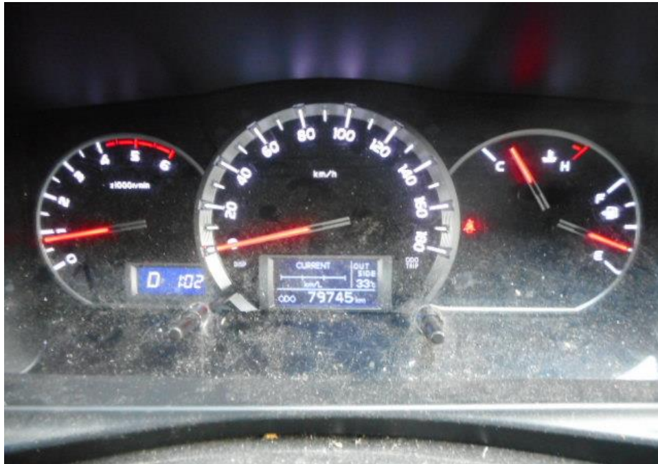
Photo 27 shows no warning lights illuminated on the instrument panel of the Motor Van after the engine was cranked. This would suggest that there was no abnormality to the electronic operating system of the Motor Van, like the ABS and etc.
