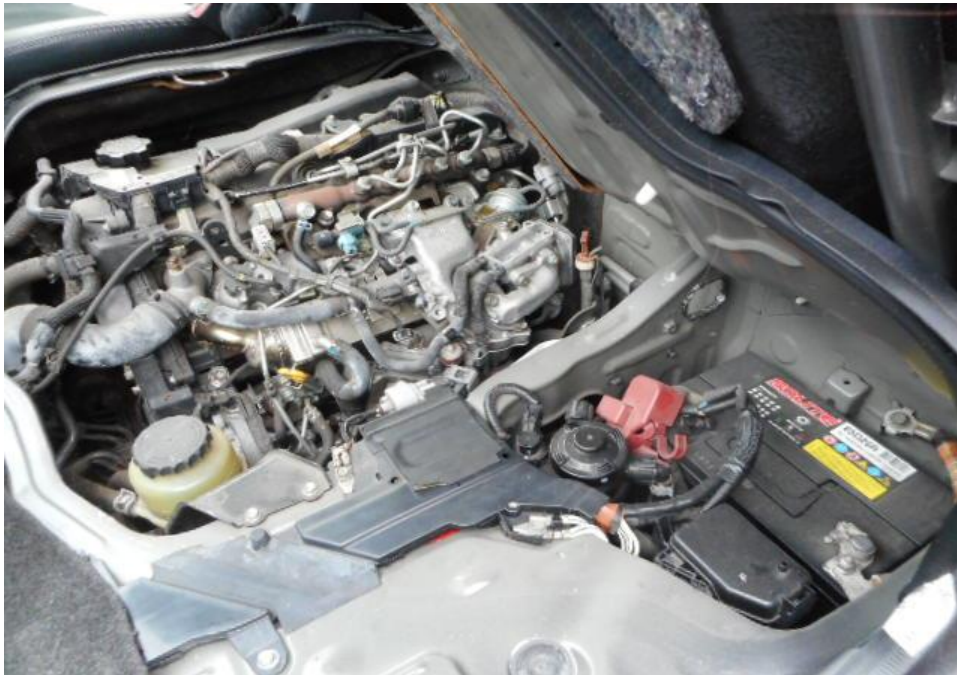
Photo 13 shows a general view of the Motor Van's engine compartment, which was accessed by lifting the front cabin of the Motor Van. I had observed the engine radiator and its engine coolant reservoir to be damaged by the accident. However, the other various parts and components inside the engine compartment were unaffected by the accident. There was also no sign(s) or indication(s) of fresh fluid leakage and/or fluid stain within the engine compartment.
