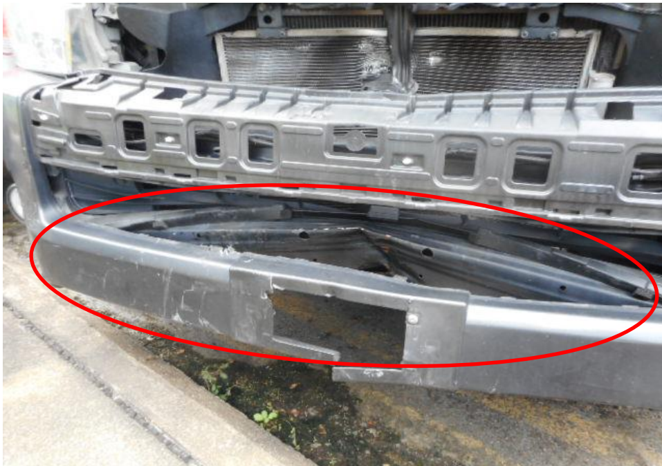
Photo 5 shows a close up view of the Motor Van's frontal portion at the time of my inspection. It appeared to have sustained damage at its frontal portion. Its front bumper and front bumper reinforcement (circled) was damage at the time of my inspection as a result of the accident.
