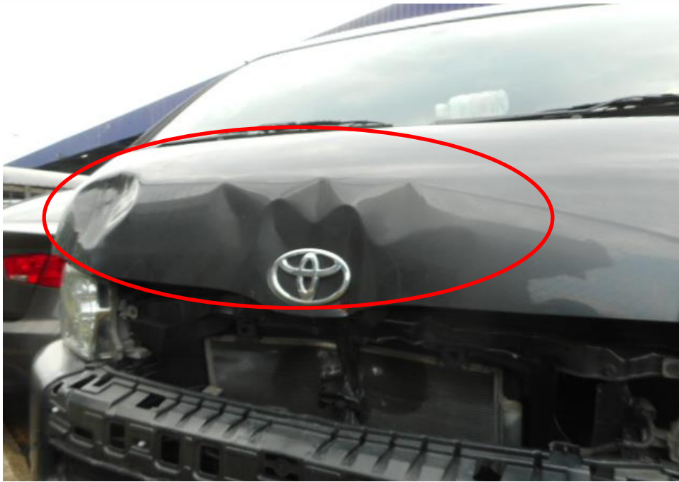
Photo 4 shows a close up view of the Motor Van's frontal portion at the time of my inspection. It appeared to have sustained damage at its frontal portion. Its front body panel (circled) was damage at the time of my inspection as a result of the accident.
