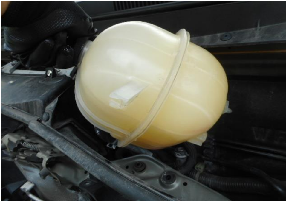
Photo 15 shows the engine coolant reservoir of the Motor Van at the time of my inspection. The engine coolant was observed to be of insufficient as the coolant reservoir was damaged as a result of the accident.
