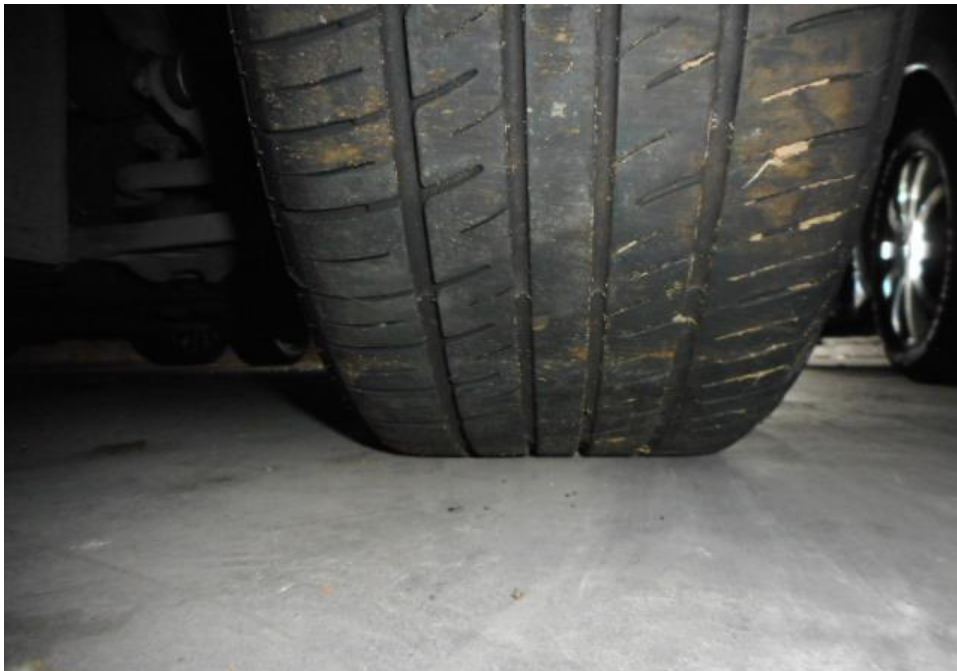
Photo 12 shows the condition of the front left tyre of the Motor Taxi, which was observed to be in serviceable condition with remaining tread depth of approximately 3.8mm. The tyre was also observed to be sufficiently inflated for vehicular operation with no tear, cut or burst mark(s).
