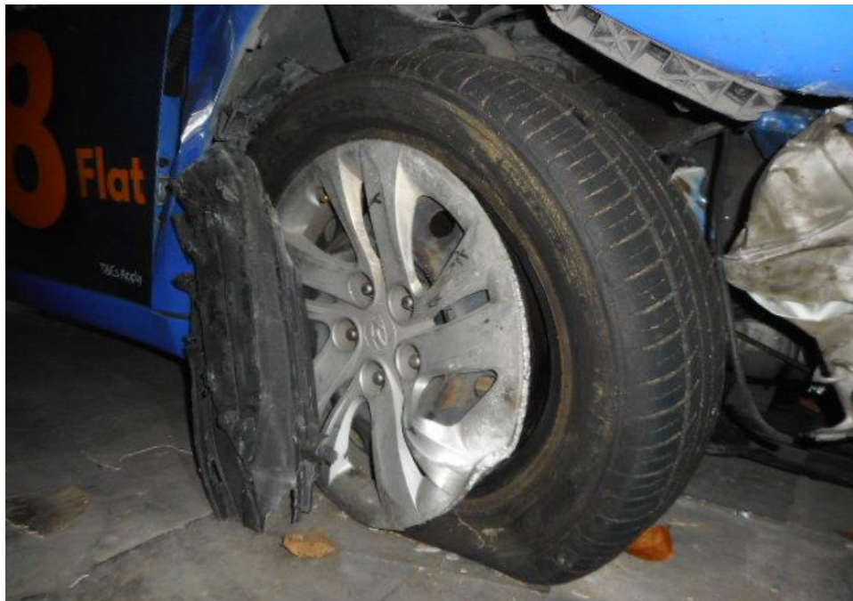
Photo 8 shows the condition of the front right tyre of the Motor Taxi, which was observed to be unserviceable condition with remaining tread depth of approximately 5mm. The tyre was observed with cut mark(s) on the inner sidewalls and there was damage observed on the wheel rims as a result of the accident.
