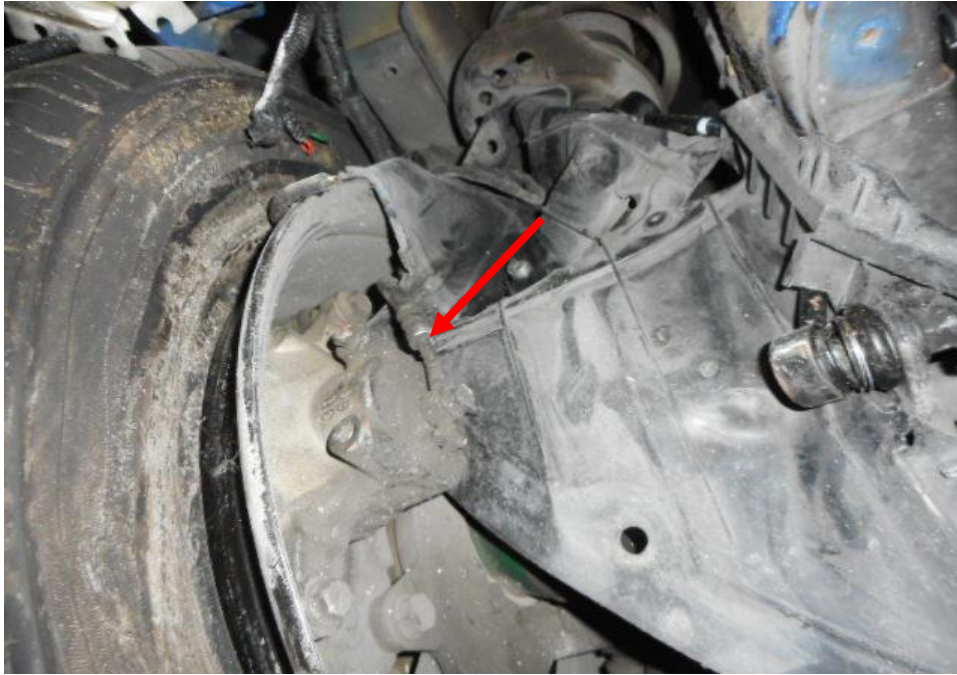
Photo 17 shows the brake hose/pipe (arrowed) at the front right wheel of the Motor Taxi. I did not observe any leakage of brake fluid at the time of my inspection of the Motor Taxi. The undercarriage components of the Motor Taxi were also all found to be intact and without any visible damage.
