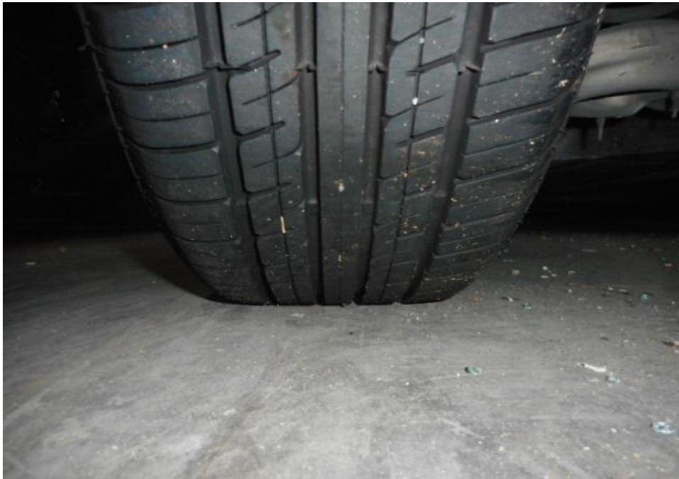
Photo 11 shows the condition of the rear left tyre of the Motor Taxi, which was observed to be in serviceable condition with remaining tread depth of approximately 7mm. The tyre was also observed to be sufficiently inflated for vehicular operation with no tear, cut or burst mark(s).
