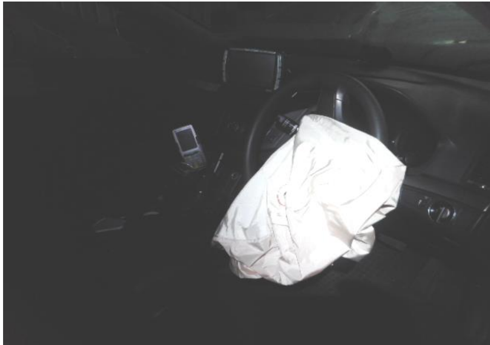
Photo 13 shows the deployment of the Supplemental Restraint System (SRS) airbag in the Motor Taxi as a result of the accident.
