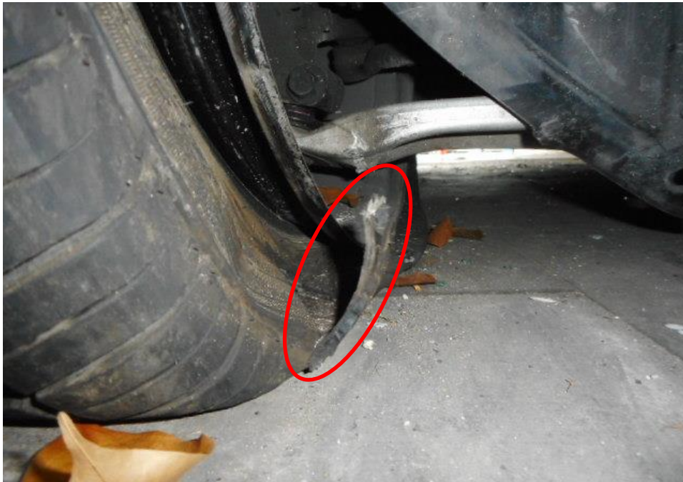
Photo 9 shows the close up view of the condition of the front right tyre of the Motor Taxi, which was observed to be unserviceable condition. The tyre was observed with cut mark(s) on the inner sidewalls and there was damage observed on the wheel rims (circled) as a result of the accident.
