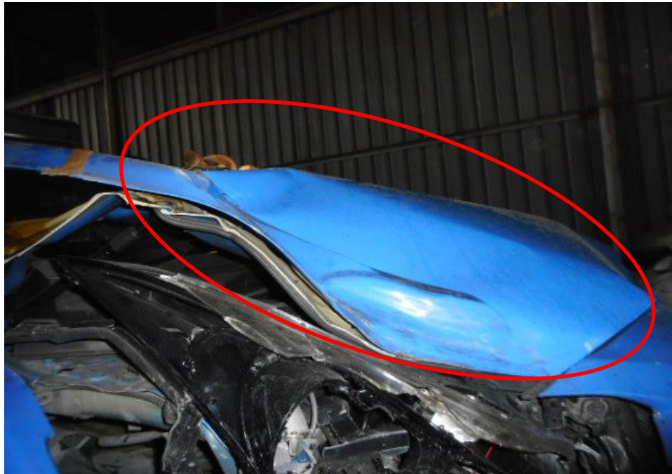
Photo 14 shows a close up view of the damaged front bonnet lock mechanism and the structure of the engine compartment of the Motor Taxi at the time of my inspection resulting it unable to open a result of the accident. (circled) (Unable to open)
