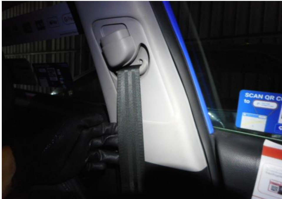
Photo 22 shows that the seat belt on the left seat was not worn at the material time of accident as the safety pre-tensioners was activated at the moment of impact and caused the seat belt to be locked into the last position.
