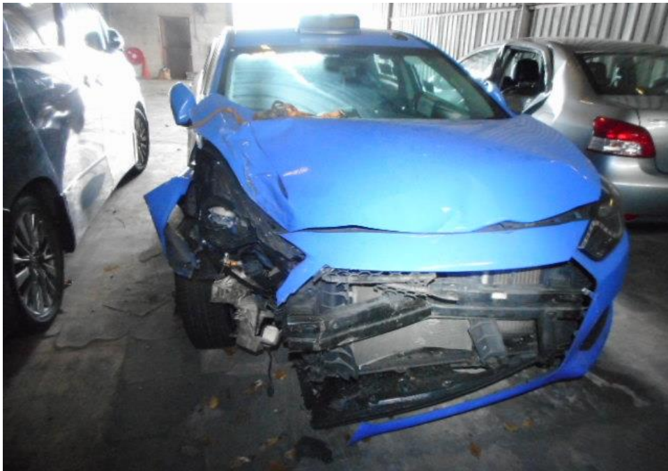
Photo 2 shows a general view of the Motor Taxi's front body at the time of my inspection. The Motor Taxi was observed to have sustained damage at its front portion. Its front bonnet, front bumper, front reinforcement panel, front right headlamp and front right fender were amongst the body parts that were damaged as a result of the accident. The Supplemental Restraint System (SRS) was activated as a result of the accident.
