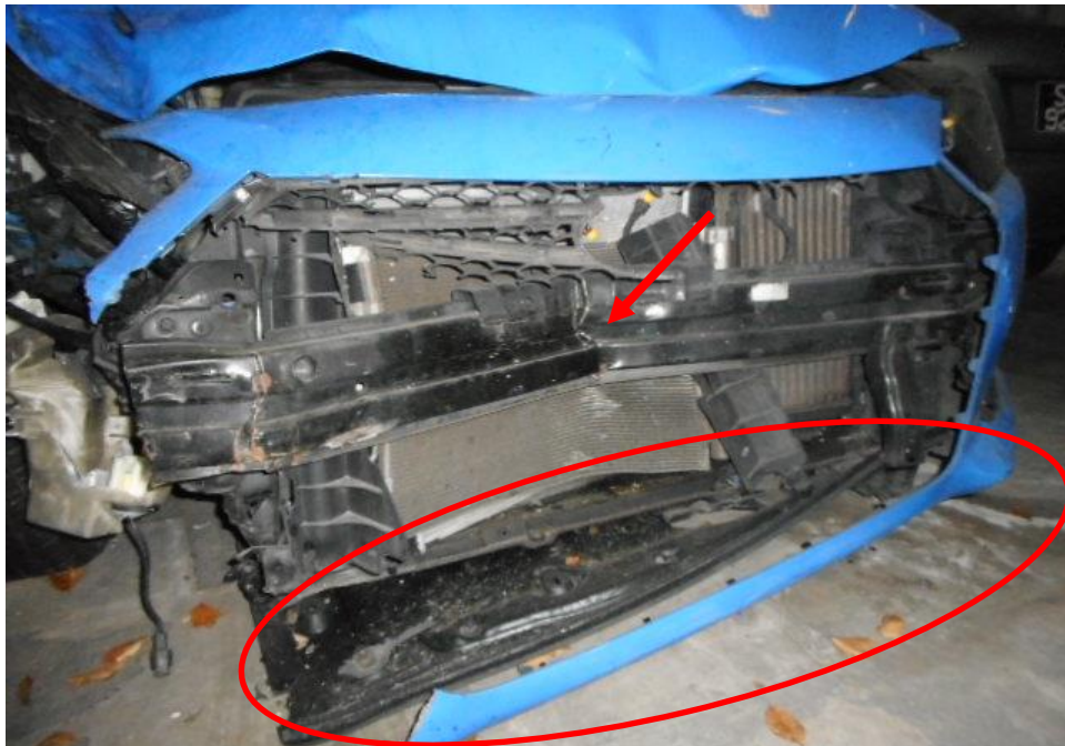
Photo 4 shows the close up view of the Motor Taxi's front body at the time of my inspection. The Motor Taxi was observed to have sustained damage at its front portion. Its front bumper (circled) and front reinforcement panel (arrowed) were amongst the body parts that were damaged as a result of the accident.
