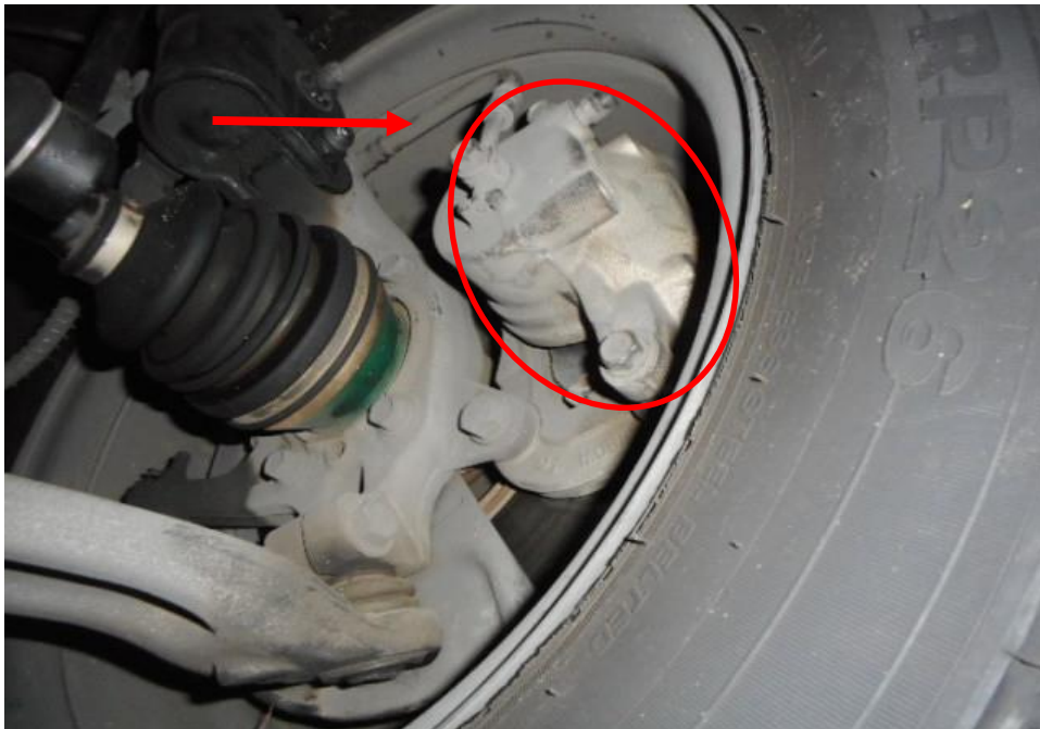
Photo 18 shows the brake hose/pipe (arrowed) at the front left wheel of the Motor Taxi. No leakage of brake fluid was observed. Visual examination of the various components of the braking system like the brake caliper (circled), brake booster, brake pedal etc had revealed all to be intact and without visible damage.
