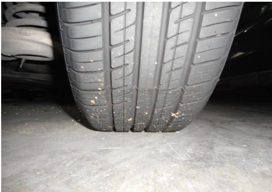
Photo 10 shows the condition of the rear right tyre of the Motor Taxi, which was observed to be in serviceable condition with remaining tread depth of approximately 6.7mm. The tyre was also observed to be sufficiently inflated for vehicular operation with no tear, cut or burst mark(s).
