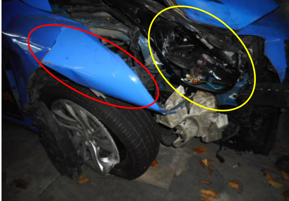
Photo 5 shows the close up view of the Motor Taxi's front body at the time of my inspection. The Motor Taxi was observed to have sustained damage at its front portion. Its front right fender (red circle) and front left headlamp (yellow circle) were amongst the body parts that were damaged as a result of the accident.
