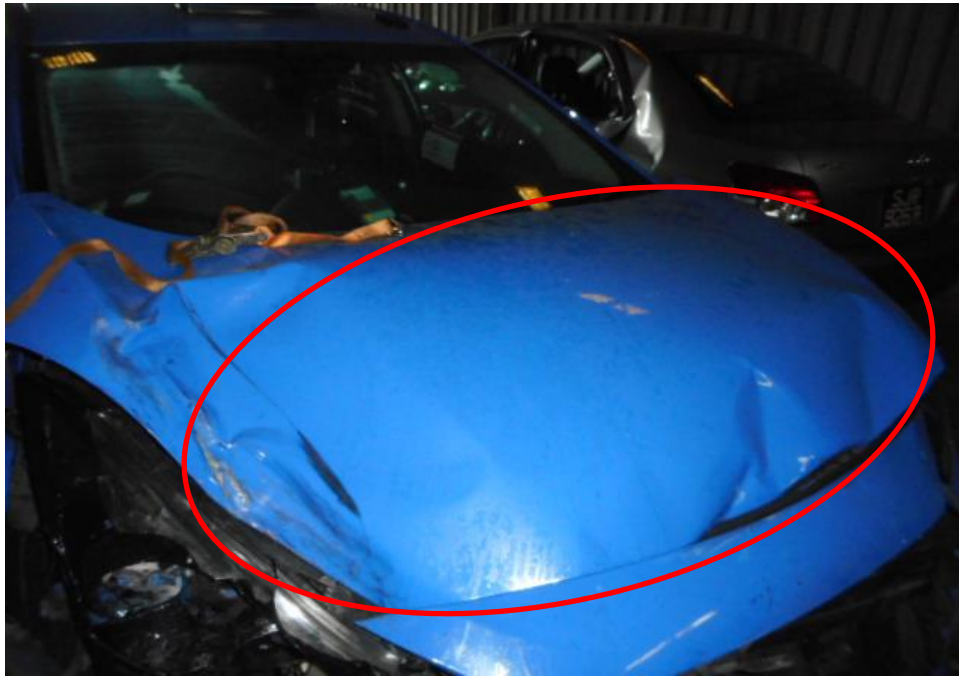
Photo 3 shows the close up view of the Motor Taxi's front body at the time of my inspection. The Motor Taxi was observed to have sustained damage at its front portion. Its front bonnet (circled) were amongst the body parts that were damaged as a result of the accident.
