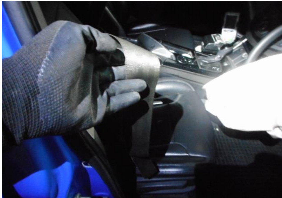
Photo 21 shows that the seat belt on the right seat was worn at the material time of accident as the safety pre-tensioners was activated at the moment of impact and caused the seat belt to be locked into the last position.
