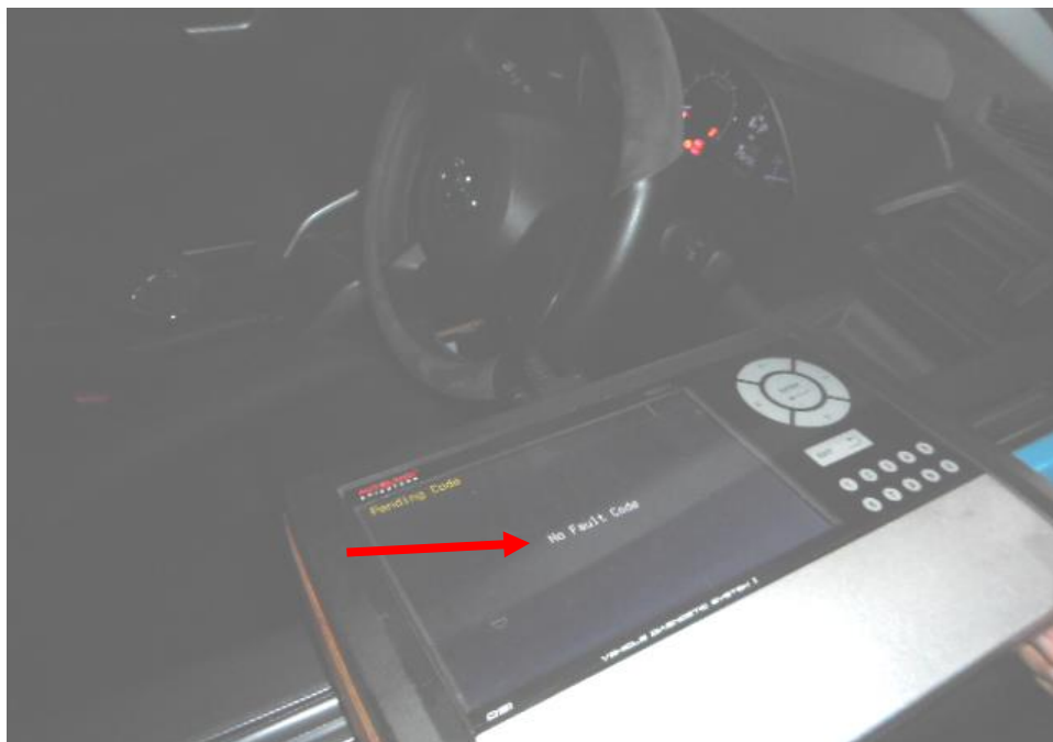
Photo 7 shows the conducted ECU diagnosis of the Insured Vehicle at the time of our inspection. There was no electronic error on the Insured Vehicle (arrowed).
