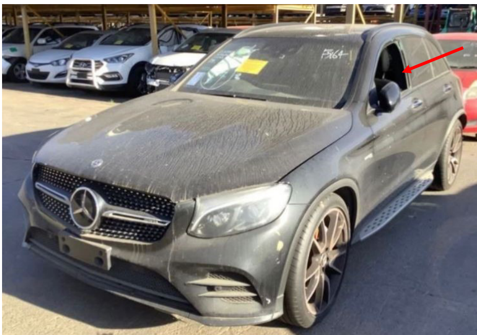
Photo 2 shows the front left body of the Motor Car prior to any repairs being carried out (photograph provided to me). No physical damage was observed to the Motor Car except for the front left passenger door window (arrowed), which was observed to be shattered.
