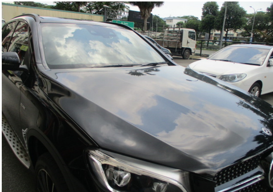
Photo 6 shows a closer view of the Motor Car's front bonnet, front windscreen and front right headlamp. In general, the Motor Car was observed to be in a relatively good general condition with no loose exterior fittings observed.
