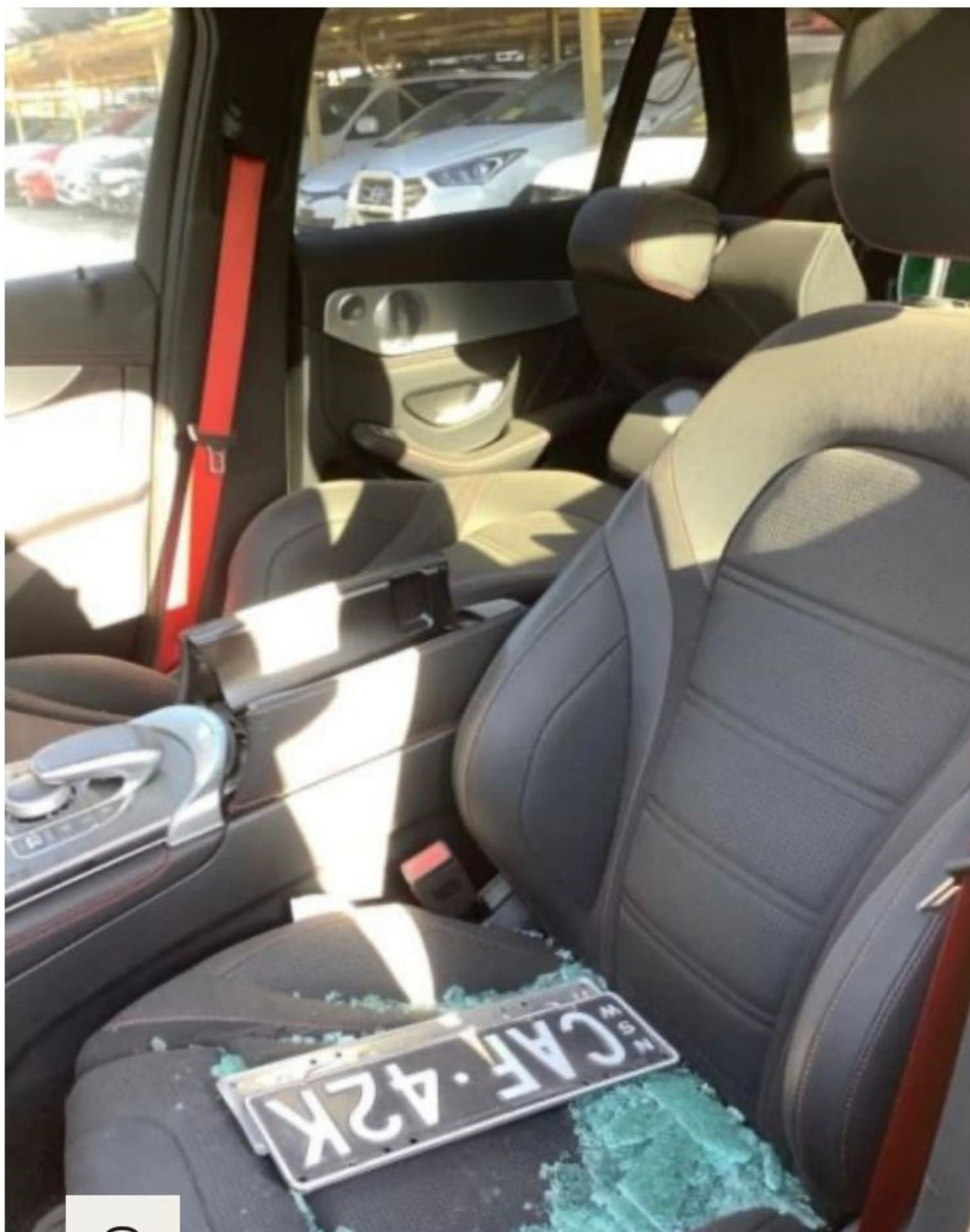
Photo 3 shows the interior compartment of the Motor Car prior to any repairs being carried out (photograph provided to me). The interior compartment was observed to be without any physical damage. The airbags of the Motor Car were not deployed as seen from the photographs that were provided to me. Broken glass fragments from the shattered front left passenger door window can be seen on the front left passenger seat of the Motor Car.
