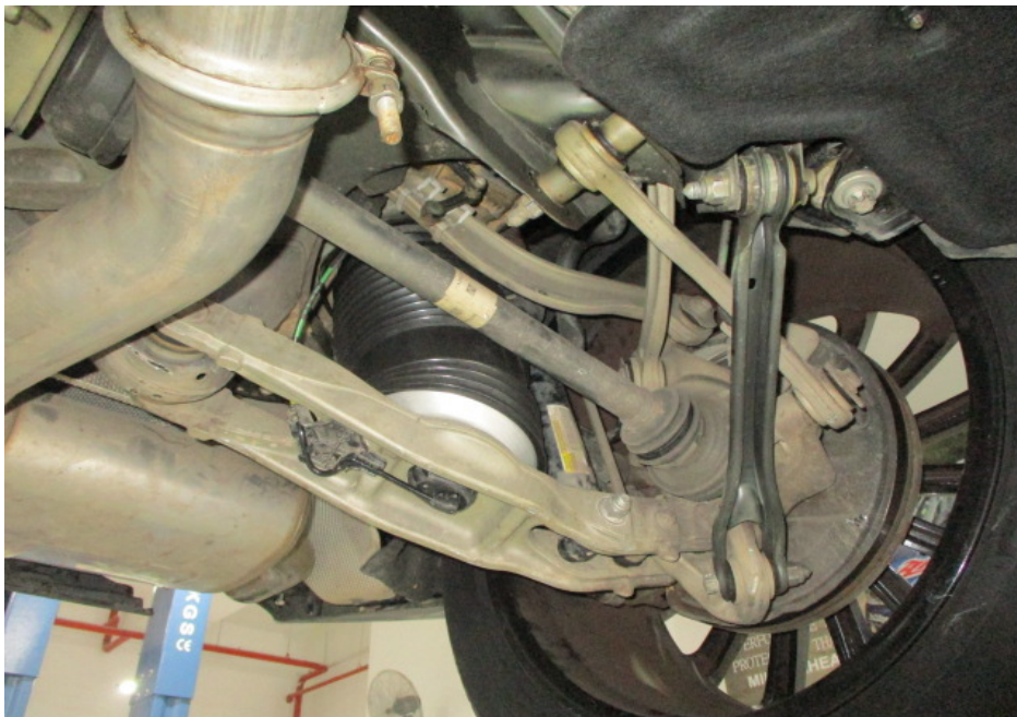
Photo 22 shows a general view of the control arms and linkages at the rear left wheel of the Motor Car. I did not observe any fluid leak and/or fluid stain on the underside of the Motor Car. All the Motor Car's undercarriage components were observed to be intact and secured in an appropriate manner.
