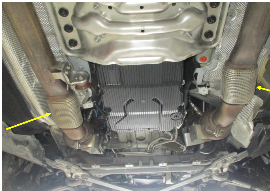
Photo 26 shows the front section of the Motor Car's exhaust system. My examination of the Motor Car's exhaust system revealed no sign(s) or indication(s) of any cut or weld marks along its exhaust pipes, on its centre resonator boxes, on its rear muffler and on its catalytic converters (arrowed).
