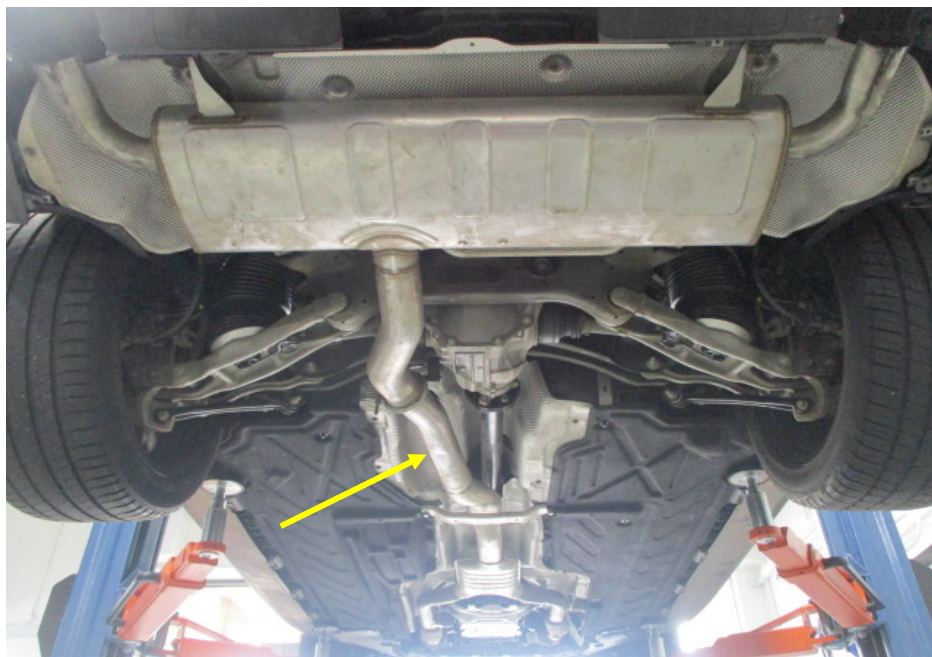
Photo 25 shows the rear section of the Motor Car's exhaust system. My examination of the Motor Car's exhaust system revealed no sign(s) or indication(s) of any cut or weld marks along its exhaust pipes (arrowed), on its centre resonator boxes, on its rear muffler and on its catalytic converters.
