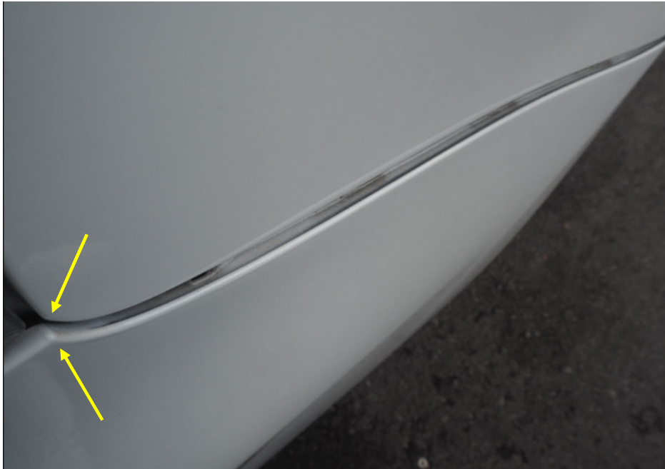
Photo 6 shows the right corner edge of the rear bumper of the Toyota. We observed that the rear bumper was dislodged at the right corner edge (arrowed).
