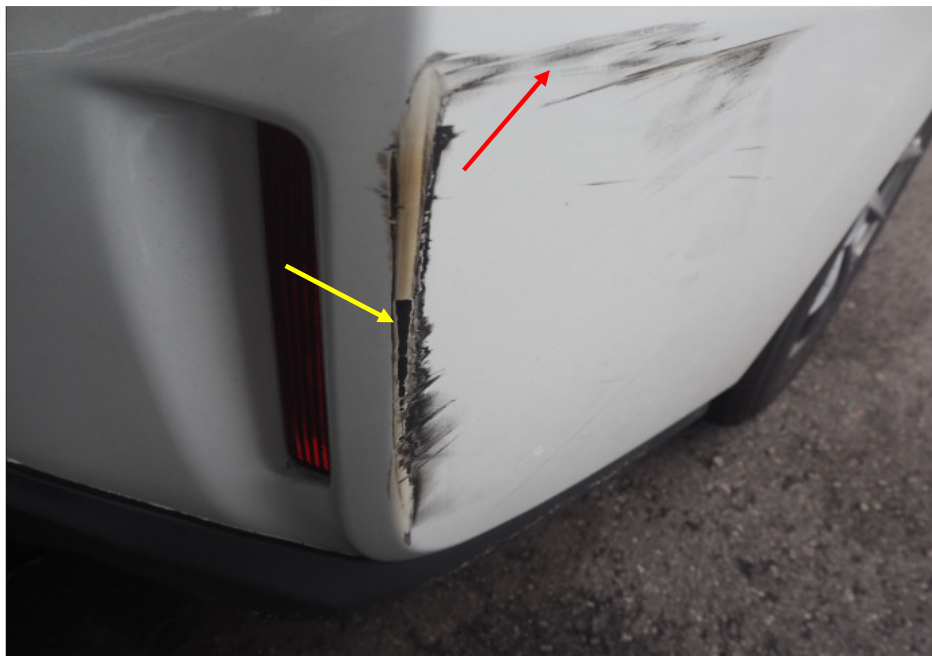
Photo 3 shows a closer view of the paint graze marks (yellow arrow) and black marks (red arrow) found on the lower right portion of the rear bumper of the Toyota.
