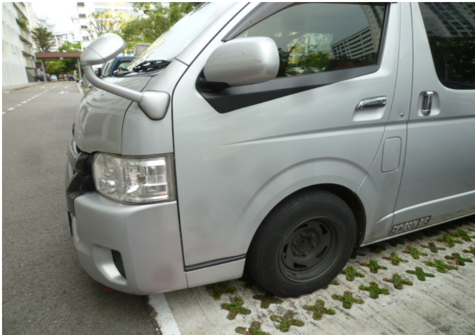
Photo 11 shows a closer view of the left frontal portion of the Hiace at the time of our physical inspection. There were no cracks or dents observed.
