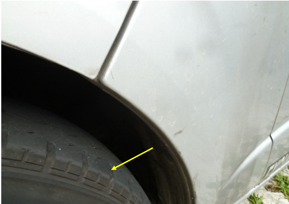
Photo 13 shows a close up view of the left front tyre of the Hiace at the time of our physical inspection. We observed that the left front tyre was observed to have protruded out from the body of the Hiace (arrowed).
