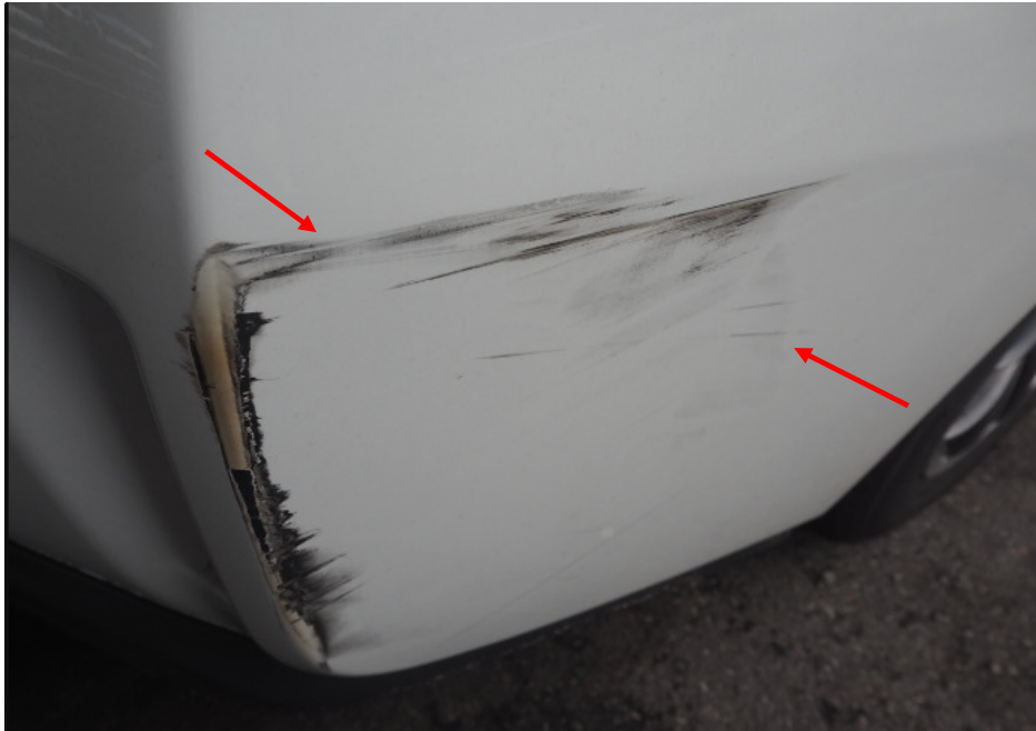
Photo 4 shows a close up view of the black marks found on the lower right portion of the rear bumper of the Toyota (arrowed).
