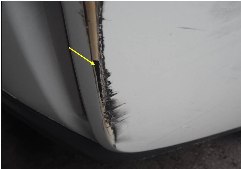
Photo 5 shows a close up view of the paint graze marks found on the lower right portion of the rear bumper of the Toyota (arrowed).
