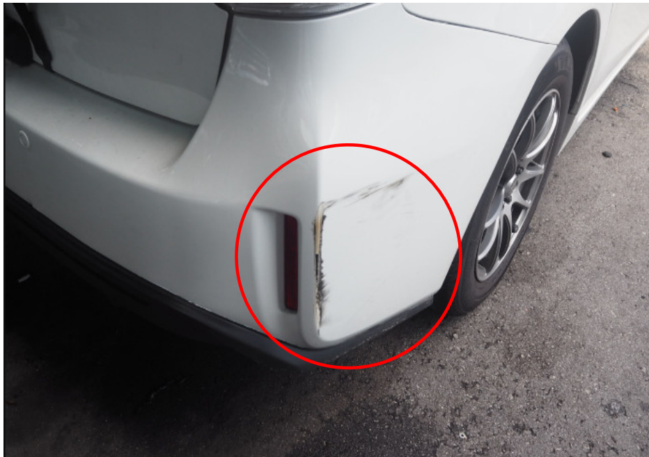
Photo 2 shows the damage observed on the right portion of the rear bumper of the Toyota (circled).
