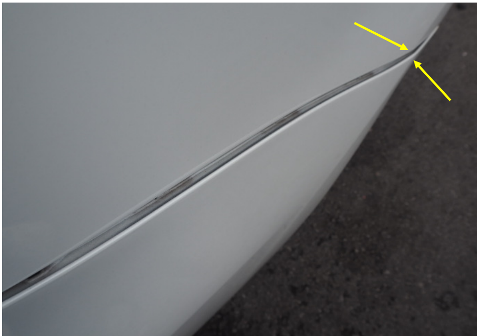
Photo 7 shows a close up view of the right corner edge of the rear bumper of the Toyota. We observed that the rear bumper was dislodged at the right corner edge (arrowed).
