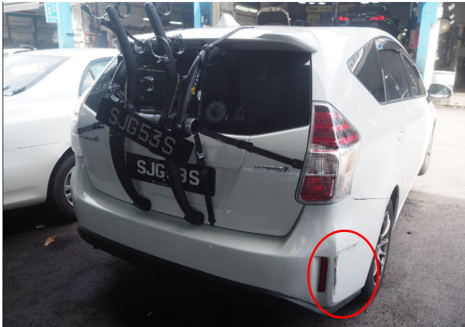
Photo 1 shows the general view of the right rear portion of the Toyota at the time of the Pre- Repair Survey conducted by LKK Auto Consultants Pte. Ltd. which was taken about 3 weeks after the accident. The damage to the Toyota was observed to be confined to the rear bumper (circled).
