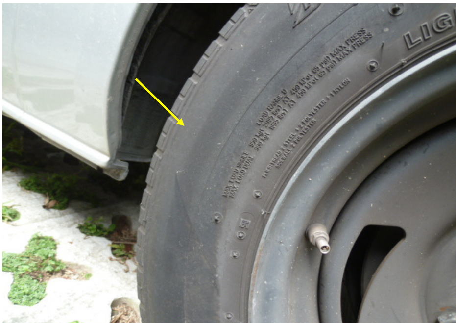
Photo 16 shows a close up view of the left front tyre of the Hiace at the time of our physical inspection. We observed that the left front tyre was observed to have protruded out from the body of the Hiace (arrowed).
