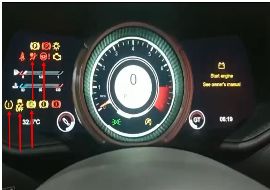
Photo 20 shows the warning lights for the various electronic safety features appearing on the instrument panel of the Motor Car during its self-test when the engine is cranked, in particular the ABS, SRS, PSS, TPM and TCS lights (arrowed).
