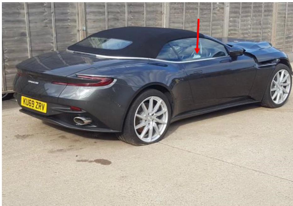
Photo 3 shows the rear right body of the Motor Car (photograph provided to me). Apart for the frontal portion, there was no physical damage seen to other areas of the Motor Car. The driver's airbag (arrowed) was deployed.
