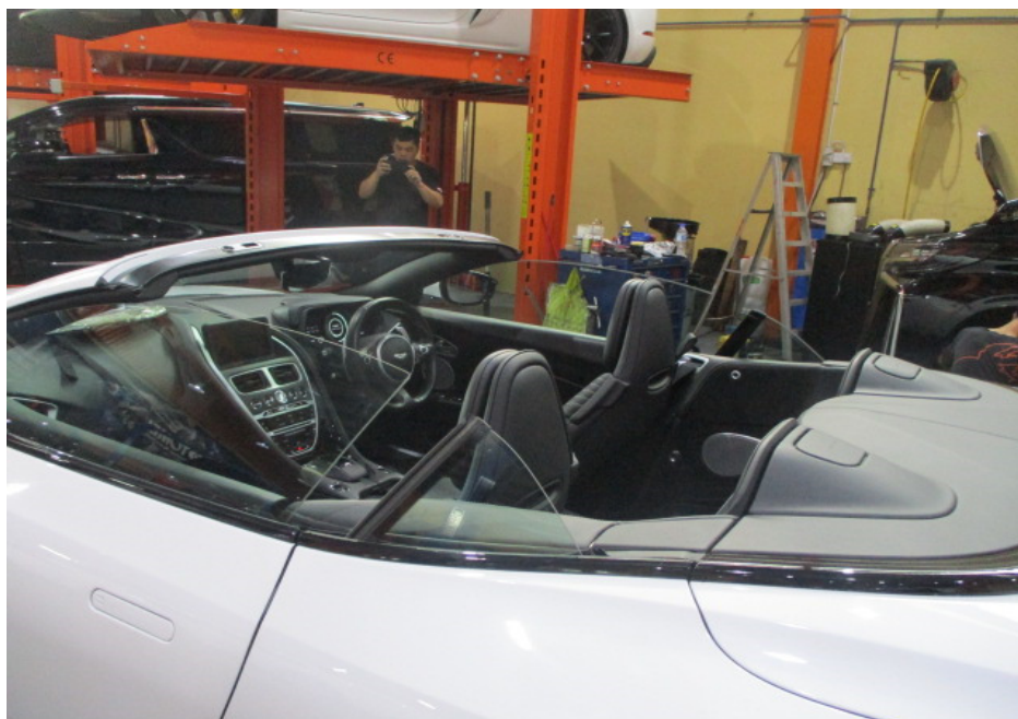
Photo 14 shows the Motor Car with its soft top in a completely opened position. It was observed that as a safety feature, the soft top could only open and close when the Motor Car was in a stationary position. When opened, the soft top is completely folded into the rear storage compartment with no parts protruding out of the Motor Car's body. The soft top was also found adequately secured to the "A" pillar after closing.
