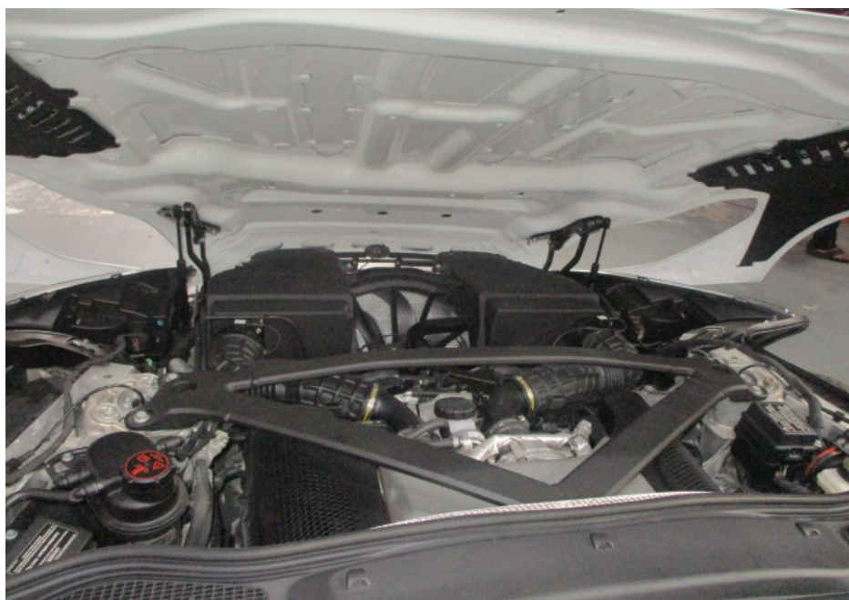
Photo 16 shows a general view of the engine compartment of the Motor Car at the time of my inspection. The various parts and components inside the engine compartment were all observed to be intact and properly fitted. There was also no sign(s) or indication(s) of fluid leak and/or fluid stain found inside the engine compartment. The repair/restoration works carried out to the various parts within the engine compartment like the aircon condenser, radiator, cooling fan, air intake boxes and front support panel amongst others were reasonably adequate and in order.
