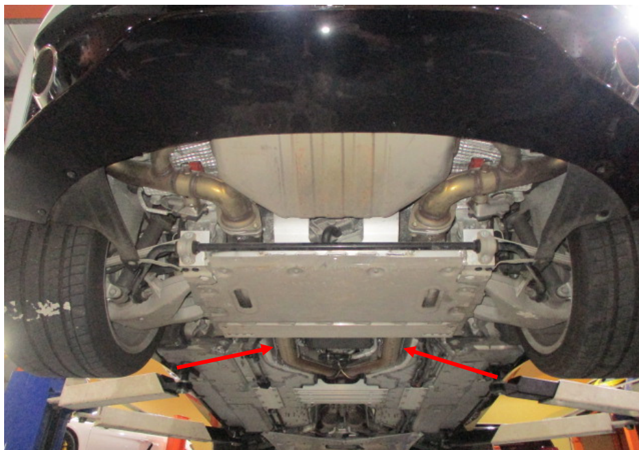
Photo 27 shows the rear section of the Motor Car's exhaust system. My examination of the Motor Car's exhaust system revealed no sign(s) or indication(s) of any cut or weld marks along its exhaust pipes (arrowed), on its centre resonator boxes, on its rear mufflers and on its catalytic converters.
