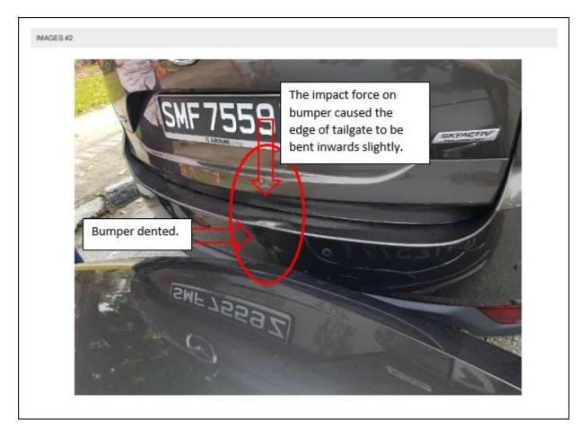
The rear bumper badly dented due to impact force caused by your vehicle, and you can look at rear bumper lower black area deformed which is Matt black colour and it cannot be spray painting and need to be replaced. In view of the nature bumper which is made of plastic material, it is not possible to restore back to pre-accident condition based on damage profile.
