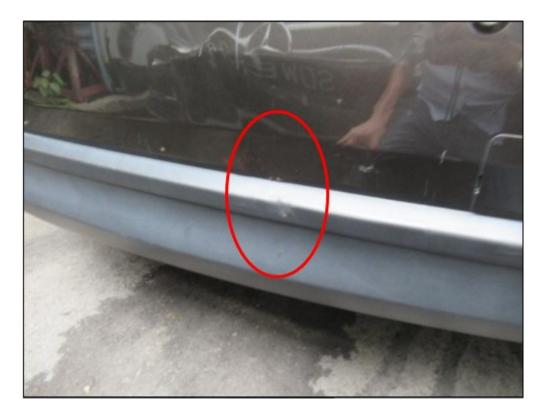
As for the reverse sensor which is fitted at the rear bumper, the impact caused short circuit to the sensor. Our surveyor who conducted inspection had tested the rear reverse sensor and confirmed that the sensor was intermittent malfunction. Thus, it needs to be replaced.
