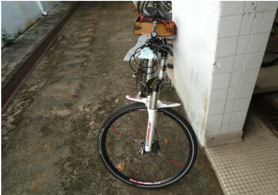
Photo 17 shows the front wheel of the Bicycle turned towards its full right. Turning the Bicycle's handle bar towards the right did not produce any abnormal free play and/or resistance. This would indicate that the steering system of the Bicycle was in serviceable condition at the time of our inspection.
