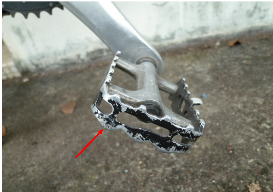
Photo 8 shows the damages of grazing nature on the right pedal of the Bicycle at the time of our inspection.
