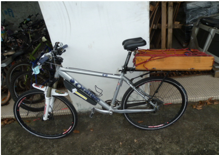
Photo 4 shows the left body of the Bicycle at time of our inspection. The Bicycle had sustained damages all around. The body parts that were found to have been damaged include its right hand brake lever, right handlebar grip, left fork stem, right pedal, left rear frame and rack, amongst others as a result of the accident.
