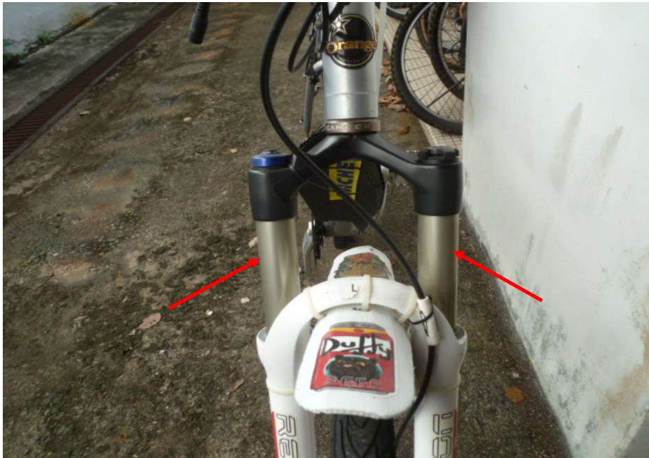
Photo 16 shows the front fork assembly (arrowed) of the Bicycle. The front forks and fork bracket of the Bicycle were both found to be intact and undamaged. Turning the Bicycle's handle bar towards the left and right did not produce any abnormal free play. The steering system of the Bicycle was in serviceable condition at the time of our inspection.
