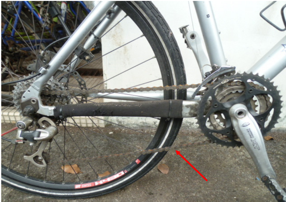
Photo 14 shows the general view of the gear train of the Bicycle, which was observed to be intact with no misalignment (arrowed). It was also adequately lubricated for operating purposes.
