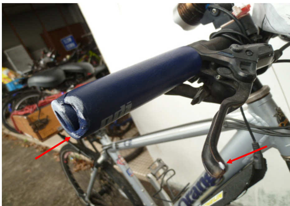
Photo 6 shows the damaged right hand brake lever and right handlebar grip (arrowed) of the Bicycle at the time of our inspection.
