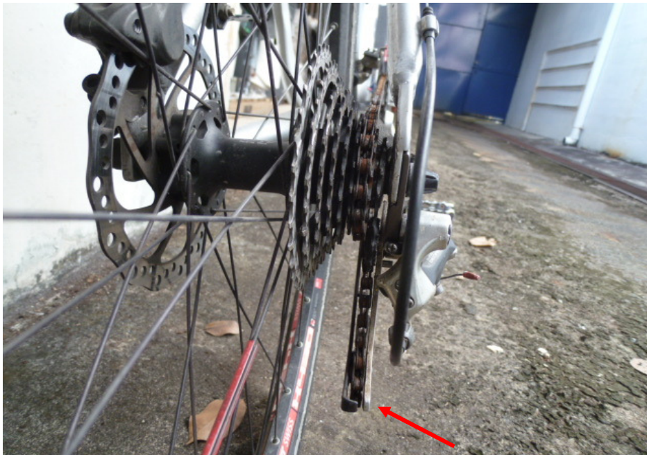
Photo 15 shows a closer view of the gear train of the Bicycle, which was observed to be intact with no misalignment (arrowed). It was also adequately lubricated for operating purposes.
