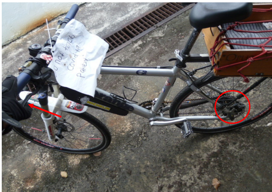
Photo 21 shows a static brake test conducted on the Bicycle's rear brake. There was some resistance felt upon pressing the right hand brake lever (arrowed). It also shows that the rear brake pads responded to the gripping action (circled) after depressing the right hand brake lever.
