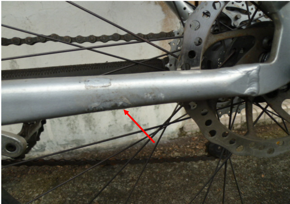
Photo 9 shows the damages of grazing nature on the left rear frame of the Bicycle at the time of our inspection (arrowed).
