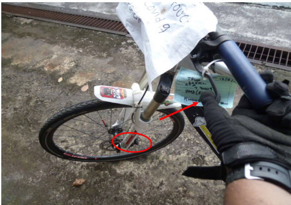
Photo 19 shows a static brake test conducted on the Bicycle's front brake. There was some resistance felt upon pressing the left hand brake lever (arrowed). It also shows that the front brake pads responded to the gripping action (circled) after depressing the right hand brake lever.
