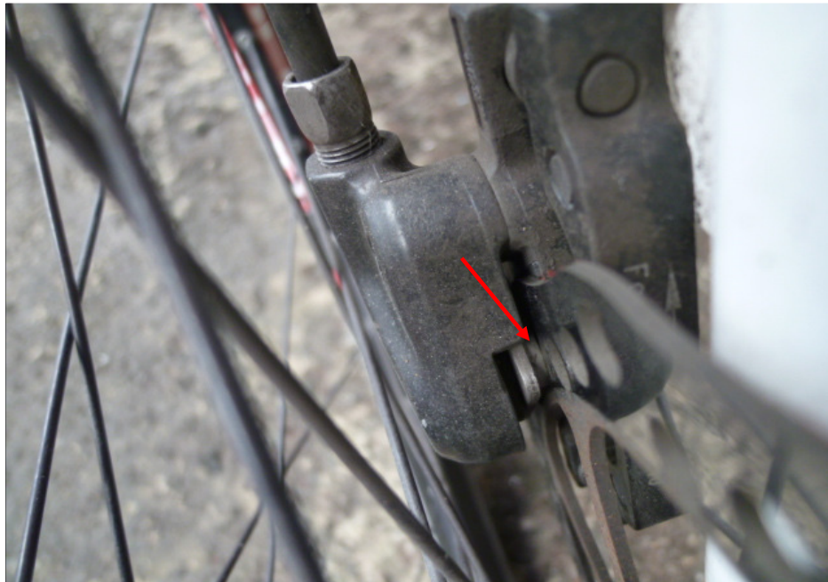
Photo 20 shows a close up view of the front brake pads responding to the gripping action. The front brake pads pressed against the front brake disc (arrowed) upon depressing the left hand brake lever. This had appeared to indicate that the front brake of the Bicycle was in serviceable condition.
