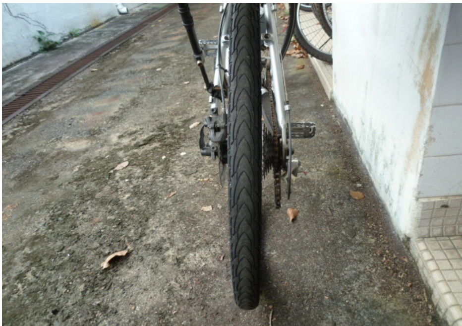
Photo 12 shows the rear tyre of the Bicycle. The pattern of the tread was clearly visible. There was no tear, burst mark(s) and/or punctured hole(s) on the sidewalls as well as across the tread of the front tyre. However the rear tyre was observed to be deflated.
