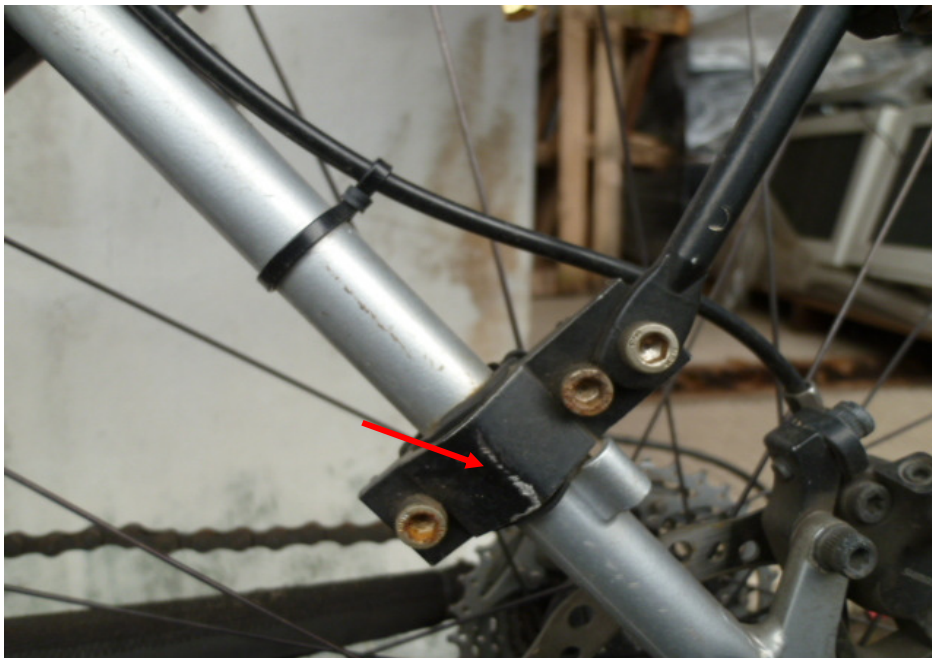
Photo 10 shows a close-up view of the damages of grazing nature on the rack (arrowed) of the Bicycle as a result of the accident.
