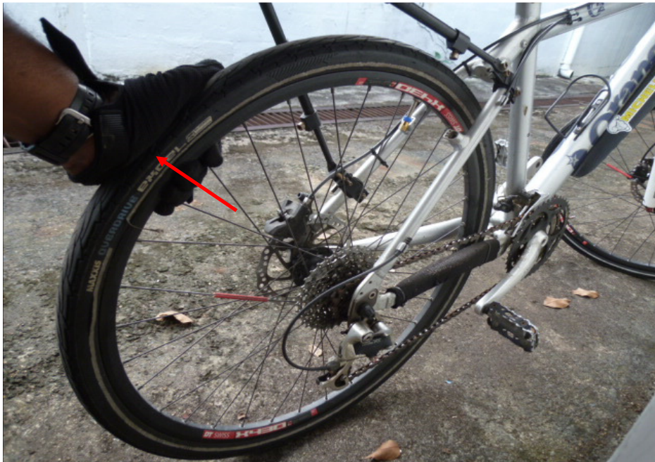
Photo 13 shows the deflated rear tyre of the Bicycle (arrowed).
