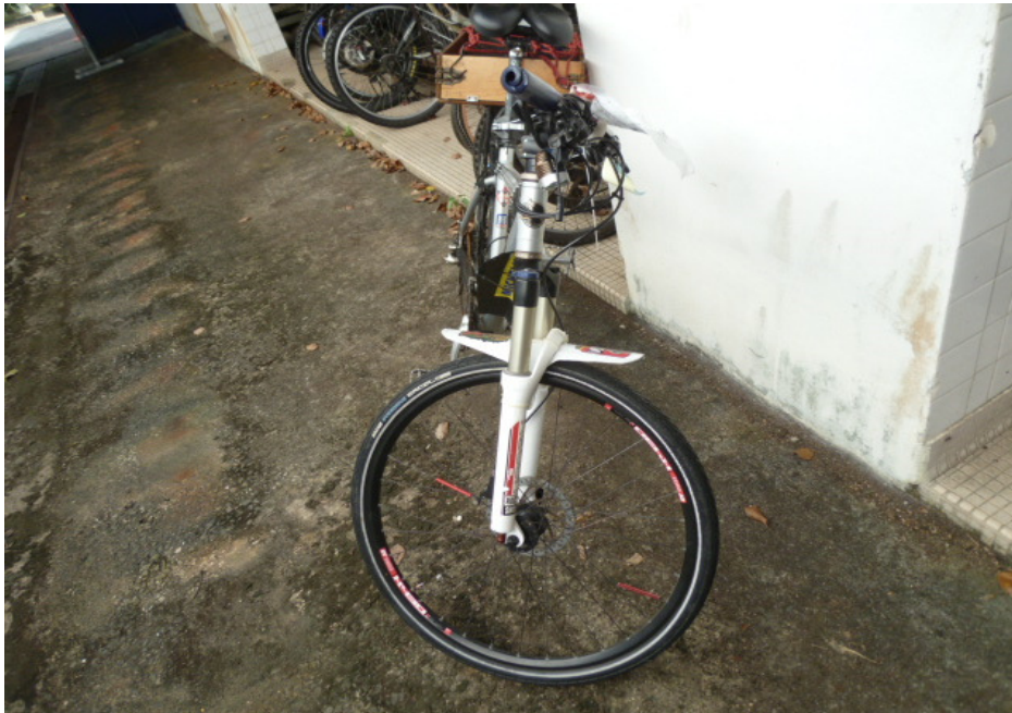
Photo 18 shows the front wheel of the Bicycle turned towards its full left. Turning the Bicycle's handle bar towards the left did not produce any abnormal free play and/or resistance. This would indicate that the steering system of the Bicycle was in serviceable condition at the time of our inspection.
