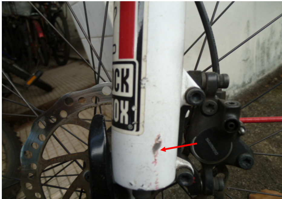
Photo 7 shows the damages of grazing nature on the left fork stem (arrowed) of the Bicycle at the time of our inspection.
