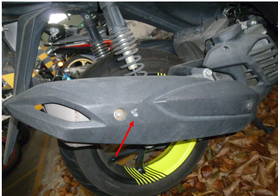
Photo 12 shows a closer view of the grazed exhaust muffler heat shield of the Motorcycle at the time of our inspection (arrowed).
