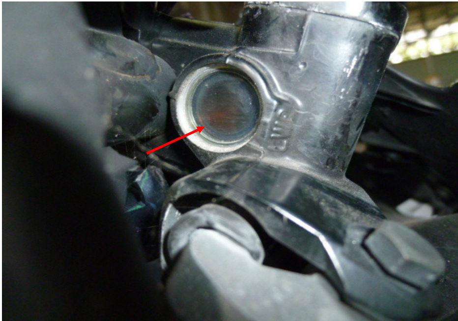
Photo 26 shows the brake fluid reservoir for the front brake of the Motorcycle. The brake fluid was observed to be of sufficient level for operational purposes and without any contamination (arrowed).
