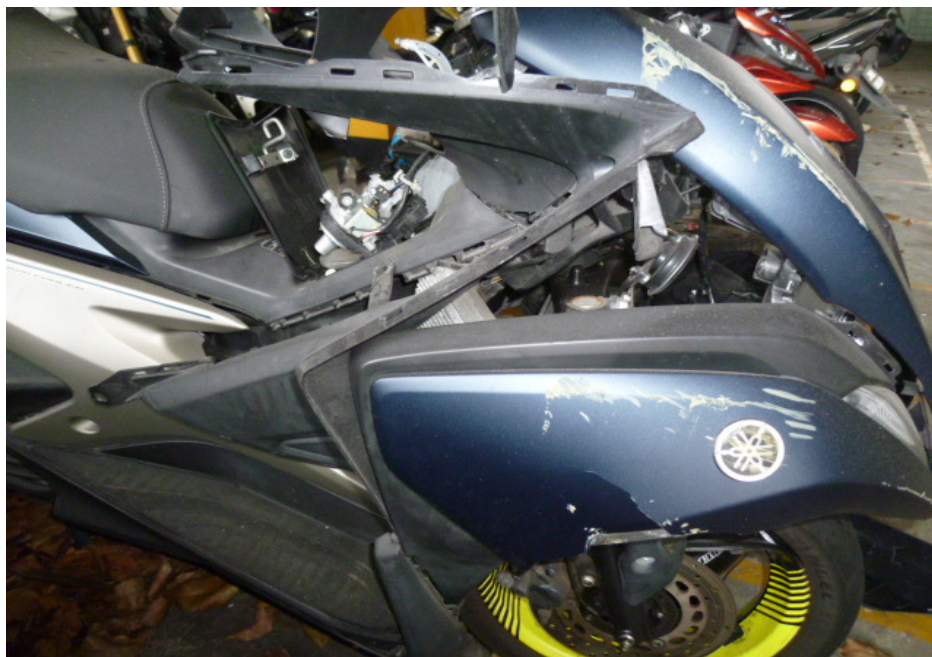
Photo 9 shows the broken right side cowling of the Motorcycle as a result of the accident.
