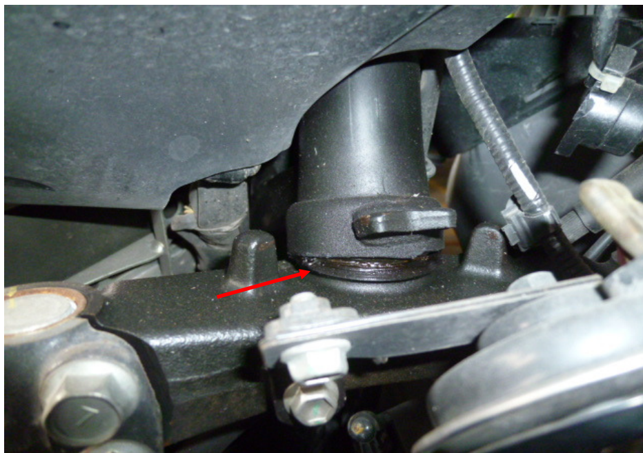
Photo 24 shows the steering stem of the Motorcycle. The steering stem observed to be bent (arrowed) as a result of the accident. We were hence not able to conduct any tests on the steering system of the Motorcycle.
