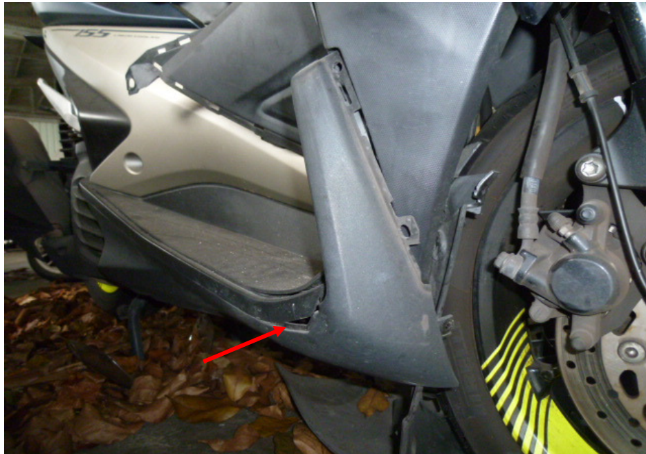
Photo 11 shows a closer view of the cracked right bottom side cowling of the Motorcycle as a result of the accident (arrowed).
