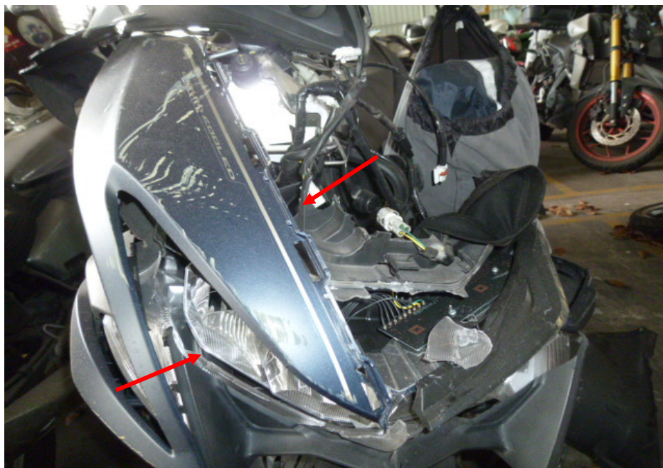
Photo 8 shows a closer view of the cracked headlight assembly and front cowling of the Motorcycle which were observed to be damaged due to the accident (arrowed).
