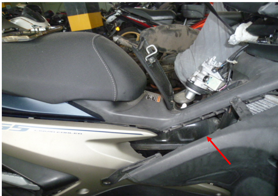
Photo 13 shows a closer view of the deformed right side cover of the Motorcycle at the time of our inspection (arrowed).
