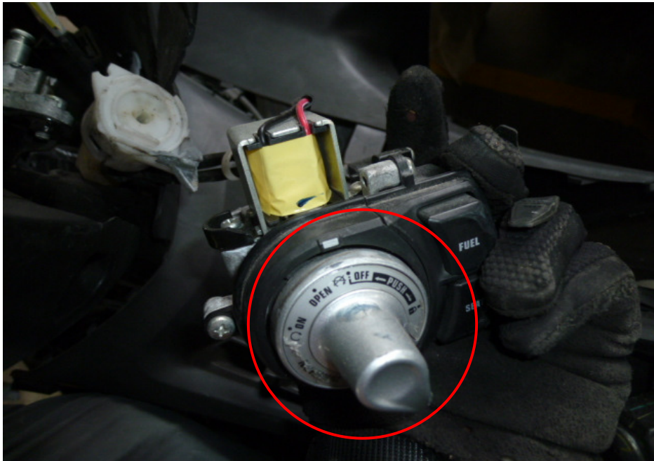
Photo 1 shows the broken ignition of the Motorcycle as a result of the accident (circled).
