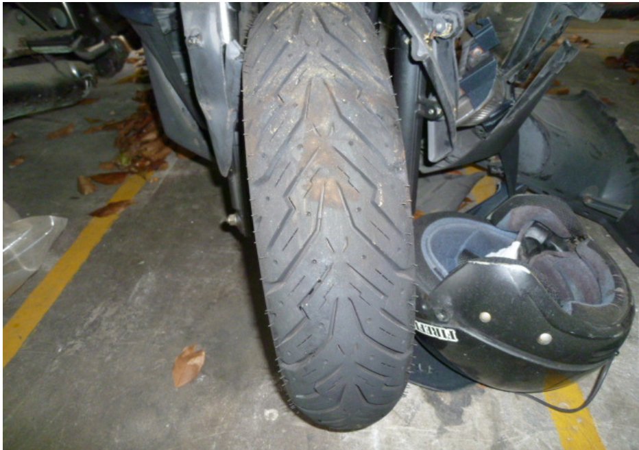
Photo 15 shows the condition of the Motorcycle's front tyre. The front tyre was observed to be in serviceable condition with remaining tread depth of approximately 8mm. There was no tear, burst mark(s) and/or punctured hole(s) on the sidewalls as well as across the tread of the front tyre. However the front tyre was observed to be deflated.
