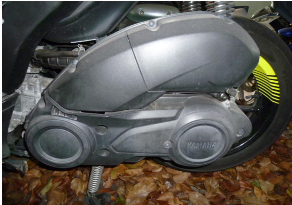
Photo 19 shows the drive train cover of the Motorcycle which was found to be intact without any misalignment.
