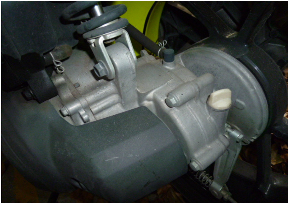
Photo 20 shows the drive train of the Motorcycle which was found to be intact without any misalignment.
