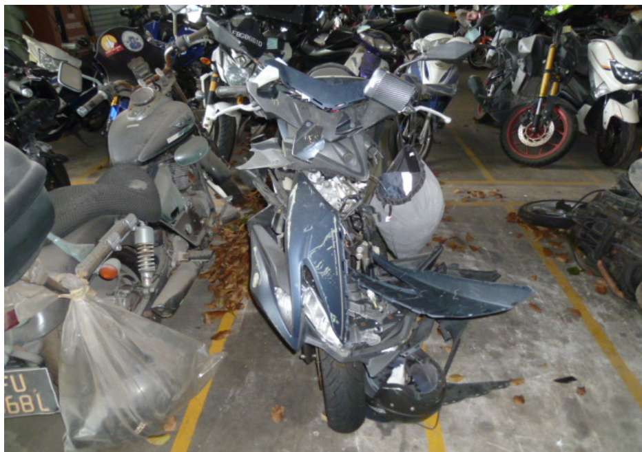
Photo 5 shows a general view of the frontal portion of the Motorcycle at the time of our inspection. The Motorcycle was observed to have sustained damages all around. The body parts that were found to have been damaged include its windshield, headlight assembly, head cowl, front cowl, front mudguard, front fork assembly, front wheel rim, ignition, side cowlings, right bottom side cowl, right side cover, left rear side cover and exhaust muffler heat shield, amongst others as a result of the accident.
