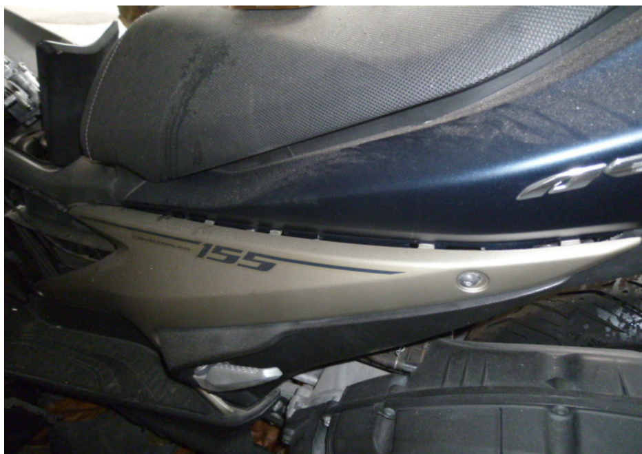
Photo 14 shows a closer view of the deformed left rear side cover of the Motorcycle as a result of the accident (circled).
