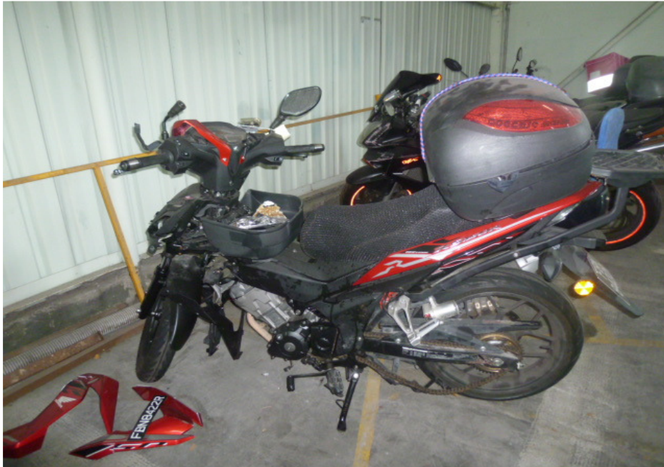
Photo 3 shows a general view of the left body of the Motorcycle at the time of our inspection. The Motorcycle had sustained damages all around. Body parts that were found to have been damaged include its headlight assembly, head cowling, front cowling, side cowlings, front mudguard, left side mirror, left handlebar end, clutch lever, front basket, radiator, left rear side cover, rear brake pedal, right front footrest and top box rack, amongst others.
