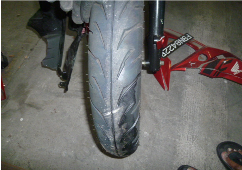
Photo 15 shows the condition of the Motorcycle's front tyre. The front tyre was observed to be in serviceable condition with remaining tread depth of approximately 4mm. We did not observe any tear, burst mark(s) and/or punctured hole(s) on the sidewalls as well as across the tread of the front tyre. The front tyre was also observed to be sufficiently inflated for vehicular operation.
