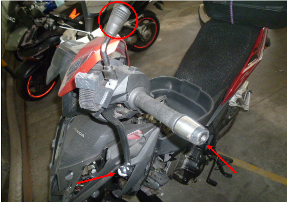
Photo 7 shows a close up view of the missing left side mirror (circled) as well as the clutch lever and left handlebar end (arrowed) of the Motorcycle. These parts were amongst the body parts of the Motorcycle which were damaged as a result of the accident.
