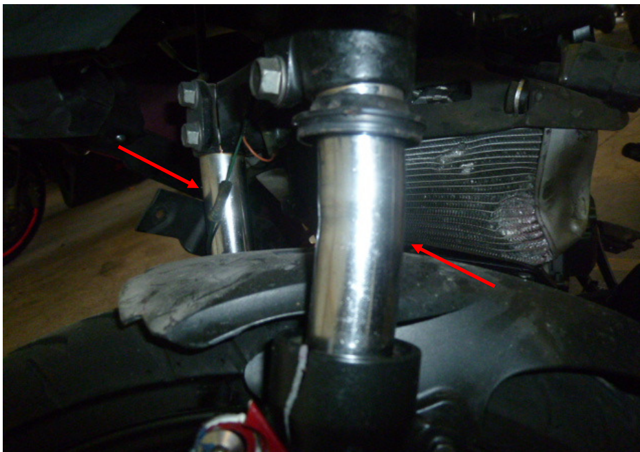
Photo 21 shows the front fork assembly of the Motorcycle. The front forks (arrowed) were observed to be bent inwards as a result of the accident. We were hence not able to conduct any tests on the steering system of the Motorcycle.
