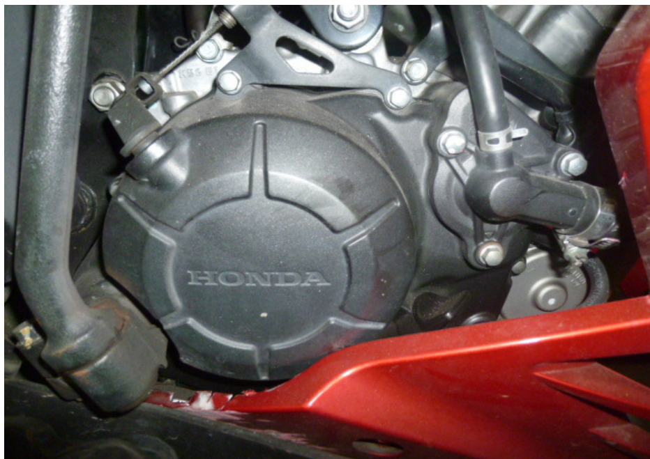
Photo 17 shows the right side of the engine of the Motorcycle at the time of our inspection. The various engine related parts and components were found to be intact with no visible damage. There was also no sign(s) or indication(s) of fluid leak observed around the right engine area of the Motorcycle.
