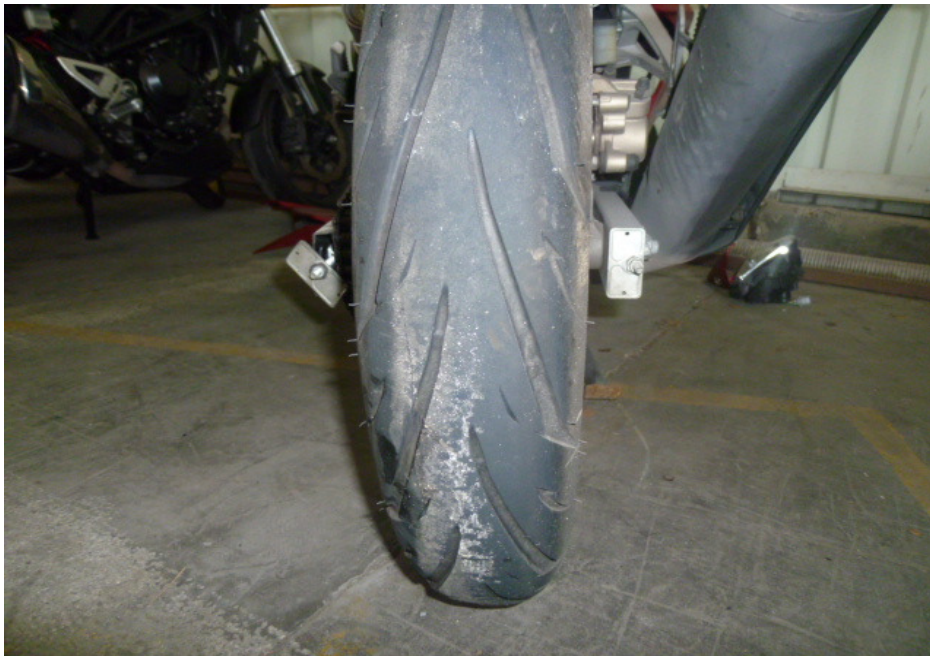
Photo 16 shows the condition of the Motorcycle's rear tyre. The rear tyre was observed to be in serviceable condition with remaining tread depth of approximately 4mm. The rear tyre was also observed to be sufficiently inflated for vehicular operation. We did not observe any tear, burst mark(s) and/or punctured hole(s) on the sidewalls as well as across the tread of the rear tyre.
