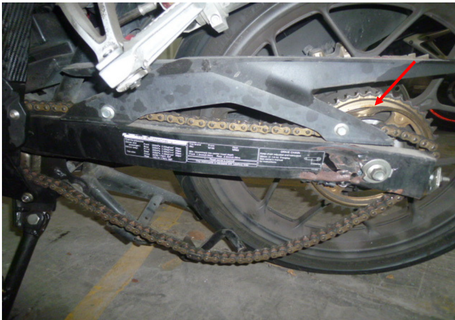
Photo 19 shows the general view of the gear train of the Motorcycle which was found to be damaged as a result of the accident. The chain was also observed to be dislodged from the gear train due to the deformed rear sprocket most likely as a result of the accident (arrowed). The chain was also found not to be adequately lubricated for operating purposes.
