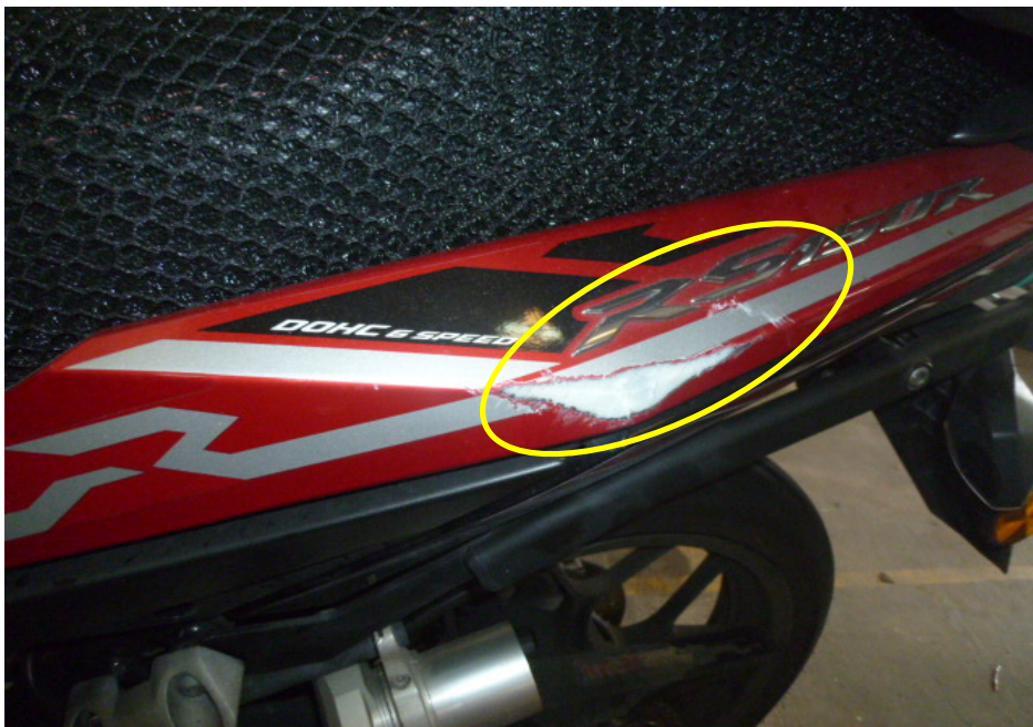
Photo 10 shows a closer view of the left rear side cover, which was amongst the body parts of the Motorcycle that had sustained damages of grazing nature as a result of the accident (circled).
