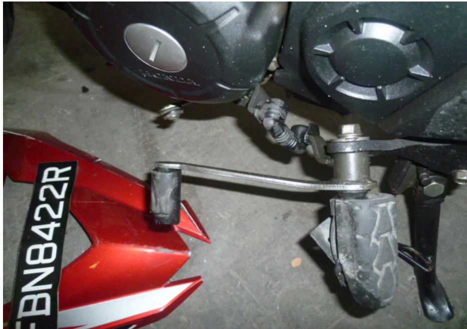
Photo 1 shows the broken gear shift pedal of the Motorcycle as a result of the accident. Hence the mileage was not recorded at the time of our inspection as we were unable to engage the Neutral gear to kickstart the Motorcycle.
