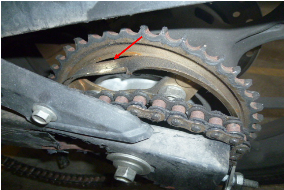
Photo 20 shows a closer view of the dislodged chain from the gear train due to the deformed rear sprocket most likely as a result of the accident (arrowed). The chain was also found not to be adequately lubricated for operating purposes.
