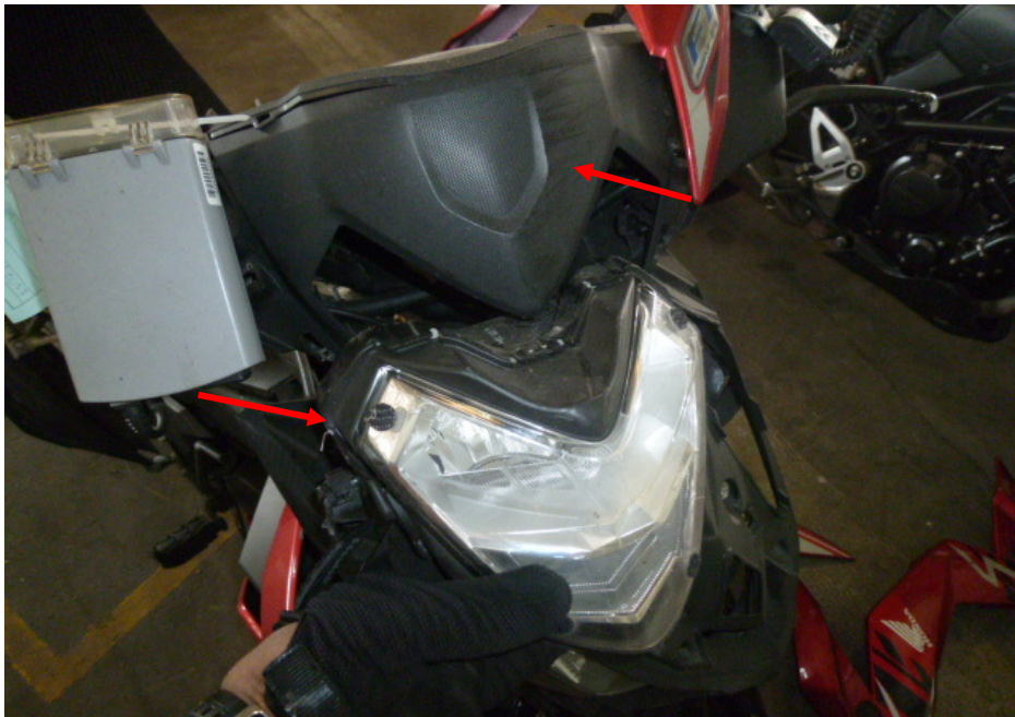
Photo 4 shows the general view of the headlight assembly and head cowling (arrowed) of the Motorcycle which was amongst the body parts of the Motorcycle that had sustained damage as a result of the accident.
