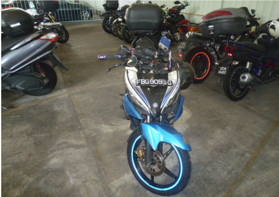
Photo 2 shows a general view of the frontal portion of the Motorcycle at the time of our inspection. The Motorcycle had sustained damages all around. Body parts that were found to have been damaged include its head cowling, front cowling, speedometer gauge, front mudguard, side cowlings, side mirrors, front brake lever, clutch lever, rear brake pedal and top box, amongst others.
