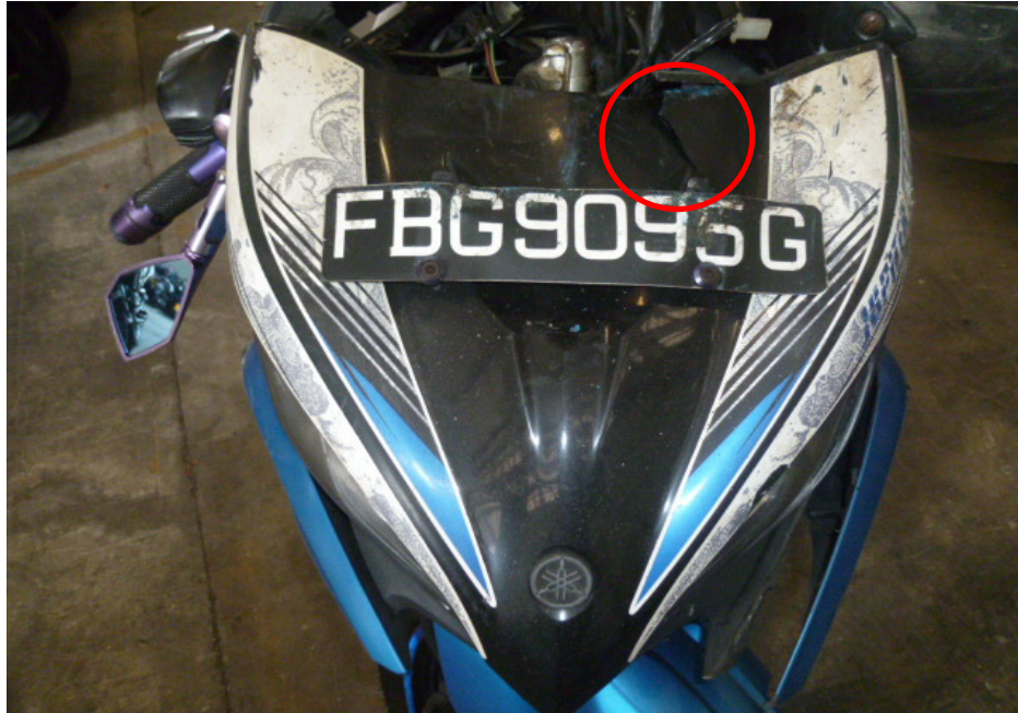
Photo 4 shows a closer view of the front cowling (arrowed) which was amongst the body parts at the front body of the Motorcycle that had sustained damage as a result of the accident (circled).
