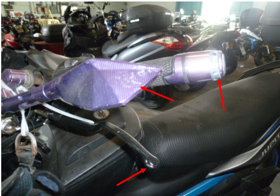
Photo 5 shows a closer view of the clutch lever, left side mirror and left handlebar end of the Motorcycle (arrowed). These parts were amongst the body parts of the Motorcycle which were damaged as a result of the accident.
