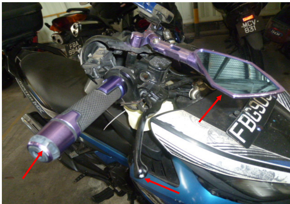
Photo 5 shows a closer view of the front brake lever, right side mirror and right handlebar end of the Motorcycle (arrowed). These parts were amongst the body parts of the Motorcycle which were damaged as a result of the accident.
