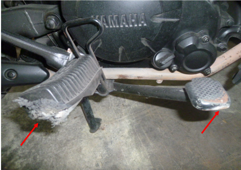
Photo 8 shows a closer view of the right front foot rest and rear brake pedal (arrowed) which were amongst the body parts of the Motorcycle that had sustained damages as a result of the accident.
