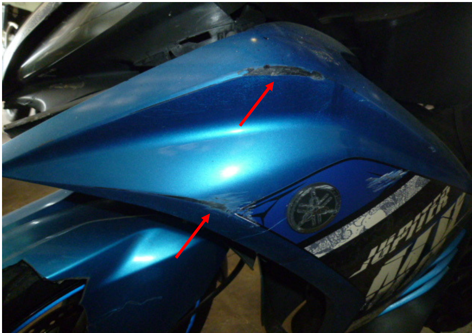
Photo 9 shows a closer view of the left cowling which was amongst the body parts at the front body of the Motorcycle that had sustained damages as a result of the accident (arrowed).
