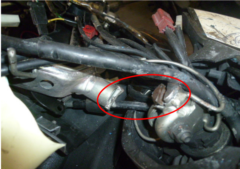
Photo 19 shows the steering stem of the Motorcycle. The steering stem (circled) was observed to be broken as a result of the accident. We were hence not able to conduct any tests on the steering system of the Motorcycle.
