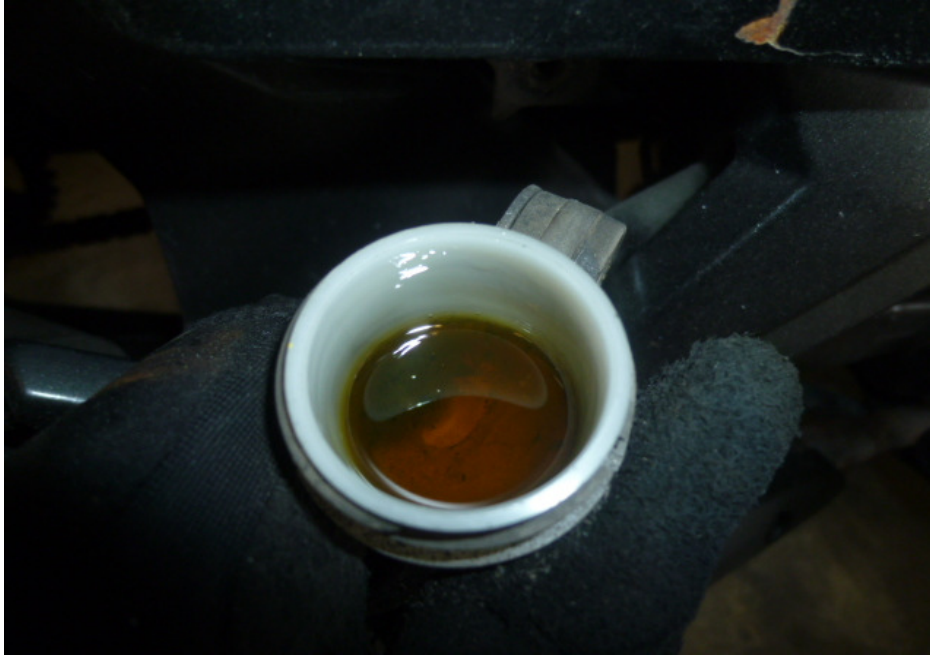
Photo 26 shows the brake fluid reservoir for the rear brake of the Motorcycle. The brake fluid was observed to be without contamination and of sufficient level for operational purposes.
