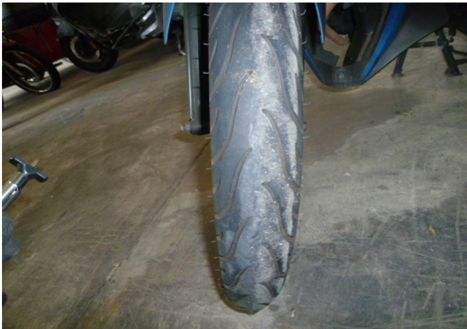
Photo 13 shows the condition of the Motorcycle's front tyre. The front tyre was observed to be in serviceable condition with remaining tread depth of approximately 4mm. The tyre was also observed to be sufficiently inflated for vehicular operation. We did not observe any tear, burst mark(s) and/or punctured hole(s) on the sidewalls as well as across the tread of the front tyre.
