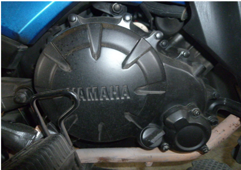
Photo 16 shows the right side of the engine of the Motorcycle at the time of our inspection. The various engine related parts and components were found to be intact with no visible damage. There was also no sign(s) or indication(s) of fluid leak observed around the right engine area of the Motorcycle.
