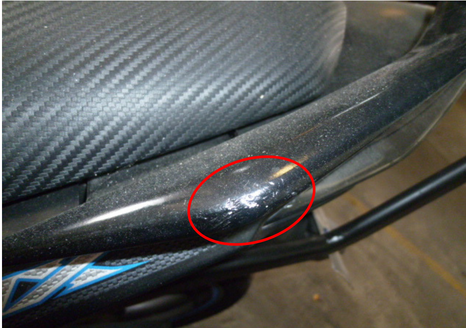
Photo 10 shows a closer view of the grazed left pillion grab rail which was amongst the body parts of the Motorcycle as a result of the accident (circled).
