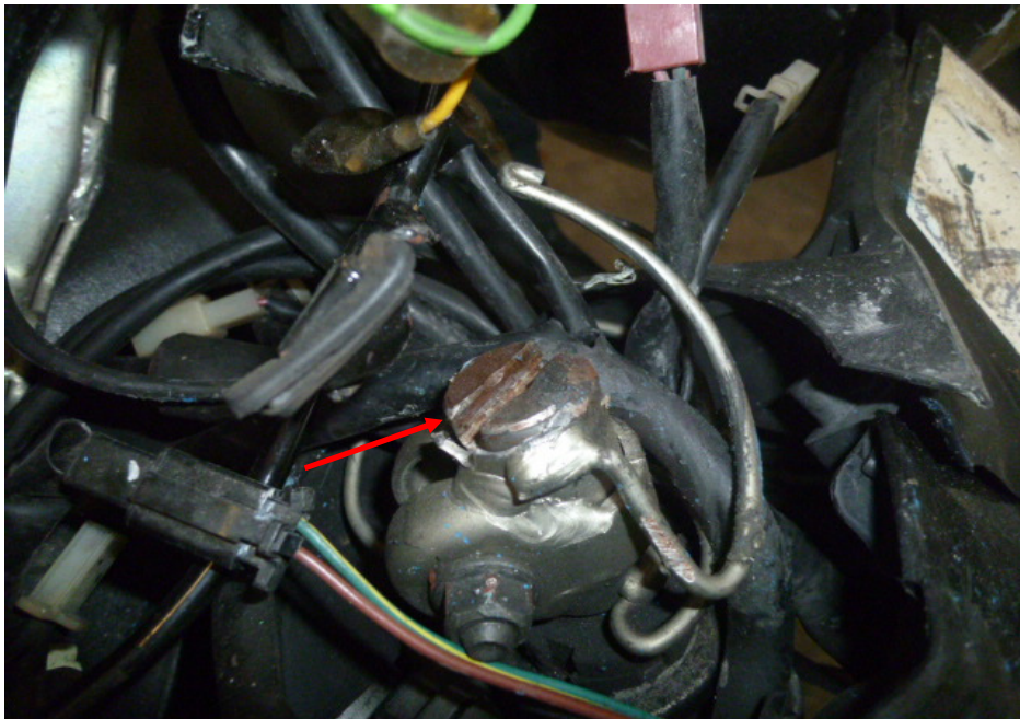
Photo 20 shows a close up view of the steering stem of the Motorcycle. The steering stem (arrowed) was observed to be broken as a result of the accident.
