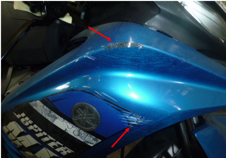
Photo 7 shows a closer view of the right cowling which was amongst the body parts at the front body of the Motorcycle that had sustained damages as a result of the accident (arrowed).
