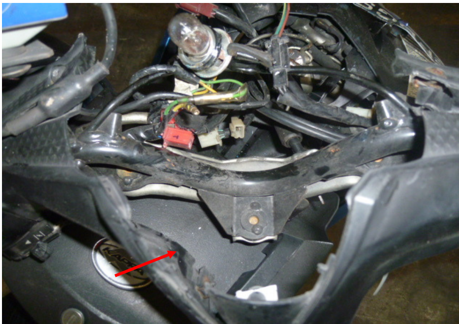
Photo 3 shows a closer view of the cracked head cowling (arrowed) which was amongst the body parts at the front body of the Motorcycle that had sustained damage as a result of the accident (circled).
