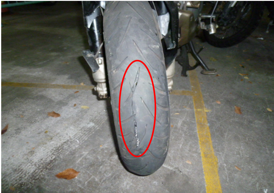
Photo 13 shows the condition of the Motorcycle's front tyre. The front tyre was observed to be in serviceable condition with remaining tread depth of approximately 4mm. The tyre was observed to be deflated. We also observed a tear on the front tyre as a result of the accident (circled).
