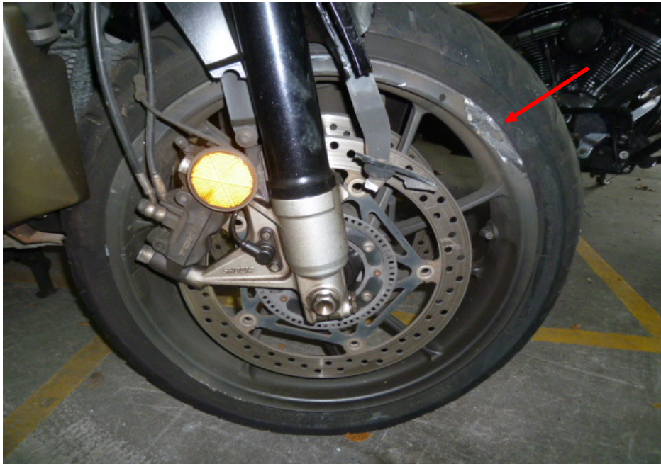
Photo 15 shows the deflated front tyre and grazed front wheel rim (arrowed) of the Motorcycle as a result of the accident at the time of our inspection.
