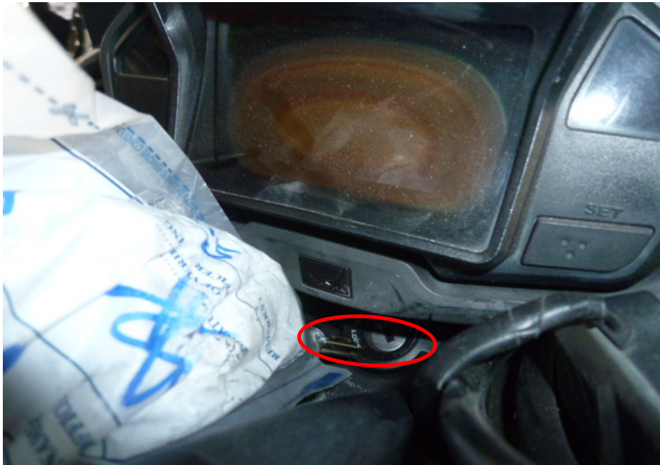
Photo 1 shows mileage of the Motorcycle which could not be recorded at the time of our inspection due to the damages sustained to the speedometer gauge. (circled).
