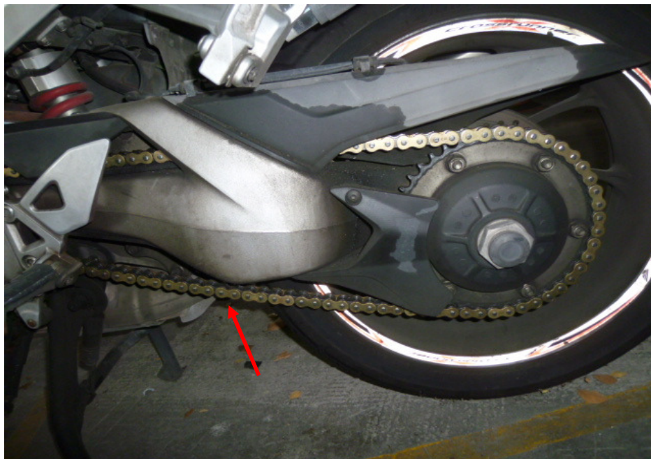
Photo 19 shows the general view of the gear chain (arrowed) of the Motorcycle, which was observed to be intact with no misalignment. It was also adequately lubricated for operating purposes.
