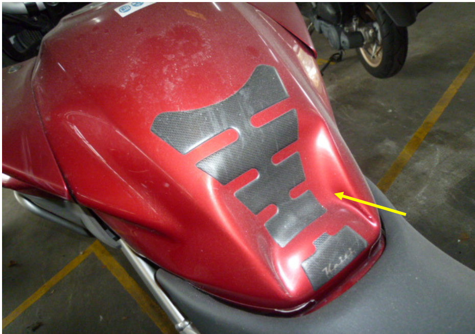
Photo 10 shows a closer view of the dented petrol tank of the Motorcycle as a result of the accident (arrowed).
