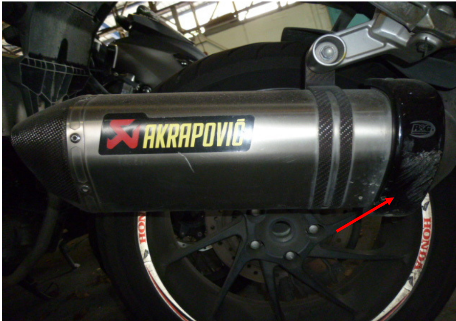
Photo 11 shows a closer view of the exhaust muffler protector which was amongst the body parts of the Motorcycle that had sustained damages of grazing nature as a result of the accident (arrowed).
