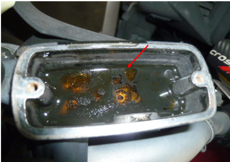
Photo 22 shows the hydraulic clutch fluid reservoir for the hydraulic clutch system of the Motorcycle. The hydraulic clutch fluid was observed to be of sufficient level for operational purposes. However it was also found to be slightly contaminated (arrowed).
