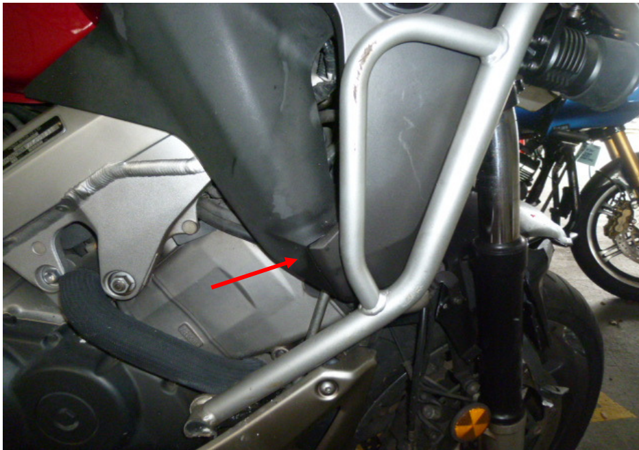
Photo 12 shows a closer view of the cracked right cowling of the Motorcycle as a result of the accident (arrowed).
