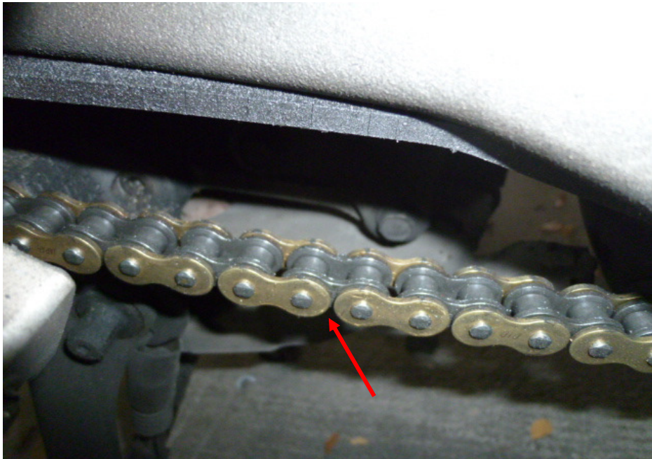
Photo 20 shows a closer view of the gear chain (arrowed) of the Motorcycle, which was observed to be intact with no misalignment. It was also adequately lubricated for operating purposes.
