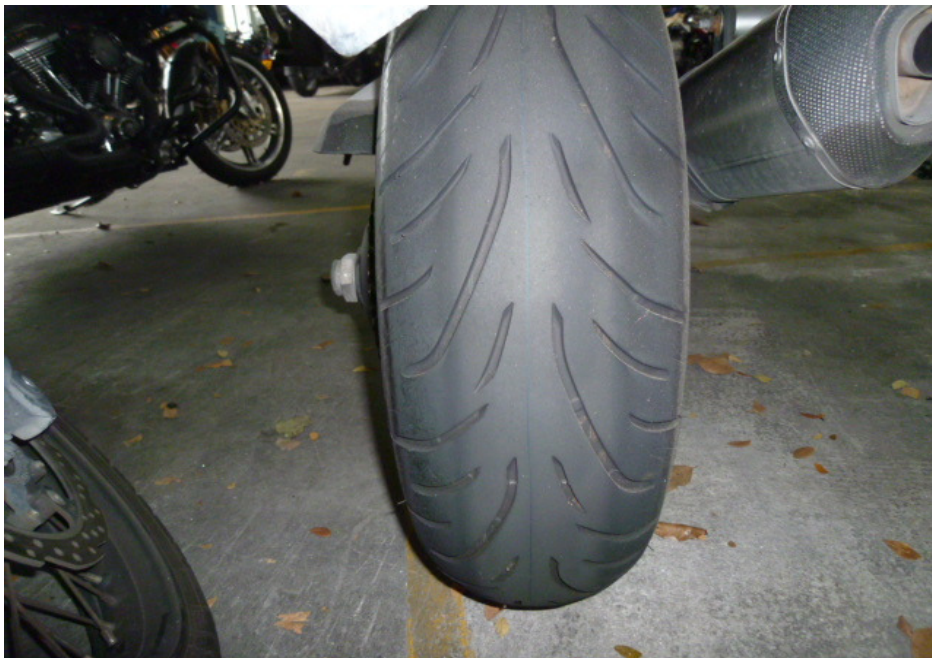
Photo 16 shows the condition of the Motorcycle's rear tyre. The rear tyre was observed to be in serviceable condition with remaining tread depth of approximately 6mm. The tyre was also observed to be sufficiently inflated for vehicular operation. We did not observe any tear, burst mark(s) and/or punctured hole(s) on the sidewalls as well as across the tread of the rear tyre.
