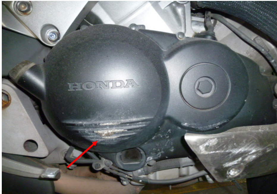
Photo 18 shows the right side of the engine of the Motorcycle at the time of our inspection. The various left engine components had sustained damage of grazing nature as a result of the accident (arrowed) however the engine components were still intact. There was also no fluid leak and/or fluid stain found around the right engine area of the Motorcycle.
