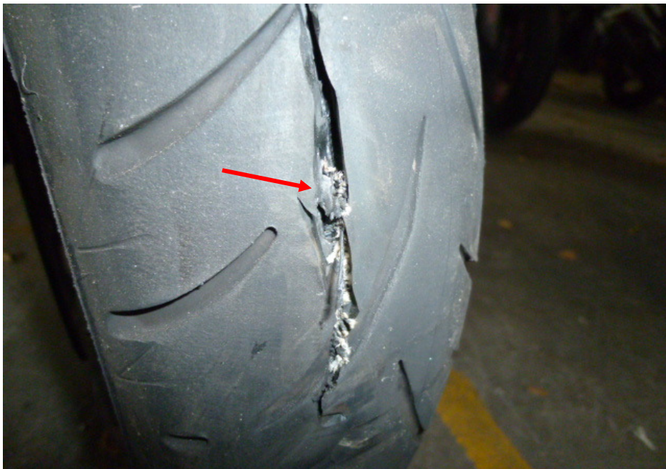
Photo 14 shows a closer view of the tear on the front tyre as a result of the accident (arrowed).
