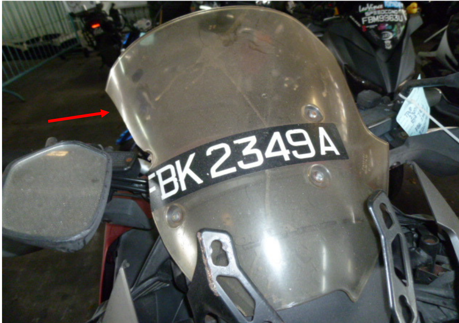
Photo 5 shows a close up view of the broken windshield was amongst the body parts of the Motorcycle that had sustained damage as a result of the accident (arrowed).
