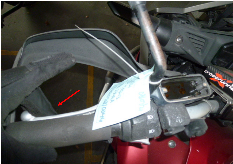
Photo 23 shows the clutch lever being depressed. There was some resistance felt (spongy like feel) upon pressing the clutch lever (arrowed). This would indicate that there is no leakage of pressure/vacuum in the hydraulic clutch system.
