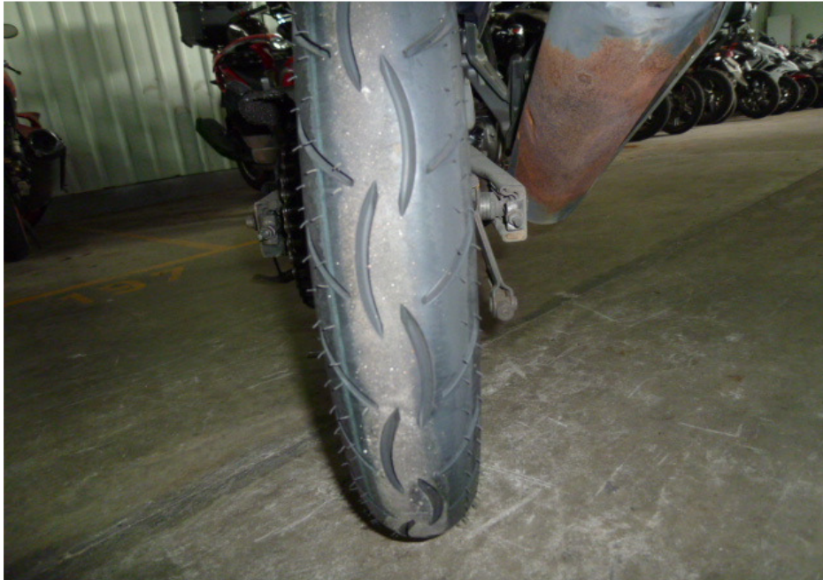
Photo 18 shows the condition of the Motorcycle's rear tyre. The rear tyre was observed to be in serviceable condition with remaining tread depth of approximately 7mm. The tyre was also observed to be sufficiently inflated for vehicular operation. We did not observe any tear, burst mark(s) and/or punctured hole(s) on the sidewalls as well as across the tread of the rear tyre.
