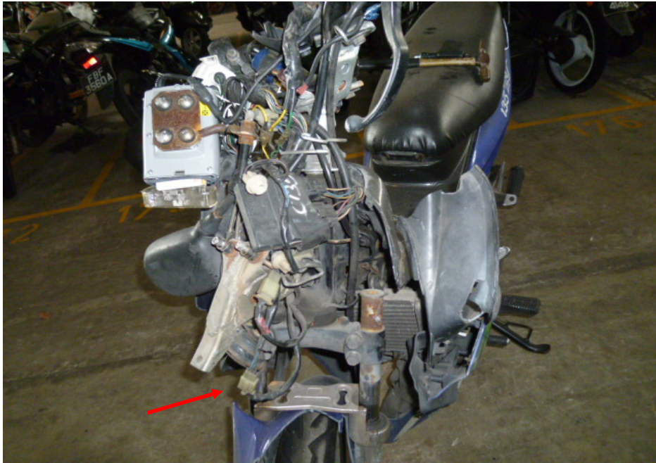
Photo 14 shows the missing front cowling of the Motorcycle at the time of our inspection (arrowed).
