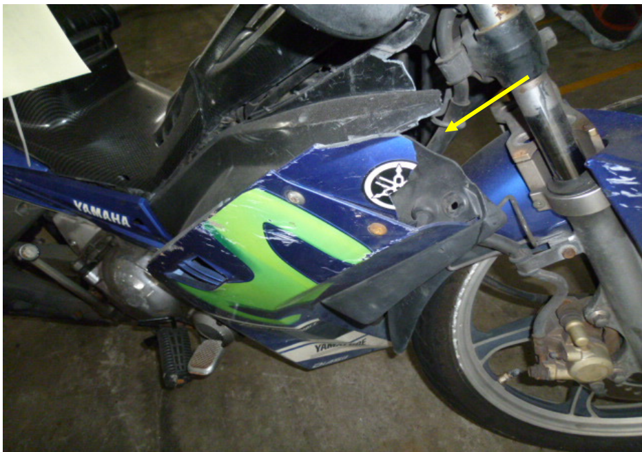
Photo 9 shows a closer view of the right cowling which was amongst the body parts at the front body of the Motorcycle that had sustained damages as a result of the accident (arrowed).
