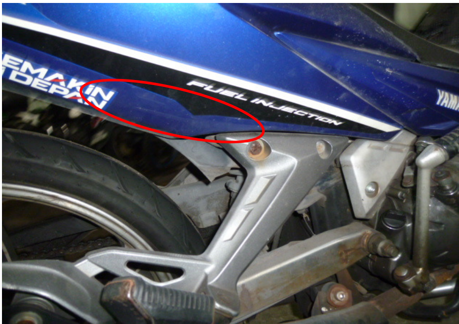
Photo 11 shows a closer view of the right rear side cover which was amongst the body parts of the Motorcycle that had sustained damages of grazing nature as a result of the accident (circled).
