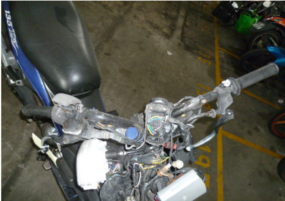
Photo 12 shows a closer view of the bent handlebar which were amongst the body parts of the Motorcycle that had sustained damage as a result of the accident.
