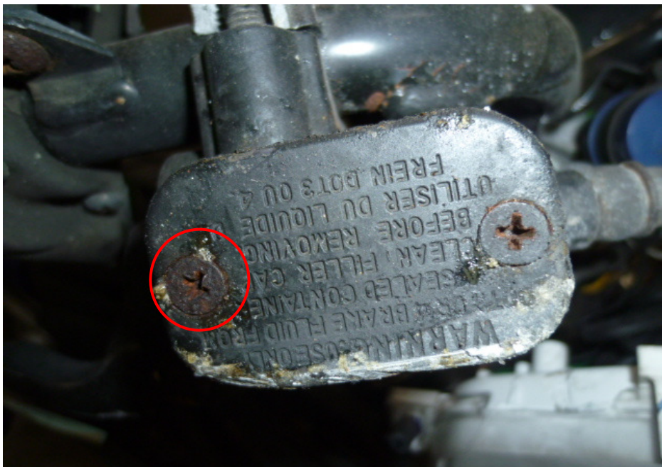
Photo 26 shows the brake fluid reservoir cover for the front brake of the Motorcycle. We were unable to examine whether the brake fluid was of sufficient level and without contamination for operational purposes due to the worn out screw (circled).
