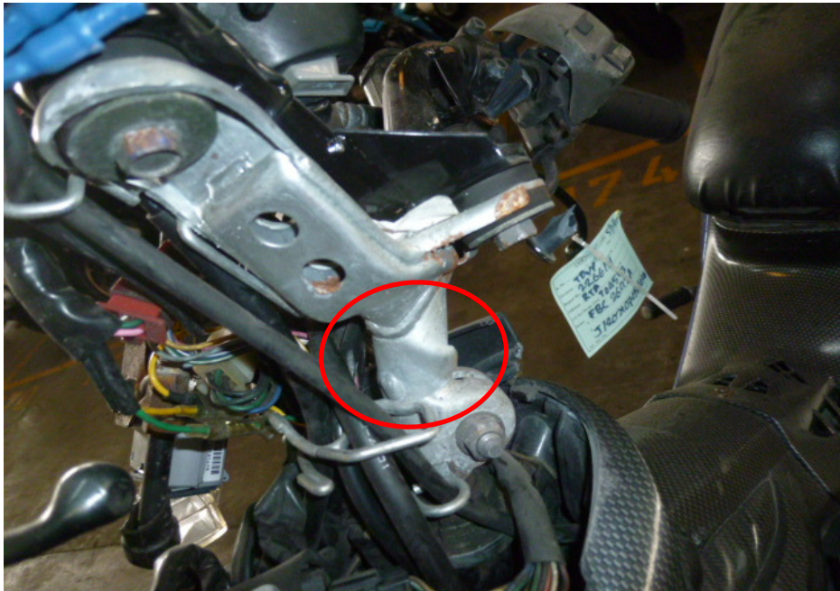
Photo 23 shows the steering stem of the Motorcycle. The steering stem (circled) was observed to be broken as a result of the accident. We were hence not able to conduct any tests on the steering system of the Motorcycle.
