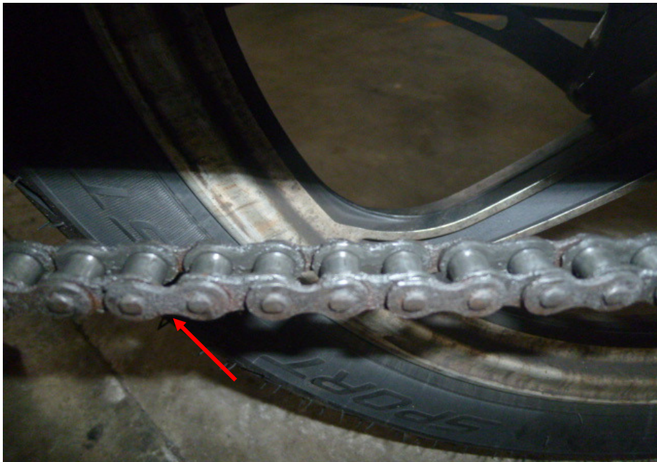
Photo 22 shows the closer view of the gear train (arrowed) of the Motorcycle, which was observed to be intact with no misalignment. It was also adequately lubricated for operating purposes.
