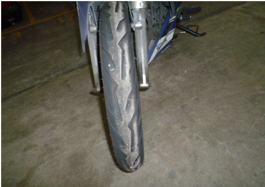
Photo 17 shows the front tyre of the Motorcycle at the time of our inspection. The front tyre was observed to be in serviceable condition with remaining tread depth of approximately 3mm. The pattern of the tread was also clearly visible. There was no tear, burst mark(s) and/or punctured hole(s) on the sidewalls as well as across the tread of the front tyre.
