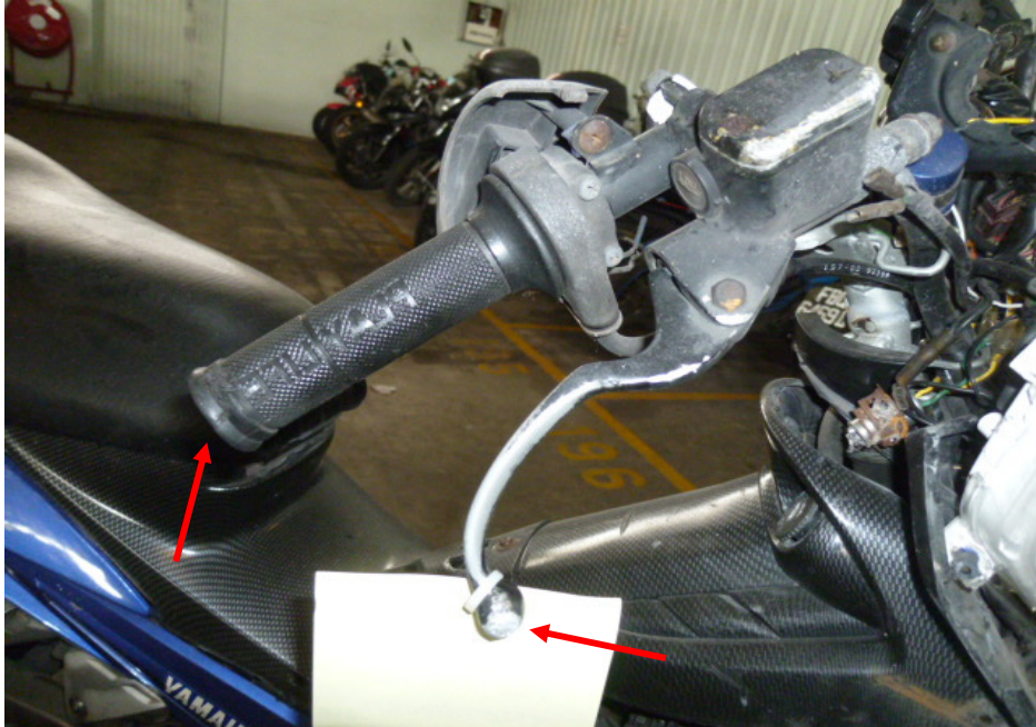
Photo 6 shows a closer view of the front brake lever and left handlebar end of the Motorcycle (arrowed). These parts were amongst the body parts of the Motorcycle which were damaged as a result of the accident.
