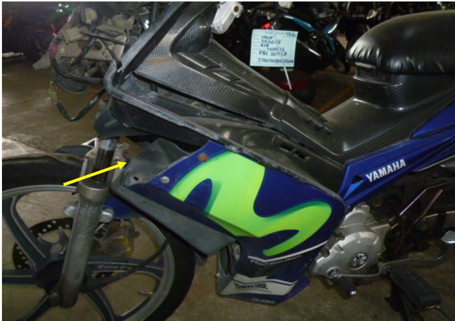
Photo 10 shows a closer view of the cracked left cowling which was amongst the body parts at the front body of the Motorcycle that had sustained damages as a result of the accident (arrowed).
