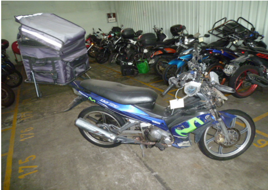
Photo 4 shows a general view of the right body of the Motorcycle at the time of our inspection. The Motorcycle had sustained damages all around. Body parts that were found to have been damaged include its headlight assembly, front cowlings, steering stem, front mudguard, handlebar, side mirrors, side cowlings, front brake lever, clutch lever, right rear side cover, rear brake pedal, right front footrest, top box rack and exhaust muffler heat shield, amongst others.
