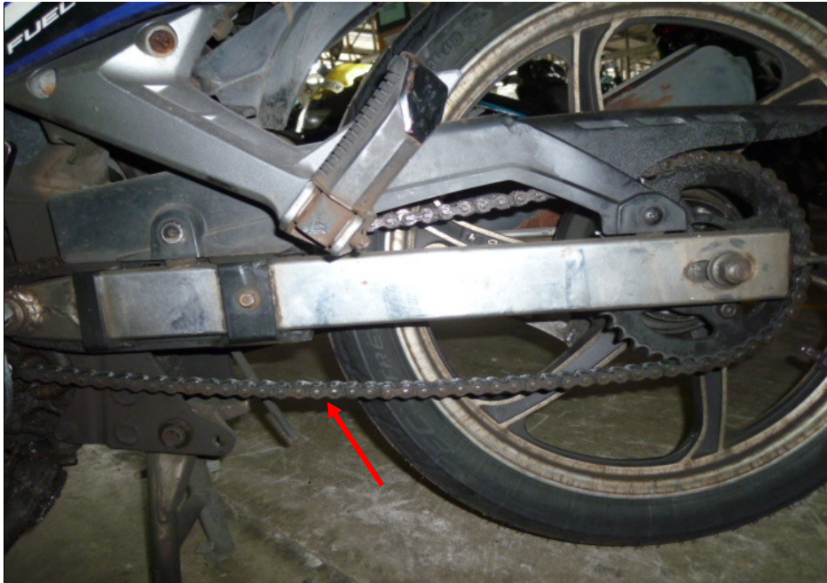
Photo 21 shows the gear chain (arrowed) of the Motorcycle, which was observed to be intact with no misalignment. It was also adequately lubricated for operating purposes. The gear train rotates the rear wheel of the Motorcycle.
