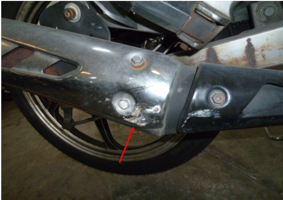
Photo 16 shows a closer view of the grazed exhaust muffler heat shield of the Motorcycle as a result of the accident (arrowed).
