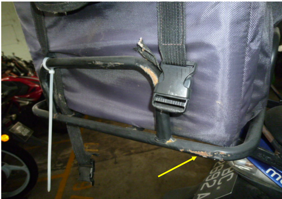
Photo 15 shows a closer view of the top box rack which was amongst the body parts of the Motorcycle that had sustained damages of grazing nature as a result of the accident (arrowed).
