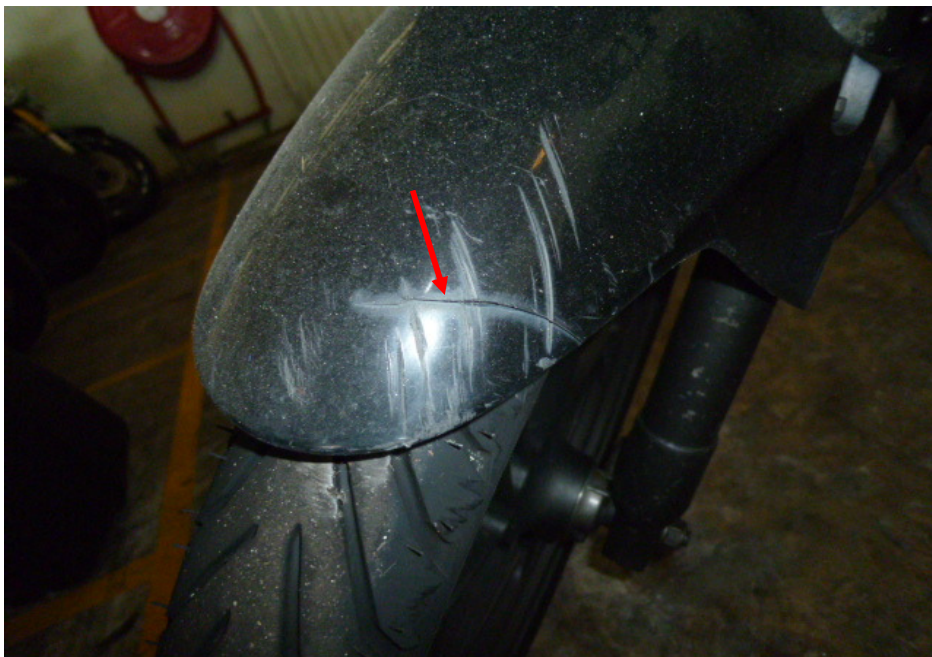
Photo 10 shows a close up view of the cracked front mudguard of the Motorcycle as a result of the accident (arrowed).
