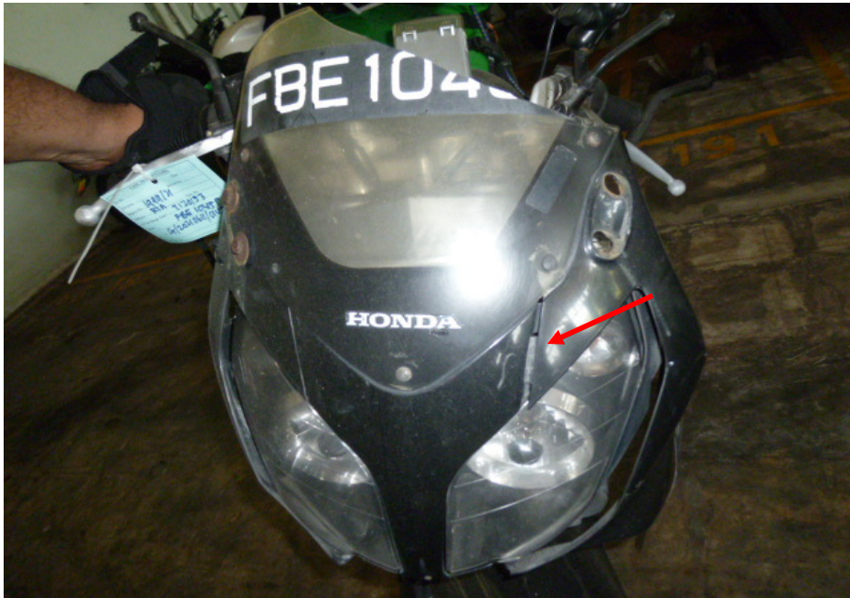
Photo 6 shows the general view of the front cowling of the Motorcycle which was amongst the body parts of the Motorcycle that had sustained damage as a result of the accident (arrowed).
