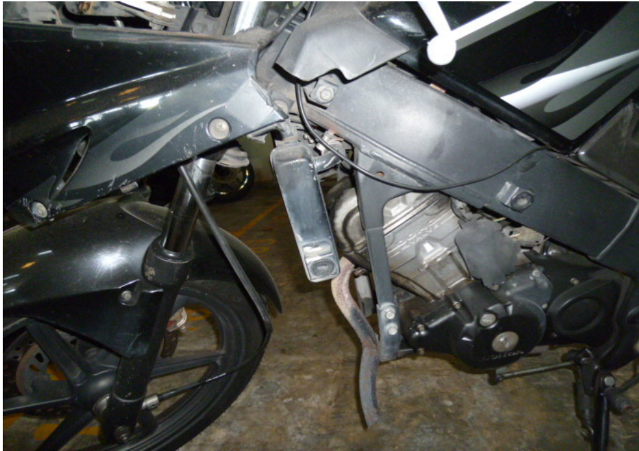
Photo 7 shows the missing left cowling of the Motorcycle as a result of the accident.
