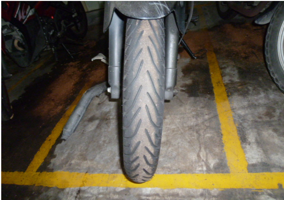
Photo 15 shows the condition of the Motorcycle's front tyre. The front tyre was observed to be in serviceable condition with remaining tread depth of approximately 5mm. We did not observe any tear, burst mark(s) and/or punctured hole(s) on the sidewalls as well as across the tread of the front tyre. The front tyre was also observed to be sufficiently inflated for vehicular operation.
