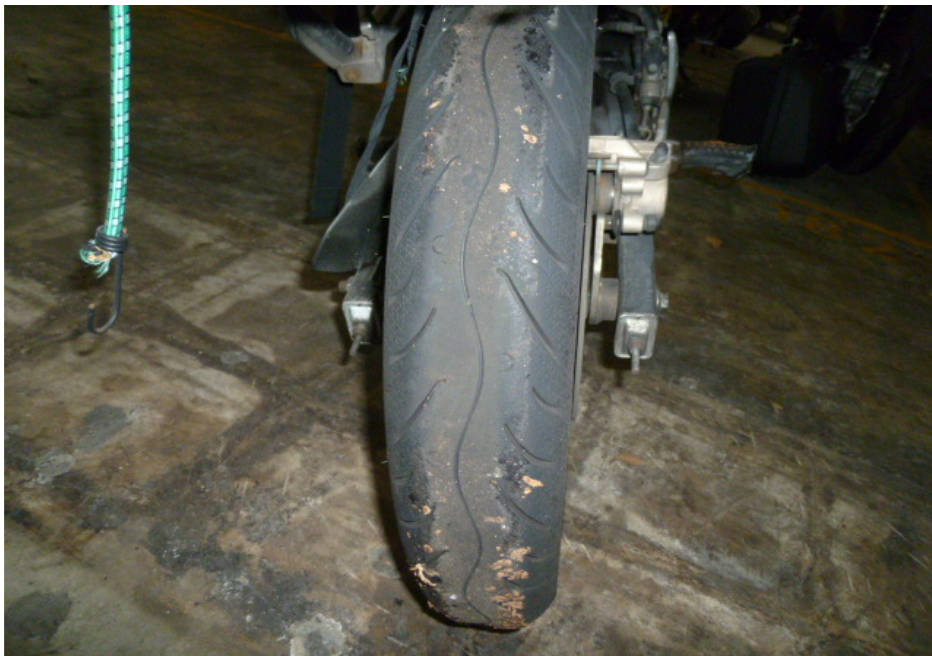
Photo 16 shows the condition of the Motorcycle's rear tyre. The rear tyre was observed to be in serviceable condition with remaining tread depth of approximately 2mm. We did not observe any tear, burst mark(s) and/or punctured hole(s) on the sidewalls as well as across the tread of the rear tyre. However the front tyre was observed to be deflated as a result of the accident.
