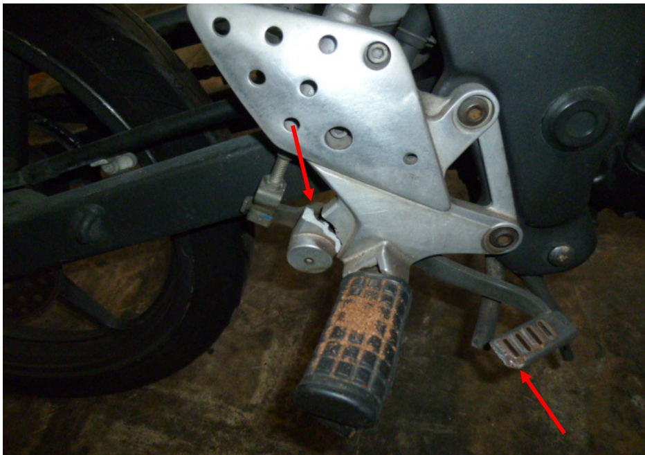
Photo 12 shows the bent rear brake pedal and broken right front footrest which were amongst the body parts of the Motorcycle that had sustained damage as a result of the accident (arrowed).
