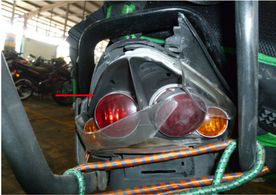
Photo 13 shows the broken tail light assembly which was amongst the body parts of the Motorcycle that had sustained damage as a result of the accident (arrowed).
