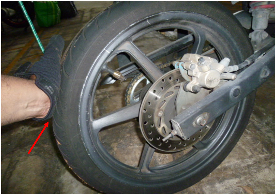
Photo 17 shows a closer view of the deflated rear tyre of the Motorcycle as a result of the accident (arrowed).
