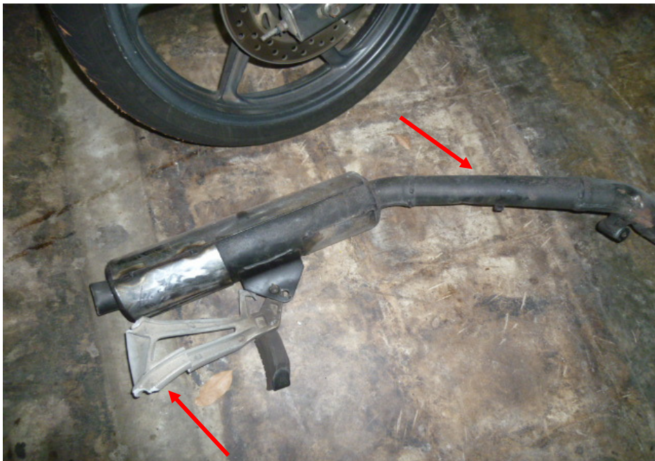
Photo 14 shows the broken exhaust muffler and right pillion foot peg bracket (arrowed) of the Motorcycle as a result of the accident.
