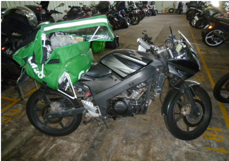
Photo 4 shows a general view of the right body of the Motorcycle at the time of our inspection. The Motorcycle had sustained damages all around. Body parts that were found to have been damaged include its windshield, front cowling, side cowlings, front mudguard, right side mirror, right handlebar end, front brake lever, left rear side cover, rear brake pedal, right front footrest bracket, tail light assembly, exhaust muffler and right pillion foot peg bracket, amongst others.
