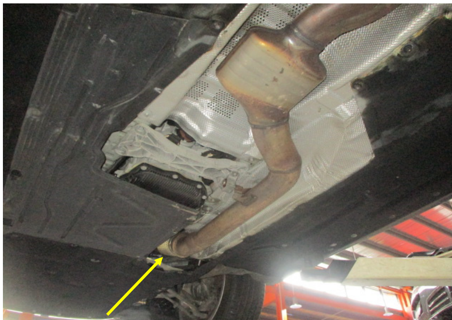
Photo 25 shows the front section of the Motor Car's exhaust system. My examination of the Motor Car's exhaust system revealed no sign(s) or indication(s) of any cut or weld marks along its exhaust pipes, on its rear muffler, on its centre resonator boxes and on its catalytic converter (arrowed).
