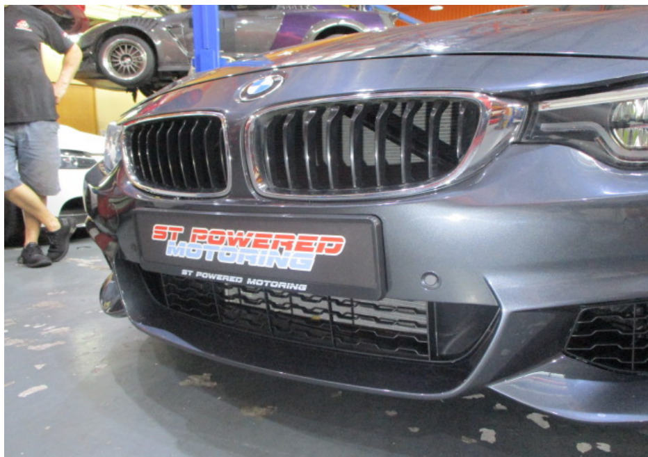
Photo 10 shows a closer view of the Motor Car's front bumper, front bumper sensors, front bumper centre lower grille, oil cooler and radiator grilles. The body parts at the frontal portion of the Motor Car were visually examined and it was observed that the repair/restoration works carried out to the damaged area of the Motor Car (refer to photograph 1 & 2 above) were reasonably adequate and in order.
