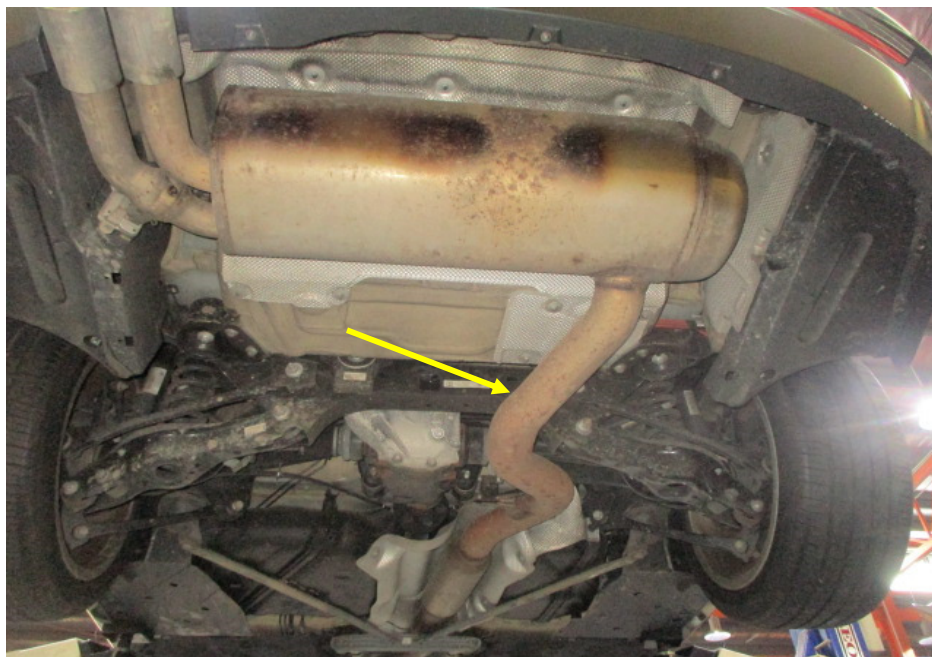
Photo 24 shows the rear section of the Motor Car's exhaust system. My examination of the Motor Car's exhaust system revealed no sign(s) or indication(s) of any cut or weld marks along its exhaust pipes (arrowed), on its rear muffler, on its centre resonator boxes and on its catalytic converter.
