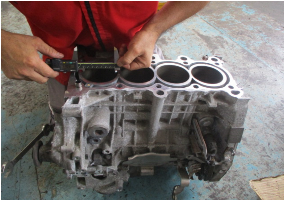
Photo 7 shows measurement being carried out to the bore of cylinder 1 of the Honda engine. The measurements were carried out using a digital Vernier Caliper that was calibrated before the start of the measurements.
