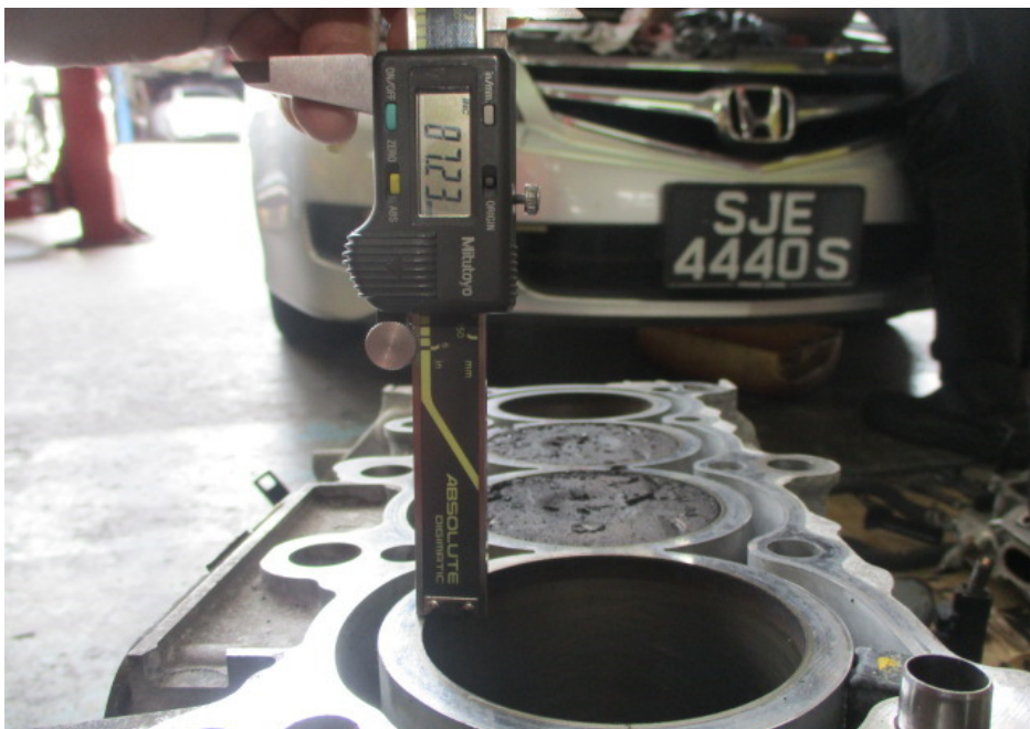
Photo 10 shows the stroke measurement of cylinder 1, which was recorded to be 87.23mm.
