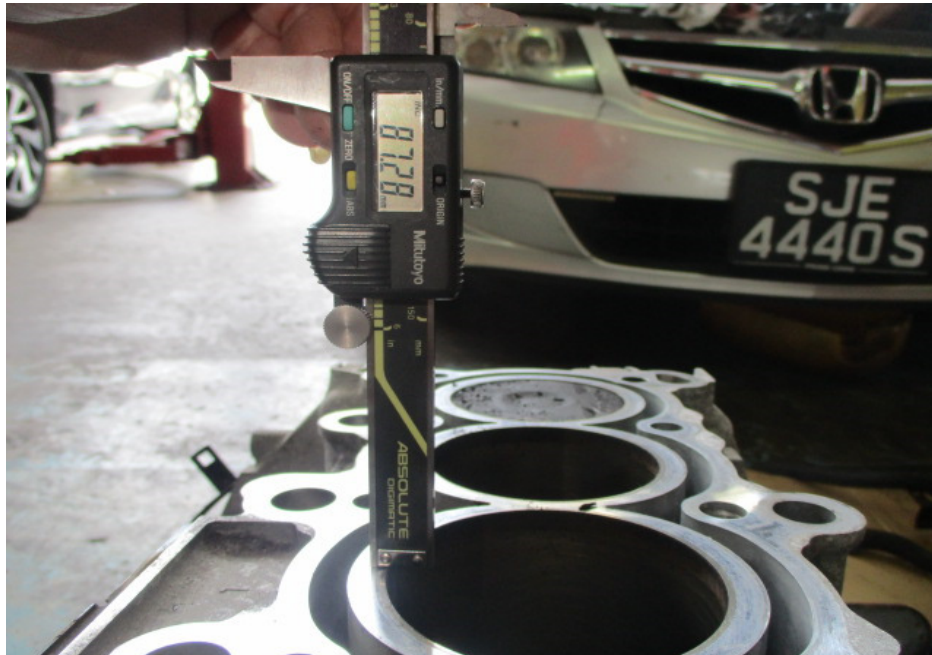
Photo 13 shows the stroke measurement of cylinder 2, which was recorded to be 87.28mm.
