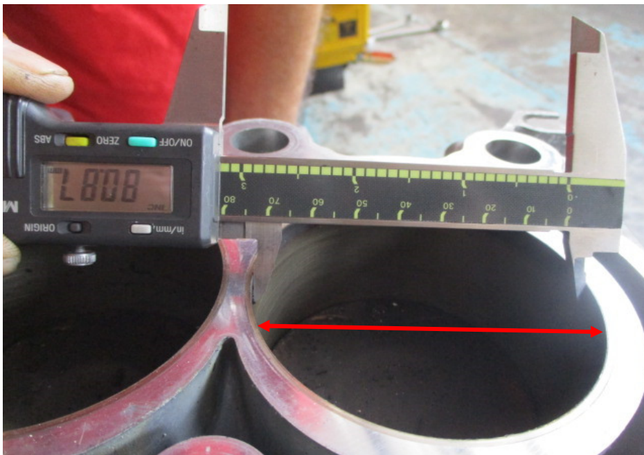
Photo 18 shows measurement being carried out to the bore (arrowed) of cylinder 4 of the Honda engine. The bore measurement of cylinder 4 was recorded to be 80.87mm.
