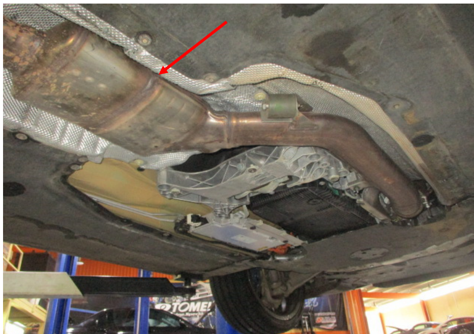
Photo 26 shows a general view of the Motor Car's exhaust system (front section). My examination of the Motor Car's exhaust system revealed no sign(s) or indication(s) of any cut or weld marks along its exhaust pipes, on its centre resonator box (arrowed), on its catalytic converter and on its rear muffler.
