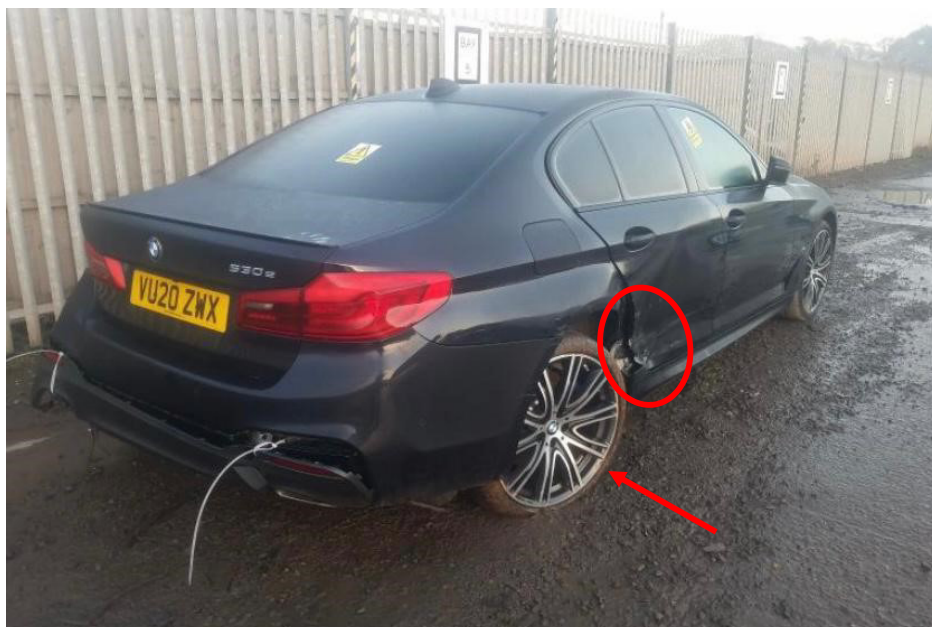
Photo 2 shows the rear right body of the Motor Car (photograph provided to me). The Motor Car was observed to have sustained damage to its rear right portion (circled). Body parts damaged include the rear right fender and rear right door. The orientation of the rear right wheel (arrowed) and rear left wheel (refer to photograph 4 below) suggest damage to the rear undercarriage parts of the Motor Car. The rear right tyre was also observed to be punctured.
