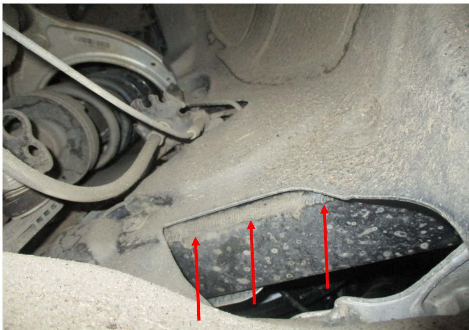
Photo 30 shows the chassis/structural body at the underside front right of the Motor Car. The original factory sealant (arrowed) at the joints along the chassis/structural body was observed to be untouched. In general, I had found no work was carried out on the chassis/structural body of the Motor Car. The chassis/structural body of the Motor Ca was originally fitted.
