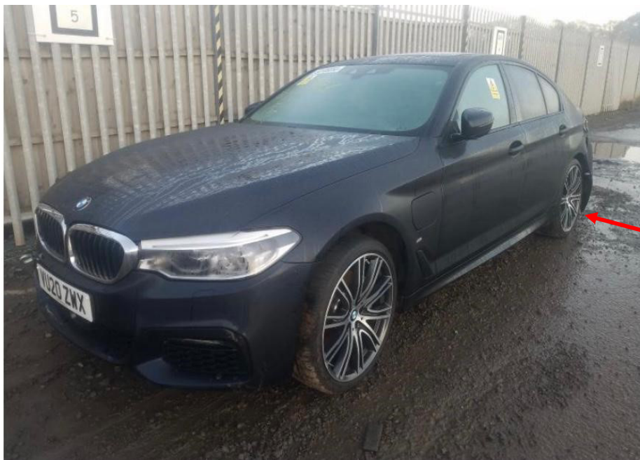
Photo 3 shows the front left body of the Motor Car (photograph provided to me). No physical damage was observed to the frontal portion of the Motor Car. The orientation of the rear left wheel (arrowed) and rear right wheel (refer to photograph 1 above) suggest damage to the rear undercarriage parts of the Motor Car.
