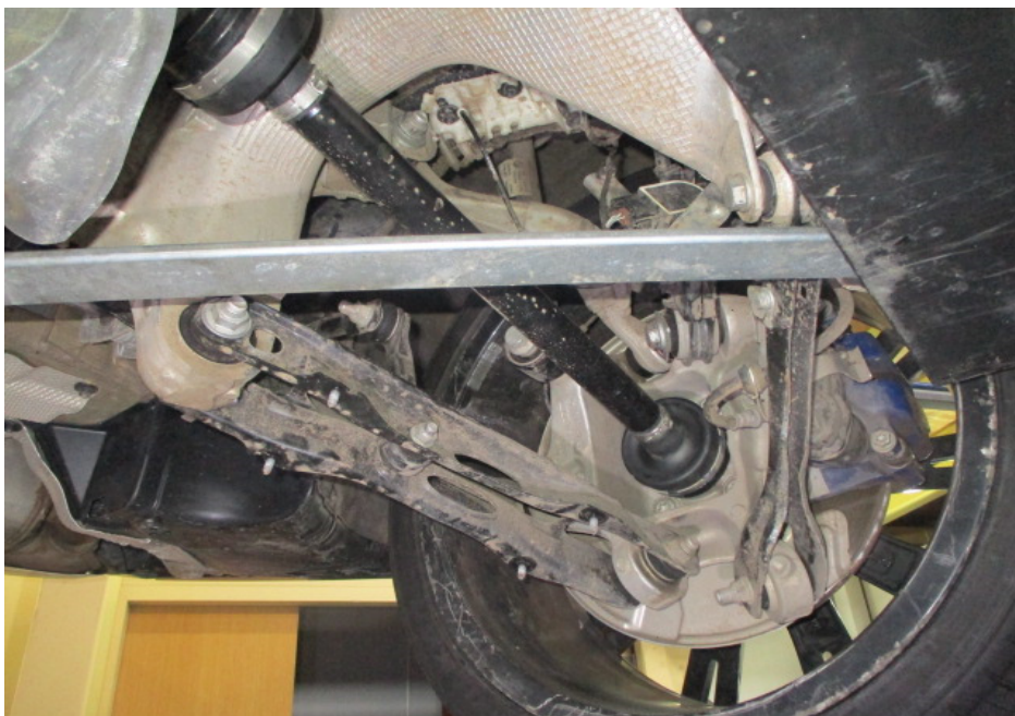
Photo 23 shows the various undercarriage components at the rear left wheel of the Motor Car. The mechanical components, control arms and linkages were all found to be intact and secured in an appropriate manner.
