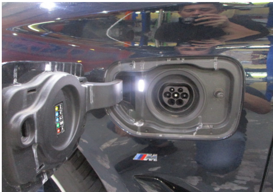
Photo 12 shows the charging socket and charging socket cover of the Motor Car. The charging socket pins were observed to be undamaged.
