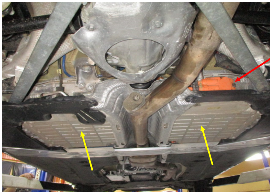
Photo 27 shows the Motor Car's electric battery (yellow arrow) that was fitted at the underside centre of the Motor Car. The cable connections (red arrow) were checked and found to be securely fitted into the respective connectors. The electric battery was also observed to be fitted securely. The electric cables connecting the electric motor within the engine compartment (refer to photograph 15 above) to the electric battery were securely fitted into the respective connectors and protected by dust covers.
