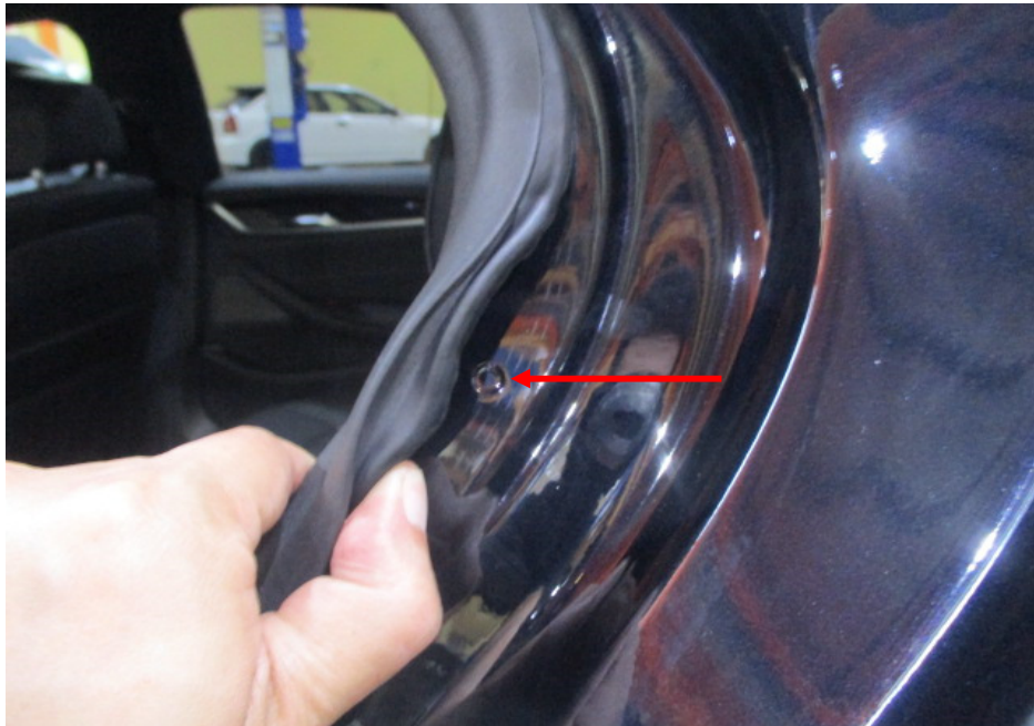
Photo 34 shows the left side "C" pillar of the Motor Car. I did not find any weld marks other than original spot weld marks (arrowed) on the left side "C" pillar of the Motor Car which, indicates that there was no re-welding works carried out. In general, I had found all the non-detachable body panels of the Motor Car to be originally fitted at the time of my inspection.
