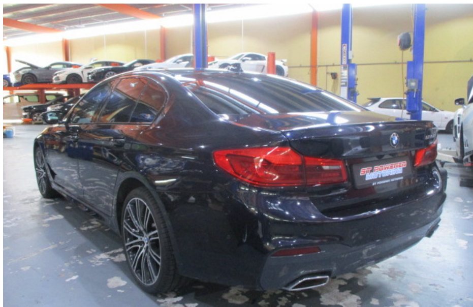
Photo 5 shows a general view of the rear left body of the Motor Car at the time of my inspection. The Motor Car was observed to be in a relatively good general condition with no loose exterior fittings observed. The body parts at the rear left portion of the Motor Car were visually examined and it was observed that the repair/restoration works carried out to the damaged area of the Motor Car (refer to photograph 4 above) were reasonably adequate and in order.
