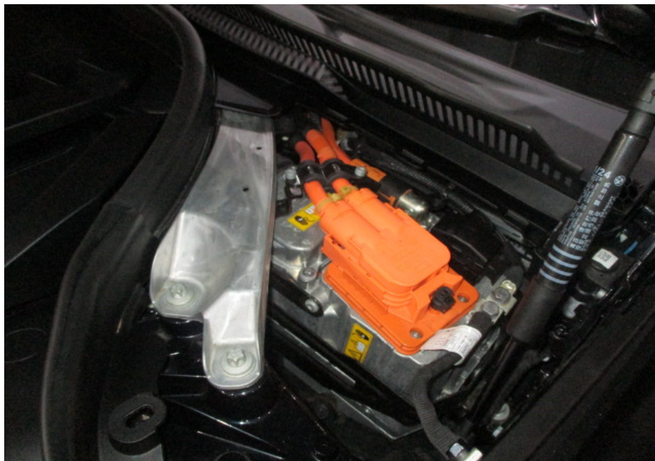
Photo 15 shows a general view of the electric motor that was fitted in the engine compartment of the Motor Car. The cable connections were checked and found to be securely fitted into the respective connectors. The electric cables connecting the electric motor to the electric battery, located at the underside centre (refer to photograph 27 below), were securely fitted into the respective connectors and protected by dust covers.
