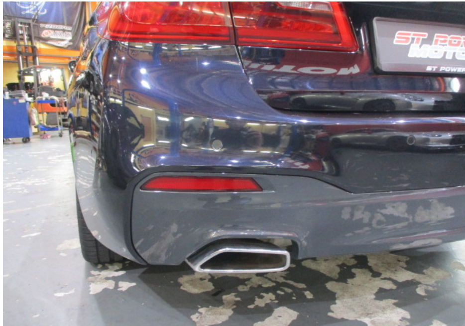
Photo 6 shows a closer view of the Motor Car's rear bumper, rear bumper lower cover, rear bumper left reflector and rear left taillamp. The body parts at the rear left portion of the Motor Car were visually examined and it was observed that the repair/restoration works carried out to the damaged area of the Motor Car (refer to photograph 4 above) were reasonably adequate and in order.
