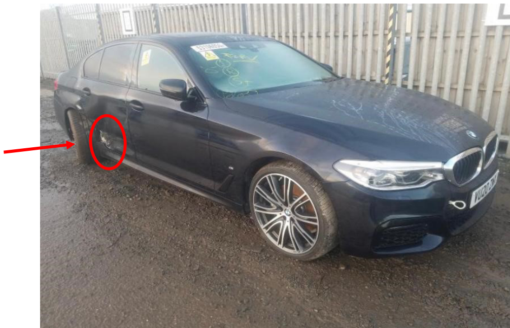
Photo 1 shows the front right body of the Motor Car (photograph provided to me). The Motor Car was observed to have sustained damage to its rear right portion (circled). Body parts damaged include the rear right fender and rear right door. The orientation of the rear right wheel (arrowed) and rear left wheel (refer to photograph 3 below) suggest damage to the rear undercarriage parts of the Motor Car.
