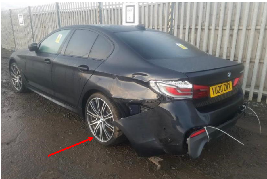
Photo 4 shows the rear left body of the Motor Car (photograph provided to me). Apart from the rear right portion, the Motor Car had also sustained damage to its rear left portion. The rear bumper, rear left fender, and rear left taillamp were amongst the body parts that were observed to have been damaged. The orientation of the rear left wheel (arrowed) and rear right wheel (refer to photograph 2 above) suggest damage to the rear undercarriage parts of the Motor Car.
