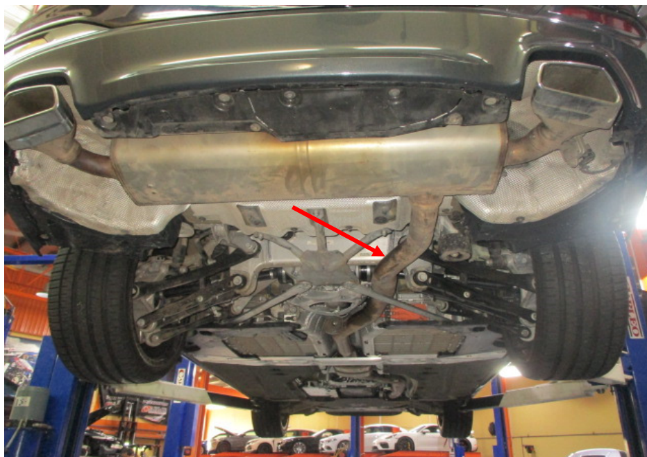
Photo 25 shows a general view of the Motor Car's exhaust system (rear section). My examination of the Motor Car's exhaust system revealed no sign(s) or indication(s) of any cut or weld marks along its exhaust pipes (arrowed), on its centre resonator box, on its catalytic converter and on its rear muffler.
