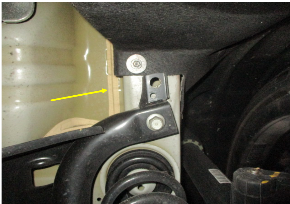
Photo 26 shows the chassis/structural body at the underside rear right of the Motor Car. I did not find any weld marks other than original spot weld marks on the chassis/structural body of the Motor Car. The original factory sealant (arrowed) at the joints along the chassis/structural body was untouched, indicating no work was done on the chassis/structural body of the Motor Car and that the chassis/structural body was originally fitted.
