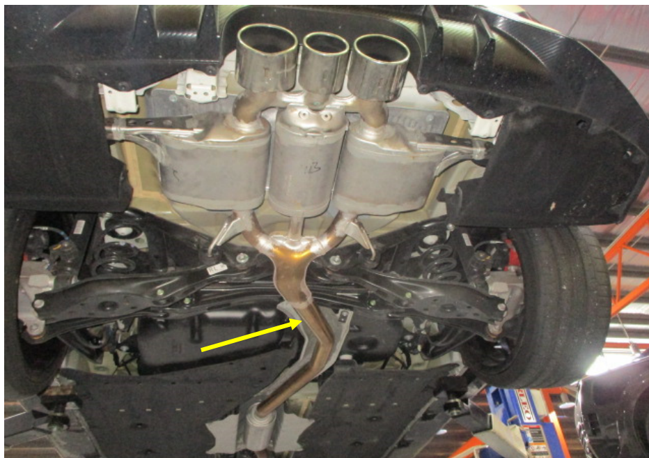
Photo 24 shows the rear section of the Motor Car's exhaust system. My examination of the Motor Car's exhaust system revealed no sign(s) or indication(s) of any cut or weld marks along its exhaust pipes (arrowed), on its rear mufflers, on its centre resonator boxes and on its catalytic converter.
