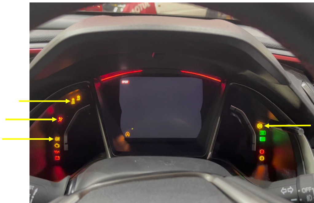
Photo 17 shows the warning lights for the various electronic safety features appearing on the instrument panel of the Motor Car during its self-test when the engine is cranked, in particular the ABS, SRS, VSA and EPS lights (arrowed).
