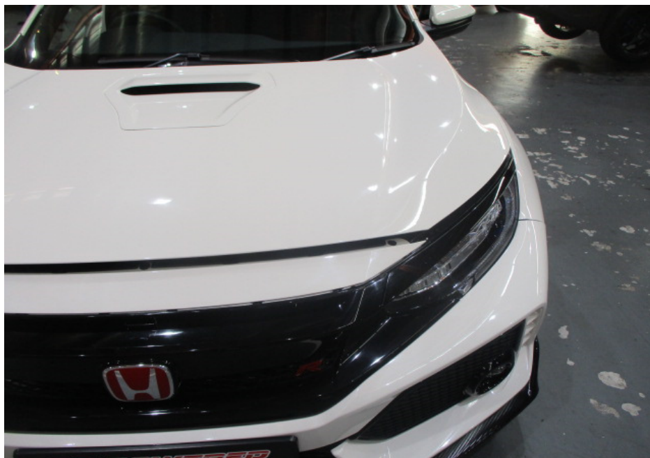
Photo 10 shows a closer view of the Motor Car's front bumper, front left headlamp, front bonnet and radiator grille at the time of my inspection. The body parts at the frontal portion of the Motor Car were visually examined and it was observed that the repair/restoration works carried out to the damaged area of the Motor Car (refer to photograph 1 & 2 above) were reasonably adequate and in order.
