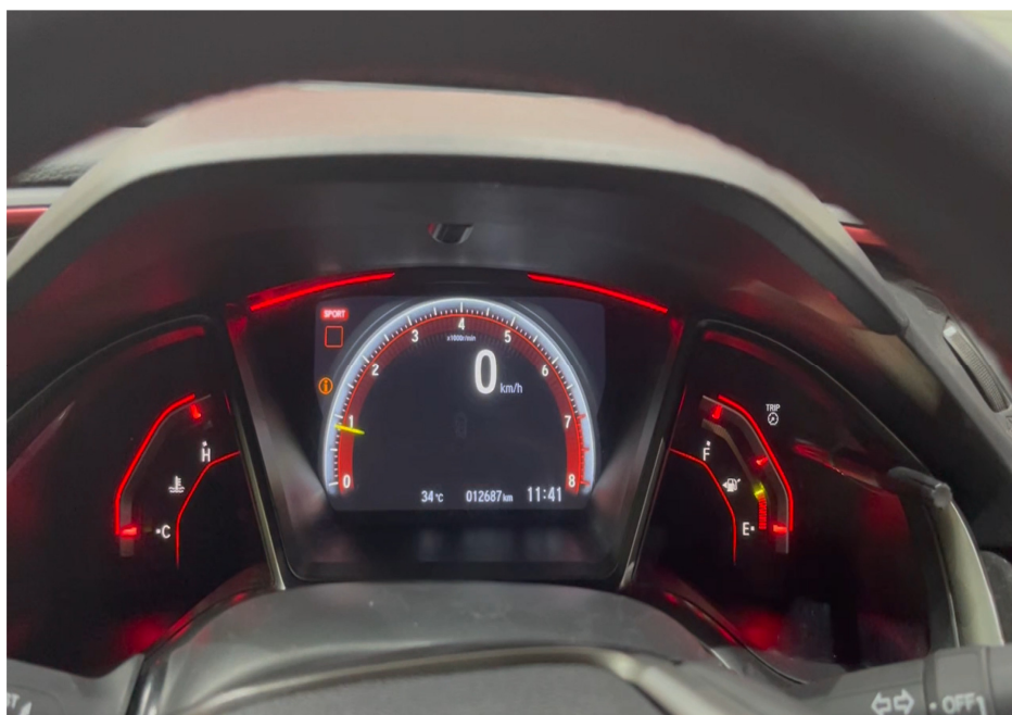
Photo 18 shows the respective warning lights no longer illuminated, indicating that there is no fault detected to the ABS, SRS, VSA and EPS systems of the Motor Car during the self-test. These electronic systems were hence in working condition at the time of my inspection.
