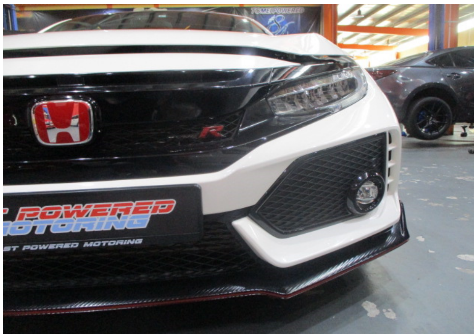
Photo 9 shows a closer view of the Motor Car's front bumper, front bumper lower spoiler, front bumper left lower grille, front left fog lamp, front left headlamp and radiator grille. The body parts at the frontal portion of the Motor Car were visually examined and it was observed that the repair/restoration works carried out to the damaged area of the Motor Car (refer to photograph 1 & 2 above) were reasonably adequate and in order.
