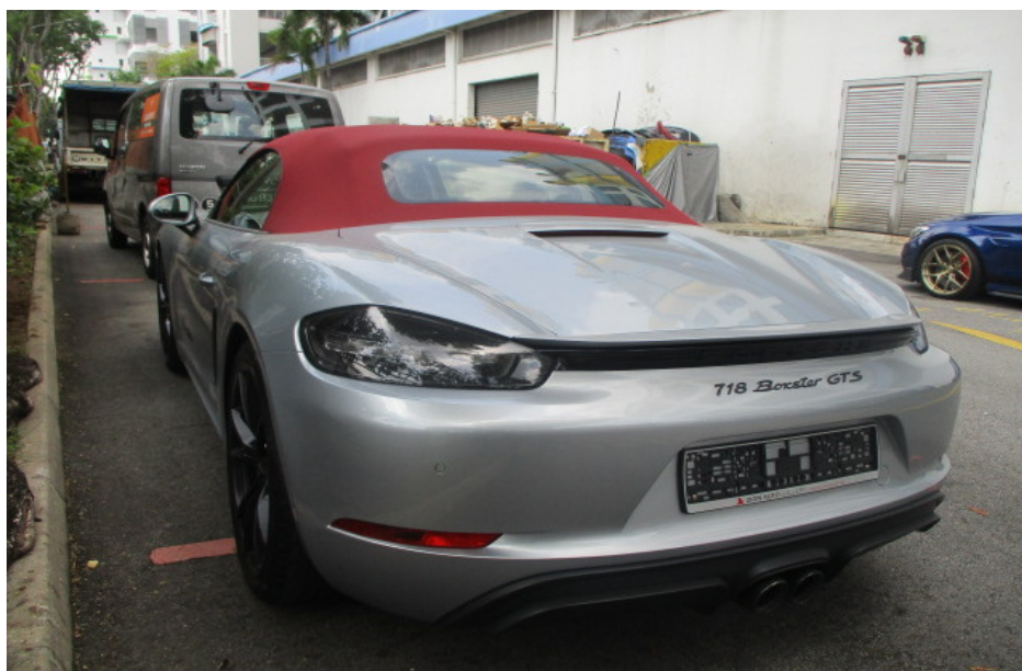
Photo 13 shows a general view of the rear left body of the Motor Car at the time of my inspection. The Motor Car was observed to be in a relatively good general condition with no loose exterior fittings observed. The body parts at the left side portion of the Motor Car were visually examined and it was observed that the repair/restoration works carried out to the damaged area of the Motor Car (refer to photograph 1 & 3 above) were reasonably adequate and in order.
