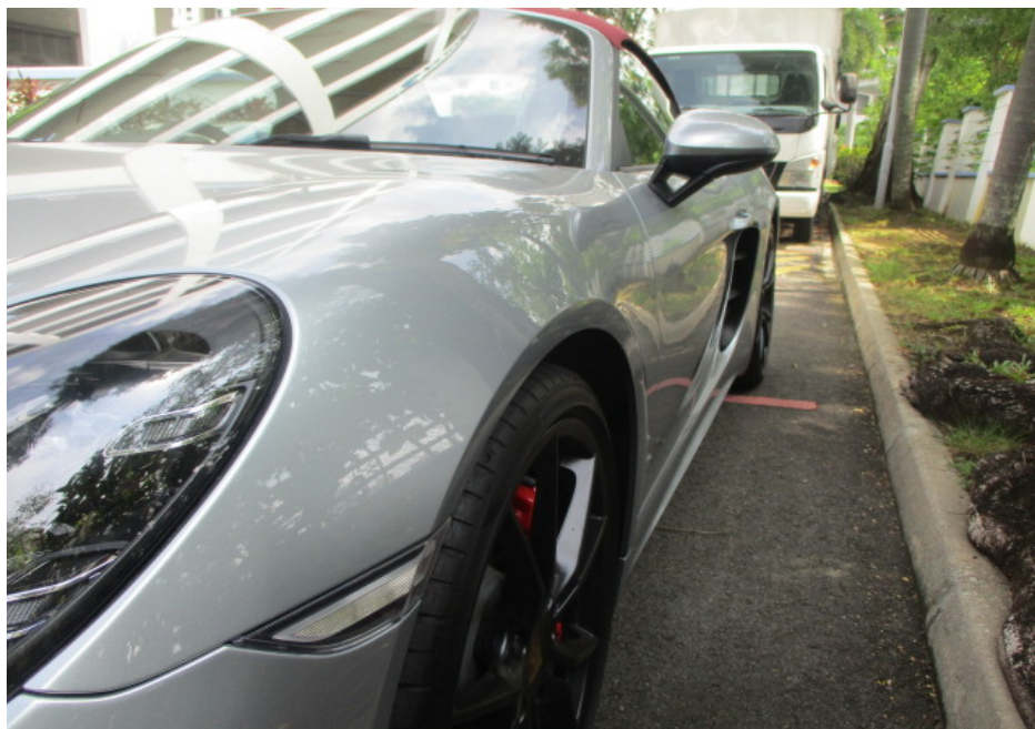
Photo 8 shows a closer view of the Motor Car's front left headlamp, front left signal lamp, front left fender and front left wing mirror. The body parts at the left side portion of the Motor Car were visually examined and it was observed that the repair/restoration works carried out to the damaged area of the Motor Car (refer to photograph 1 & 3 above) were reasonably adequate and in order.
