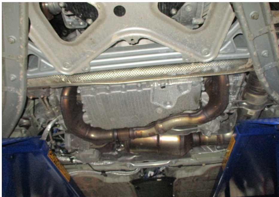
Photo 31 shows the Motor Car's catalytic converters. My examination of the Motor Car's exhaust system revealed no sign(s) or indication(s) of any cut or weld marks along its exhaust pipes, on its catalytic converters and on its rear mufflers.
