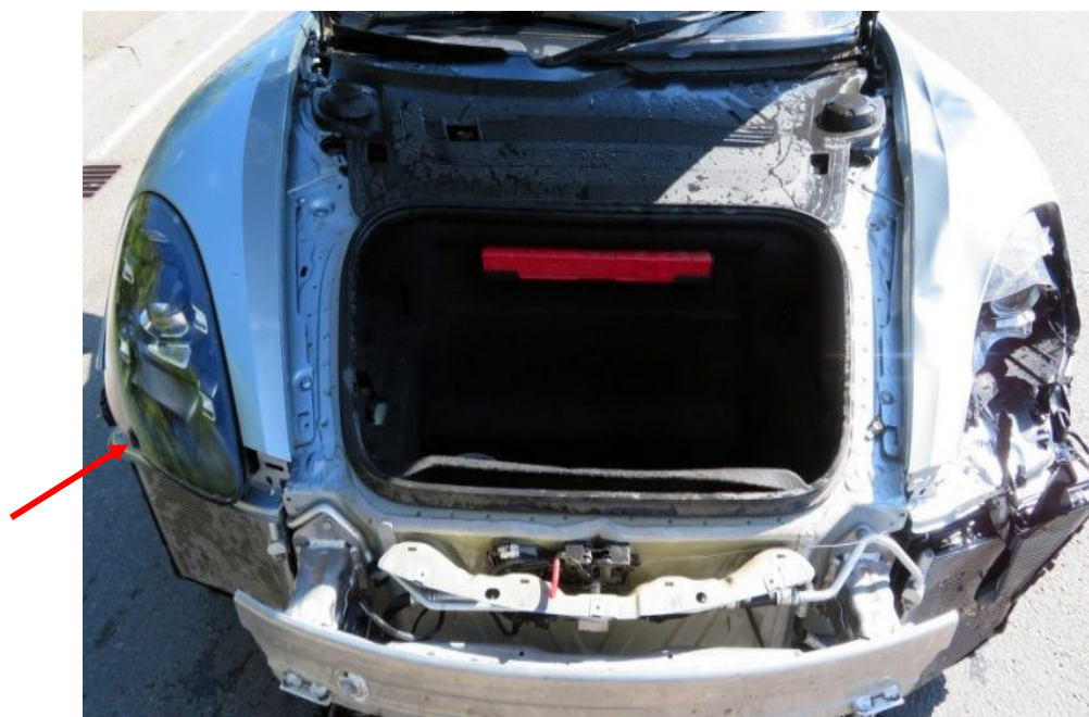
Photo 2 shows the front bonnet compartment of the Motor Car (photograph provided to me). The front right headlamp was observed to be damaged (arrowed) whilst the front bumper and front bonnet compartment inner trims amongst others were observed to be missing/dislodged/damaged.
