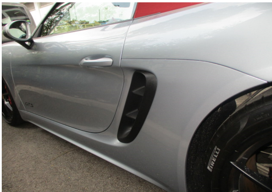
Photo 15 shows a closer view of the Motor Car's rear left fender, front left door, front left door outer handle, left side rocker panel garnish and left side air vent. The body parts at the left side portion of the Motor Car were visually examined and it was observed that the repair/restoration works carried out to the damaged area of the Motor Car (refer to photograph 3 above) were reasonably adequate and in order.
