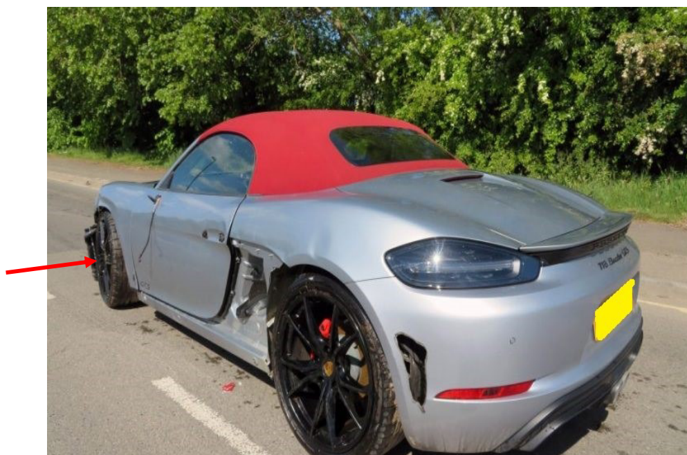
Photo 3 shows the rear left body of the Motor Car (photograph provided to me). The Motor Car was observed to have sustained damage along its entire left side. The rear bumper, rear left fender, front left door, front left door outer handle, front left wing mirror, left side air vent and left side rocker panel garnish were amongst the body parts that were observed to have been damaged. The orientation of the front left wheel (arrowed) and front right wheel (refer to photograph 4 below) suggest damage to the front undercarriage parts of the Motor Car.
