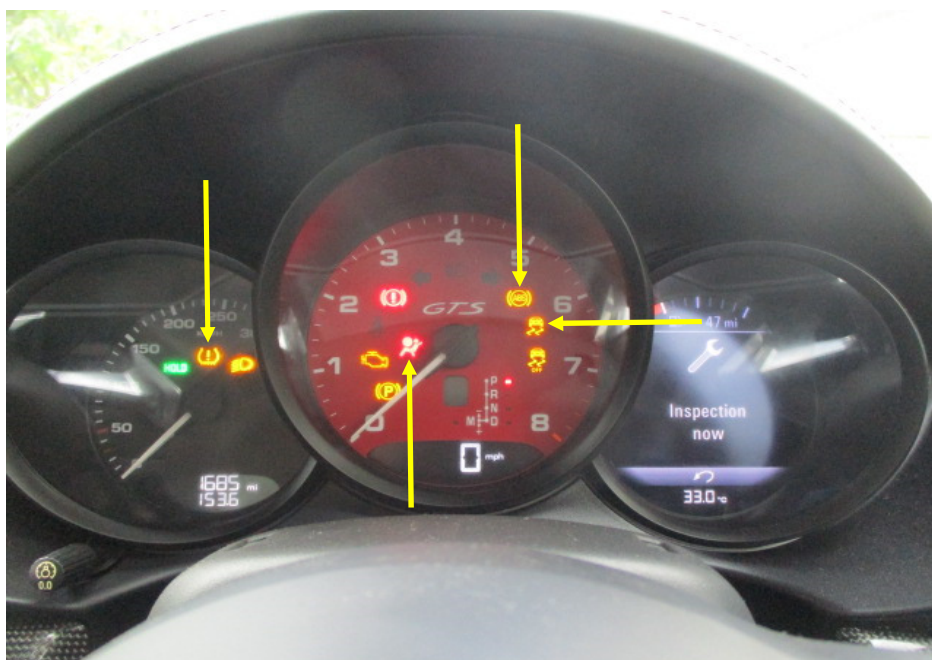
Photo 23 shows the warning lights for the various electronic safety features appearing on the instrument panel of the Motor Car during its self-test when the engine is cranked, in particular the ABS, SRS, TPM and TCS lights (arrowed).
