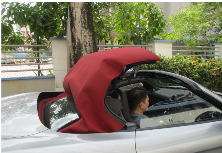
Photo 21 shows the Motor Car's soft top being tested. It was observed that as a safety feature, the soft top roof could only open and close when the Motor Car was in a stationary position. When in an open position, the soft top roof is completely folded into its rear compartment with no parts protruding out of the Motor Car's body. The soft top roof was also found adequately secured to the "A" pillar after closing.
