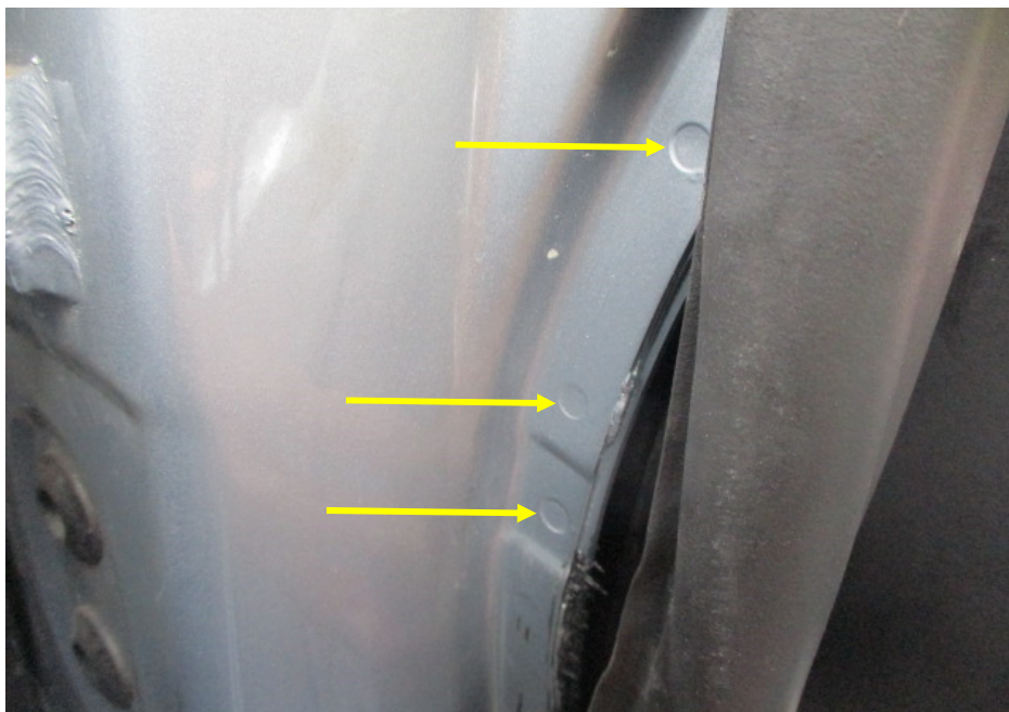
Photo 40 shows the left side "A" pillar of the Motor Car. I did not find any weld marks other than original spot weld marks (arrowed) on the left side "A" pillar of the Motor Car, which indicates that there was no re-welding works carried out. In general, I had found all the non-detachable body panels of the Motor Car to be originally fitted at the time of my inspection.
