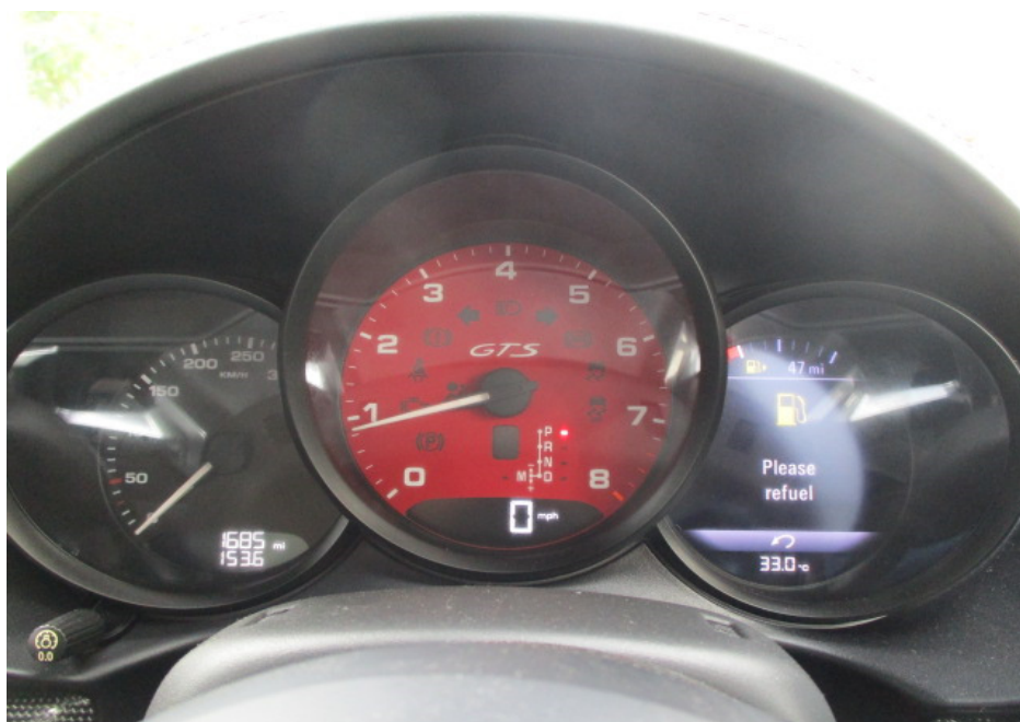
Photo 24 shows the respective warning lights no longer illuminated, indicating that there is no fault detected to the ABS, SRS, TPM and TCS systems of the Motor Car during the self-test. These electronic systems were hence in working condition at the time of my inspection.
