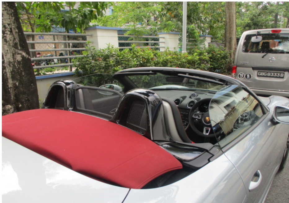
Photo 22 shows the Motor Car with its soft top roof in an open position. When in an open position, the soft top roof is completely folded into its rear compartment with no parts protruding out of the Motor Car's body. The soft top roof was also found adequately secured to the "A" pillar after closing.
