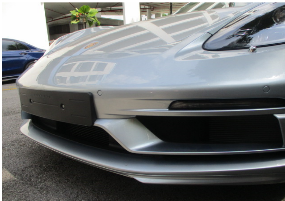
Photo 7 shows a closer view of the Motor Car's front bumper, front bumper lower spoiler, front bumper sensors, front left headlamp and front left day light. The body parts at the frontal portion of the Motor Car were visually examined and it was observed that the repair/restoration works carried out to the damaged area of the Motor Car (refer to photograph 1 & 2 above) were reasonably adequate and in order.
