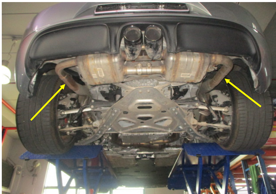
Photo 30 shows the Motor Car's rear mufflers (arrowed). My examination of the Motor Car's exhaust system revealed no sign(s) or indication(s) of any cut or weld marks along its exhaust pipes, on its catalytic converters and on its rear mufflers.
