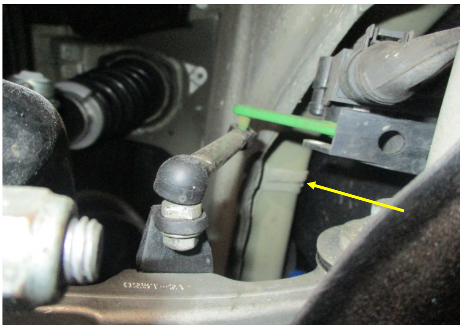
Photo 37 shows the chassis/structural body at the underside front left of the Motor Car. The original factory sealant (arrowed) at the joints along the chassis/structural body was observed to be untouched. In general, I had found no work was carried out on the chassis/structural body of the Motor Car. The chassis/structural body of the Motor Car was originally fitted.
