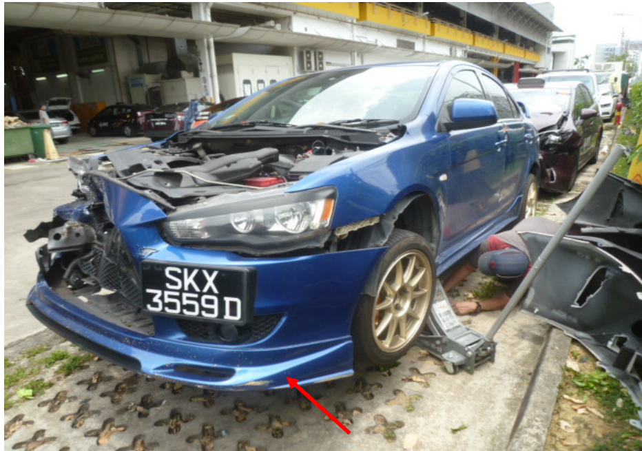
Photo 16 shows a general view of the aftermarket front bumper found fitted onto the Insured Vehicle at the time of our inspection (arrowed).
