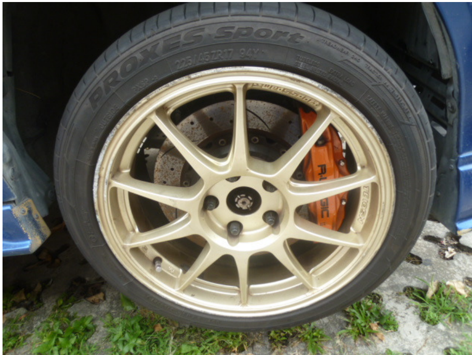
Photo 11 shows the non-standard rim found to be fitted on the Insured Vehicle at the time of our inspection. The 17- inch alloy rims fitted on the Insured Vehicle were not the standard type for the Insured Vehicle.
