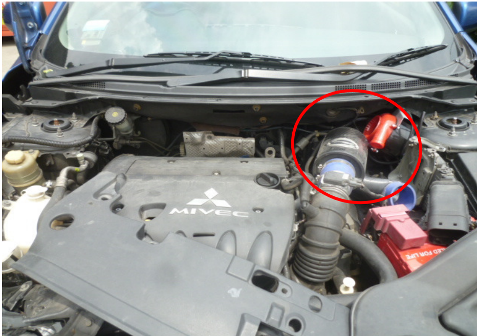
Photo 6 shows a general view of the engine compartment of the Insured Vehicle. Additional non-standard parts were found fitted. This includes a non- standard open- pod air filter and universal turbine electronic turbo blow- off valve simulator (circled).
