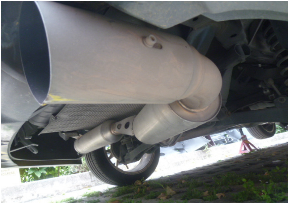
Photo 12 shows a front view of the non-standard rear exhaust muffler that was found to be fitted on the Insured Vehicle at the time of our inspection.
