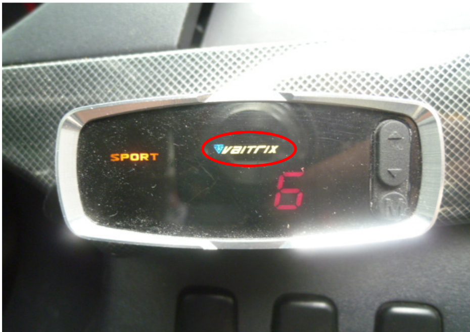
Photo 9 shows the electronic throttle controller additionally fitted onto the Insured Vehicle upon our inspection. The brand of the throttle controller was 'VAITRIX' (circled).
