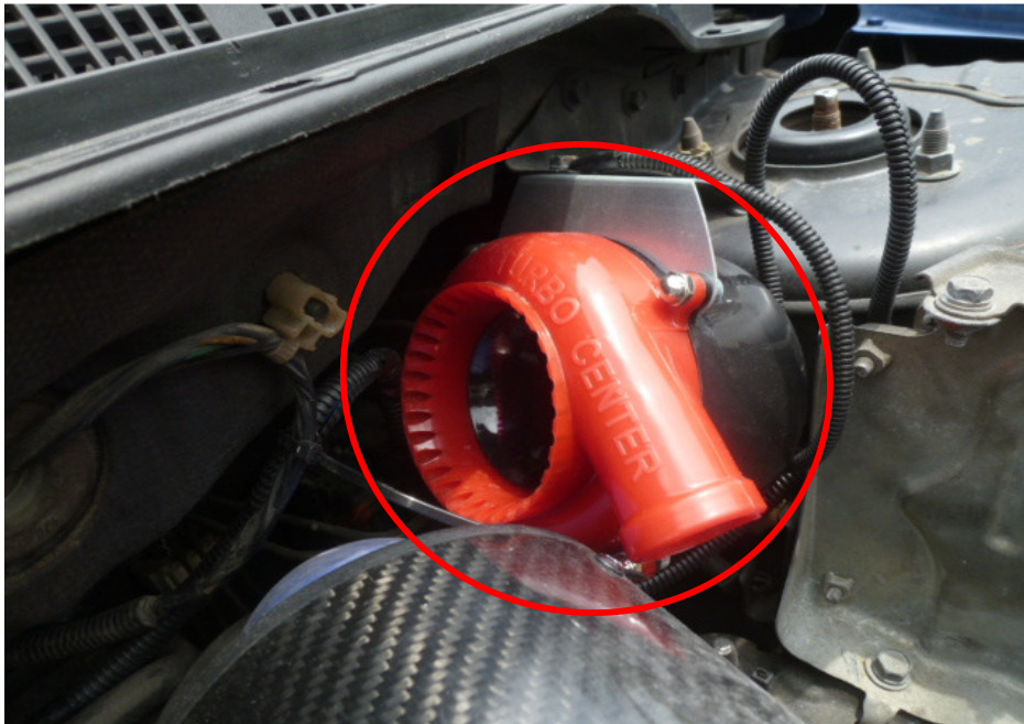
Photo 8 shows a close up view of the non- standard universal turbine electronic turbo blow- off valve simulator fitted onto the Insured Vehicle upon our inspection (circled).
