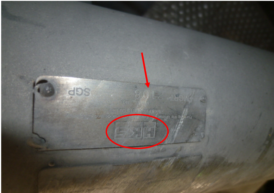
Photo 13 shows a close up view of the underside of the non-standard rear exhaust muffler that was found to be fitted on the Insured Vehicle at the time of our inspection. The brand of the rear exhaust muffler was 'HKS' (circled). The serial number of the rear exhaust muffler was '2108' (arrowed).
