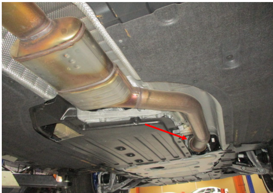
Photo 25 shows the front section of the Motor Car's exhaust system. My examination of the Motor Car's exhaust system revealed no sign(s) or indication(s) of any cut or weld marks along its exhaust pipes, on its rear muffler, on its centre resonator box and on its catalytic converter (arrowed).
