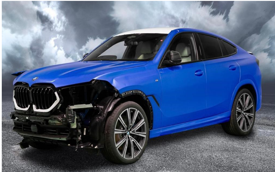
Photo 1 shows the front left body of the Motor Car (photograph provided to me). The photographs provided to me had showed damage to the frontal portion of the Motor Car. Body parts damaged include the front left fender and front left fender wheel arc garnish amongst others. The front left day light, front left headlamp, front bumper and all its related parts and attachments like the front bumper centre lower grille, front bumper left lower grille and front bumper sensors amongst others were observed to be damaged/dislodged/missing.
