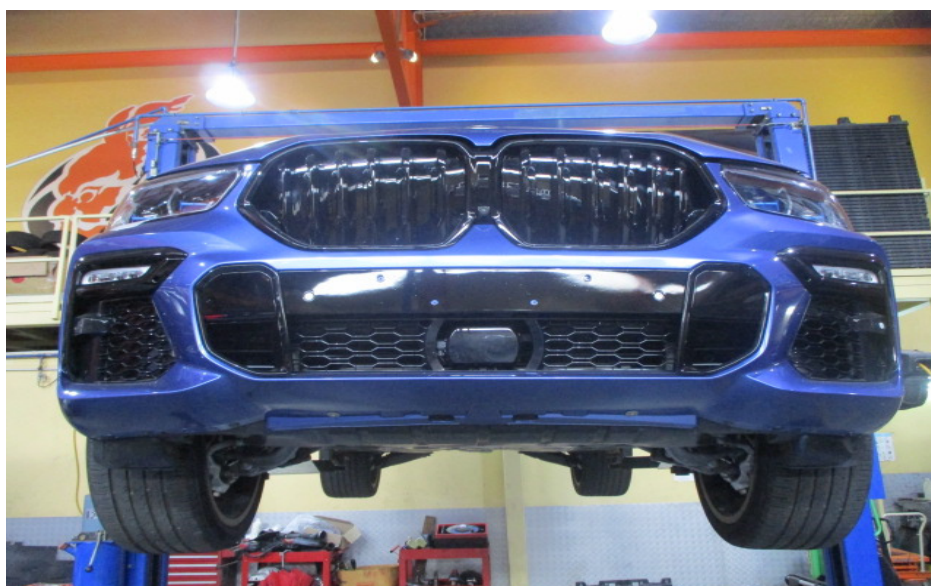
Photo 19 shows the Motor Car hoisted up for checks on its undercarriage. There was no sign(s) or indication(s) of fluid leakage and/or fluid stain(s) on the underside of the Motor Car. The undercarriage components of the Motor Car were also all observed to be intact and secured in an appropriate manner.
