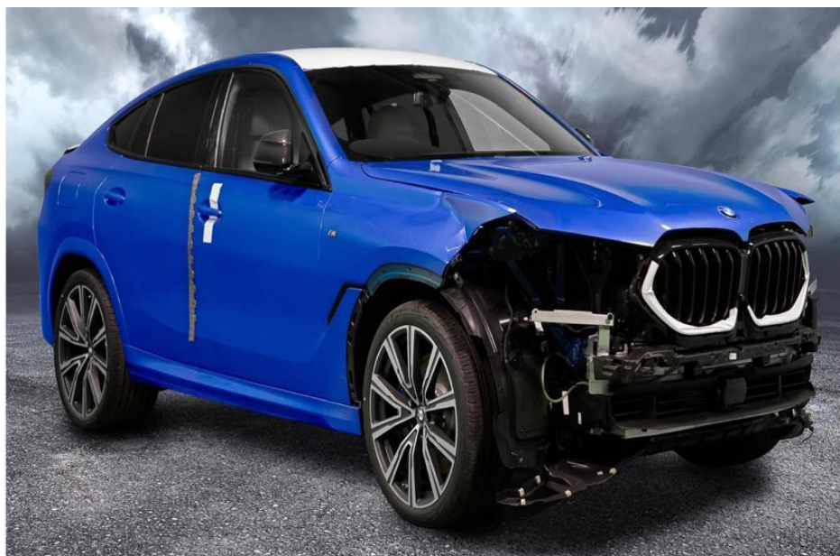
Photo 2 shows the front right body of the Motor Car (photograph provided to me). The photographs provided to me had showed damage to the frontal portion of the Motor Car. Body parts damaged include the front right fender and front right fender wheel arc garnish amongst others. The front right day light, front right headlamp, front bumper and all its related parts and attachments like the front bumper centre lower grille, front bumper right lower grille and front bumper sensors amongst others were observed to be damaged/dislodged/missing.
