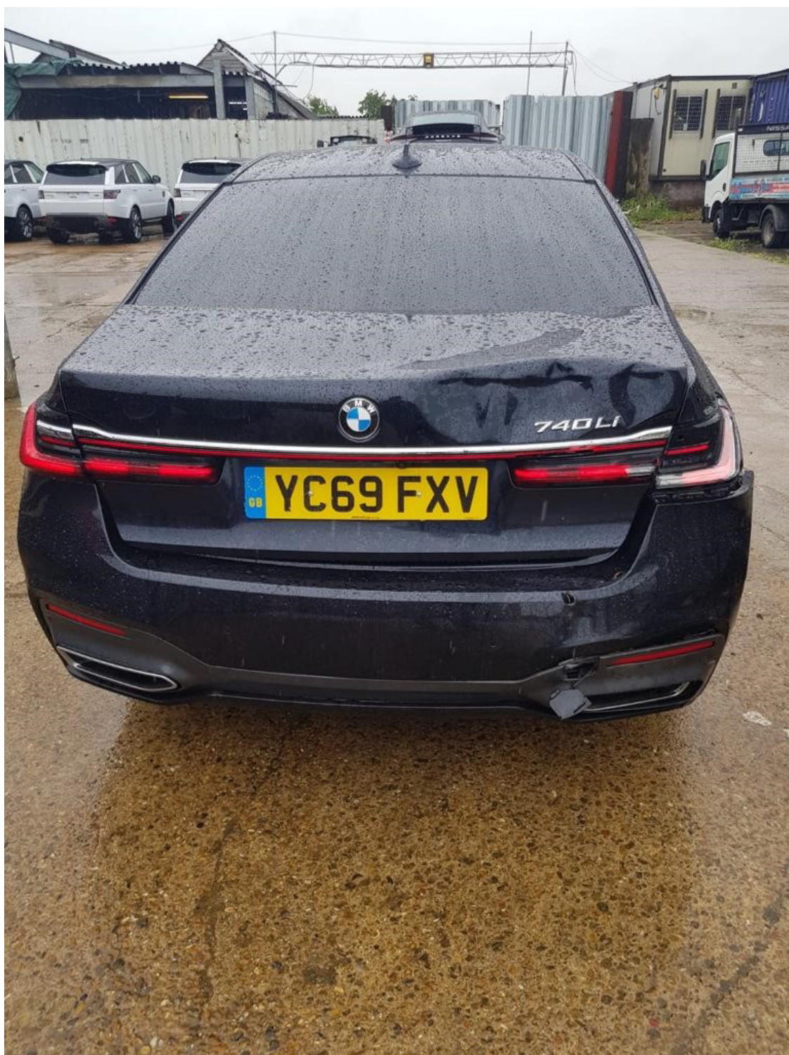
Photo 1 shows the rear body of the Motor Car (photograph provided to me). The Motor Car was observed to have sustained damage at its rear right portion. Body parts damaged include the rear bumper, rear bumper lower cover, rear bootlid, rear bootlid upper chrome moulding, rear bootlid upper reflector, rear right bootlid lamp and rear right taillamp amongst others.
