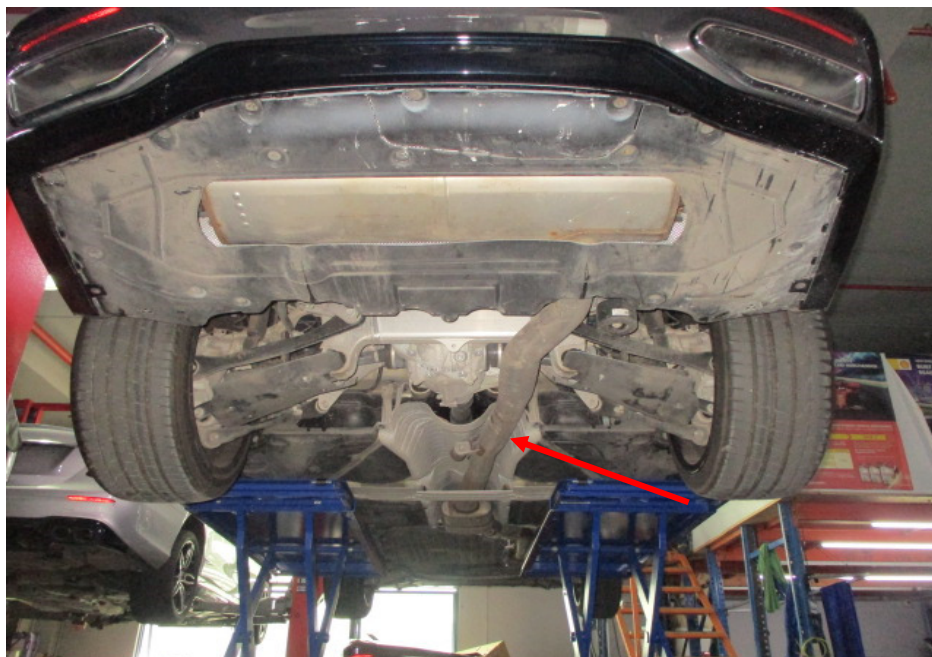
Photo 20 shows a general view of the rear section of the Motor Car's exhaust system. My examination of the Motor Car's exhaust system revealed no sign(s) or indication(s) of any cut or weld marks along its exhaust pipes (arrowed), on its centre resonator box, on its catalytic converter and on its rear muffler.
