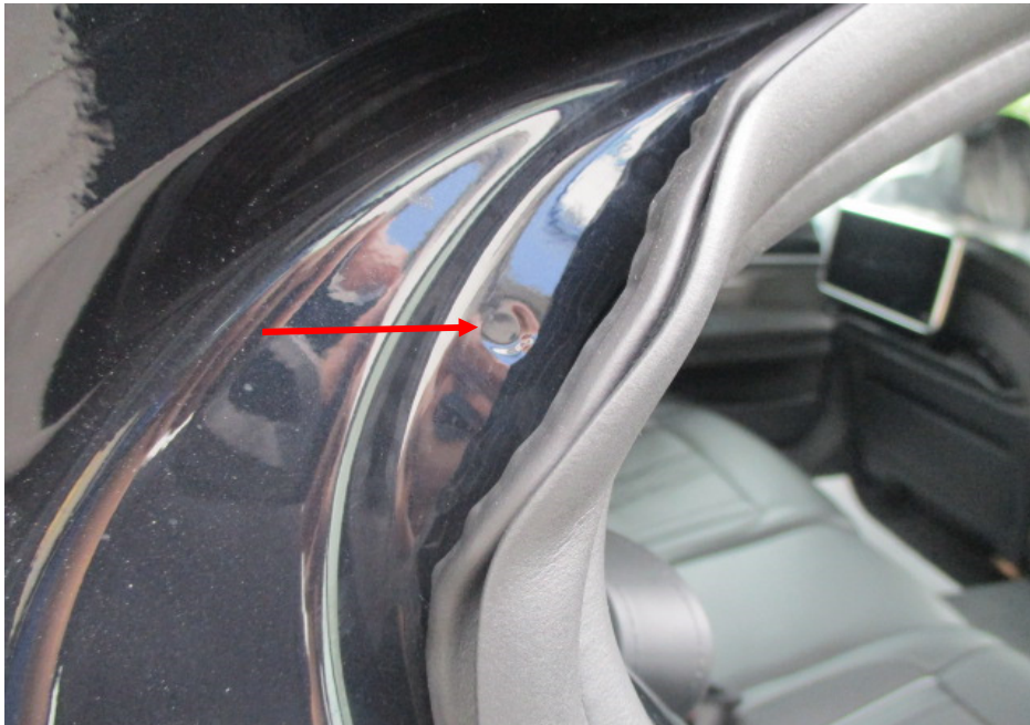
Photo 26 shows the right side "C" pillar of the Motor Car. I did not find any weld marks other than original spot weld marks (arrowed) on the right side "C" pillar of the Motor Car which, indicates that there was no re-welding works carried out. In general, I had found all the non-detachable body panels of the Motor Car to be originally fitted at the time of my inspection.
