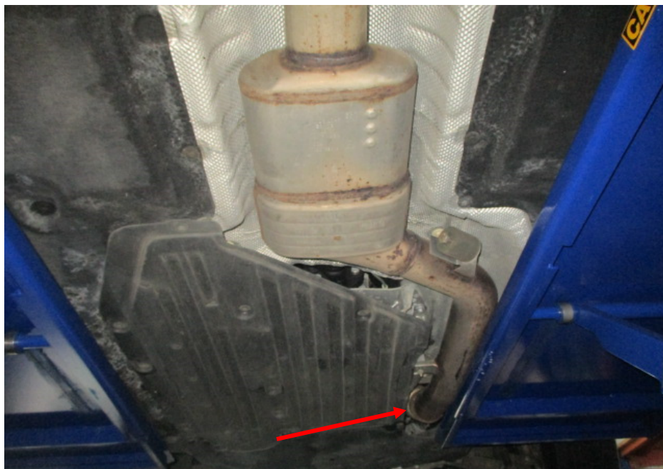
Photo 21 shows a general view of the front section of the Motor Car's exhaust system. My examination of the Motor Car's exhaust system revealed no sign(s) or indication(s) of any cut or weld marks along its exhaust pipes, on its centre resonator box, on its catalytic converter (arrowed) and on its rear muffler.
