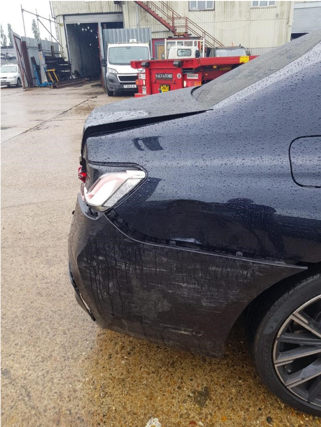
Photo 2 shows another view of the damaged rear bumper, rear bootlid and rear right taillamp of the Motor Car (photograph provided to me).
