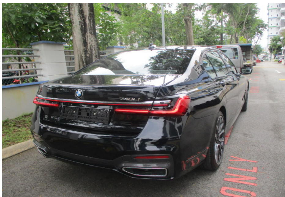
Photo 3 shows a general view of the rear right body of the Motor Car at the time of my inspection. The Motor Car was observed to be in a relatively good general condition with no loose exterior fittings observed. The body parts at the rear right portion of the Motor Car were visually examined, and it was observed that the repair/restoration works carried out to the damaged area of the Motor Car (refer to photograph 1 & 2) were reasonably adequate and in order.
