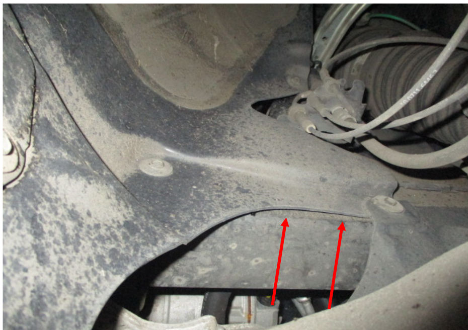
Photo 23 shows the chassis/structural body at the underside front left of the Motor Car. The original factory sealant (arrowed) at the joints along the chassis/structural body was observed to be untouched. In general, I had found no work was carried out on the chassis/structural body of the Motor Car. The chassis/structural body of the Motor Car was originally fitted.
