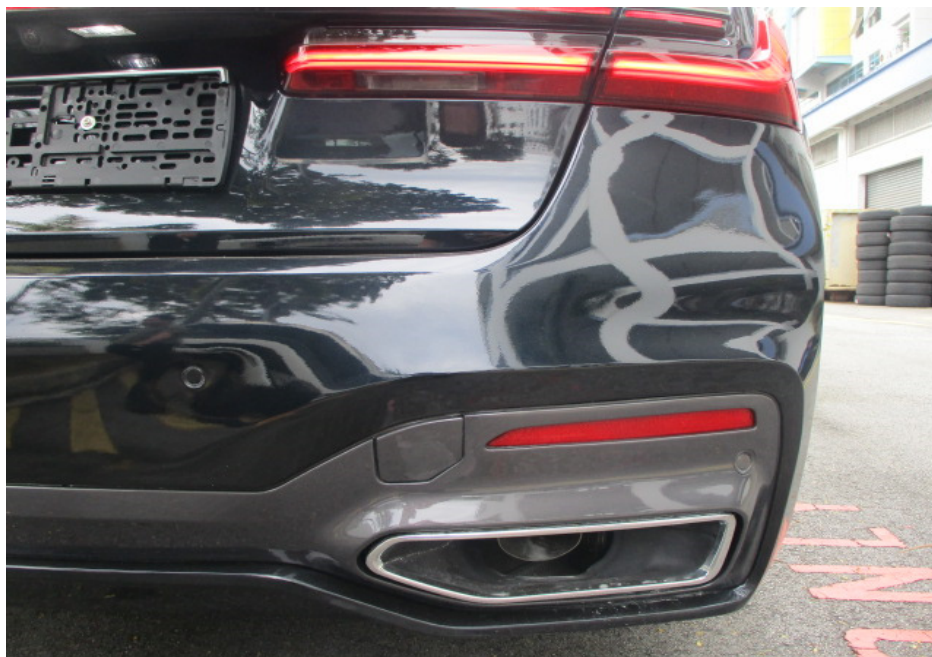
Photo 4 shows a closer view of the Motor Car's rear bumper, rear bumper lower cover, rear right bootlid lamp and rear right taillamp. The body parts at the rear right portion of the Motor Car were visually examined, and it was observed that the repair/restoration works carried out to the damaged area of the Motor Car (refer to photograph 1 & 2 above) were reasonably adequate and in order.
