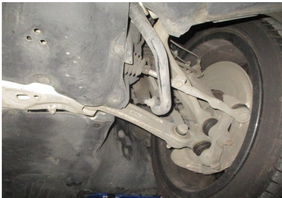
Photo 18 shows the various undercarriage components at the front left wheel of the Motor Car. The mechanical components, control arms and linkages were all found to be intact and secured in an appropriate manner.
