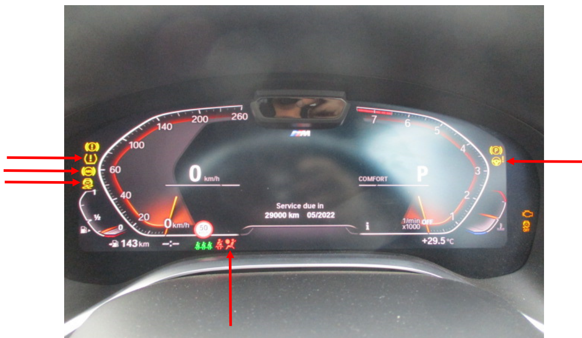
Photo 13 shows the warning lights for the various electronic safety features appearing on the instrument panel of the Motor Car during its self-test when the engine is cranked, in particular the ABS, SRS, IAS, TPM and DSC lights (arrowed).
