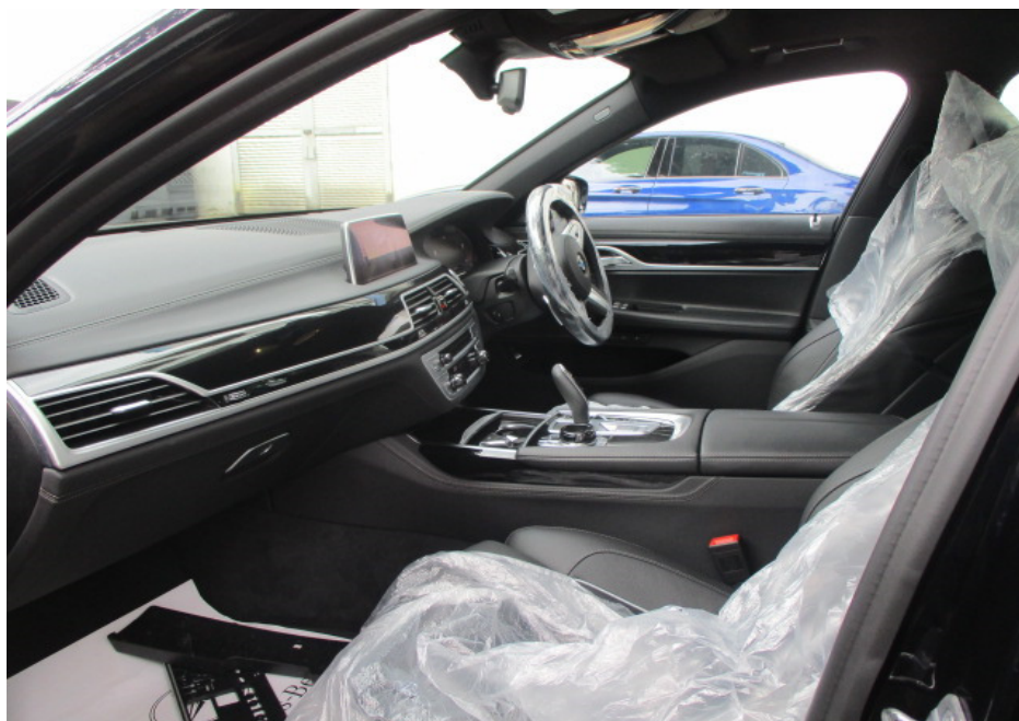
Photo 11 shows the interior compartment of the Motor Car at the time of my inspection. The various parts and components, trims, carpet and upholstery inside the interior compartment were all observed to be intact and properly fitted.
