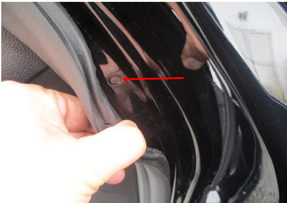
Photo 27 shows the right side "A" pillar of the Motor Car. I did not find any weld marks other than original spot weld marks (arrowed) on the right side "A" pillar of the Motor Car which, indicates that there was no re-welding works carried out. In general, I had found all the non-detachable body panels of the Motor Car to be originally fitted at the time of my inspection.
