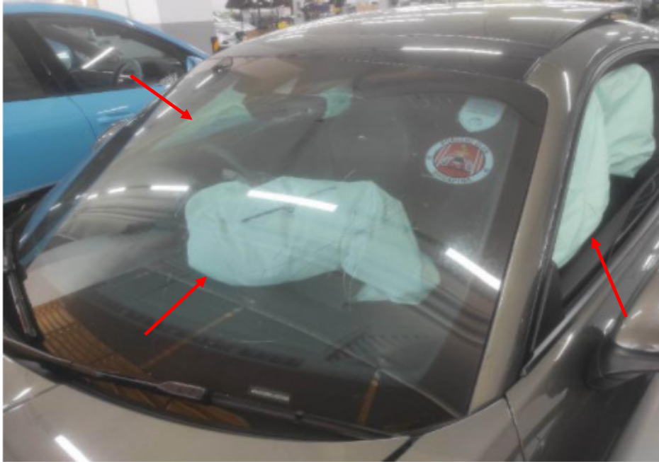
Photo 8 shows the remains of the front and side airbags in the interior compartment of the Insured Vehicle (arrowed) which corroborates with Mr Tan's statement that the airbags were deployed post- incident.
