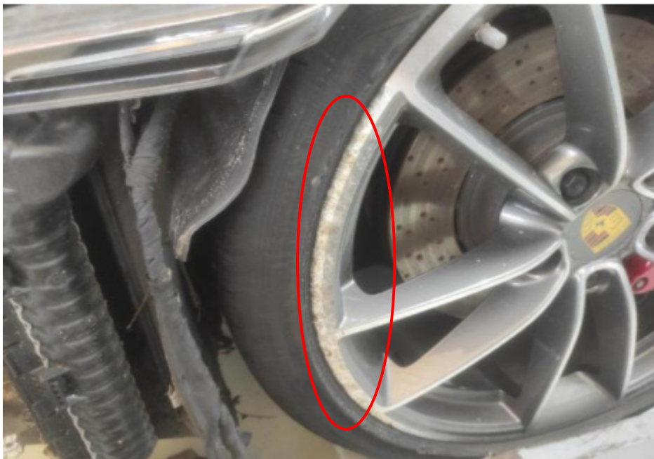
Photo 9 shows some relatively minor marks of grazing nature observed around the edges of the front left wheel rim (circled) as a result of Mr Tan grazing the railings.
