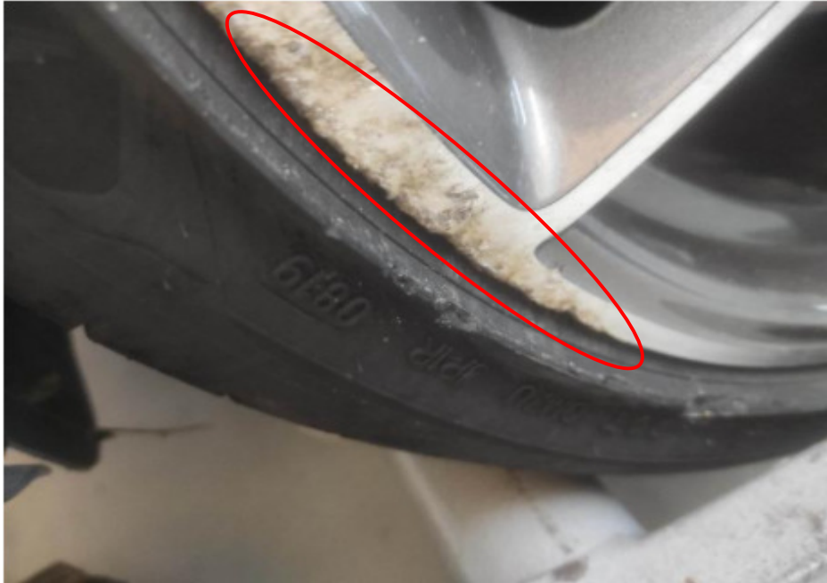
Photo 10 shows a close up view of the relatively minor marks of grazing nature observed around the edges of the front left wheel rim (circled) as a result of Mr Tan grazing the railings.
