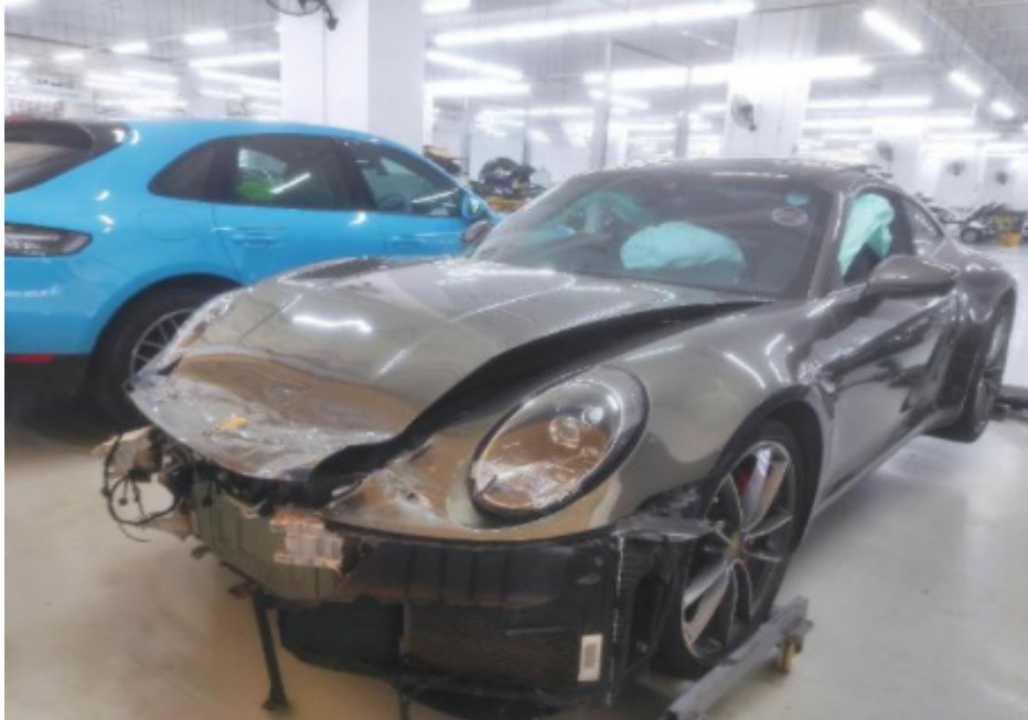
Photo 6 shows the frontal portion of the Insured during the physical inspection at Stuttgart. The Insured Vehicle had sustained significant damages to its frontal portion, particularly to its front bonnet, front bumper, front fenders and headlamps as a result of the incident.
