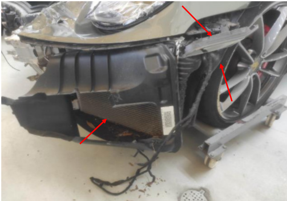
Photo 7 shows upon closer inspection, the Insured Vehicle also sustained damages to the front bumper retainer, left front fender shield and radiator (arrowed).
