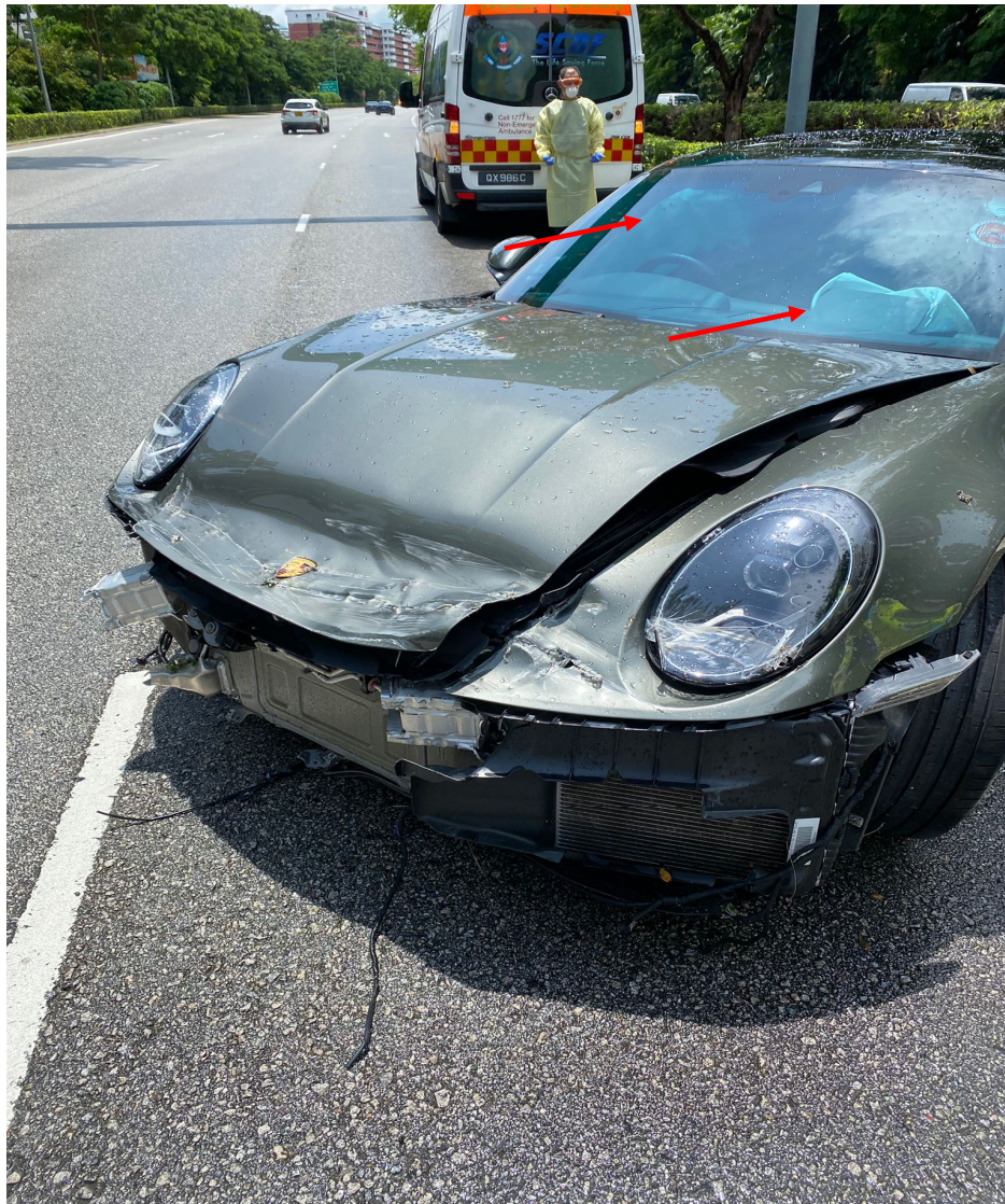
Photo 4 shows the frontal portion of the Insured Vehicle post- incident. The Insured Vehicle had sustained damages at its frontal portion. The deployed airbags in the Insured Vehicle (arrowed) correlates with Mr Tan's statement that the front and side airbags were deployed after the Insured Vehicle spun out of control and collided into the railings after he drove through a puddle of water.
