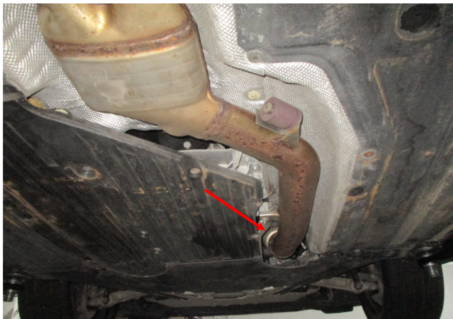
Photo 26 shows the front section of the Motor Car's exhaust system. My examination of the Motor Car's exhaust system revealed no sign(s) or indication(s) of any cut or weld marks along its exhaust pipes, on its rear muffler, on its centre resonator box and on its catalytic converter (arrowed).
