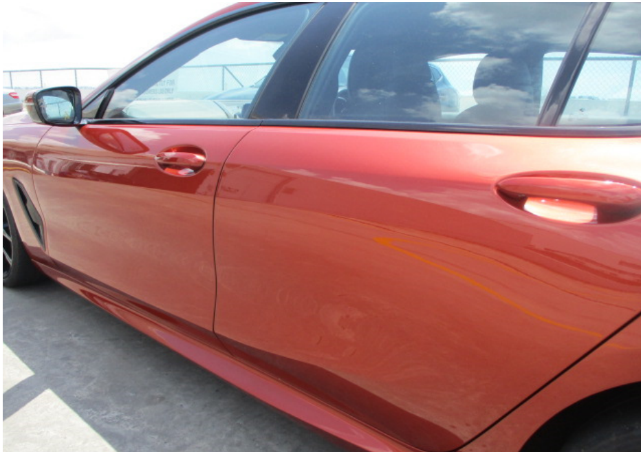
Photo 10 shows a closer view of the Motor Car's rear left door, rear left door outer handle cover and front left door. The body parts along the entire left side portion of the Motor Car were visually examined and it was observed that the repair/restoration works carried out to the damaged area of the Motor Car (refer to photograph 1 - 4 above) were reasonably adequate and in order.
