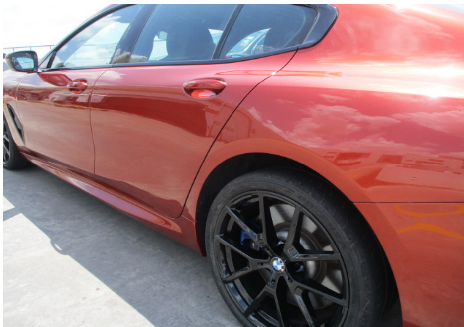
Photo 9 shows a closer view of the Motor Car's rear left fender, rear left wheel rim and rear left door. The body parts along the entire left side portion of the Motor Car were visually examined and it was observed that the repair/restoration works carried out to the damaged area of the Motor Car (refer to photograph 1 - 4 above) were reasonably adequate and in order.
