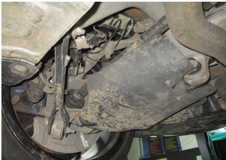
Photo 24 shows the various undercarriage components at the rear right wheel of the Motor Car. The mechanical components, control arms and linkages were all found to be intact and secured in an appropriate manner. I also did not observe any fluid leak and/or fluid stain on the underside of the Motor Car.
