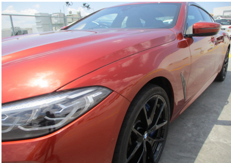
Photo 12 shows a closer view of the Motor Car's front bumper and front left fender. The body parts along the entire left side portion of the Motor Car were visually examined and it was observed that the repair/restoration works carried out to the damaged area of the Motor Car (refer to photograph 1 - 4 above) were reasonably adequate and in order.
