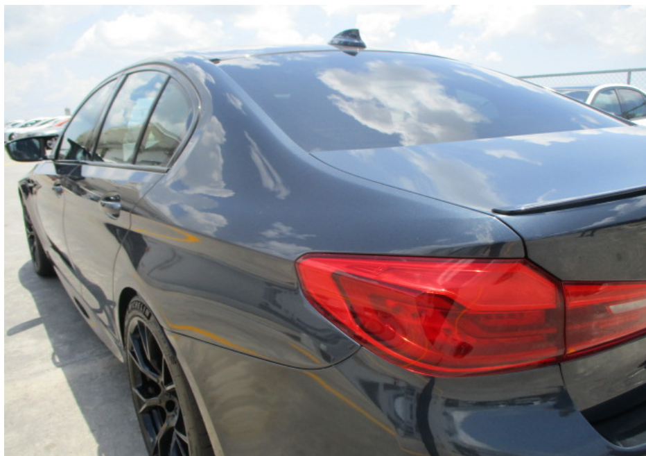
Photo 13 shows a closer view of the Motor Car's rear bumper, rear left taillamp and rear left fender. The body parts at the rear left portion of the Motor Car were visually examined and it was observed that the repair/restoration works carried out to the damaged area of the Motor Car (refer to photograph 4 & 5 above) were reasonably adequate and in order.
