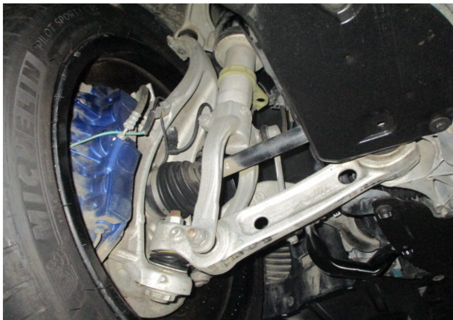
Photo 24 shows the various undercarriage components at the front left wheel of the Motor Car. The mechanical components, control arms and linkages were all found to be intact and secured in an appropriate manner. I also did not observe any fluid leak and/or fluid stain on the underside of the Motor Car.
