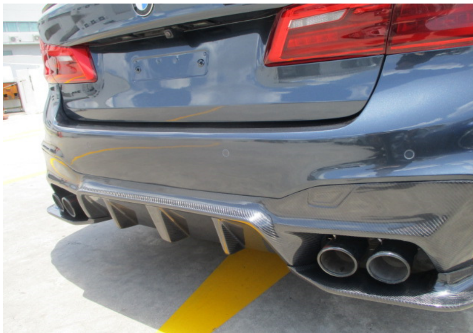
Photo 15 shows a closer view of the Motor Car's rear bumper, rear bumper lower garnish, rear bumper sensors and rear right exhaust muffler. The body parts at the rear portion of the Motor Car were visually examined and it was observed that the repair/restoration works carried out to the damaged area of the Motor Car (refer to photograph 4 & 6 above) were reasonably adequate and in order.
