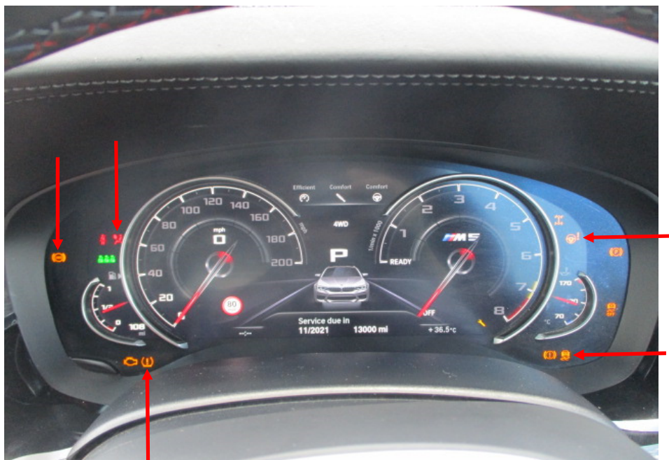
Photo 20 shows the warning lights for the various electronic safety features appearing on the instrument panel of the Motor Car during its self-test when the engine is cranked, in particular the ABS, SRS, IAS, TPM and DSC lights (arrowed).
