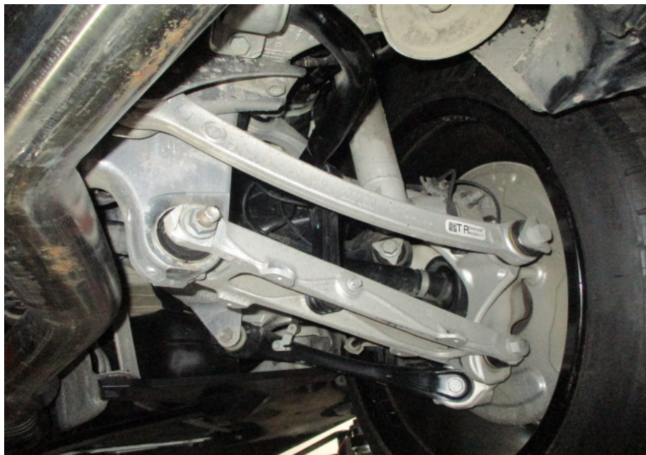
Photo 26 shows the various undercarriage components at the rear right wheel of the Motor Car. The mechanical components, control arms and linkages were all found to be intact and secured in an appropriate manner. I also did not observe any fluid leak and/or fluid stain on the underside of the Motor Car.
