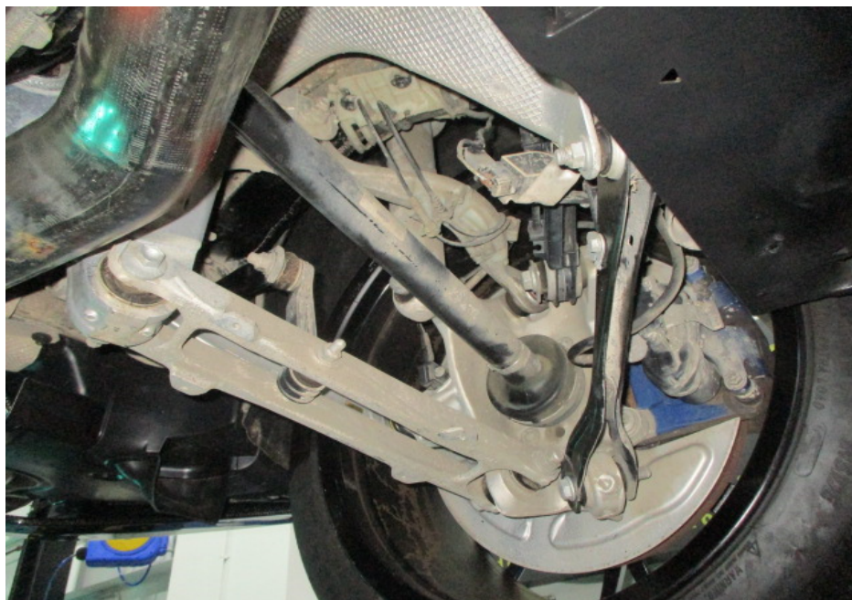
Photo 25 shows the various undercarriage components at the rear left wheel of the Motor Car. The mechanical components, control arms and linkages were all found to be intact and secured in an appropriate manner.
