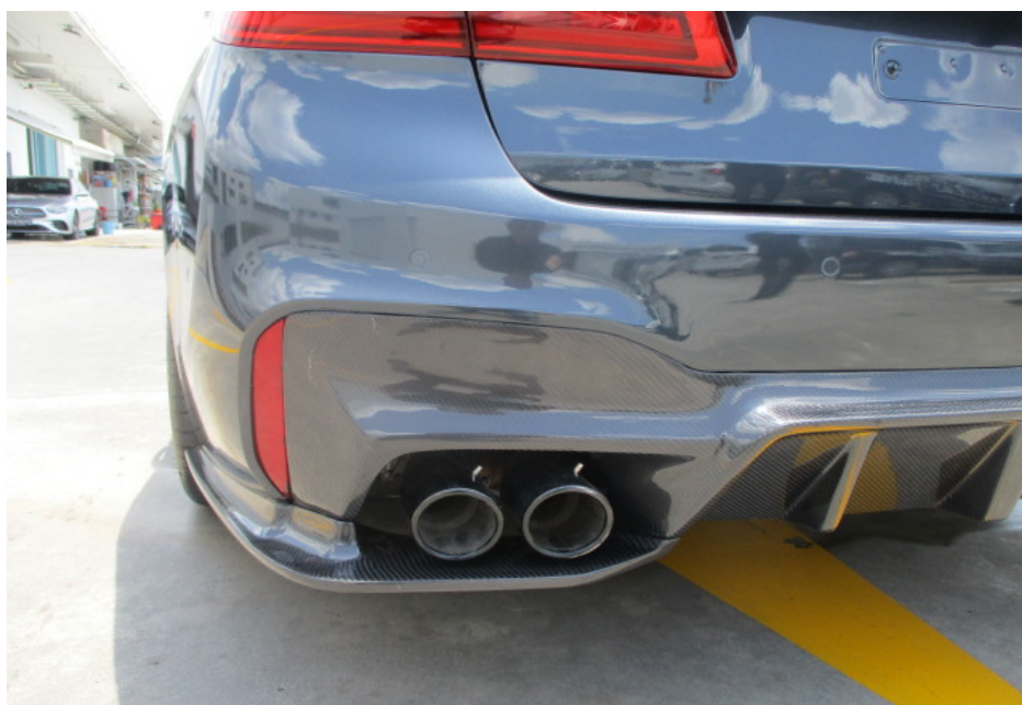
Photo 12 shows a closer view of the Motor Car's rear bumper, rear bumper left reflector, rear bumper lower garnish and rear left exhaust muffler. The body parts at the rear left portion of the Motor Car were visually examined and it was observed that the repair/restoration works carried out to the damaged area of the Motor Car (refer to photograph 4 & 5 above) were reasonably adequate and in order.
