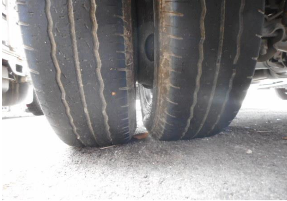
Photo 10 shows the condition of the rear left tyres of the Motor Lorry, which was observed to be in serviceable condition with remaining tread depth of approximately 3mm. The tyres, which were wrapped around standard steel wheel rim, were also observed to be sufficiently inflated for vehicular operation.
