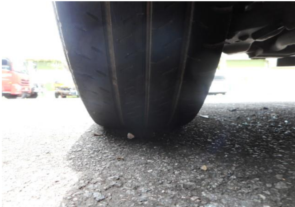
Photo 11 shows the condition of the rear right tyres of the Motor Lorry, which were observed to be in serviceable condition with remaining, tread depth of approximately 5.5mm. There was also no tear, cut or burst mark(s) on the outer and the inner sidewalls as well as across the tread of the 6 tyres that were fitted on the Motor Lorry.
