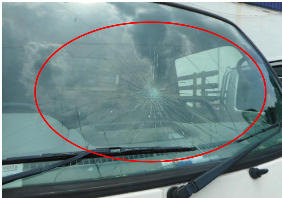
Photo 3 shows a close up view of the Motor Lorry's front portion at the time of my inspection. Its front windscreen (circled) was damage at the time of my inspection as a result of the accident.
