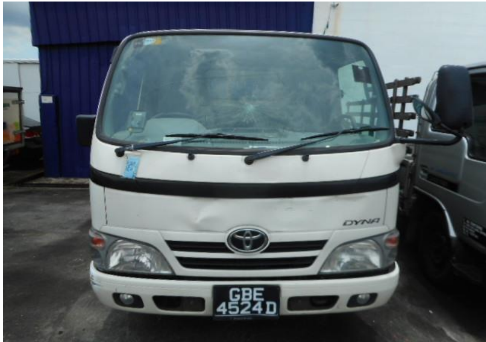
Photo 2 shows a general view of the Motor Lorry's frontal portion at the time of my inspection. It appeared to have sustained damage at its front portion. Its front windscreen, front bumper and front body panel were damage at the time of my inspection as a result of the accident.
