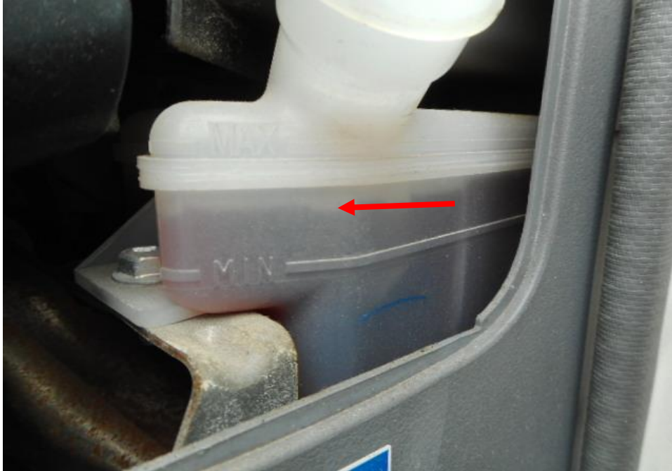
Photo 13 shows the brake fluid reservoir of the Motor Lorry at the time of my inspection. The brake fluid was observed to be of sufficient level (arrowed) and without any visible contamination.
