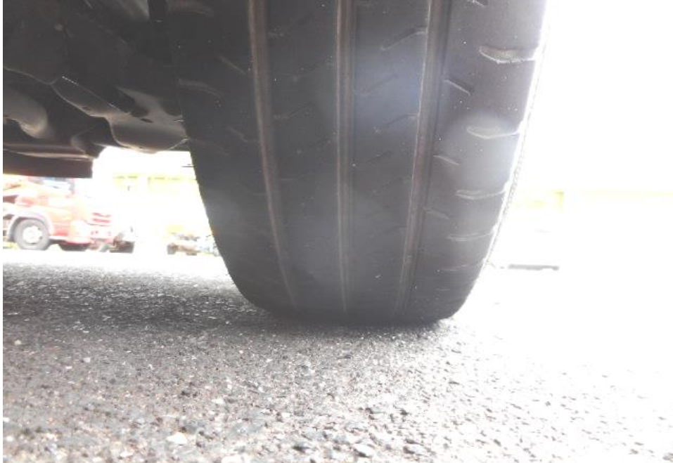
Photo 8 shows the condition of the front right tyre of the Motor Lorry, which was observed to be in serviceable condition with remaining tread depth of approximately 6mm. The tyre, which was wrapped around standard steel wheel rim, was also observed to be sufficiently inflated for vehicular operation. There was no tear, cut or burst mark(s) on the outer and the inner sidewalls as well as across the tread of the 6 tyres that were fitted on the Motor Lorry.
