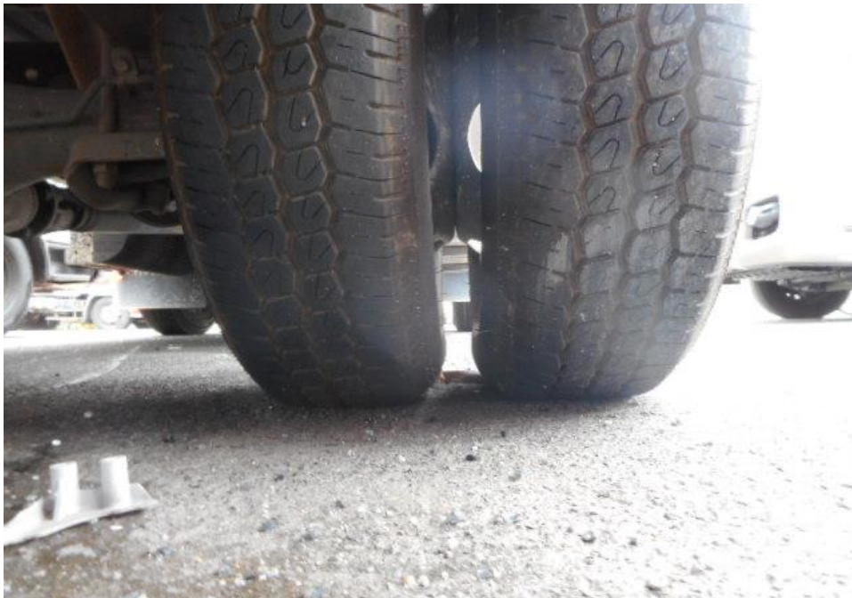
Photo 9 shows the condition of the rear right tyre of the Motor Lorry, which was observed to be in serviceable condition with remaining tread depth of approximately 5.7mm. The tyre, which was wrapped around standard steel wheel rim, it was observed to be sufficiently inflated for vehicular operation.
