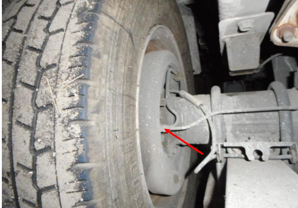
Photo 25 shows the brake pipe (arrowed) at the rear left wheel of the Motor Lorry. I did not observe any leakage of brake fluid at the time of my inspection of the Motor Lorry. My static tests of the Motor Lorry's braking system, along with my visual examination of the various mechanical components in the braking system had indicated that there was no internal leakage of pressure/vacuum. Hence the braking system of the Motor Lorry was likely to be in serviceable condition at the material time of accident.
