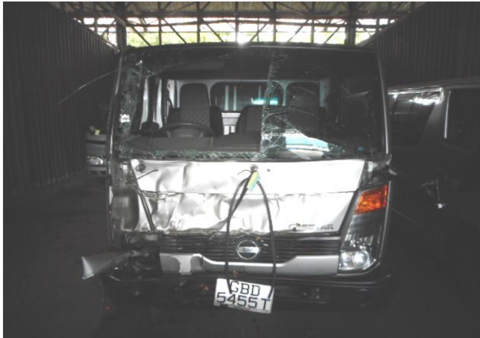
Photo 1 shows a general view of the Motor Lorry's frontal portion at the time of my inspection. It appeared to have sustained damage at its front portion. Its front, right and rear portion. Its front windscreen, front body panel, front right headlamp, front bumper, right door and rear body panel were damage at the time of my inspection as a result of the accident.
