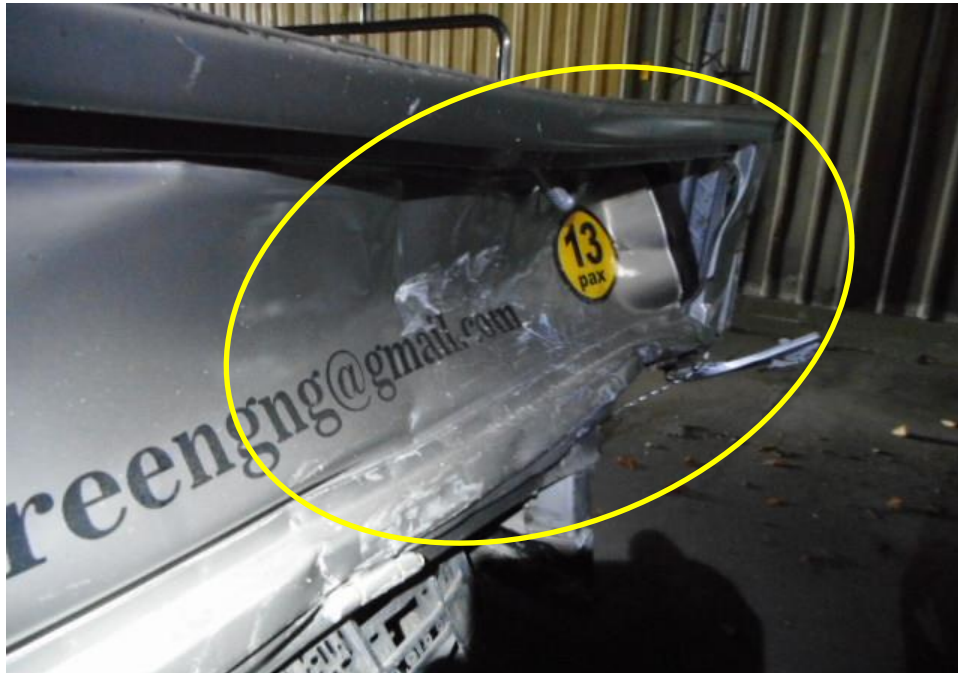
Photo 8 shows a close up view of the rear body of the Motor Lorry at the time of my inspection. Its rear body panel (circled) was damage at the time of my inspection as a result of the accident.
