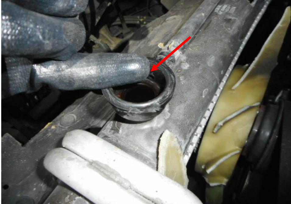
Photo 16 shows the engine coolant reservoir of the Motor Lorry at the time of my inspection. The engine coolant was observed to be of insufficient level (arrowed) as the radiator was damaged as a result of the accident.
