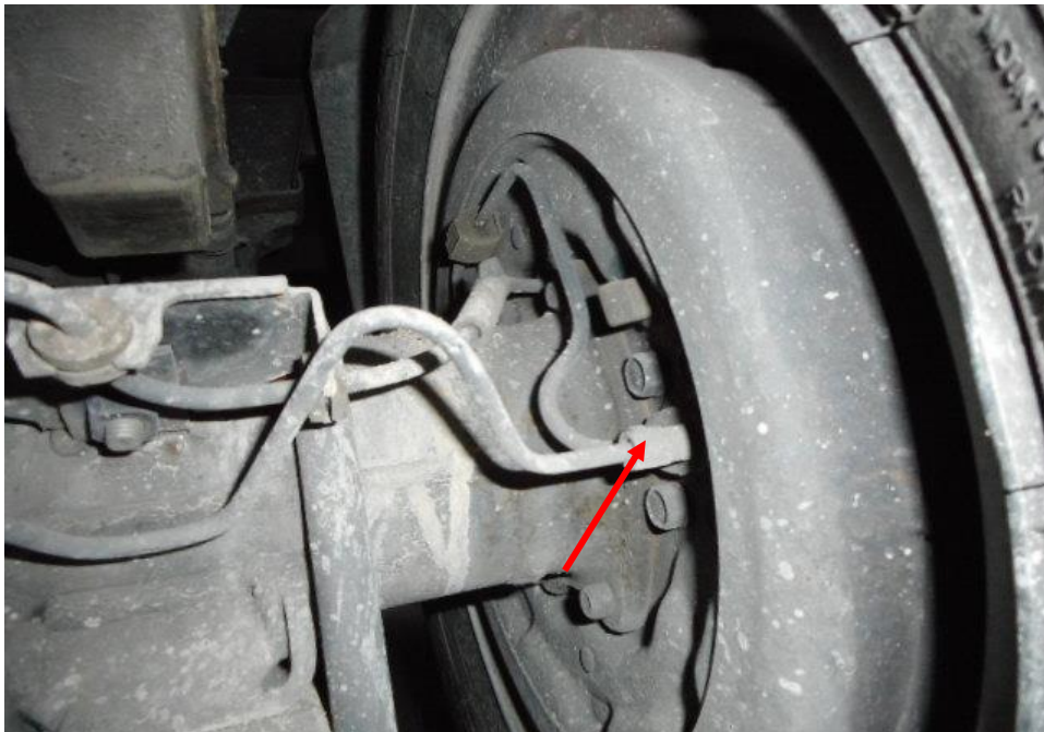
Photo 24 shows the brake pipe (arrowed) at the rear right wheel of the Motor Lorry. I did not observe any leakage of brake fluid at the time of my inspection of the Motor Lorry. My static tests of the Motor Lorry's braking system, along with my visual examination of the various mechanical components in the braking system, had indicated that there was no internal leakage of pressure/vacuum. Hence the braking system of the Motor Lorry was likely to be in serviceable condition at the material time of accident.
