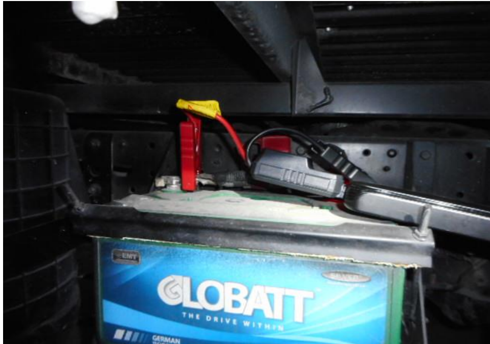
Photo 21 shows the jumpstarting process of the Motor Lorry's engine. The engine of the Motor Lorry's was unable to be jumpstarted up despite multiple attempts in starting it.
