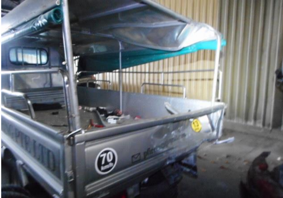
Photo 7 shows a general view of the rear body of the Motor Lorry at the time of my inspection. Its rear body panel (circled) was damage at the time of my inspection as a result of the accident.
