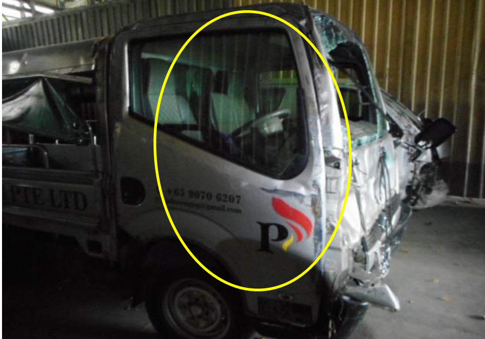
Photo 5 shows a close up view of the right body of the Motor Lorry at the time of my inspection. Its right door (circled) was damage at the time of my inspection as a result of the accident.
