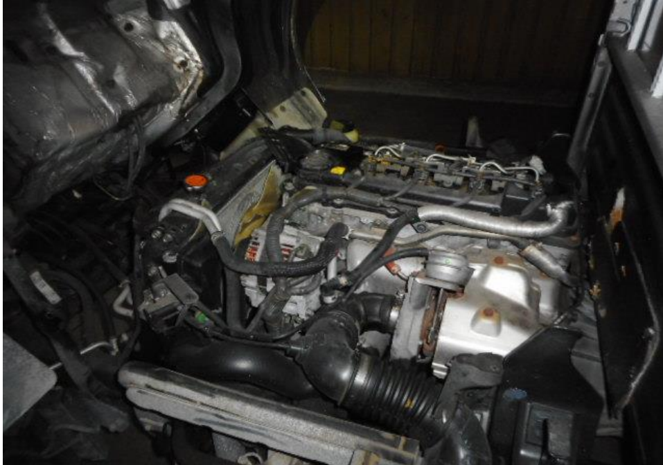
Photo 14 shows a general view of the Motor Lorry's engine compartment, which was accessed by lifting the front cabin of the Motor Lorry. The engine radiator was found to be damaged due to the result of the accident. However, the other various parts and components inside the engine compartment were unaffected by the accident. There was also no sign(s) or indication(s) of fresh fluid leakage and/or fluid stain within the engine compartment.
