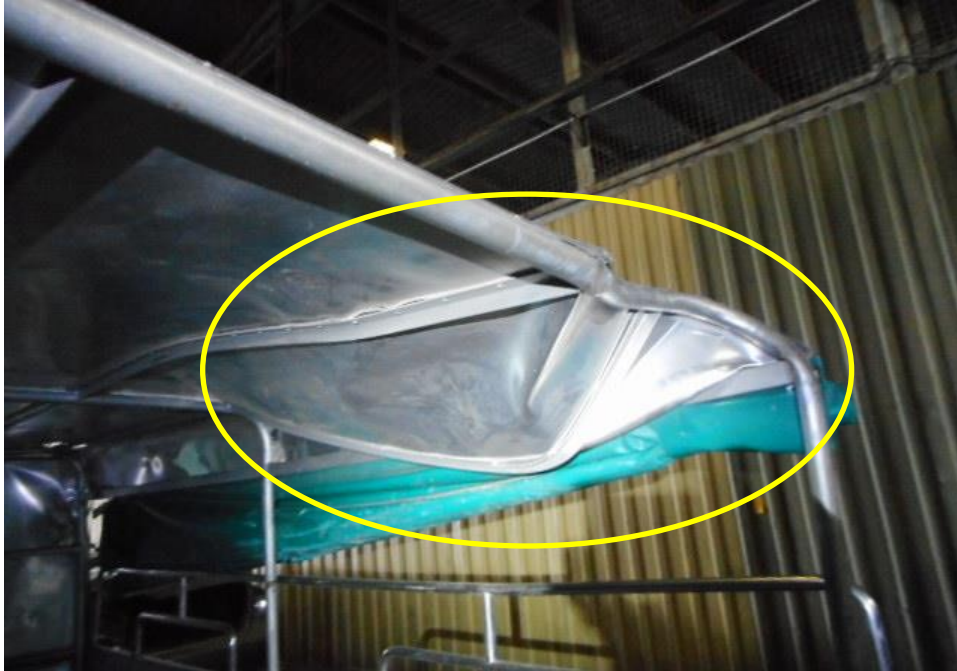
Photo 9 shows a close up view of the rear body of the Motor Lorry at the time of my inspection. Its rear body panel (circled) was damage at the time of my inspection as a result of the accident.
