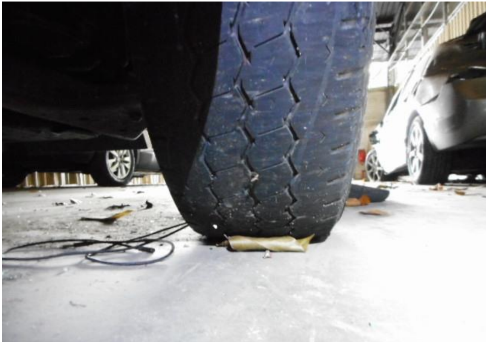
Photo 10 shows the condition of the front right tyre of the Motor Lorry, which was observed to be in serviceable condition with remaining tread depth of approximately 3mm. The tyre, which was wrapped around standard steel wheel rim, it was observed to be sufficiently inflated for vehicular operation.
