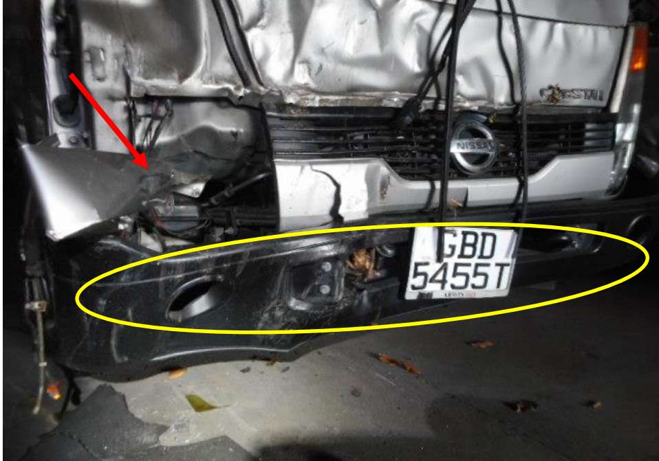
Photo 3 shows a close up view of the Motor Lorry's front portion at the time of my inspection. Its front right headlamp (arrowed) and front bumper (circled) was damage at the time of my inspection as a result of the accident.
