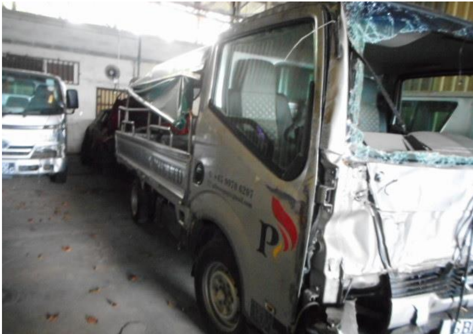
Photo 4 shows a general view of the right body of the Motor Lorry at the time of my inspection. Its right door was damage at the time of my inspection as a result of the accident.
