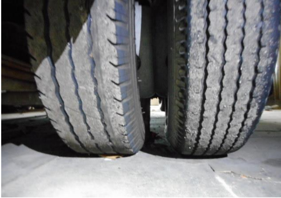
Photo 11 shows the condition of the rear right tyre of the Motor Lorry, which was observed to be in serviceable condition with remaining tread depth of approximately 2.8mm. The tyre, which was wrapped around standard steel wheel rim, it was observed to be sufficiently inflated for vehicular operation.
