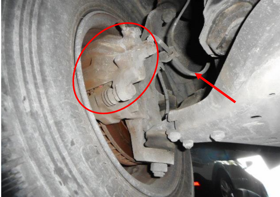
Photo 27 shows the brake hose/pipe (arrowed) at the front left wheel of the Motor Lorry. No leakage of brake fluid was observed. Visual examination of the various components of the braking system like the brake caliper (circled), brake booster, brake pedal etc had revealed all to be intact and without visible damage at the time of accident. There was also no sign of fluid stain(s) observed on the various undercarriage components.
