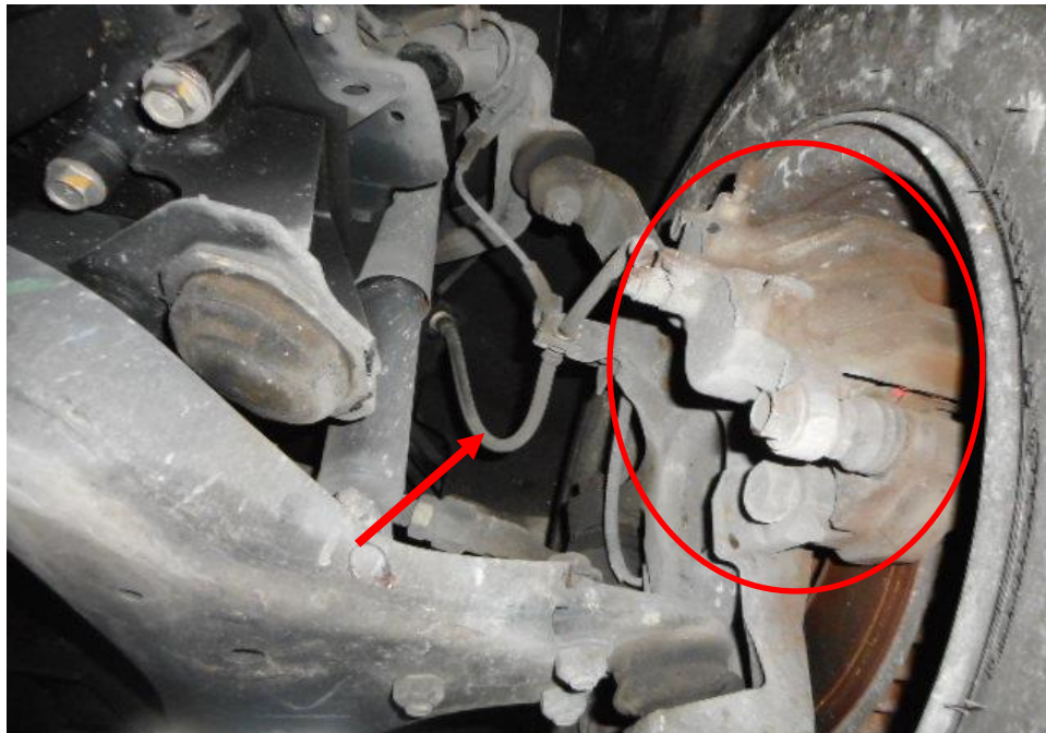
Photo 26 shows the brake hose/pipe (arrowed) at the front right wheel of the Motor Lorry. No leakage of brake fluid was observed. Visual examination of the various components of the braking system like the brake caliper (circled), brake booster, brake pedal etc had revealed all to be intact and without visible damage at the time of accident. There was also no sign of fluid stain(s) observed on the various undercarriage components.
