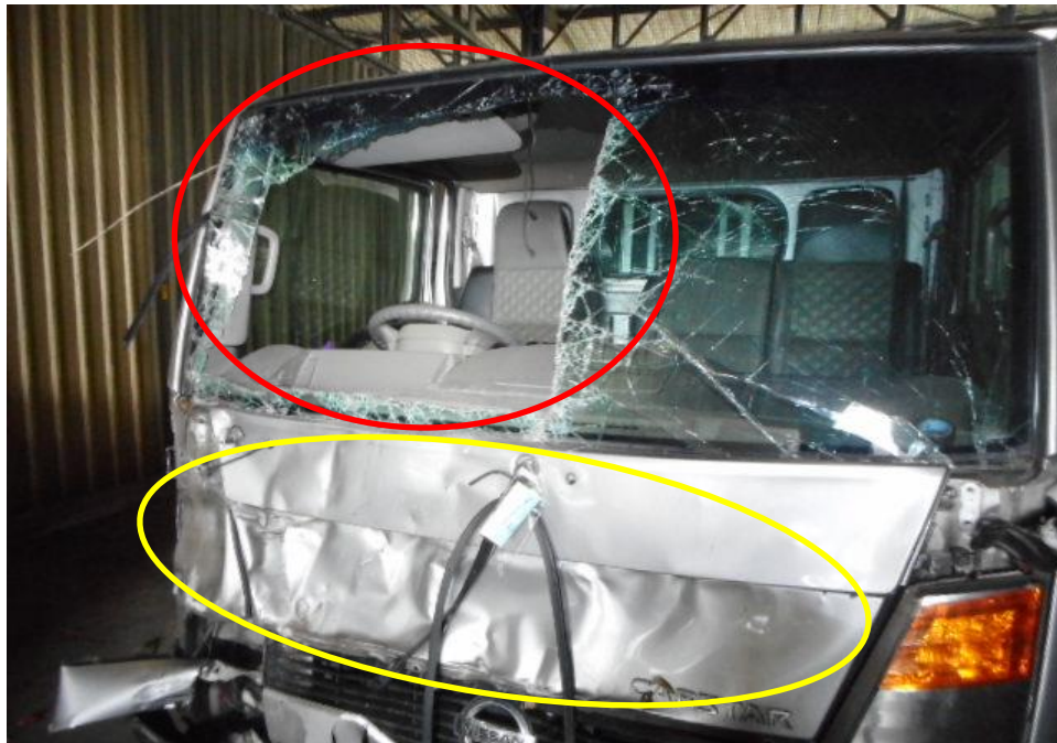
Photo 2 shows a close up view of the Motor Lorry's front portion at the time of my inspection. Its front windscreen (red circle) and front body panel (yellow circle) was damage at the time of my inspection as a result of the accident.
