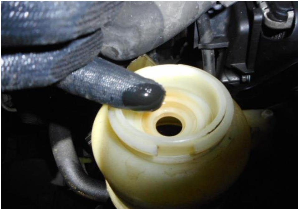
Photo 19 shows the power steering fluid reservoir of the Motor Lorry at the time of my inspection. The power steering fluid was observed to be of sufficient level (arrowed) and without any visible contamination.
