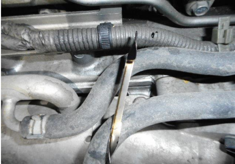
Photo 18 shows the engine oil dip stick of the Motor Lorry at the time of my inspection. The engine oil was observed to be of sufficient level and without any visible contamination.
