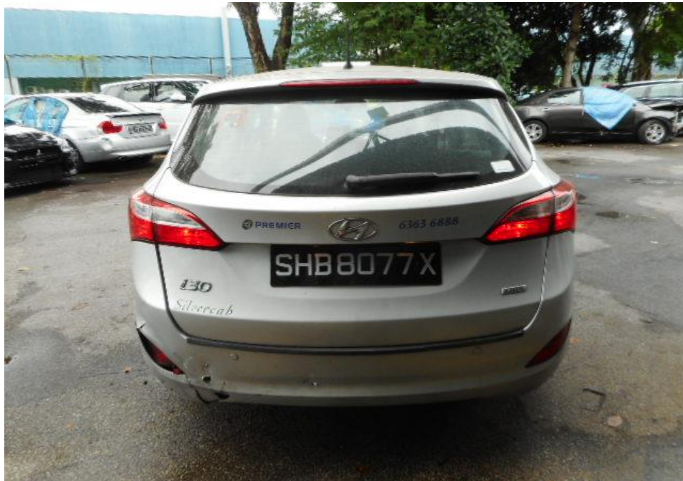
Photo 2 shows the general view of the Motor Taxi's rear body at the time of my inspection. The Motor Taxi rear portion of the Motor Taxi was observed to have sustained damage. Its rear bumper was the body part that were damaged as a result of the accident.
