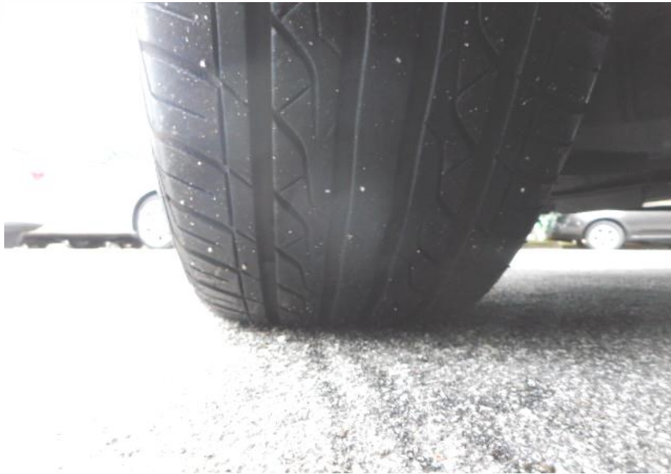
Photo 10 shows the condition of the front left tyre of the Motor Taxi, which was observed to be in serviceable condition with remaining tread depth of approximately 5.1mm. There was also no tear, cut or burst mark(s) on the outer and the inner sidewalls as well as across the tread of the Motor Taxi's 4 tyres.
