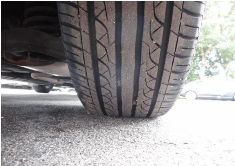
Photo 8 shows the condition of the rear right tyre of the Motor Taxi, which was observed to be in serviceable condition with remaining tread depth of approximately 5mm. The tyre was also observed to be sufficiently inflated for vehicular operation with no tear, cut or burst mark(s).
