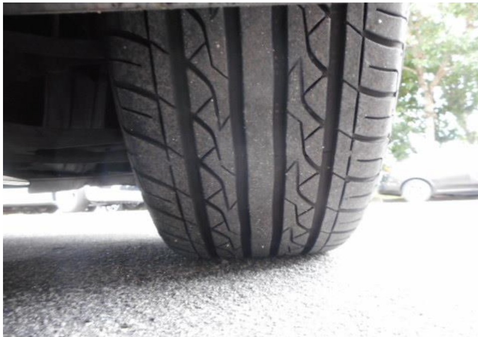
Photo 7 shows the condition of the front right tyre of the Motor Taxi, which was observed to be in serviceable condition with remaining tread depth of approximately 5.1mm. The tyre was sufficiently inflated for vehicular operation with no tear, cut or burst mark(s) on the outer and the inner sidewalls as well as across the tread. The 4 tyres of the Motor Taxi were wrapped around standard steel wheel rims without any damage.
