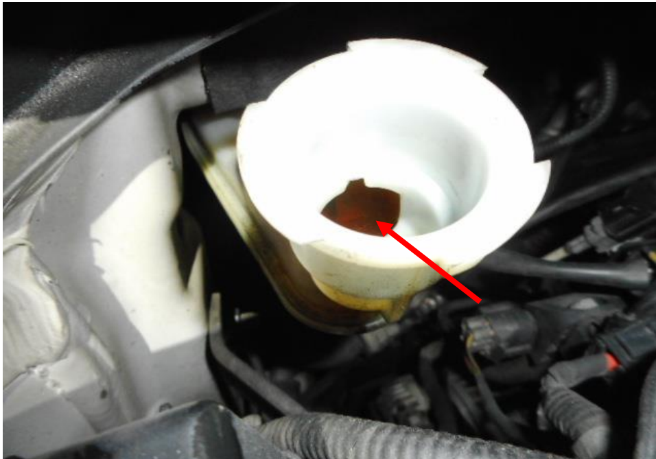
Photo 12 shows the brake fluid reservoir of the Motor Taxi at the time of my inspection. The brake fluid was observed to be of sufficient level (arrowed) and without any visible contamination.
