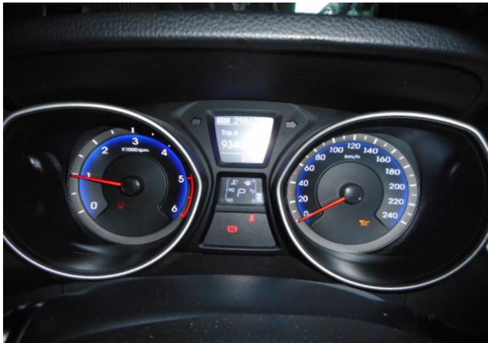
Photo 24 shows no warning lights illuminated on the instrument panel of the Motor Taxi after the engine was cranked. This would suggest that there was no abnormality to the electronic operating system of the Motor Taxi, like the ABS, EPS, SRS, and TC etc.
