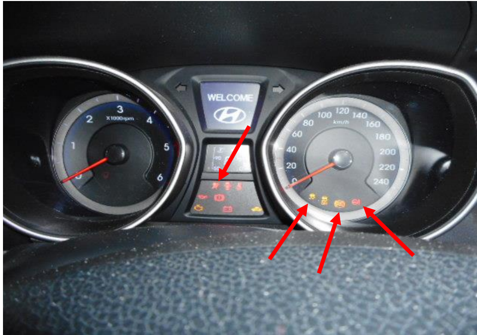
Photo 23 shows the warning light for Anti-Lock Brake System (ABS) and Power Steering System (EPS), Supplemental Restraint System (SRS) and Traction Control (TC) (arrowed) appearing on the instrument panel of the Motor Taxi during the self-test of its various electronic operating systems when its engine was cranked.
