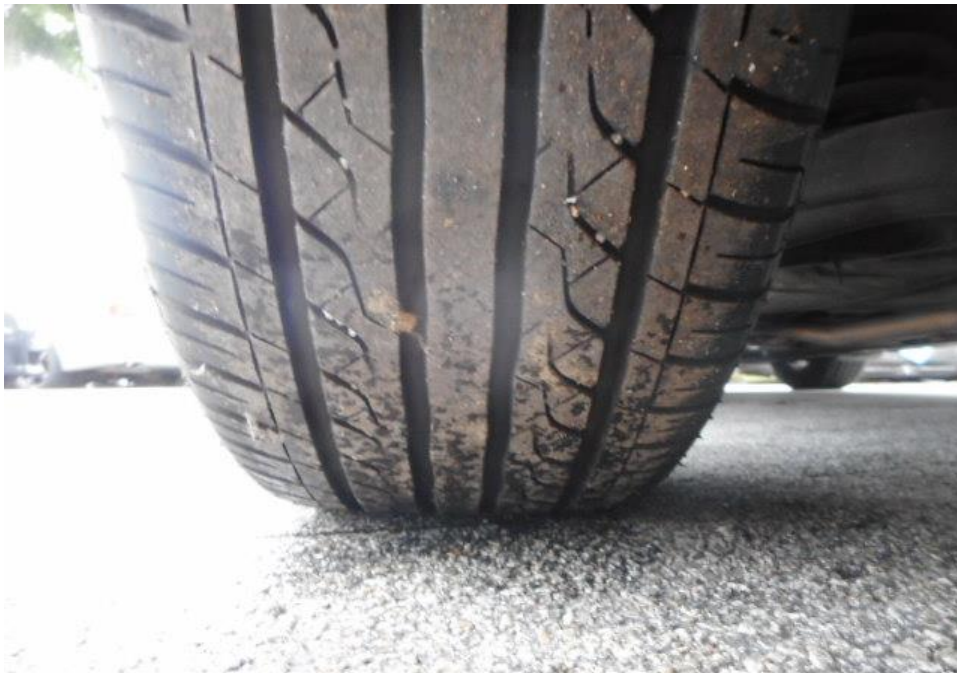
Photo 9 shows the condition of the rear left tyre of the Motor Taxi, which was observed to be in serviceable condition with remaining tread depth of approximately 4.7mm. The tyre, which was wrapped around steel wheel rim, was also observed to be sufficiently inflated for vehicular operation. The 4 tyres of the Motor Taxi were wrapped around standard steel wheel rims.
