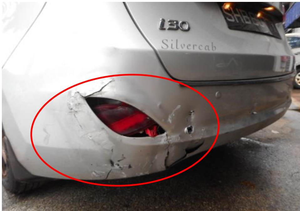
Photo 3 shows the close up view of the Motor Taxi's rear body at the time of my inspection. The Motor Taxi was observed to have sustained damage at its rear bumper (circled) (arrowed) as a result of the accident.
