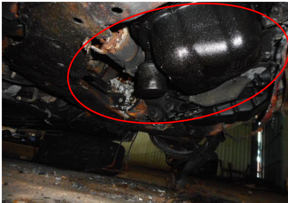
Photo 14 shows the undercarriage of the Motor Car, at the area where the engine housing and transmission housing are located. I observed sign(s) of fluid leak and fluid stain(s) on the underside of the Motor Car as a result of the accident and fire damage.
