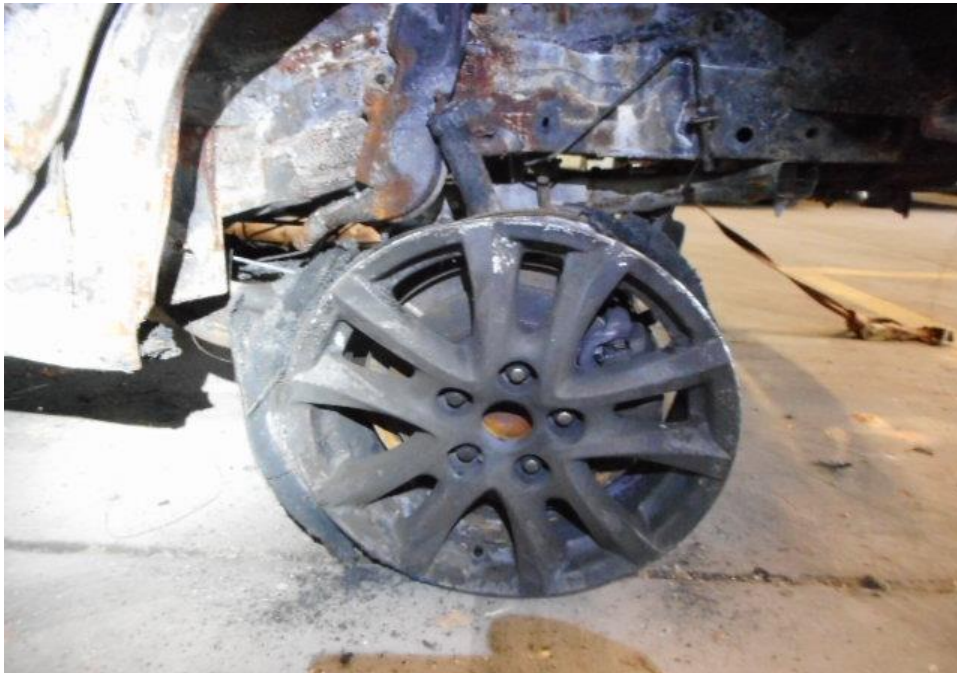
Photo 9 shows the condition of the rear left tyre and rim of the Motor Car, which was observed to be burned and damaged as a result of the accident.
