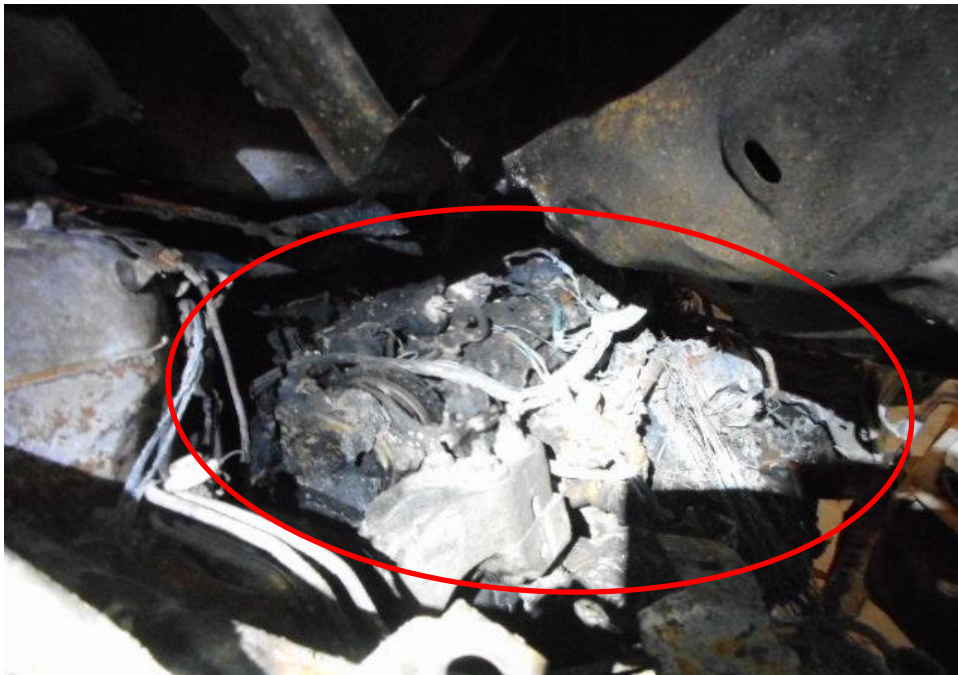
Photo 12 shows the close up view of the Motor Car's engine compartments at the time of my inspection. Its engine and various components in the engine compartments (circled) were burned and damaged as a result of the accident.
