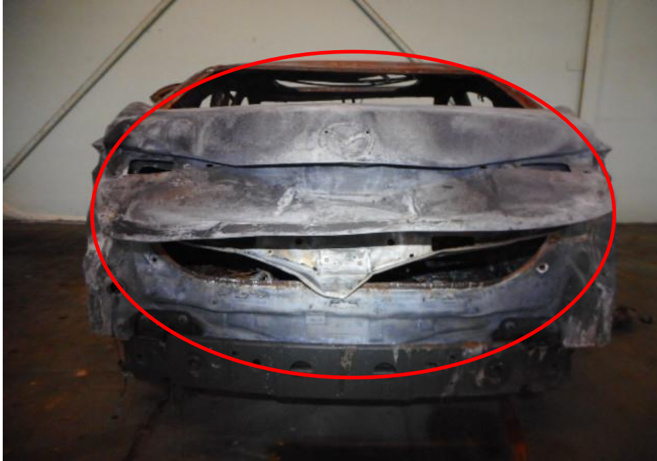
Photo 6 shows a close up view of the Motor Car's rear at the time of my inspection. The Motor Car was observed to have sustained damage at its rear portion. Its rear body panels (circled) were amongst the body parts that were burned and damaged as a result of the accident.
