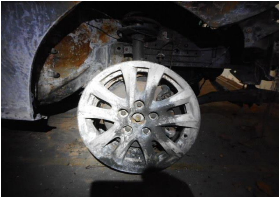
Photo 7 shows the condition of the front right tyre and rim of the Motor Car, which was observed to be burned and damaged as a result of the accident.
