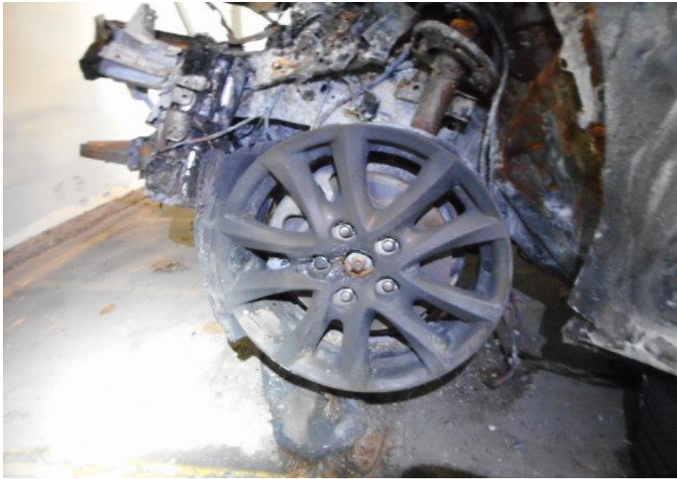
Photo 10 shows the condition of the front left tyre and rim of the Motor Car, which was observed to be burned and damaged as a result of the accident.
