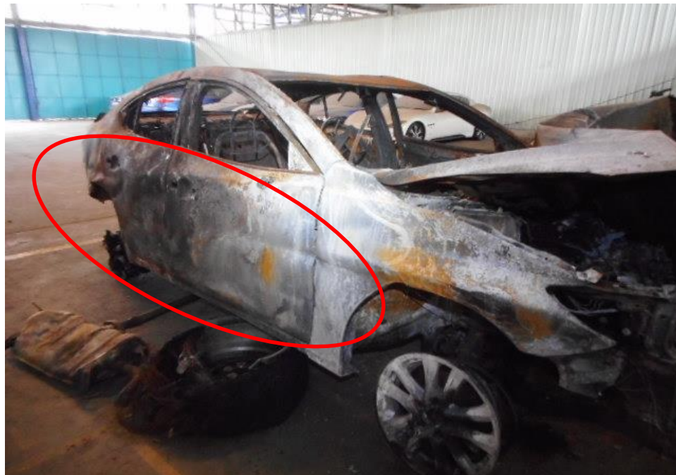
Photo 3 shows a general view of the Motor Car's right body at the time of my inspection. The Motor Car was observed to have sustained damage at its right portion. Its right body panels (circled) were amongst the body parts that were burned and damaged as a result of the accident.
