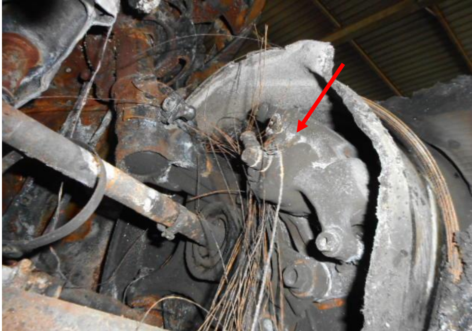
Photo 18 shows the brake caliper (arrowed) at the front left wheel of the Motor Car. The component was observed to sustain fire damage as a result of the accident.
