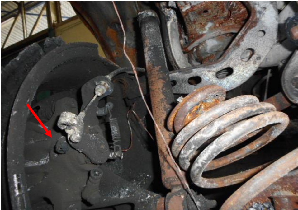
Photo 16 shows the brake caliper (arrowed) at the rear left wheel of the Motor Car. The component was observed to sustain fire damage as a result of the accident.
