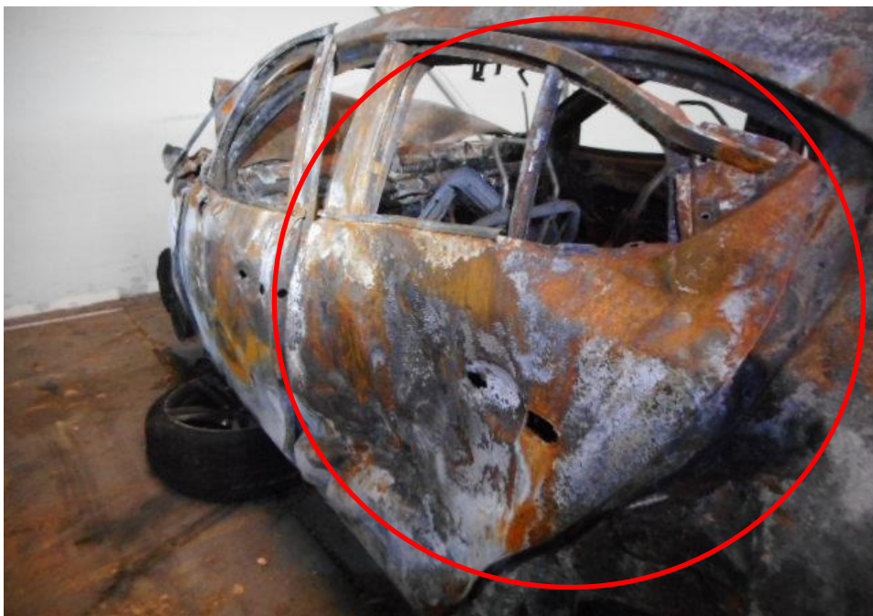
Photo 5 shows a close up view of the Motor Car's left at the time of my inspection. The Motor Car was observed to have sustained damage at its left portion. Its left body panels (circled) were amongst the body parts that were burned and damaged as a result of the accident.
