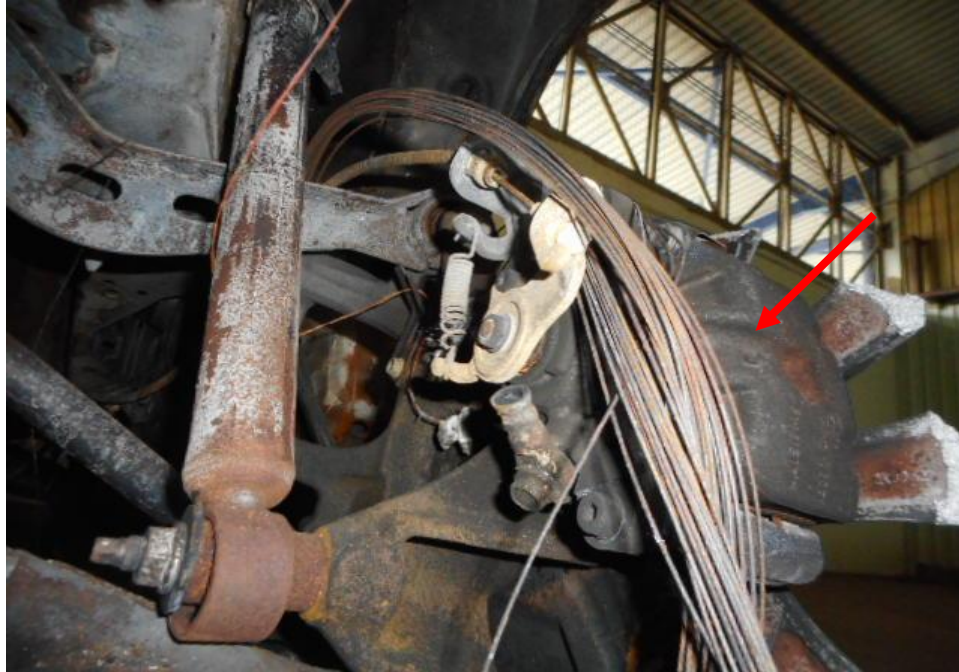
Photo 15 shows the brake caliper (arrowed) at the rear right wheel of the Motor Car. The component was observed to sustain fire damage as a result of the accident.
