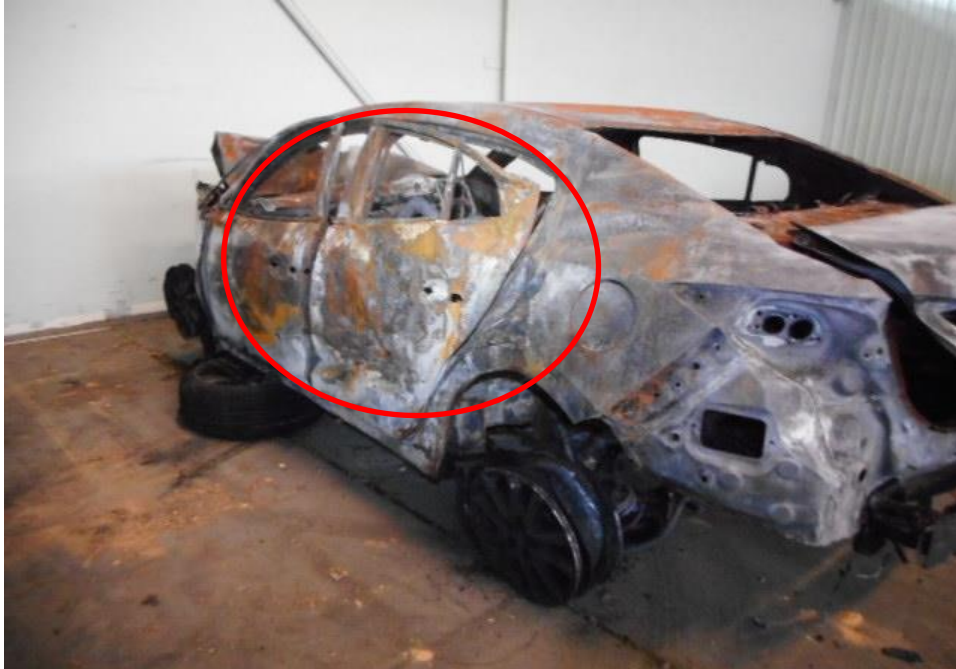
Photo 4 shows a general view of the Motor Car's left at the time of my inspection. The Motor Car was observed to have sustained damage at its right portion. Its left body panels (circled) were amongst the body parts that were burned and damaged as a result of the accident.
