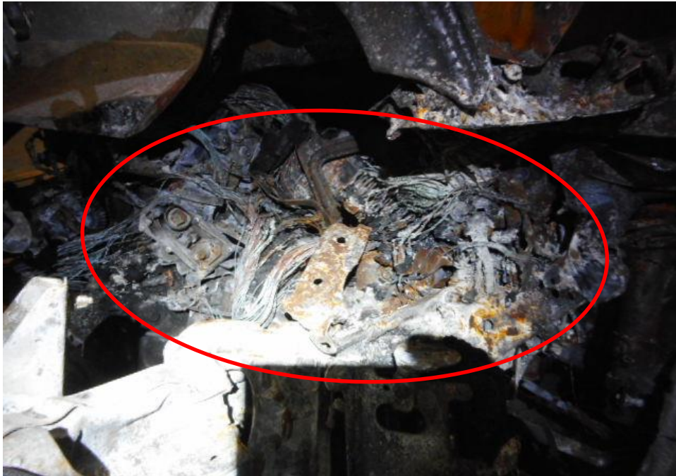
Photo 13 shows the close up view of the Motor Car's engine compartments at the time of my inspection. Its engine and various components in the engine compartments (circled) were burned and damaged as a result of the accident.
