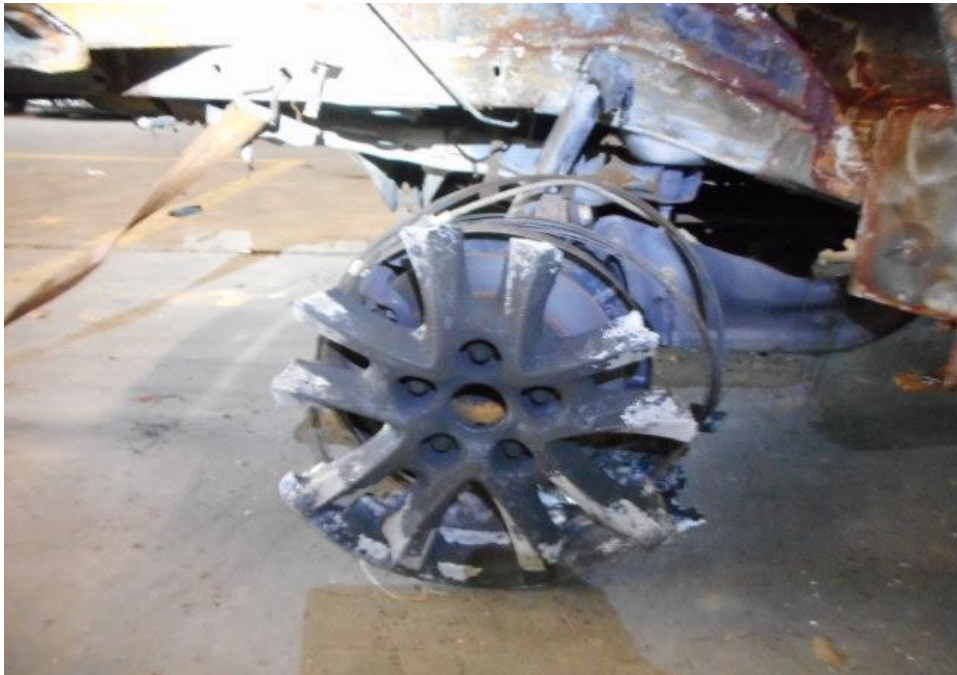
Photo 8 shows the condition of the rear right tyre and rim of the Motor Car, which was observed to be burned, damaged and broken as a result of the accident.
