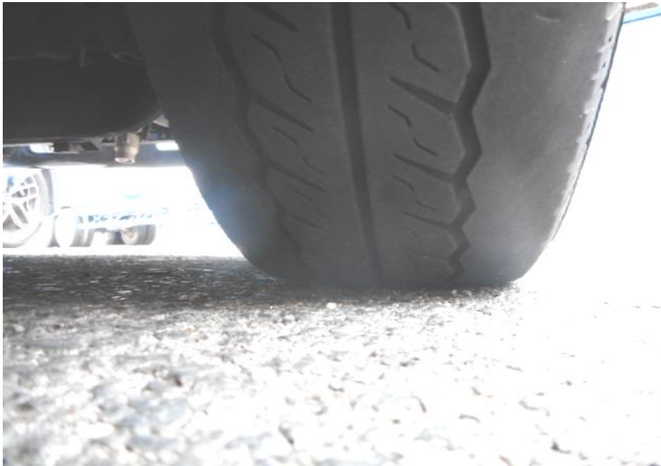
Photo 7 shows the condition of the front right tyre of the Motor Lorry, which was observed to be in serviceable condition with remaining tread depth of approximately 2.4mm. The tyre, which was wrapped around standard steel wheel rim, was also observed to be sufficiently inflated for vehicular operation. There was no tear, cut or burst mark(s) on the outer and the inner sidewalls as well as across the tread of the 6 tyres that were fitted on the Motor Lorry.
