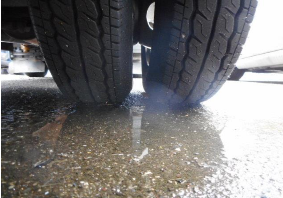
Photo 8 shows the condition of the rear right tyre of the Motor Lorry, which was observed to be in serviceable condition with remaining tread depth of approximately 5.6mm. The tyre, which was wrapped around standard steel wheel rim, it was observed to be sufficiently inflated for vehicular operation.
