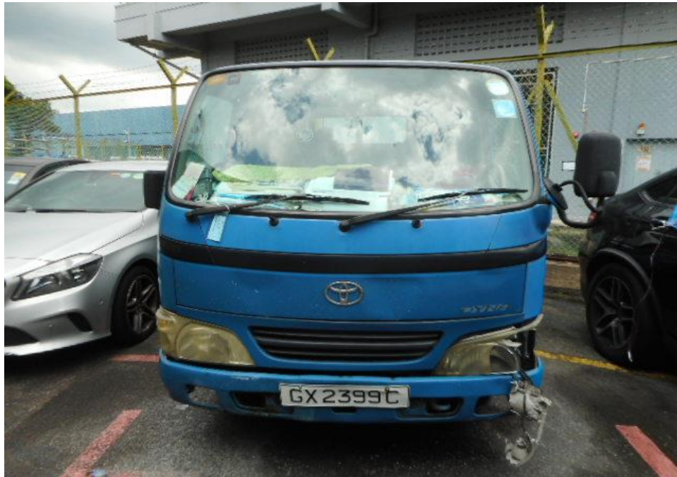
Photo 2 shows a general view of the Motor Lorry's frontal portion at the time of my inspection. It appeared to have sustained damage at its front portion. Its front body panel and front left headlamp were damaged at the time of my inspection as a result of the accident.
