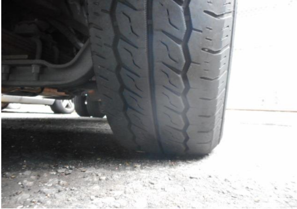
Photo 10 shows the condition of the rear right tyres of the Motor Lorry, which were observed to be in serviceable condition with remaining, tread depth of approximately 5.6mm. There was also no tear, cut or burst mark(s) on the outer and the inner sidewalls as well as across the tread of the 6 tyres that were fitted on the Motor Lorry.
