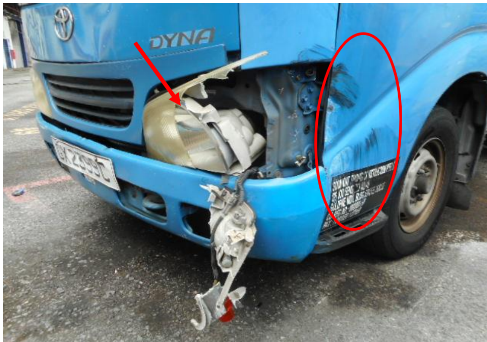
Photo 3 shows a close up view of the Motor Lorry's front portion at the time of my inspection. Its front body panel (circled) and front left headlamp (arrowed) was damaged at the time of my inspection as a result of the accident.
