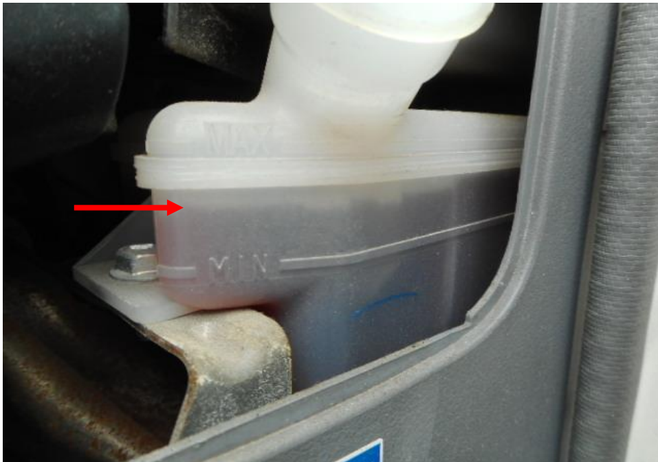
Photo 12 shows the brake fluid reservoir of the Motor Lorry at the time of my inspection. The brake fluid was observed to be of sufficient level (arrowed) and without any visible contamination.
