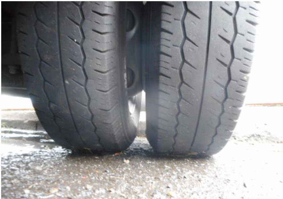
Photo 9 shows the condition of the rear left tyres of the Motor Lorry, which was observed to be in serviceable condition with remaining tread depth of approximately 2.1mm. The tyres, which were wrapped around standard steel wheel rim, were also observed to be sufficiently inflated for vehicular operation.
