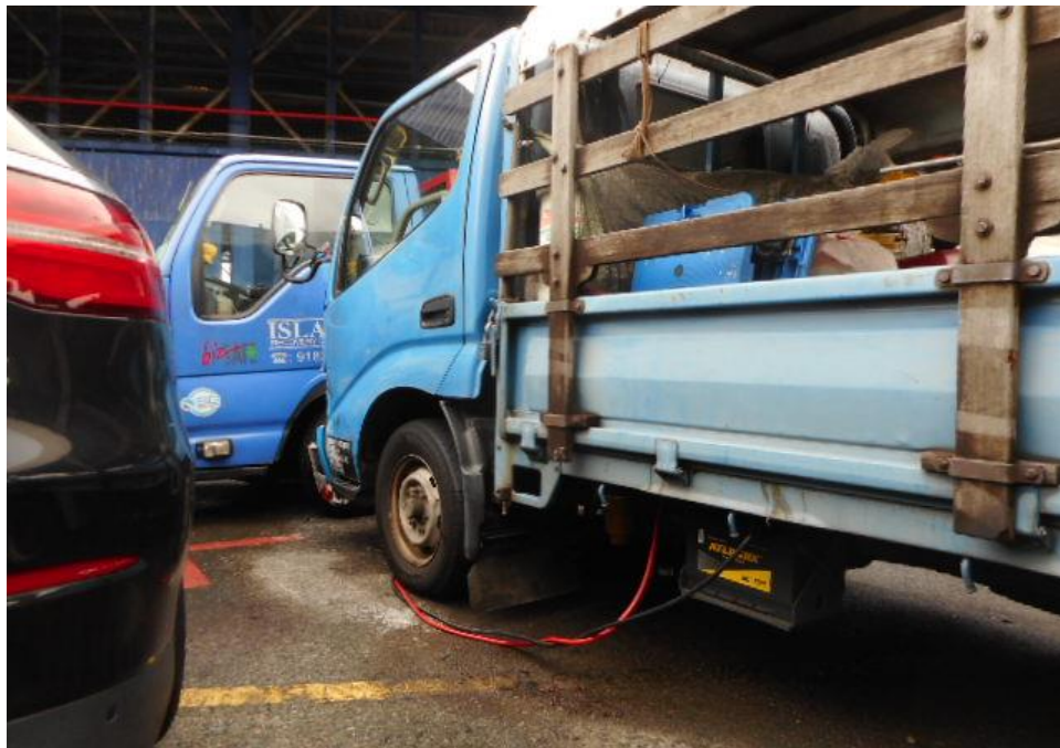
Photo 17 shows the jumpstarting process of the Motor Lorry's engine. The engine of the Motor Lorry's was unable to be jumpstarted up despite multiple attempts in starting it.
