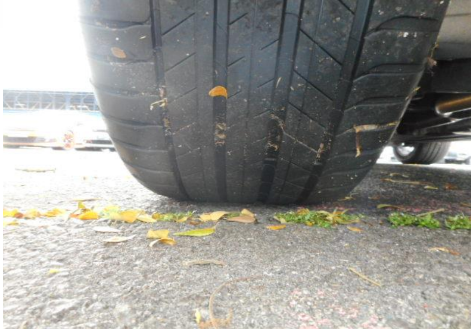
Photo 14 shows the condition of the rear left tyre of the Motor Car, which was observed to be in serviceable condition with remaining tread depth of approximately 6.2mm. The tyre, which was wrapped around steel wheel rim, was also observed to be sufficiently inflated for vehicular operation. The 4 tyres of the Motor Car were wrapped around standard steel wheel rims.
