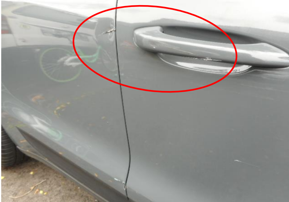
Photo 6 shows a close up view of the Motor Car's right body at the time of my inspection. The right portion of the Motor Car was observed to have sustained damage. Its right body panels (circled) was the body part that were damaged as a result of the accident.
