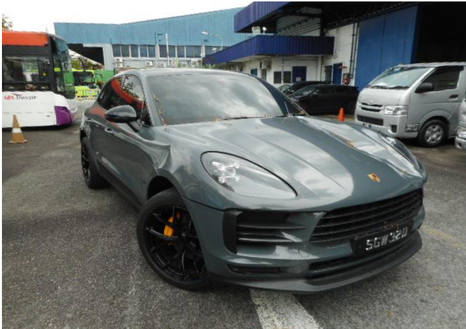
Photo 24 shows the front right wheel of the Motor Car turned to its full left. During my steering system test, I did not experience any abnormal free play and/or resistance when I had turned the steering wheel towards the left and right. This would suggest that the steering system of the Motor Car was likely to be in serviceable condition at the material time of accident.
