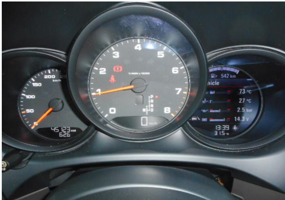
Photo 28 shows no warning lights illuminated on the instrument panel of the Motor Car after the engine was cranked. This would suggest that there was no abnormality to the electronic operating system of the Motor Car, like the ABS, EPS, TCS and SRS etc.
