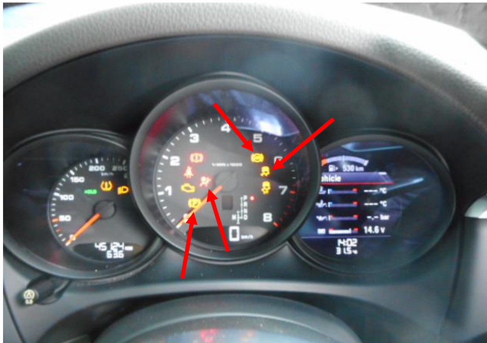
Photo 27 shows the warning light for Anti-Lock Brake System (ABS), Electric Power Steering System (EPS), Traction Control System (TCS) and Supplemental Restraint System (SRS) (arrowed) appearing on the instrument panel of the Motor Car during the self-test of its various electronic operating systems when its engine was cranked.
