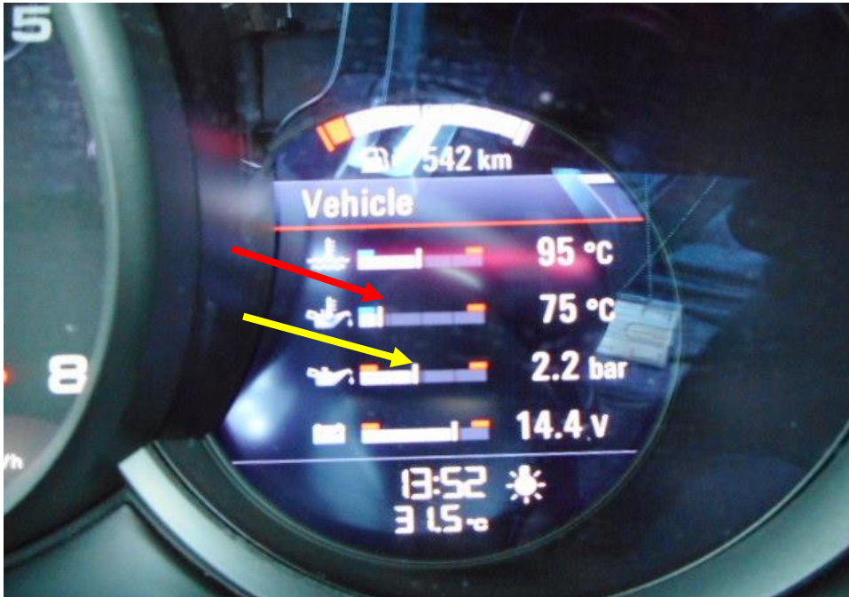
Photo 18 shows checks being carried out to the engine coolant and the engine oil on the instrument display of the Motor Car at the time of my inspection. The engine coolant (red arrow) and engine oil (yellow arrow) was observed to be of sufficient level and without any visible contamination.
