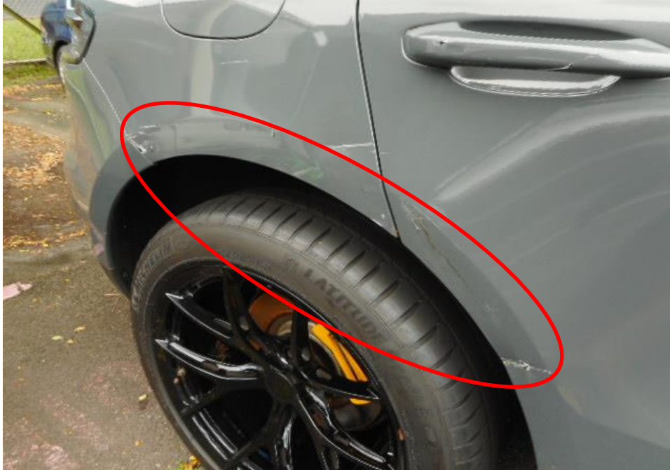
Photo 8 shows a close up view of the Motor Car's right body at the time of my inspection. The right portion of the Motor Car was observed to have sustained damage. Its right body panels (circled) was the body part that were damaged as a result of the accident.
