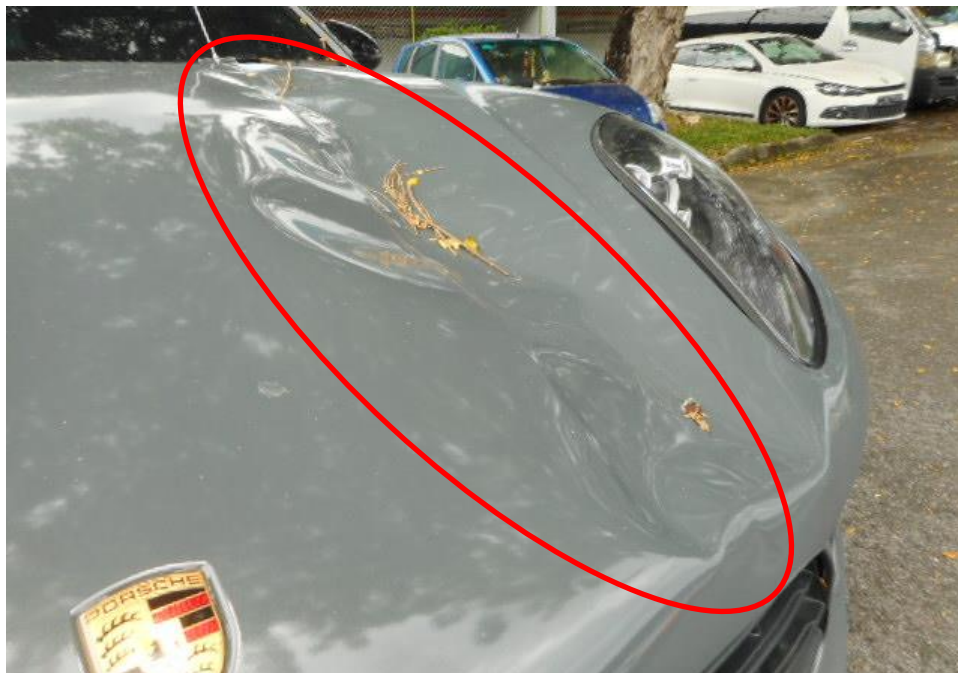
Photo 3 shows a close up view of the Motor Car's front body at the time of my inspection. The front portion of the Motor Car was observed to have sustained damage. Its front bonnet (circled) was the body part that were damaged as a result of the accident.
