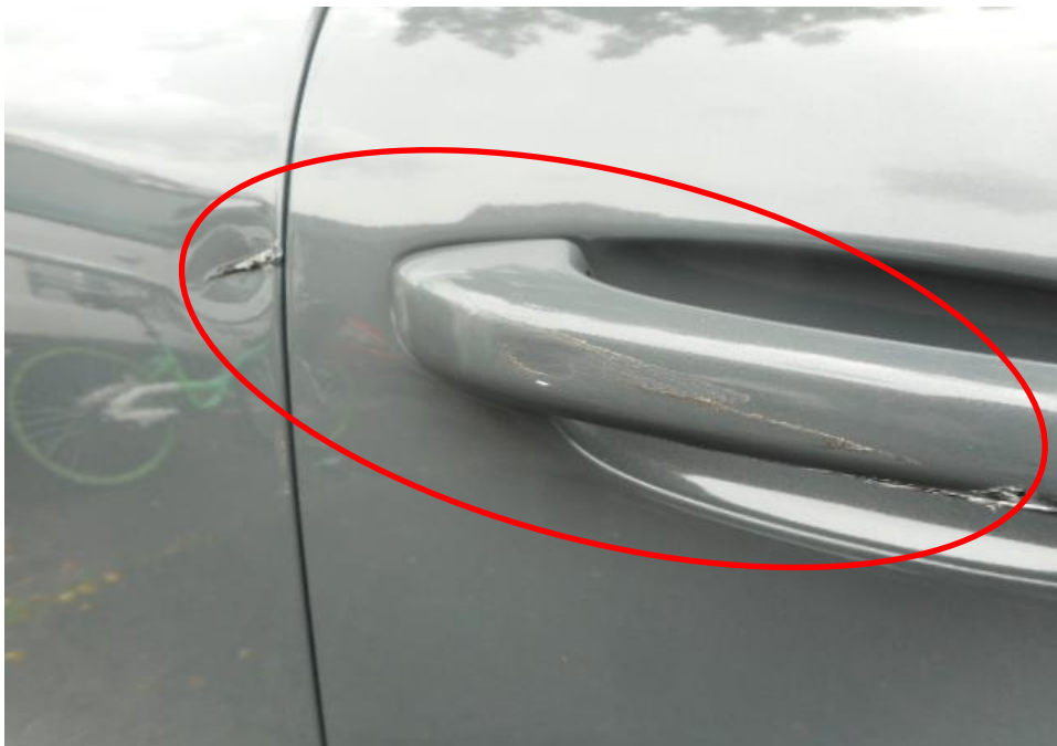
Photo 7 shows a close up view of the Motor Car's right body at the time of my inspection. The right portion of the Motor Car was observed to have sustained damage. Its right body panels (circled) was the body part that were damaged as a result of the accident.
