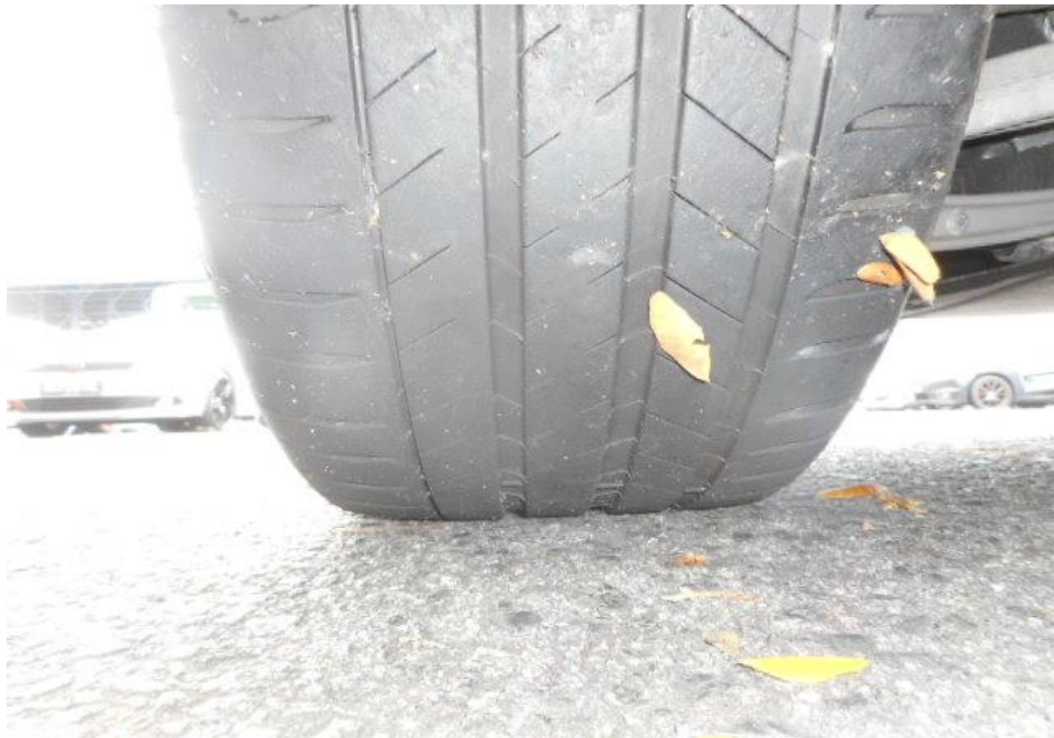
Photo 15 shows the condition of the front left tyre of the Motor Car, which was observed to be in serviceable condition with remaining tread depth of approximately 4.3mm. There was also no tear, cut or burst mark(s) on the outer and the inner sidewalls as well as across the tread of the Motor Car's 4 tyres.
