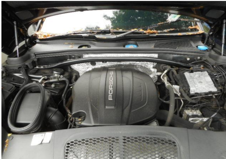
Photo 16 shows a general view of the Motor Car's engine compartment. The various parts and components inside the engine compartment were unaffected by the accident. There was also no sign(s) or indication(s) of fluid leakage and/or fluid stain within the engine compartment.
