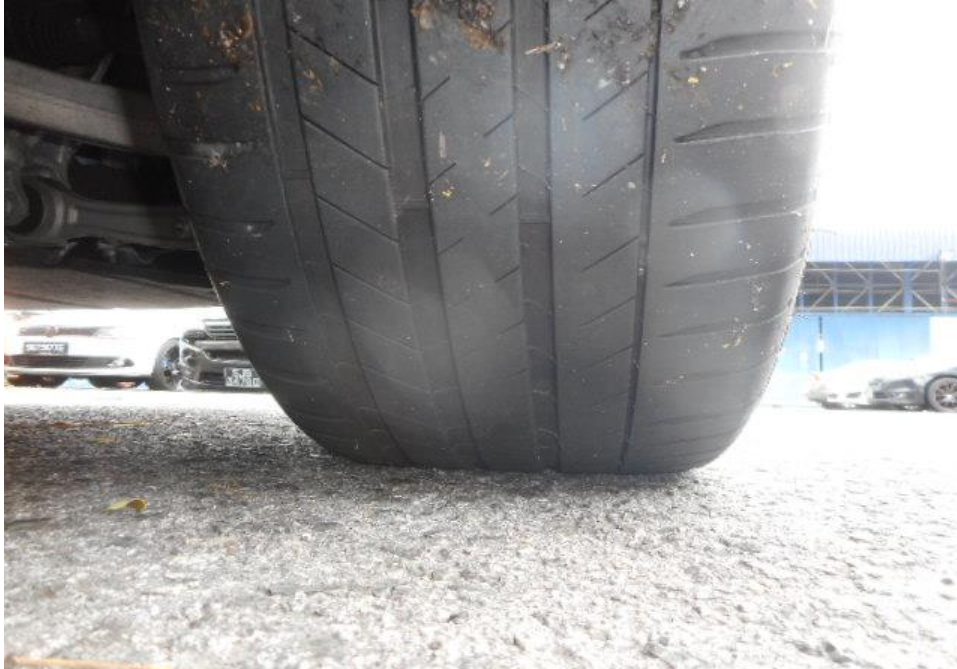
Photo 12 shows the condition of the front right tyre of the Motor Car, which was observed to be in serviceable condition with remaining tread depth of approximately 4.8mm. The tyre was sufficiently inflated for vehicular operation with no tear, cut or burst mark(s) on the outer and the inner sidewalls as well as across the tread. The 4 tyres of the Motor Car were wrapped around standard steel wheel rims without any damage.
