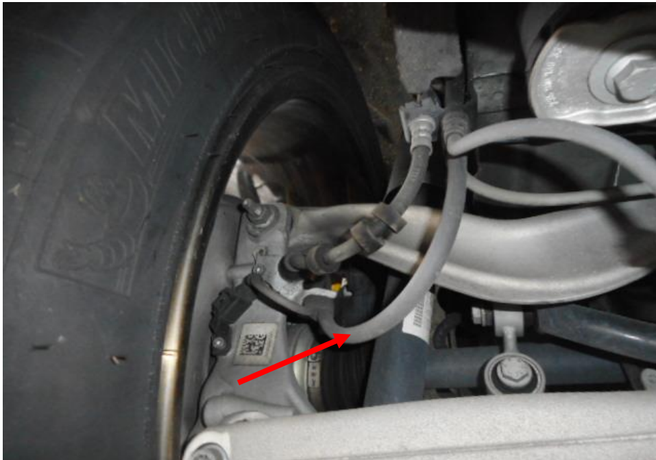
Photo 21 shows the brake hose/pipe (arrowed) at the rear left wheel of the Motor Car. I did not observe any leakage of brake fluid at the time of my inspection of the Motor Car. Static tests of the Motor Car's braking system had indicated that there was no internal leakage of pressure/vacuum. The undercarriage components of the Motor Car were also all found to be intact and without any visible damage.
