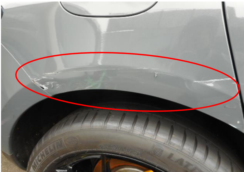
Photo 9 shows a close up view of the Motor Car's right body at the time of my inspection. The right portion of the Motor Car was observed to have sustained damage. Its right body panels (circled) was the body part that were damaged as a result of the accident.
