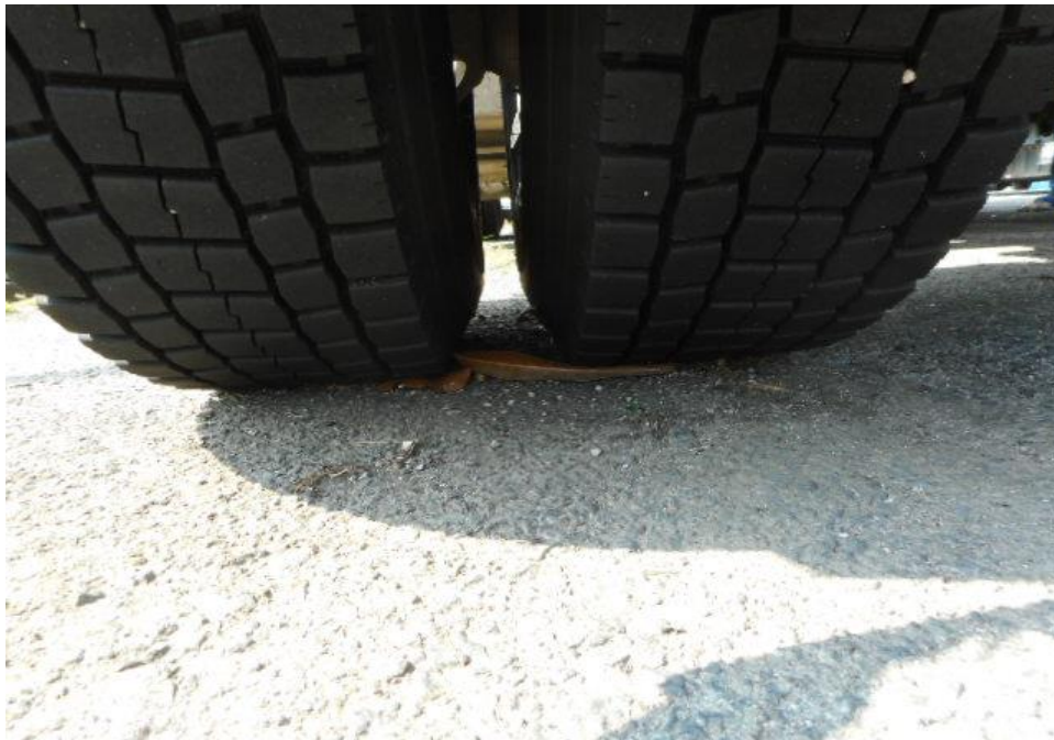
Photo 9 shows the condition of the rear left tyres of the Prime Mover, which was observed to be in serviceable condition with remaining tread depth of approximately 8.9mm. The tyres, which were wrapped around standard steel wheel rim, were also observed to be sufficiently inflated for vehicular operation. There was also no damage found on all 6 steel wheel rims of the Prime Mover.
