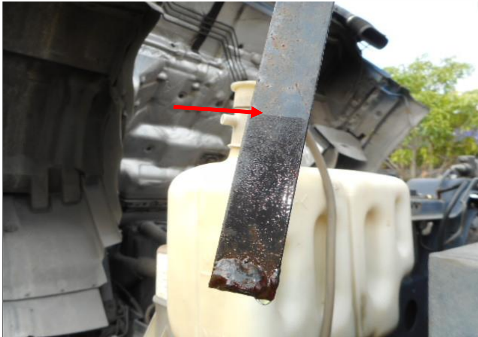
Photo 13 shows the engine coolant reservoir of the Prime Mover at the time of my inspection. The engine coolant was observed to be of sufficient level (arrowed) and without any visible contamination.
