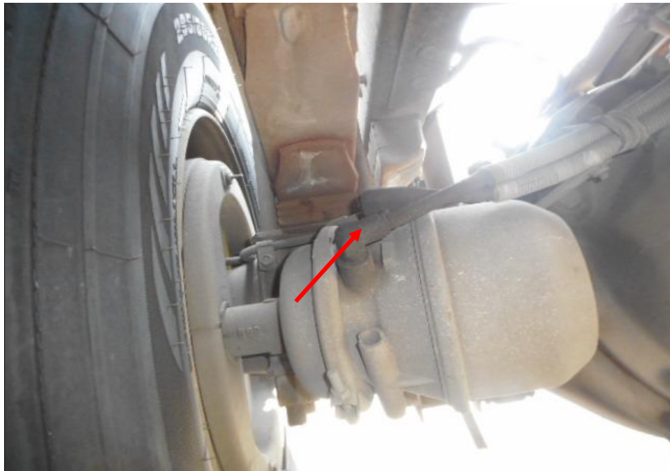
Photo 17 shows the brake pipe (arrowed) at the rear right wheel of the Prime Mover. I did not observe any leakage of brake fluid at the time of my inspection of the Prime Mover. My static tests of the Prime Mover's braking system, along with my visual examination of the various mechanical components in the braking system, had indicated that there was no internal leakage of pressure/vacuum. Hence the braking system of the Prime Mover was likely to be in serviceable condition at the material time of accident.
