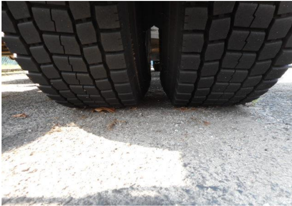
Photo 8 shows the condition of the rear right tyre of the Prime Mover, which was observed to be in serviceable condition with remaining tread depth of approximately 11mm. The tyre, which was wrapped around standard steel wheel rim, was also observed to be sufficiently inflated for vehicular operation.
