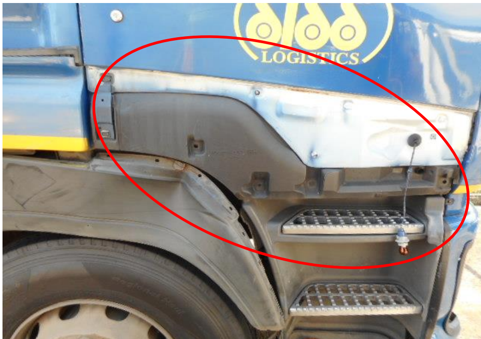
Photo 3 shows a close up view of the right body of the Prime Mover at the time of my inspection. The right portion of the Prime Mover was observed to sustained damage at the time of inspection. Its right door panel (circled) was amongst the body parts that were damaged as a result of the accident.
