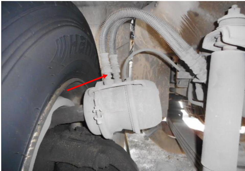
Photo 19 shows the brake pipe (arrowed) at the front right wheel of the Prime Mover. I did not observe any leakage of brake fluid at the time of my inspection of the Prime Mover. My static tests of the Prime Mover's braking system, along with my visual examination of the various mechanical components in the braking system, had indicated that there was no internal leakage of pressure/vacuum. Hence the braking system of the Prime Mover was likely to be in serviceable condition at the material time of accident.
