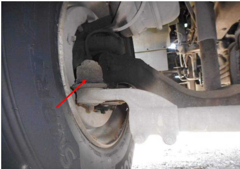
Photo 23 shows the various undercarriage components at the front left wheel of the Prime Mover, in particular the steering tie rod end (arrowed). The various undercarriage components of the Prime Mover were all found to be intact without any visible damage. There was also no sign of fluid stain(s) observed on the various undercarriage components.
