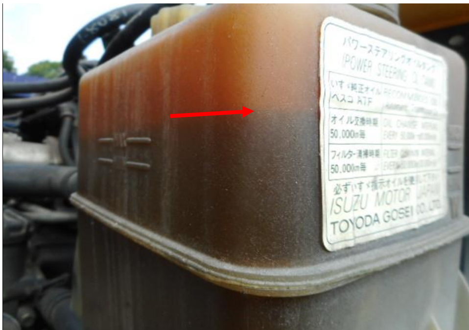
Photo 14 shows the power steering fluid reservoir of the Prime Mover at the time of my inspection. The power steering fluid was observed to be of sufficient level (arrowed) and without any visible contamination.
