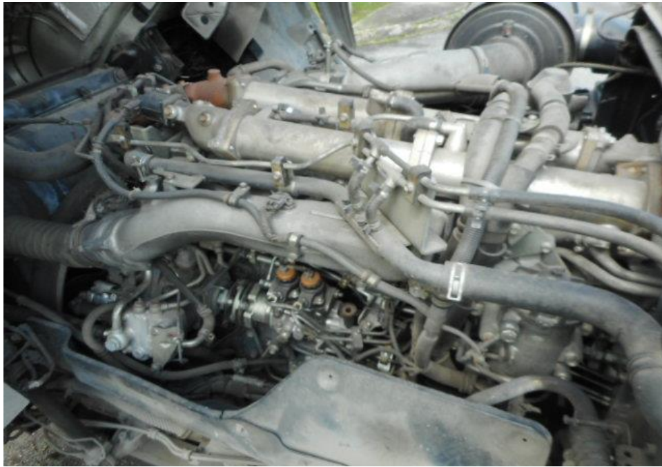
Photo 11 shows a general view of the Prime Mover's engine compartment, which was accessed by lifting the front cabin of the Prime Mover. The various parts and components inside the engine compartment were unaffected by the accident. There was also no sign(s) or indication(s) of fresh fluid leakage and/or fluid stain within the engine compartment
