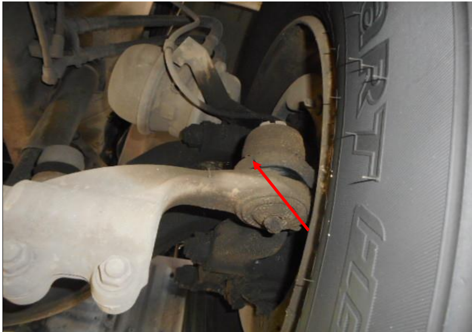
Photo 22 shows the various undercarriage components at the front right wheel of the Prime Mover, in particular the steering tie rod end (arrowed). The various steering components were all found to be intact, suggesting that the steering system of the Prime Mover was likely to be in serviceable condition at the material time of accident. There was also no sign of fluid stain(s) observed on the various undercarriage components.
