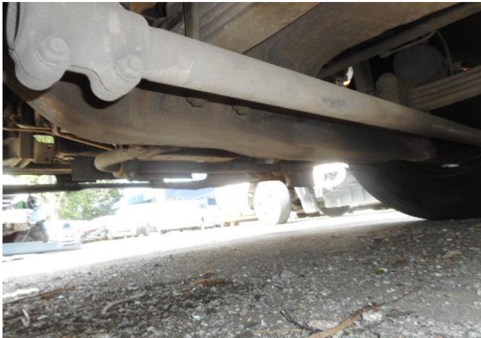
Photo 16 shows the undercarriage of the Prime Mover, at the area where the engine housing located. I did not find any sign(s) or indication(s) of fluid leak, however old fluid stain(s) was observed on the underside of the Prime Mover.
