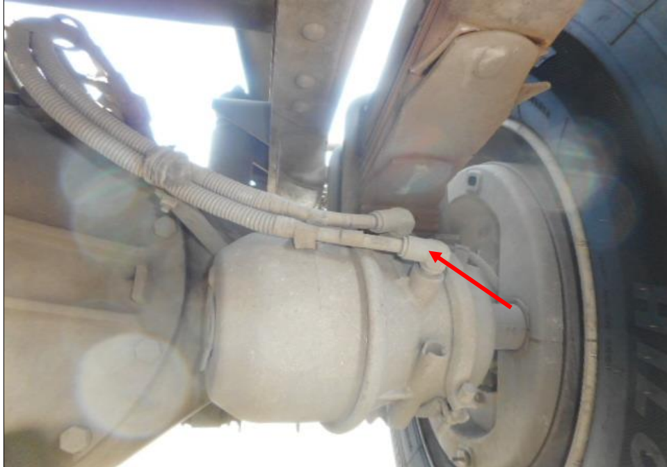
Photo 18 shows the brake pipe (arrowed) at the rear left wheel of the Prime Mover. I did not observe any leakage of brake fluid at the time of my inspection of the Prime Mover. My static tests of the Prime Mover's braking system, along with my visual examination of the various mechanical components in the braking system, had indicated that there was no internal leakage of pressure/vacuum. Hence the braking system of the Prime Mover was likely to be in serviceable condition at the material time of accident.
