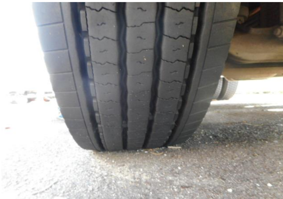
Photo 7 shows the condition of the front right tyre of the Prime Mover, which was observed to be in serviceable condition with remaining tread depth of approximately 12.4mm. The tyre, which was wrapped around standard steel wheel rim, was also observed to be sufficiently inflated for vehicular operation. There was no tear, cut or burst mark(s) on the outer and the inner sidewalls as well as across the tread of the 6 tyres that were fitted on the Prime Mover.
