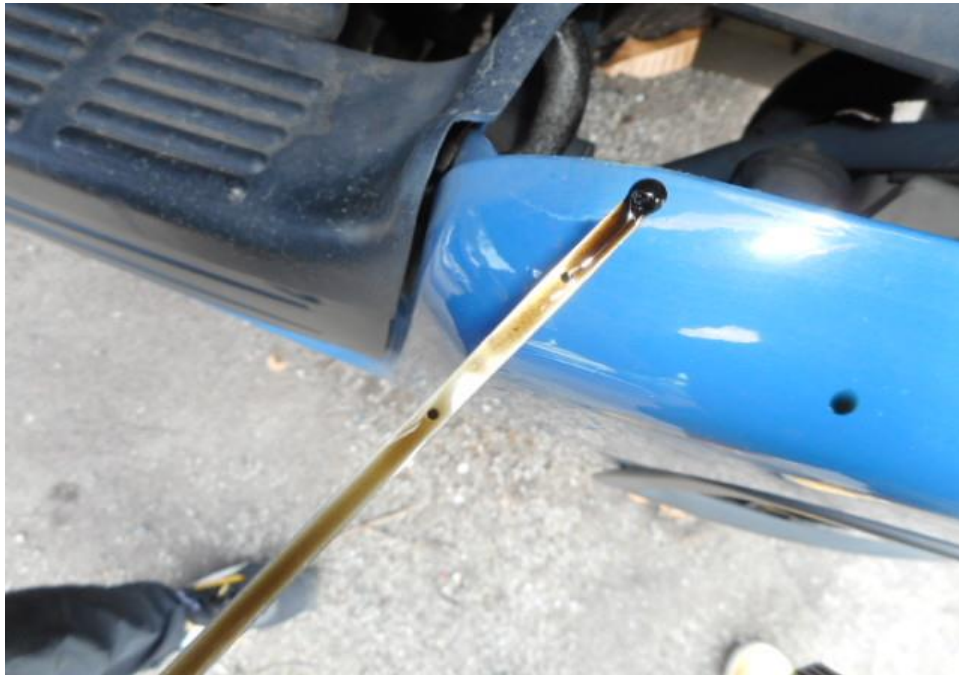
Photo 15 shows the engine oil dip stick of the Prime Mover at the time of my inspection. The engine oil was observed to be of insufficient level at the time of our inspection.
