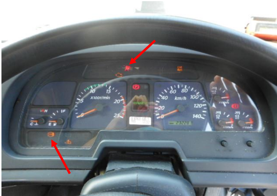
Photo 26 shows the warning light for Anti-Lock Brake System (ABS) and Supplemental Restraint System (SRS) (arrowed) appearing on the instrument panel of the Prime Mover during the self-test of its various electronic operating systems when its engine was cranked.
