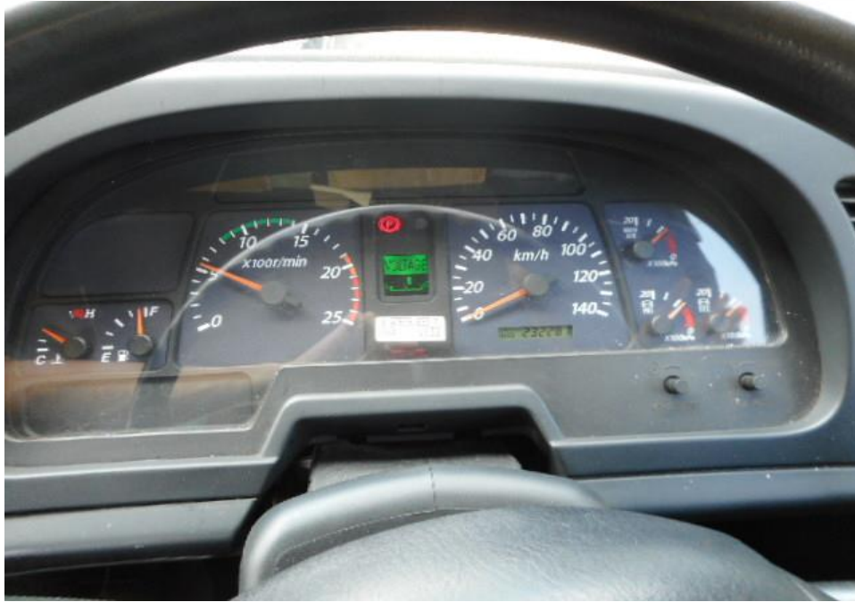
Photo 27 shows no warning lights illuminated on the instrument panel of the Prime Mover after the engine was cranked. This would suggest that there was no abnormality to the electronic operating system of the Prime Mover, like the ABS, SRS and etc.
