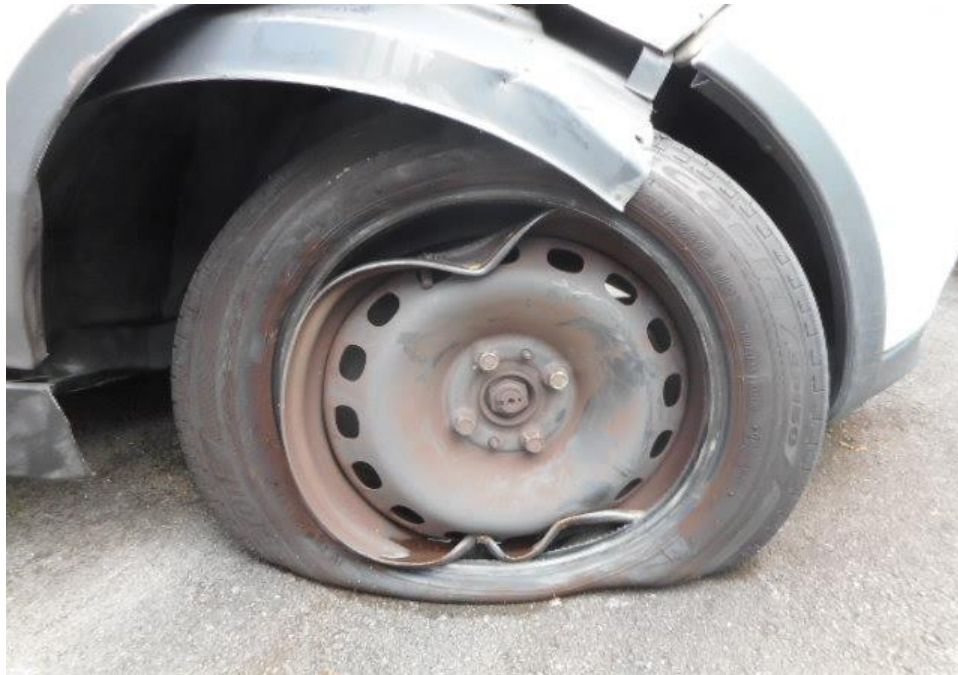
Photo 8 shows the condition of the front right tyre of the Motor Car, which was observed to be unserviceable condition with remaining tread depth of approximately 5.1mm. The tyre was observed with cut mark(s) on the outer sidewalls and there was damage observed on the wheel rims as a result of the accident.
