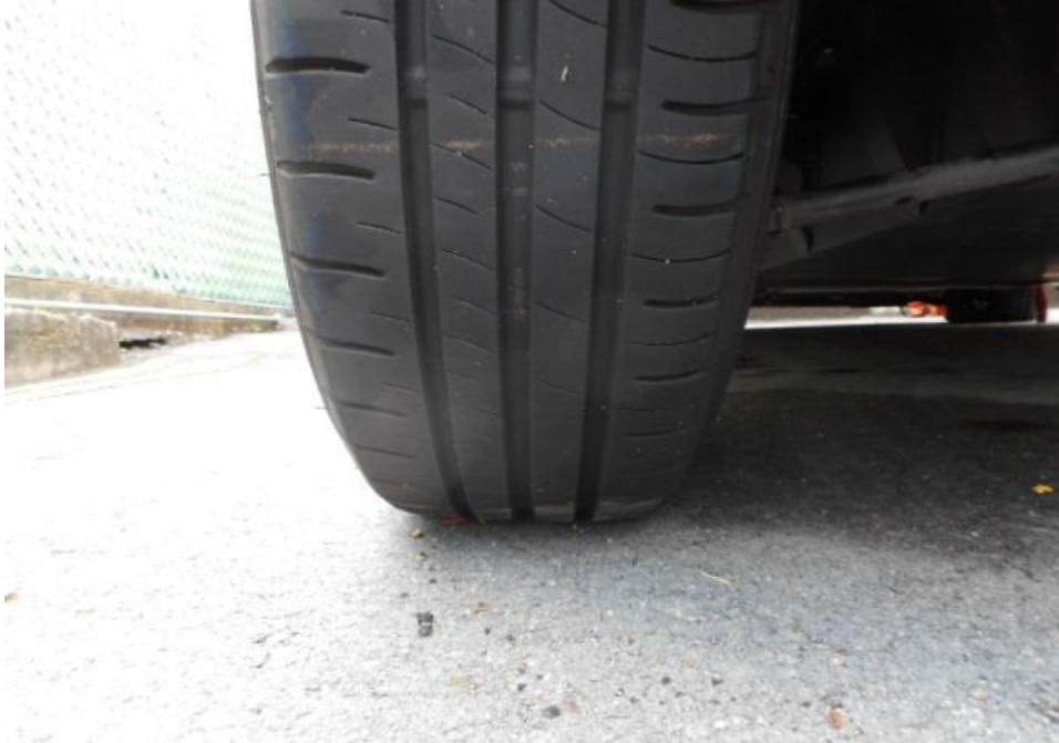
Photo 11 shows the condition of the rear left tyre of the Motor Car, which was observed to be in serviceable condition with remaining tread depth of approximately 5.5mm. The tyre was observed with cut marks and wheel rim damage as a result of the accident, however it was observed to be sufficiently inflated for vehicular operation
