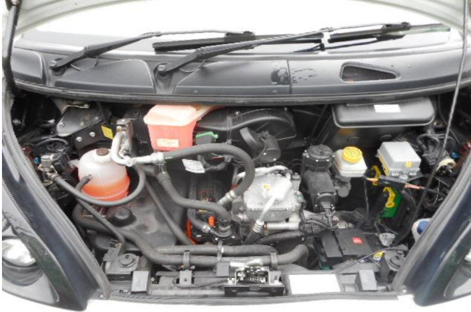
Photo 13 shows a general view of the Motor Car's engine compartment. The various parts and components inside the engine compartment were unaffected by the accident. There was also no sign(s) or indication(s) of fluid leakage and/or fluid stain within the engine compartment.
