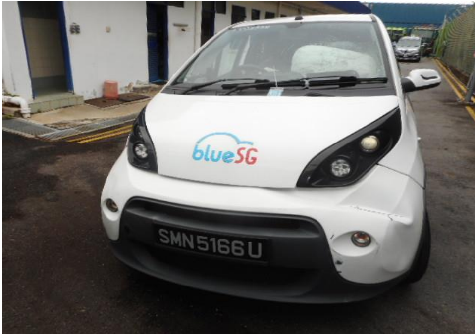
Photo 1 shows a general view of the Motor Car's front body at the time of my inspection. The Motor Car was observed to have sustained damage at its front and left portion. Its front windscreen, front bumper and front right fender were amongst the body parts that were damaged as a result of the accident.
