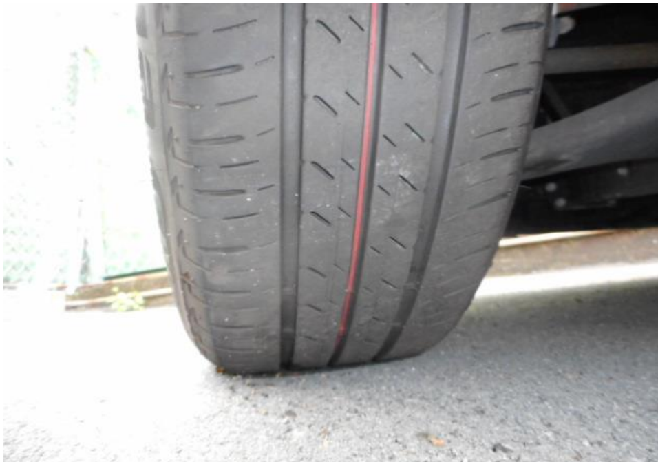
Photo 12 shows the condition of the front left tyre of the Motor Car, which was observed to be in serviceable condition with remaining tread depth of approximately 4.8mm. The tyre was observed with cut marks and wheel rim damage as a result of the accident, however it was observed to be sufficiently inflated for vehicular operation
