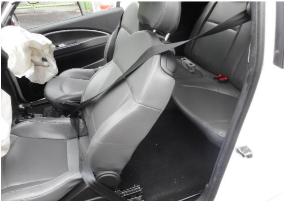
Photo 24 shows that the seat belt on the left seat tested and were able to be fastened securely into the respective pre-tensioners that were fitted at the sides of each seat.
