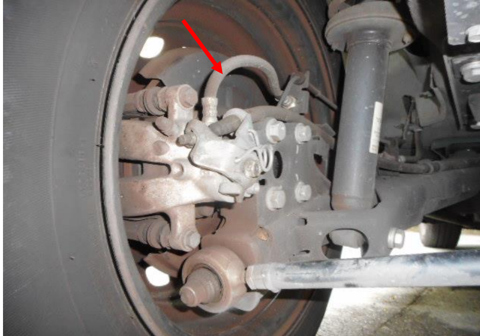
Photo 18 shows the brake hose/pipe (arrowed) at the rear left wheel of the Motor Car. I did not observe any leakage of brake fluid at the time of my inspection of the Motor Car. The undercarriage components of the Motor Car were also all found to be intact and without any visible damage.
