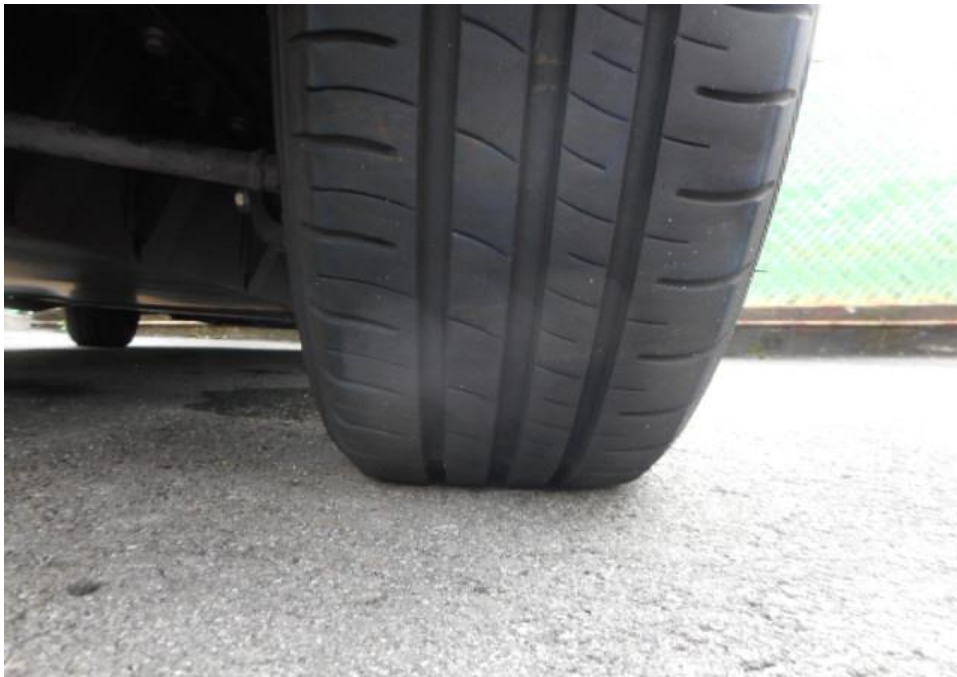
Photo 10 shows the condition of the rear right tyre of the Motor Car, which was observed to be in serviceable condition with remaining tread depth of approximately 5.8mm. The tyre was observed with cut marks and wheel rim damage as a result of the accident, however it was observed to be sufficiently inflated for vehicular operation
