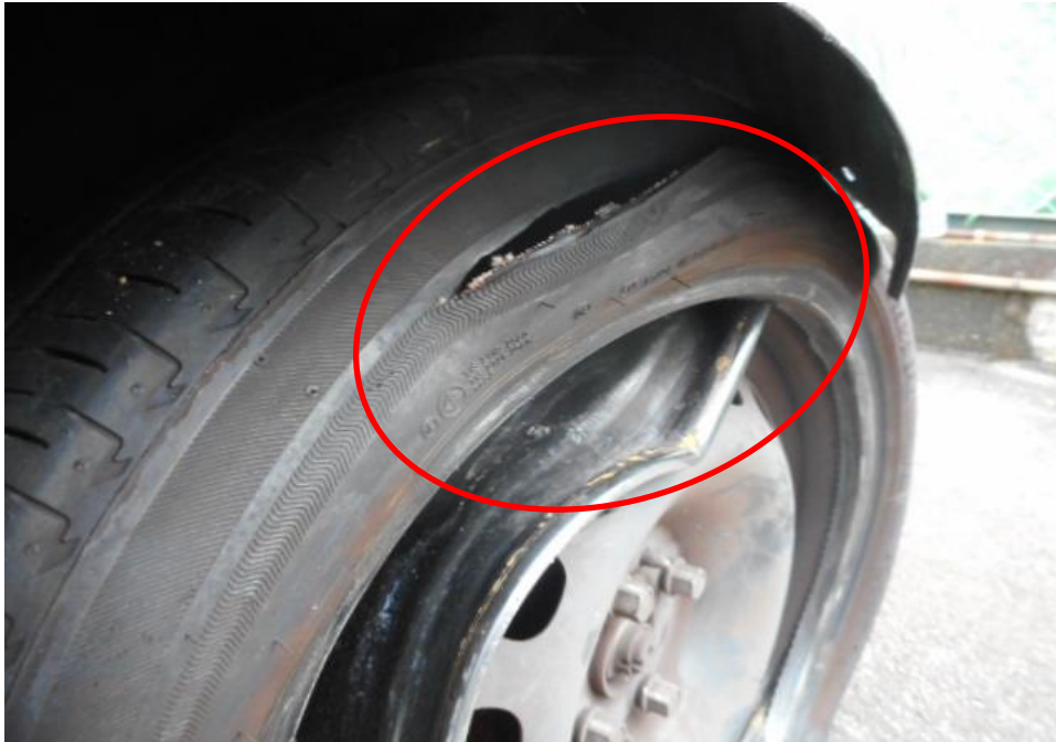
Photo 9 shows the close up view of the condition of the front right tyre of the Motor Car, which was observed to be unserviceable condition. The tyre was observed with cut mark(s) on the outer sidewalls and there was damage observed on the wheel rims (circled) as a result of the accident.
