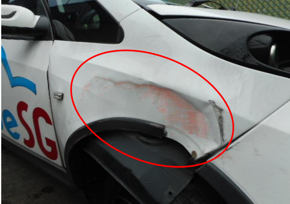
Photo 5 shows a general view of the Motor Car's front body at the time of my inspection. The Motor Car was observed to have sustained damage at its front portion. Its front right fender (circled) were amongst the body parts that were damaged as a result of the accident.
