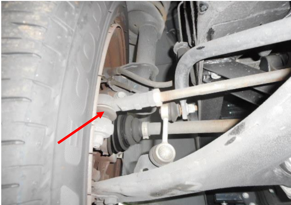
Photo 22 shows the various undercarriage components at the front left wheel of the Motor Car, in particular the steering tie rod (red arrow). The various steering components were all found to be intact. There was also no sign of fluid stain observed on the various undercarriage components at the front right wheel of the Motor Car.
