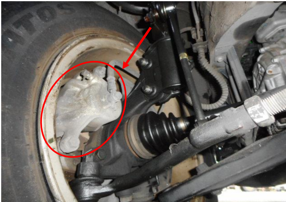
Photo 24 shows the brake hose/pipe (arrowed) at the front left wheel of the Motor Car. No leakage of brake fluid was observed. Visual examination of the various components of the braking system like the brake caliper (circled) revealed to be intact and without visible damage.
