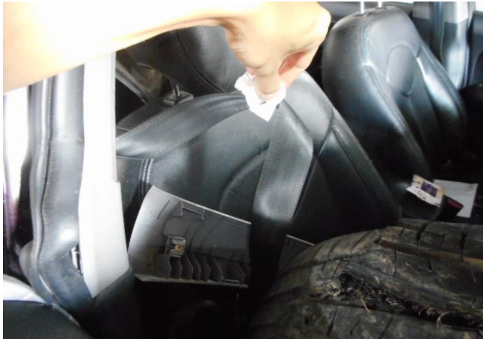
Photo 27 shows that the seat belt on the front right seat was worn at the material time of accident as the safety pre-tensioners were activated at the moment of impact and caused the seat belt to be locked into the last position.
