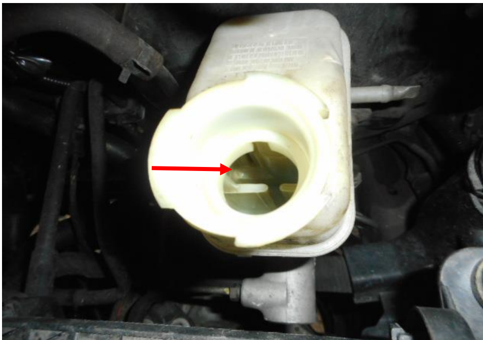
Photo 17 shows the brake fluid reservoir of the Motor Car at the time of my inspection. The brake fluid was observed to be of insufficient level (arrowed) as a result of the missing braking system of the front right braking system due to the result of the accident.
