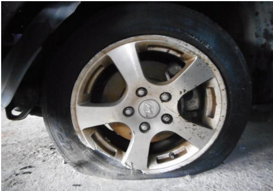
Photo 14 shows the condition of the front right tyre of the Motor Car, which was observed to be in serviceable condition with remaining tread depth of approximately 4.9mm. The tyre was observed with cut marks and wheel rim damage as a result of the accident, however it was observed to be sufficiently inflated for vehicular operation
