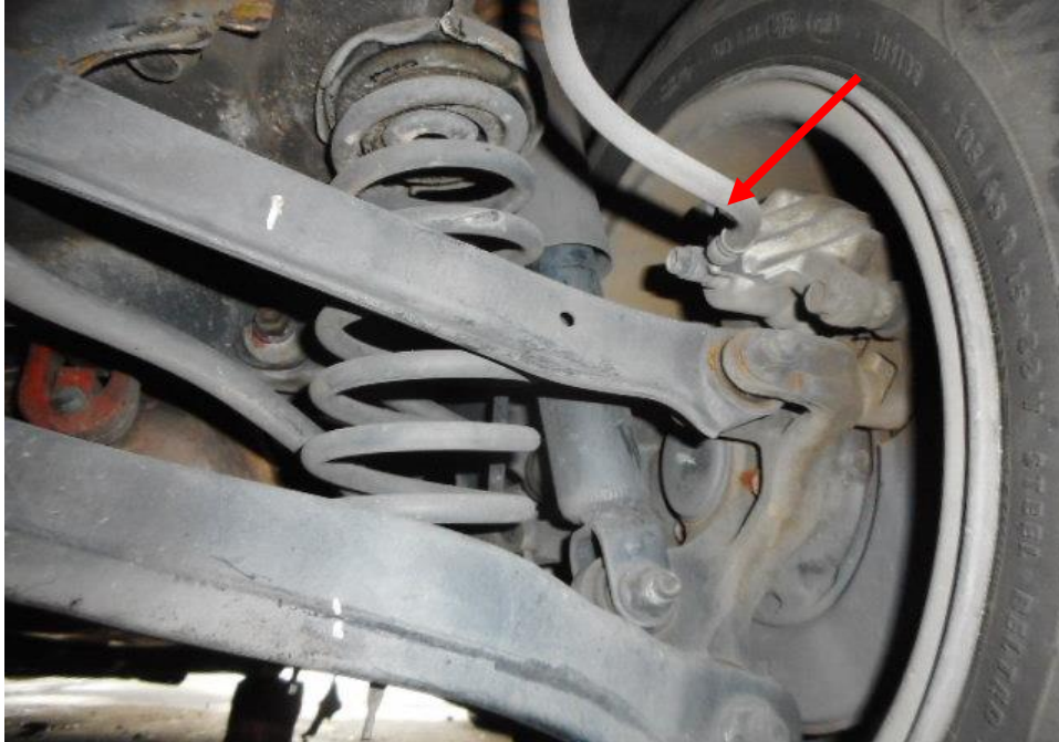
Photo 21 shows the brake hose/pipe (arrowed) at the rear right wheel of the Motor Car. No leakage of brake fluid was observed. Visual examination of the various components revealed to be intact and without visible damage.
