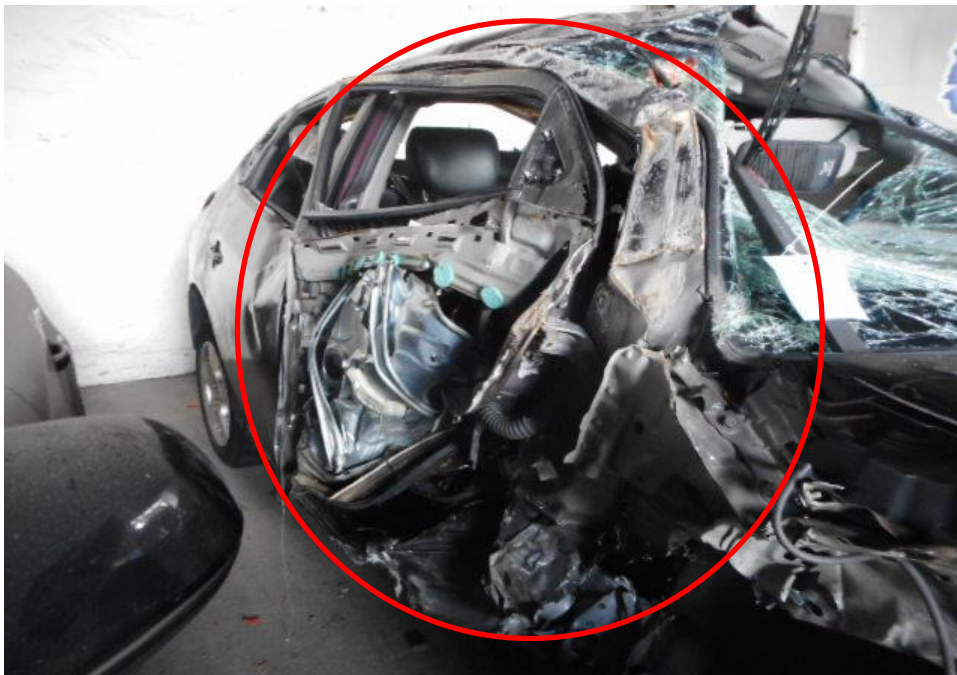
Photo 8 shows a close up view of the Motor Car's right body at the time of my inspection. The Motor Car was observed to have sustained damage at its right portion. Its right body panels (circled) were amongst the body parts that were damaged as a result of the accident.
