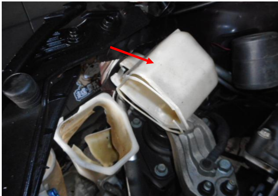
Photo 19 shows checks being carried out to the engine coolant of the Motor Car at the time of my inspection. The coolant was observed to be of insufficient level as a result of the damaged coolant reservoir (arrowed) as the result of the accident.
