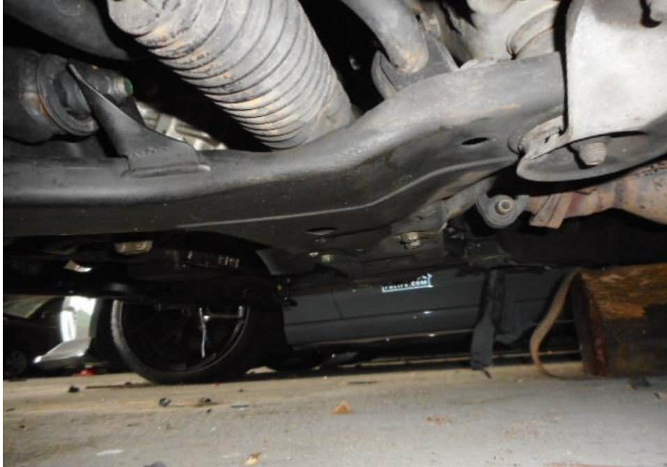
Photo 20 shows the undercarriage of the Motor Car, at the area where the engine housing and transmission housing are located. I did not find any sign(s) or indication(s) of fluid leak and/or fluid stain(s) on the underside of the Motor Car.
