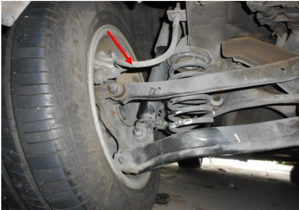
Photo 22 shows the brake hose/pipe (arrowed) at the rear left wheel of the Motor Car. No leakage of brake fluid was observed. Visual examination of the various components revealed to be intact and without visible damage.
