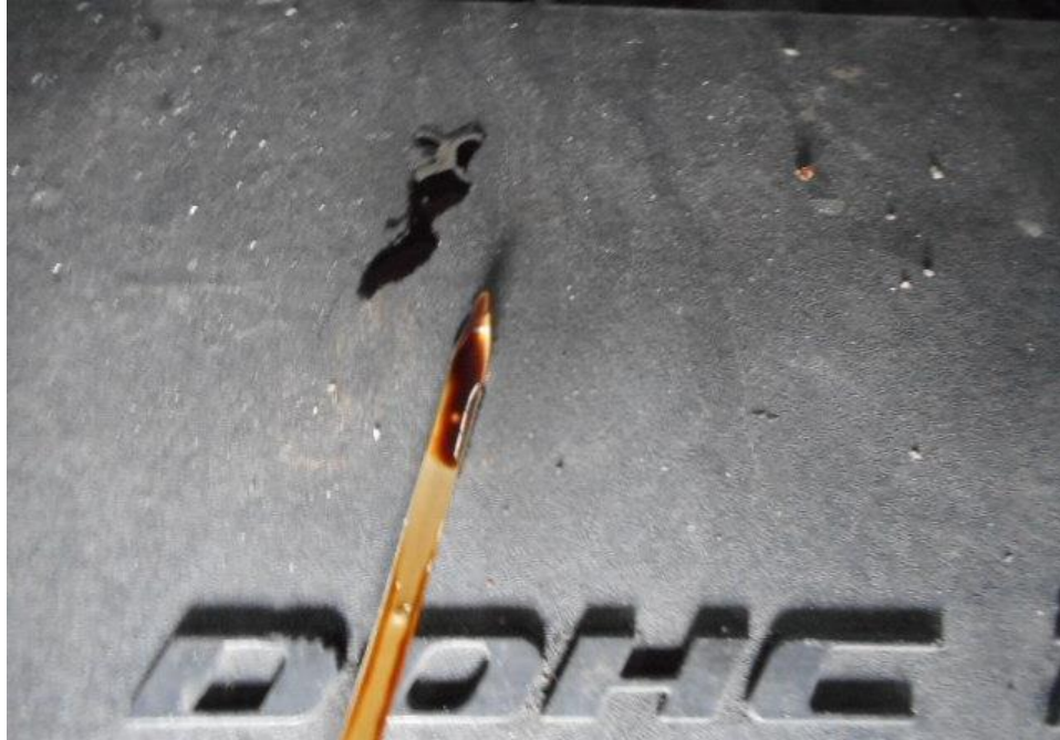
Photo 18 shows the engine oil dip stick of the Motor Car at the time of my inspection. The engine oil was observed to be of sufficient level and without any visible contamination.
