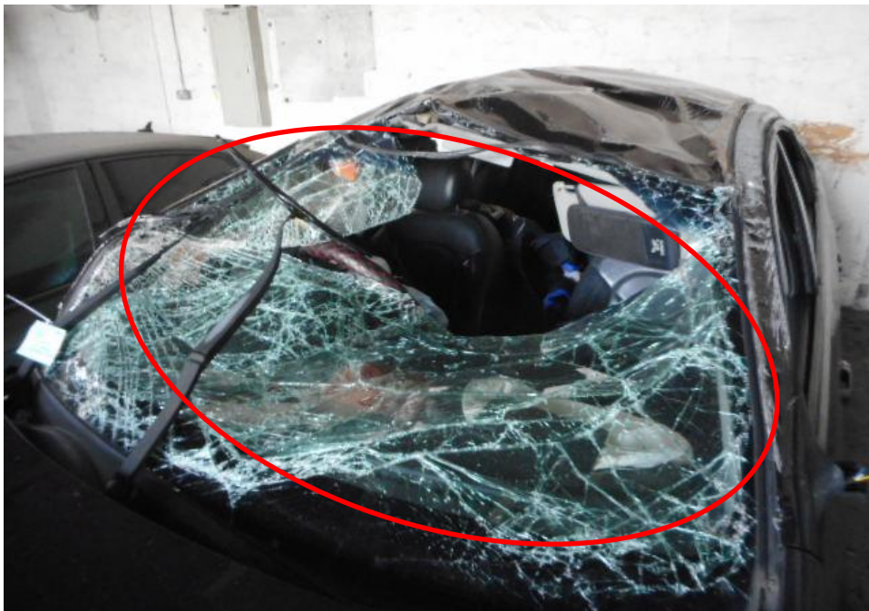
Photo 4 shows the close up view of the Motor Car's front body at the time of my inspection. The Motor Car was observed to have sustained damage at its front portion. Its front windscreen (circled) were amongst the body parts that were damaged as a result of the accident.
