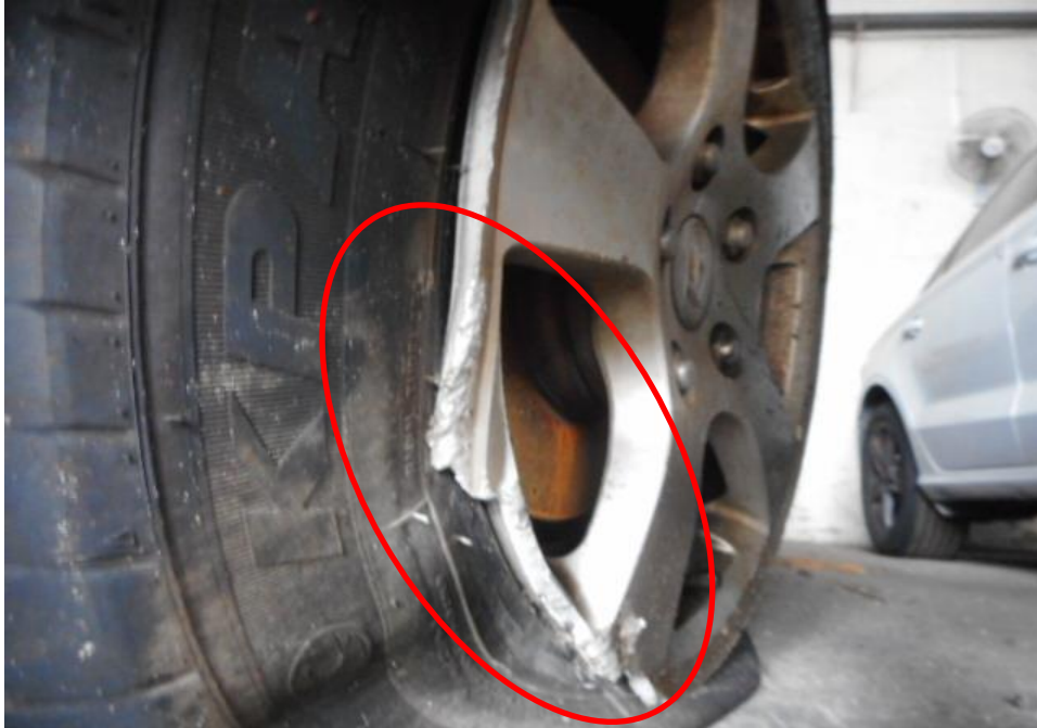
Photo 15 shows the close up view of the condition of the front left tyre of the Motor Car, which was observed to be unserviceable condition. The tyre was observed with cut mark(s) on the outer sidewalls and there was damage observed on the wheel rims (circled) as a result of the accident.
