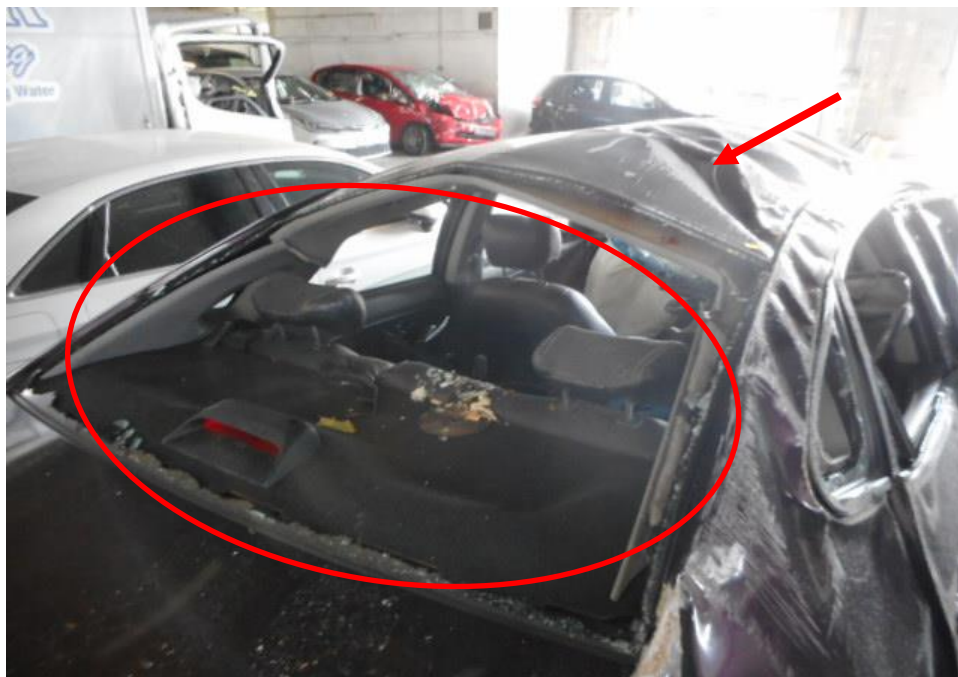
Photo 2 shows the close up view of the Motor Car's rear body at the time of my inspection. The Motor Car was observed to have sustained damage at its rear portion. Its rear windscreen (circled) and roof panel (arrowed) were amongst the body parts that were damaged as a result of the accident.
