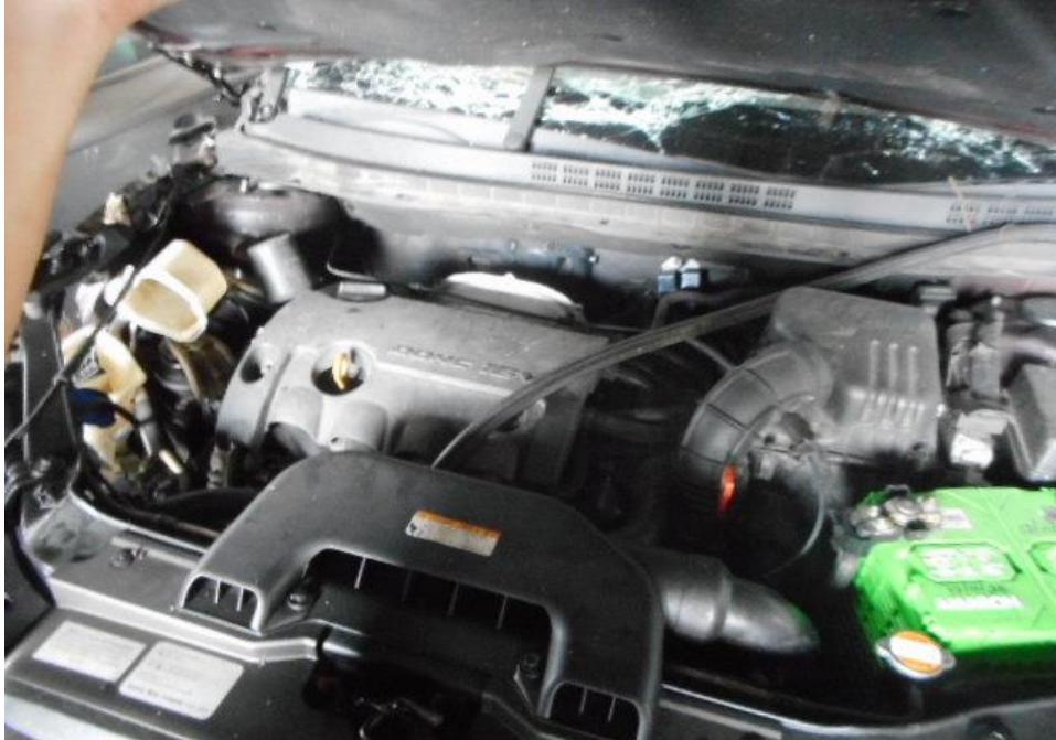
Photo 16 shows a general view of the Motor Car's engine compartment. The coolant reservoir was observed to be damaged as a result of the accident. However the other various parts and components inside the engine compartment were unaffected by the accident. There was also no sign(s) or indication(s) of fluid leakage and/or fluid stain within the engine compartment.
