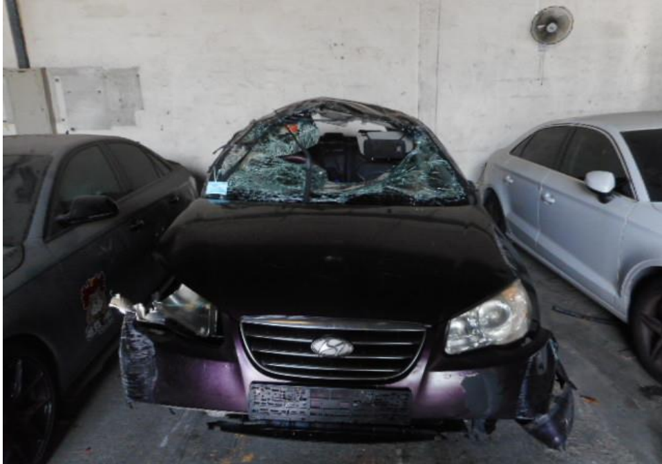
Photo 3 shows a general view of the Motor Car's front body at the time of my inspection. The Motor Car was observed to have sustained damage at its front portion. Its front windscreen, front bumper, front right headlight were amongst the body parts that were damaged as a result of the accident.
