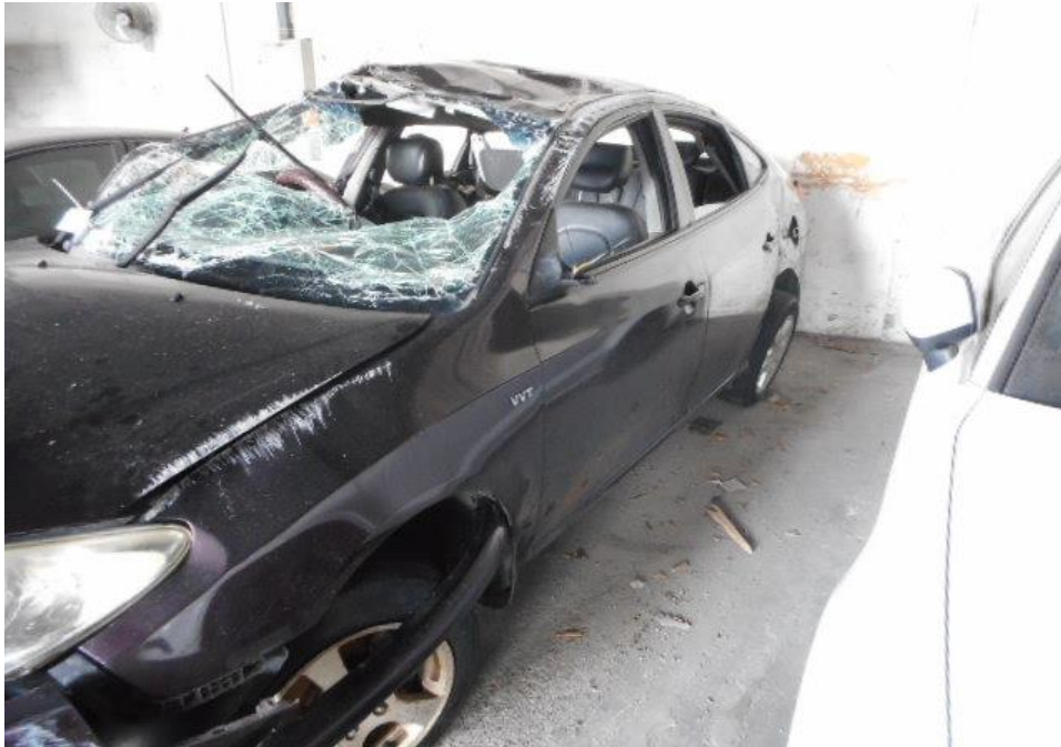
Photo 9 shows a general view of the Motor Car's right body at the time of my inspection. The Motor Car was observed to have sustained damage at its front portion. Its right body panel were amongst the body parts that were damaged as a result of the accident.
