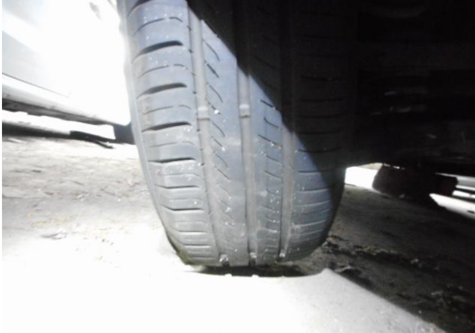
Photo 13 shows the condition of the rear right tyre of the Motor Car, which was observed to be in serviceable condition with remaining tread depth of approximately 5.5mm. The tyre was observed with cut marks and wheel rim damage as a result of the accident, however it was observed to be sufficiently inflated for vehicular operation
