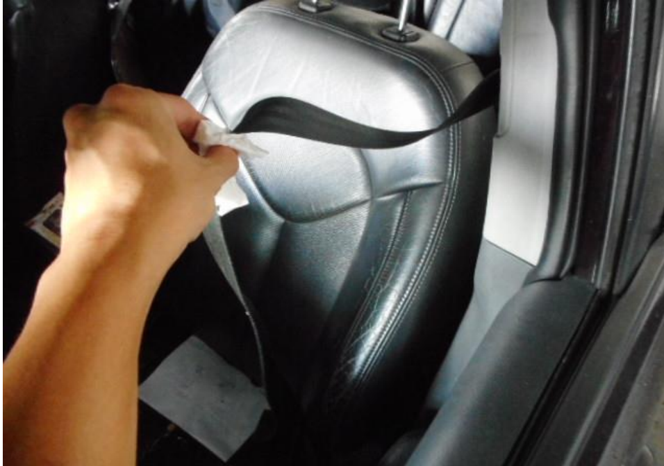
Photo 28 shows that the seat belt on the front left seat was worn at the material time of accident as the safety pre-tensioners was activated at the moment of impact and caused the seat belt to be locked into the last position.
