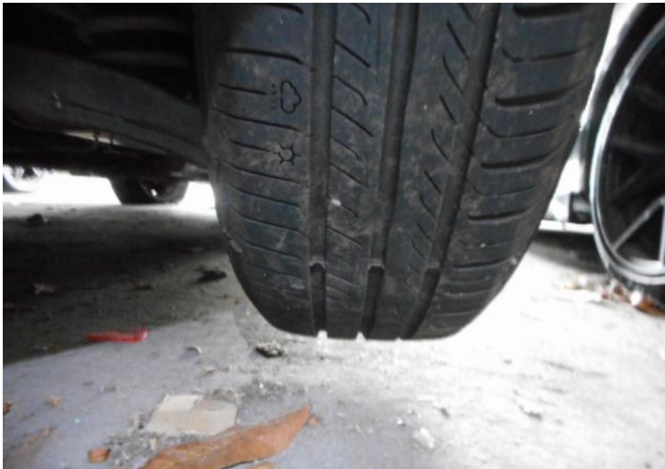
Photo 12 shows the condition of the rear left tyre of the Motor Car, which was observed to be in serviceable condition with remaining tread depth of approximately 6.1mm. The tyre was observed with cut marks and wheel rim damage as a result of the accident, however it was observed to be sufficiently inflated for vehicular operation
