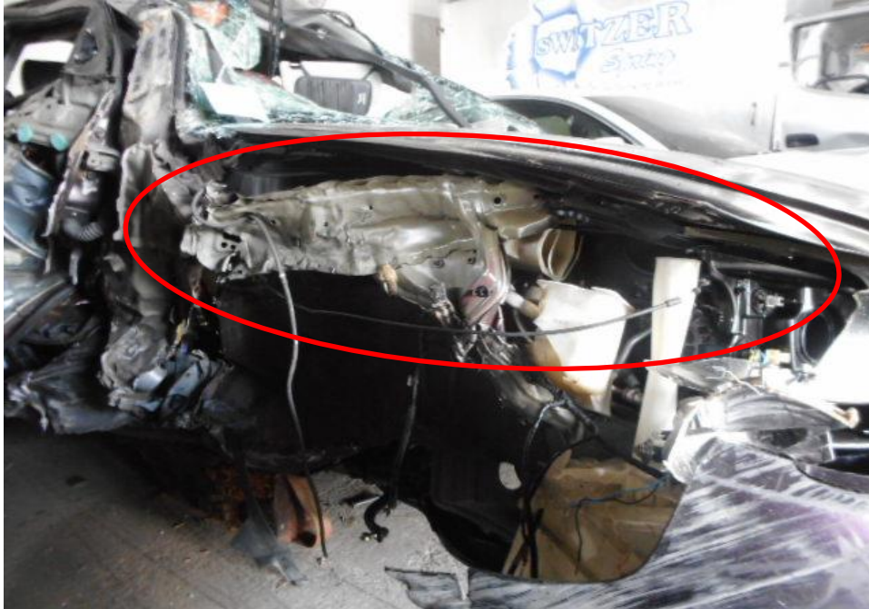
Photo 7 shows a close up view of the Motor Car's right body at the time of my inspection. The Motor Car was observed to have sustained damage at its right portion. Its right body panels (circled) were amongst the body parts that were damaged as a result of the accident.
