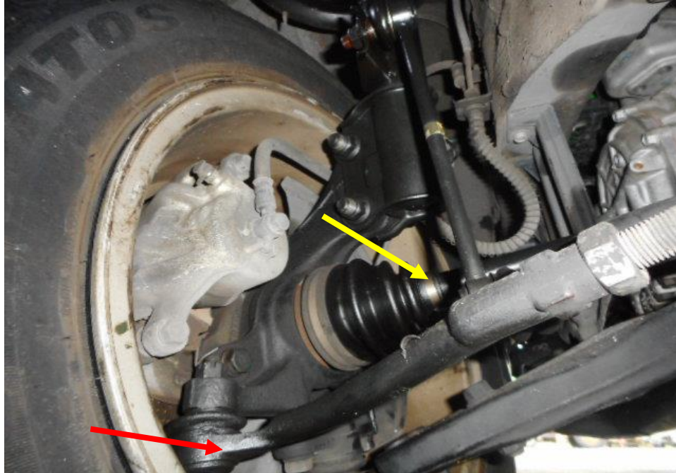
Photo 25 shows the various undercarriage components at the front left wheel of the Motor Car, in particular the steering tie rod (red arrow) and the driveshaft (yellow arrow). The various steering components were all found to be intact and undamaged by the accident.
