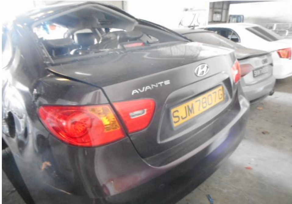
Photo 1 shows the general view of the Motor Car's rear body at the time of my inspection. The Motor Car was observed to have sustained damage at its rear portion. Its rear windscreen and roof panel were amongst the body parts that were damaged as a result of the accident.
