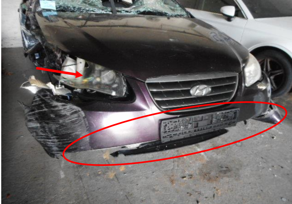
Photo 5 shows the close up view of the Motor Car's front body at the time of my inspection. The Motor Car was observed to have sustained damage at its front portion. Its front bumper (circled) and front right headlight (arrowed) were amongst the body parts that were damaged as a result of the accident.
