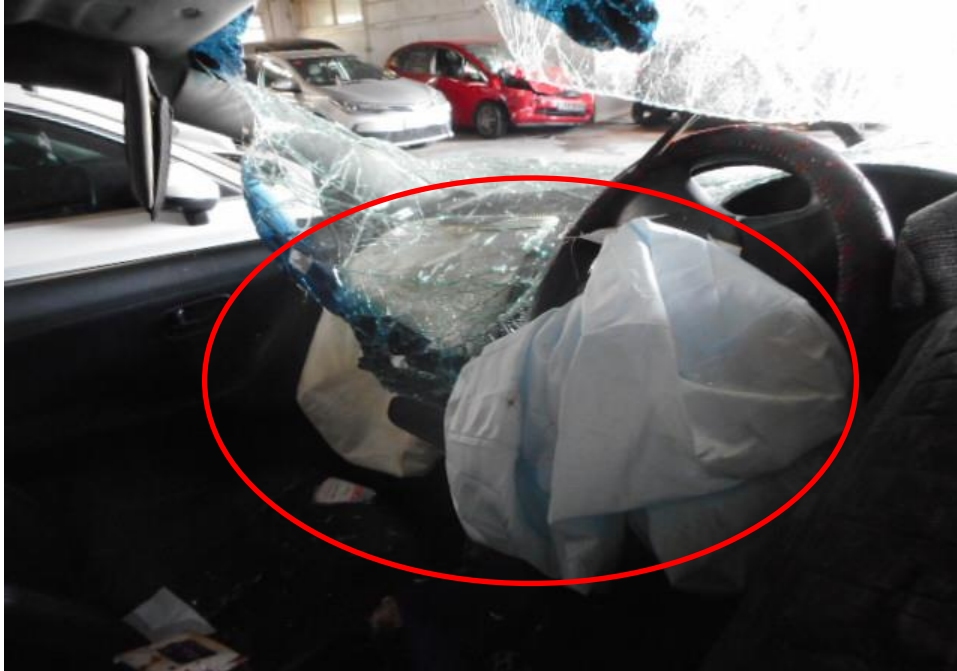
Photo 11 shows the airbag (circled) of the Supplemental Restraint System in the Motor Car's was deployed as a result of the accident at the time of my inspection.
