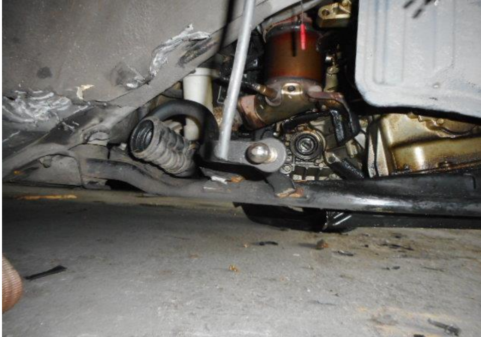
Photo 23 shows the missing front right braking system due to the result of the accident.
