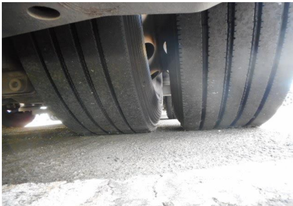
Photo 7 shows the condition of the rear right tyre of the Motor Bus, which was observed to be in serviceable condition with remaining tread depth of approximately 10mm. The tyre, which was wrapped around standard steel wheel rim, was also observed to be sufficiently inflated for vehicular operation.
