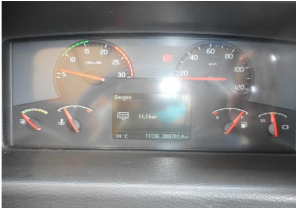
Photo 25 shows no warning lights illuminated on the instrument panel of the Motor Bus after the engine was cranked. This would suggest that there was no abnormality to the various electronic operating systems of the Motor Bus, like the TCS and etc.
