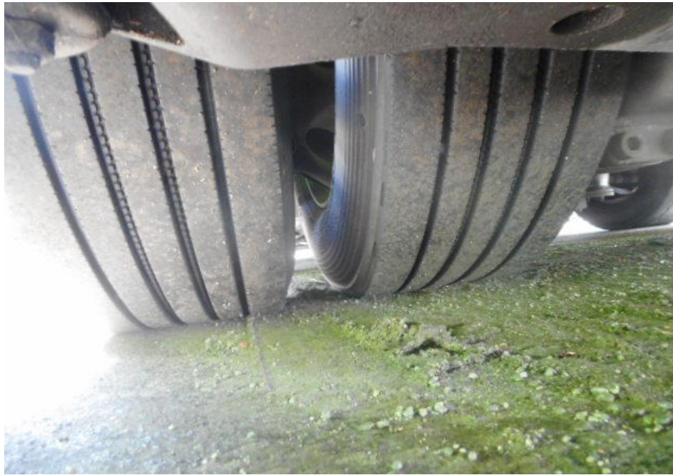
Photo 8 shows the condition of the rear left tyres of the Motor Bus, which was observed to be in serviceable condition with remaining tread depth of approximately 9.5mm. The tyres, which were wrapped around standard steel wheel rim, were also observed to be sufficiently inflated for vehicular operation. There was also no damage found on all 8 steel wheel rims of the Motor Bus.
