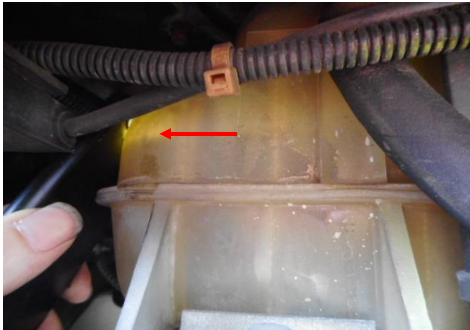
Photo 12 shows the engine coolant reservoir of the Motor Bus at the time of my inspection. The engine coolant was observed to be of sufficient level (arrowed) and without any visible contamination.
