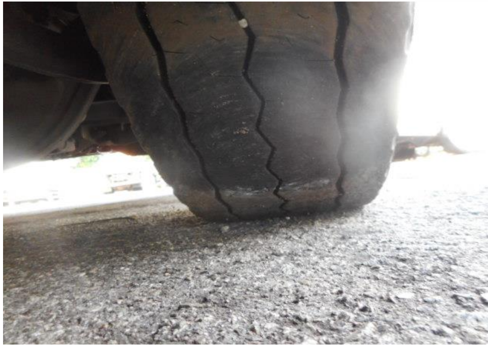
Photo 6 shows the condition of the front right tyre of the Motor Bus, which was observed to be in serviceable condition with remaining tread depth of approximately 9.8mm. The tyre, which was wrapped around standard steel wheel rim, was also observed to be sufficiently inflated for vehicular operation. There was no tear, cut or burst mark(s) on the outer and the inner sidewalls as well as across the tread of the 8 tyres that were fitted on the Motor Bus.
