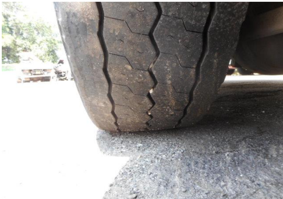
Photo 9 shows the condition of the front left tyres of the Motor Bus, which were observed to be in serviceable condition with remaining tread depth of approximately 9.1mm. There was also no tear, cut or burst mark(s) on the outer and the inner sidewalls as well as across the tread of the 8 tyres that were fitted on the Motor Bus.
