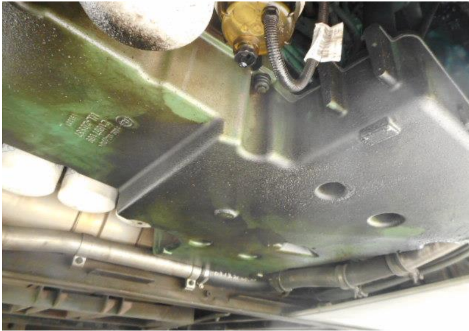
Photo 22 shows the undercarriage of the Motor Bus, at the area where the engine housing and transmission housing are located. I did not find any sign(s) or indication(s) of fluid leak and/or fluid stain(s) on the underside of the Motor Bus.
