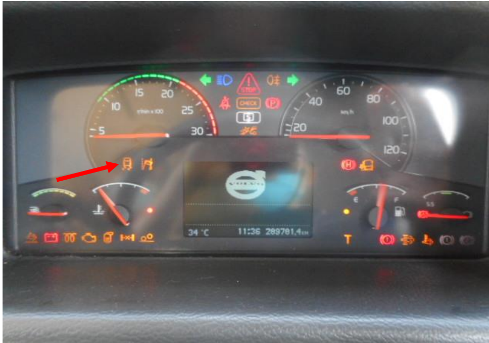
Photo 24 shows the warning light for Traction Control System (TCS) appearing on the instrument panel of the Motor Bus during the self-test of its various electronic operating systems when its engine was cranked.
