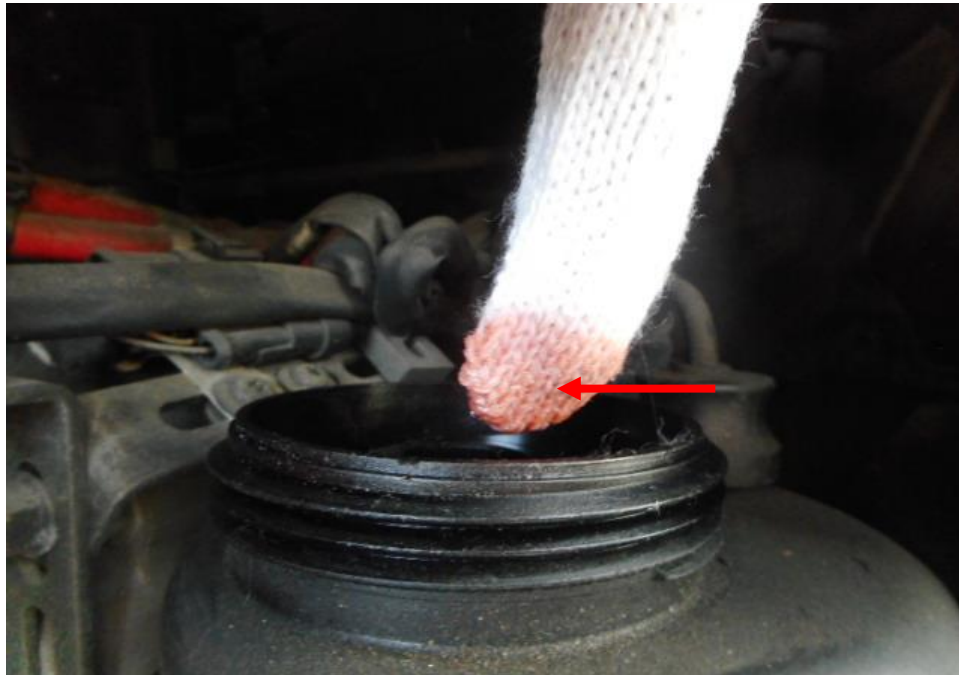
Photo 13 shows the power steering fluid reservoir of the Motor Bus at the time of my inspection. The power steering fluid was observed to be of sufficient level and without any visible contamination.
