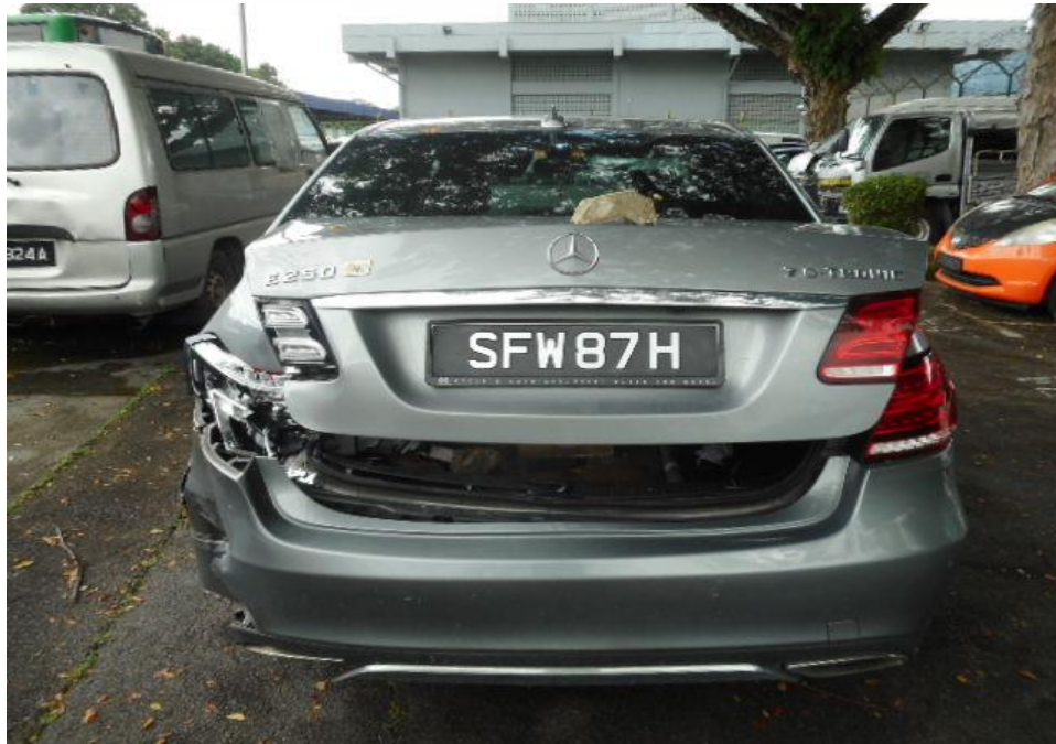
Photo 2 shows a general view of the Motor Car's rear body at the time of my inspection. The rear portion. Its rear bonnet, rear left brake lamp and rear bumper was the body parts that were damaged as a result of the accident.
