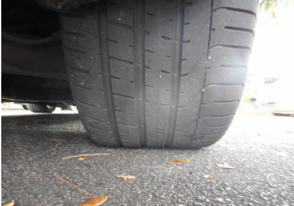
Photo 8 shows the condition of the rear right tyre of the Motor Car, which was observed to be in serviceable condition with remaining tread depth of approximately 4.9mm. The tyre was also observed to be sufficiently inflated for vehicular operation with no tear, cut or burst mark(s).
