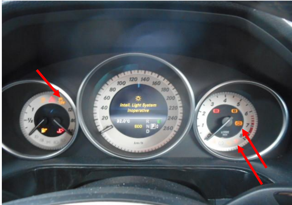
Photo 23 shows the warning light for Anti-Lock Brake System (ABS), Traction Control System (TCS) and Supplemental Restraint System (SRS) (arrowed) appearing on the instrument panel of the Motor Car during the self-test of its various electronic operating systems when its engine was cranked.
