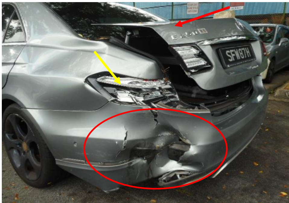
Photo 3 shows a close up view of the Motor Car's rear body at the time of my inspection. The rear portion of the Motor Car was observed to have sustained damage. Its rear bonnet (circled), rear left brake light (yellow arrow) and rear bonnet (red arrow) was the body parts that were damaged as a result of the accident.
