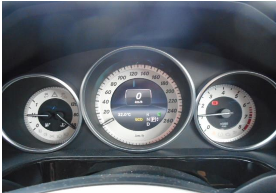
Photo 24 shows no warning lights illuminated on the instrument panel of the Motor Car after the engine was cranked. This would suggest that there was no abnormality to the electronic operating system of the Motor Car, like the ABS, TCS and SRS etc.
