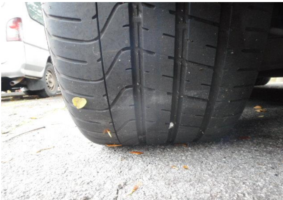
Photo 9 shows the condition of the rear left tyre of the Motor Car, which was observed to be in serviceable condition with remaining tread depth of approximately 5mm. The tyre, which was wrapped around steel wheel rim, was also observed to be sufficiently inflated for vehicular operation. The 4 tyres of the Motor Car were wrapped around standard steel wheel rims.
