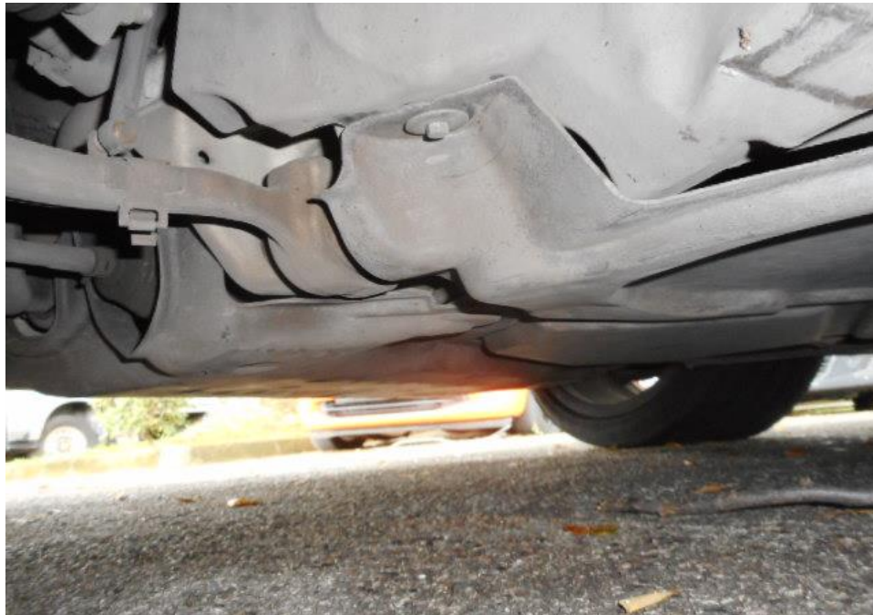
Photo 15 shows the undercarriage of the Motor Car, at the area where the engine housing and transmission housing are located. I did not find any sign(s) or indication(s) of fluid leak and/or fluid stain(s) on the underside of the Motor Car.
