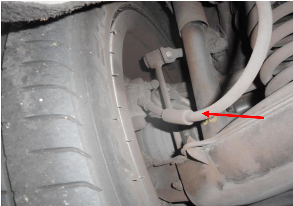
Photo 17 shows the brake hose/pipe (arrowed) at the rear left wheel of the Motor Car. I did not observe any leakage of brake fluid at the time of my inspection of the Motor Car. Static tests of the Motor Car's braking system had indicated that there was no internal leakage of pressure/vacuum. The undercarriage components of the Motor Car were also all found to be intact and without any visible damage.
