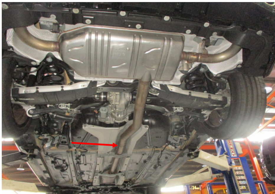
Photo 23 shows a general view of the rear section of the Motor Car's exhaust system. My examination of the Motor Car's exhaust system revealed no sign(s) or indication(s) of any cut or weld marks along its exhaust pipe (arrowed), on its catalytic converter, centre resonator box and on its rear muffler.
