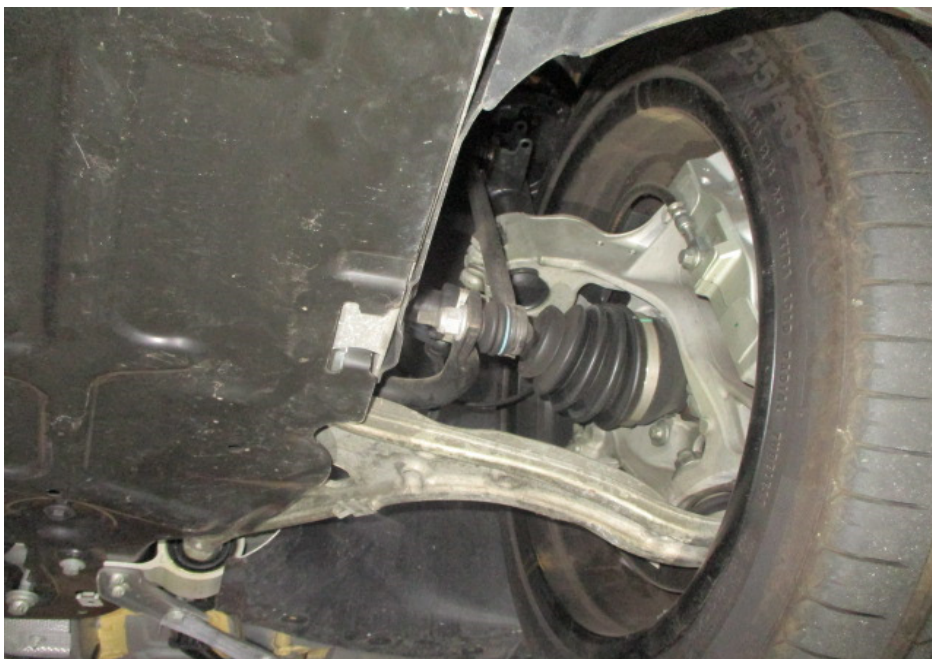
Photo 21 shows the various undercarriage components at the front left wheel of the Motor Car. The mechanical components, control arms and linkages were all found to be intact and secured in an appropriate manner.
