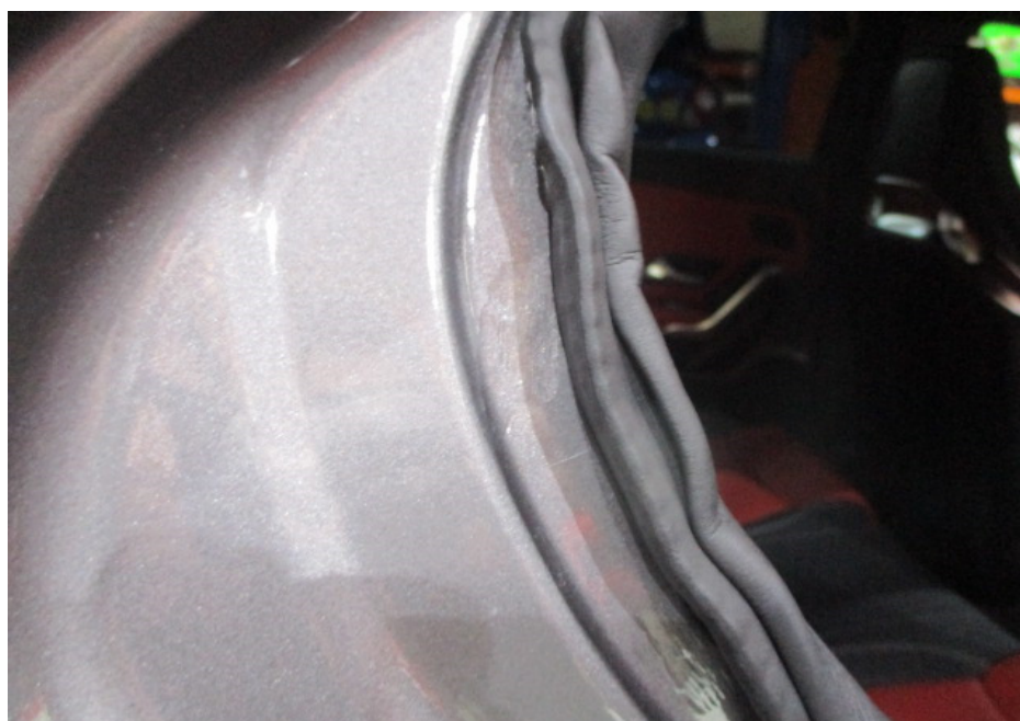
Photo 29 shows the right side "C" pillar of the Motor Car. I did not find any original weld marks at the right side "C" pillar of the Motor Car, indicating that the rear right fender of the Motor Car was replaced. The lack of original weld marks seen was due to replacement work when the replaced rear right fender was re-welded onto the Motor Car and smoothen for re-spraying work.
