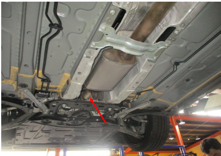
Photo 24 shows a general view of the front section of the Motor Car's exhaust system. My examination of the Motor Car's exhaust system revealed no sign(s) or indication(s) of any cut or weld marks along its exhaust pipe, on its catalytic converter (arrowed), centre resonator box and on its rear muffler.
