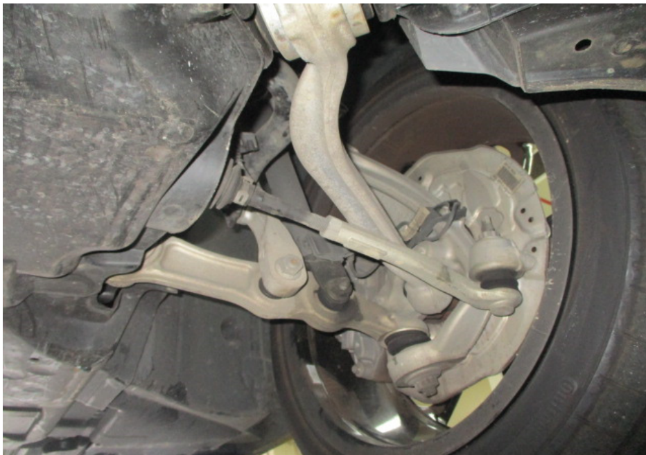
Photo 24 shows the various undercarriage components at the front left wheel of the Motor Car. The mechanical components, control arms and linkages were all found to be intact and secured in an appropriate manner.
