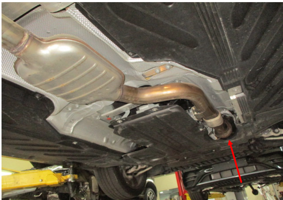
Photo 27 shows the front section of the Motor Car's exhaust system. My examination of the Motor Car's exhaust system revealed no sign(s) or indication(s) of any cut or weld marks along its exhaust pipes, on its centre resonator boxes, on its rear mufflers and on its catalytic converter (arrowed).
