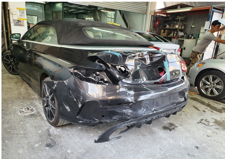
Photo 1 shows the rear left body of the Motor Car (photograph provided to me). The Motor Car was observed to have sustained damage at its rear portion. Body parts damaged include the rear bumper, rear bumper lower cover, rear bumper left reflector, rear bumper sensors, rear left exhaust garnish, rear bootlid, rear bootlid lock and rear bootlid emblem amongst others.
