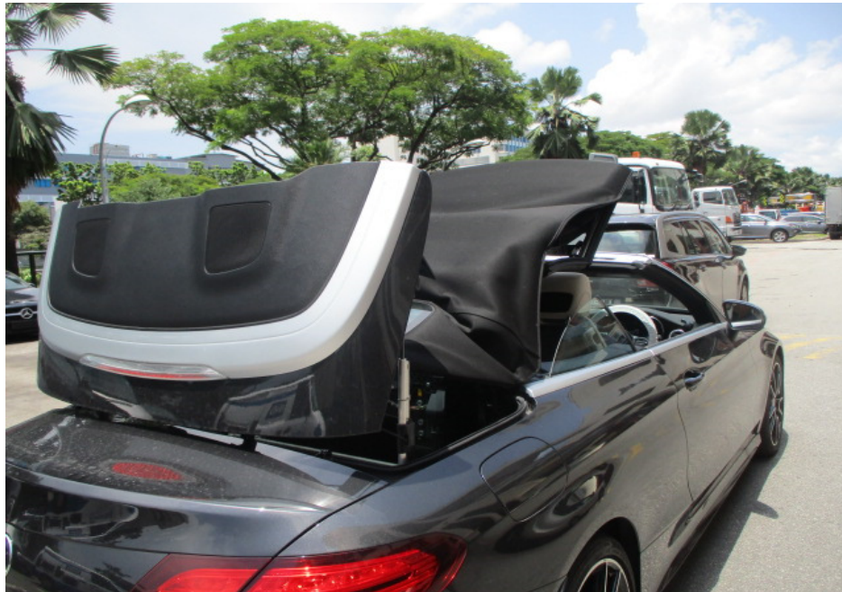
Photo 13 shows the Motor Car's soft top being tested. It was observed that as a safety feature, the soft top could only open and close when the Motor Car was in a stationary position. When opened, the soft top is completely folded into the rear storage compartment with no parts protruding out of the Motor Car's body. The soft top was also found adequately secured to the "A" pillar after closing.
