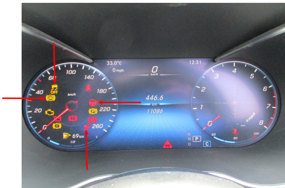
Photo 19 shows the warning lights for the various electronic safety features appearing on the instrument panel of the Motor Car during its self-test when the engine is cranked, in particular the ABS, SRS, EPS and TCS lights (arrowed).
