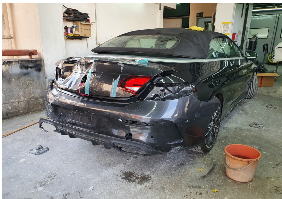
Photo 2 shows the rear right body of the Motor Car (photograph provided to me). The Motor Car was observed to have sustained damage at its rear portion. Body parts damaged include the rear bumper, rear bumper lower cover, rear bumper tow hook cover, rear bumper right reflector, rear bumper sensors, rear right exhaust garnish, rear bootlid and rear bootlid emblem amongst others.
