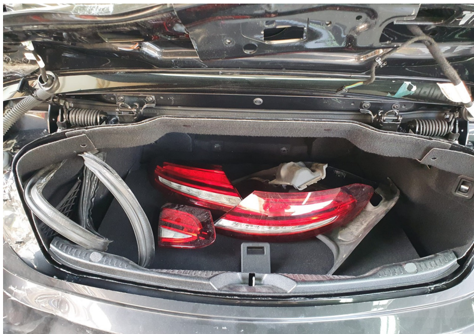
Photo 3 shows the rear boot compartment of the Motor Car (photograph provided to me). The rear right taillamp, rear left taillamp and rear left bootlid lamp placed in the rear boot compartment appears to be not damaged as seen from the photograph.
