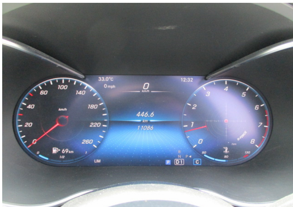
Photo 20 shows the respective warning lights no longer illuminated, indicating that there is no fault detected to the ABS, SRS, EPS TCS systems of the Motor Car during the self-test. These electronic systems were hence in working condition at the time of my inspection.
