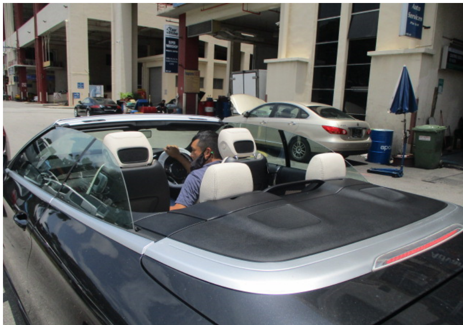
Photo 14 shows the Motor Car with its soft top completely folded. It was observed that as a safety feature, the soft top could only open and close when the Motor Car was in a stationary position. When opened, the soft top is completely folded into the rear storage compartment with no parts protruding out of the Motor Car's body. The soft top was also found adequately secured to the "A" pillar after closing.
