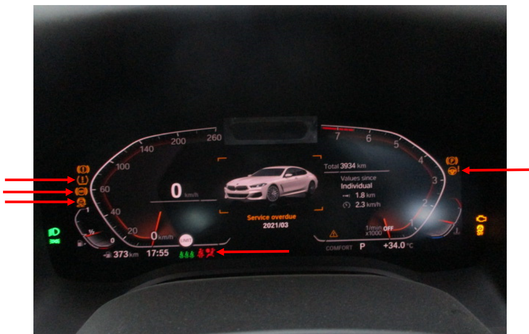
Photo 16 shows the warning lights for the various electronic safety features appearing on the instrument panel of the Motor Car during its self-test when the engine is cranked, in particular the ABS, SRS, IAS, TPM and DSC lights (arrowed).
