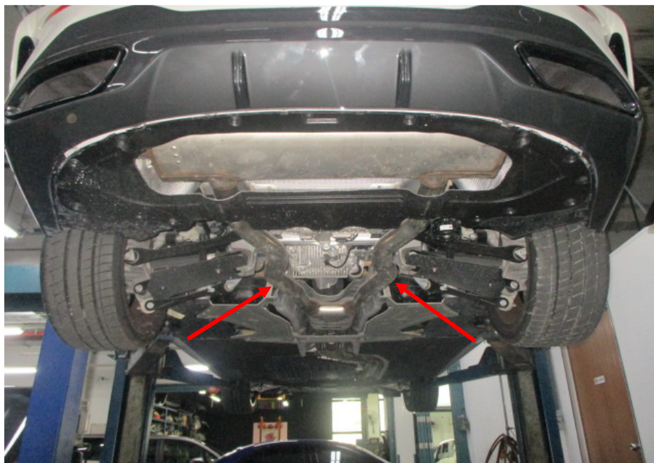
Photo 23 shows the rear section of the Motor Car's exhaust system. My examination of the Motor Car's exhaust system revealed no sign(s) or indication(s) of any cut or weld marks along its exhaust pipes (arrowed), on its centre resonator box, on its rear muffler and on its catalytic converter.
