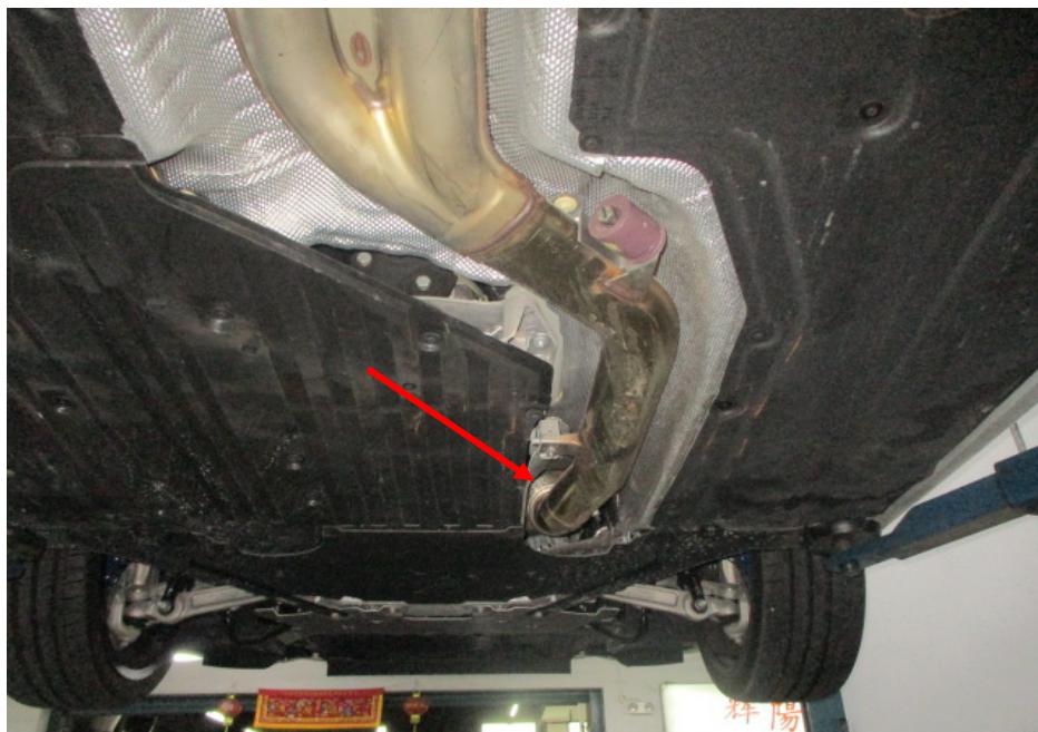
Photo 24 shows the front section of the Motor Car's exhaust system. My examination of the Motor Car's exhaust system revealed no sign(s) or indication(s) of any cut or weld marks along its exhaust pipes, on its centre resonator box, on its rear muffler and on its catalytic converter (arrowed).
