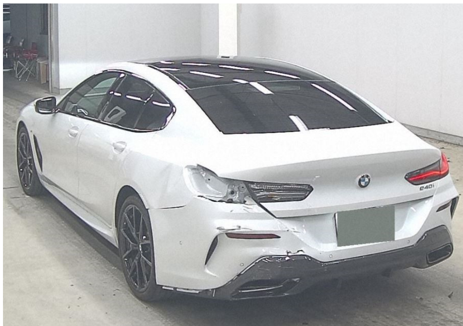
Photo 1 shows a general view of the rear left body of the Motor Car (photograph provided to me). The Motor Car was observed to have sustained relatively minor damage at its rear left portion. Body parts damaged include the rear bumper, rear bumper lower cover, rear left exhaust garnish, rear left taillamp, rear bootlid and rear left fender amongst others.
