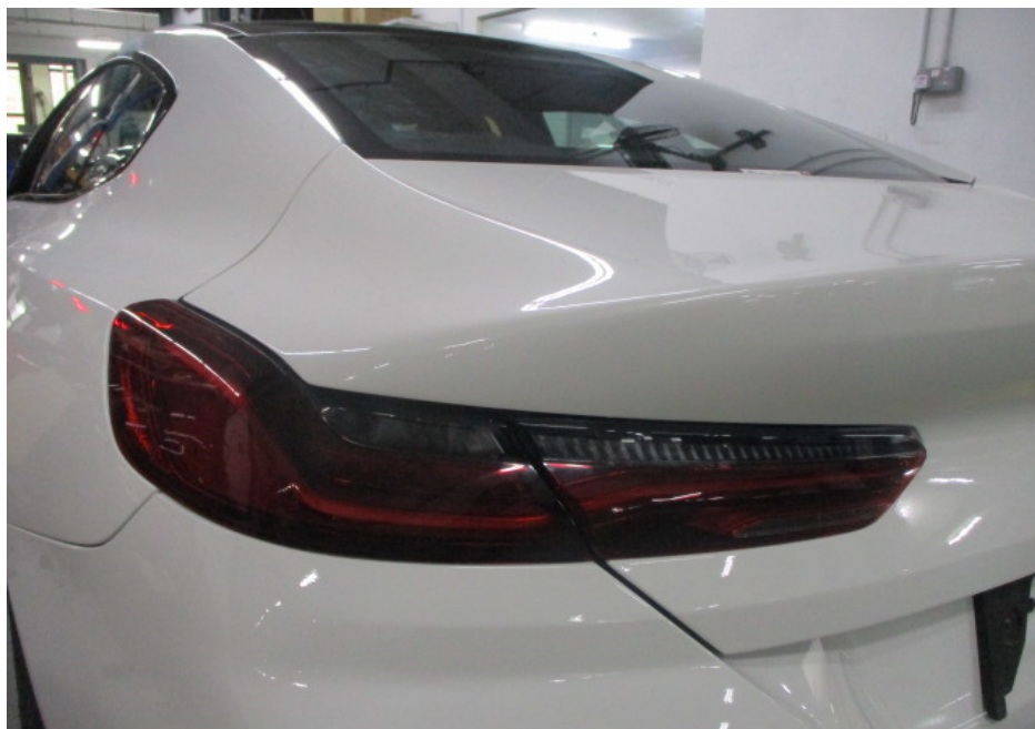
Photo 6 shows a closer view of the Motor Car's rear bootlid, rear left bootlid lamp and rear left taillamp. The body parts at the rear left portion of the Motor Car were visually examined and it was observed that the repair/restoration works carried out to the damaged area of the Motor Car (refer to photograph 1 above) were reasonably adequate and in order.
