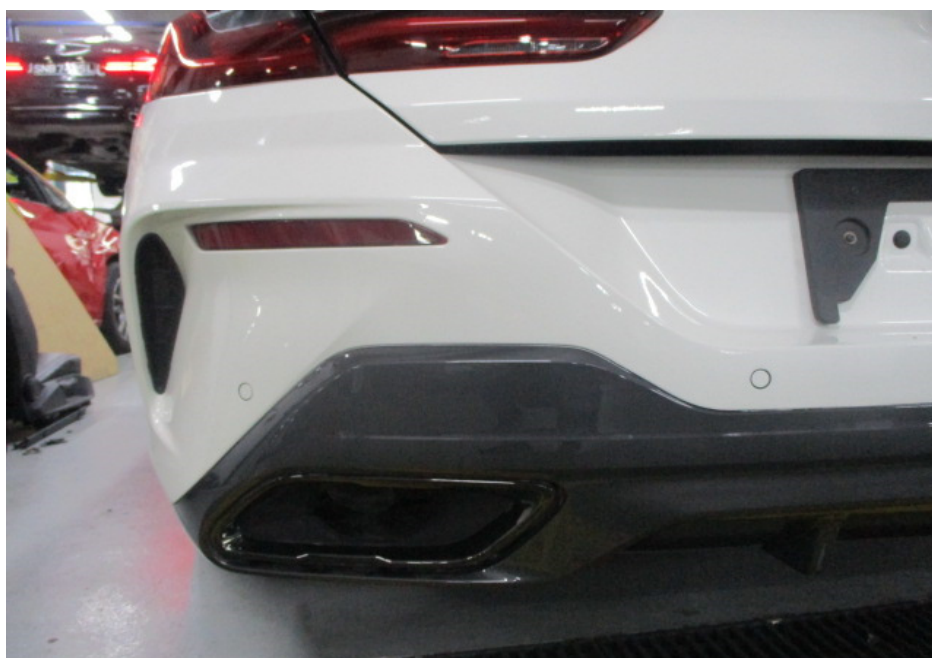
Photo 7 shows a closer view of the Motor Car's rear bumper, rear bumper lower cover and rear left exhaust garnish. The body parts at the rear left portion of the Motor Car were visually examined and it was observed that the repair/restoration works carried out to the damaged area of the Motor Car (refer to photograph 1 above) were reasonably adequate and in order.
