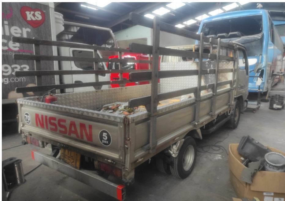
Photo 1 shows a general view of the rear right body of the Insured Vehicle at the time of inspection. The Insured Vehicle was observed to have sustained fire damage at its rear deck. This was at the right side front of the rear deck, directly behind the right side of the Insured Vehicle's front cabin.
