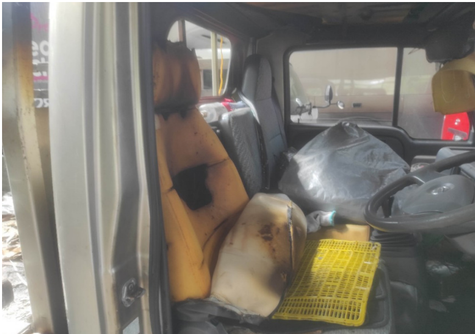
Photo 6 shows a closer view of the partially burnt driver's seat in the interior compartment of the Insured Vehicle's front cabin. The driver's seat and roof upholstery amongst others in the interior compartment of the front cabin was affected by the fire.
