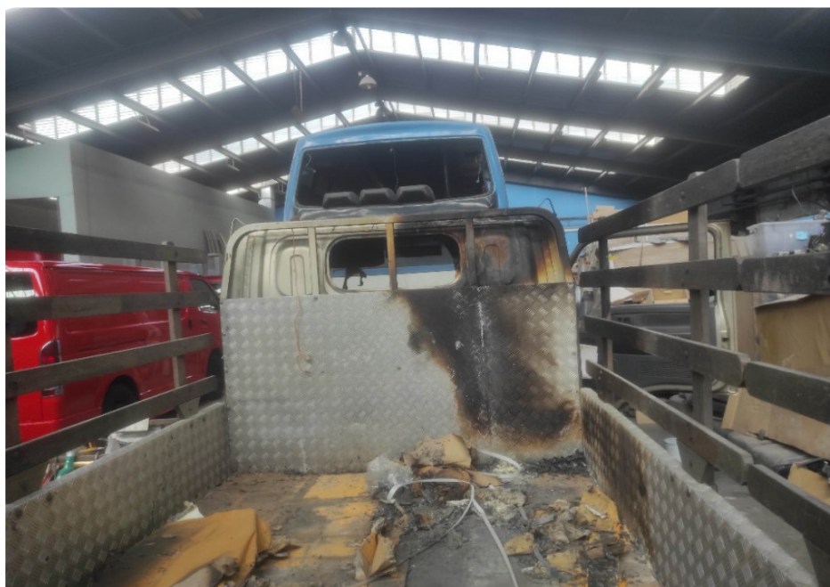
Photo 2 shows a general view of the right side front of the Insured Vehicle's rear deck. The Insured Vehicle was observed to have sustained fire damage at its rear deck. This was at the right side front of the rear deck, directly behind the right side of the Insured Vehicle's front cabin. The aluminium plates surrounding the right side front of the rear deck, the vertical wooden side gate extension at the right side front of the Insured Vehicle and the rear exterior of the front cabin at the right side amongst others, were found with fire damage.
