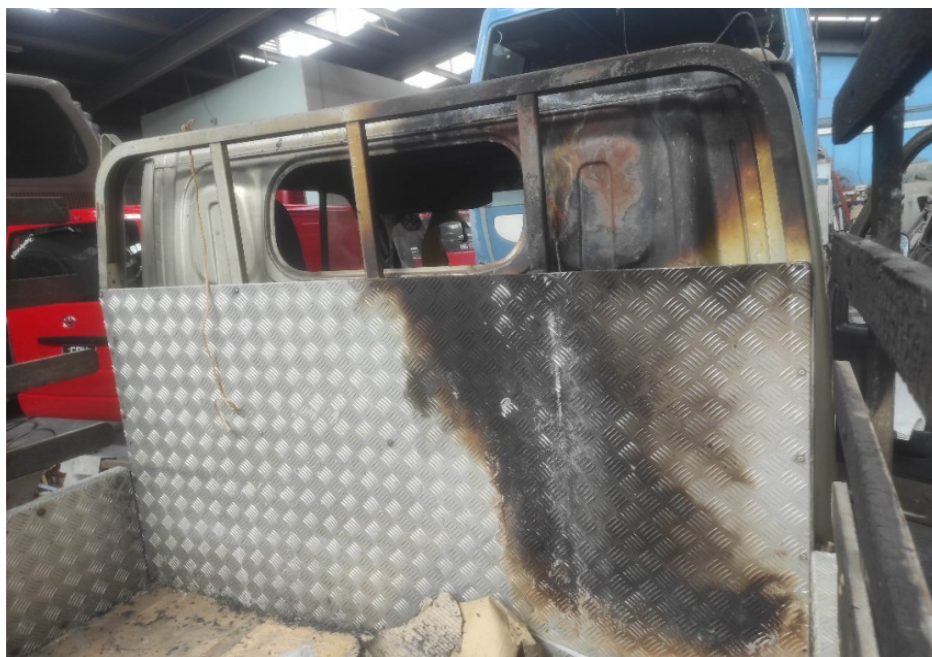
Photo 4 shows another view of the partially burnt aluminium plates surrounding the right side front of the Insured Vehicle's rear deck. The rear exterior of the front cabin at the right side was also observed to be partially burnt. The front cabin glass window was shattered as a result of the fire.
