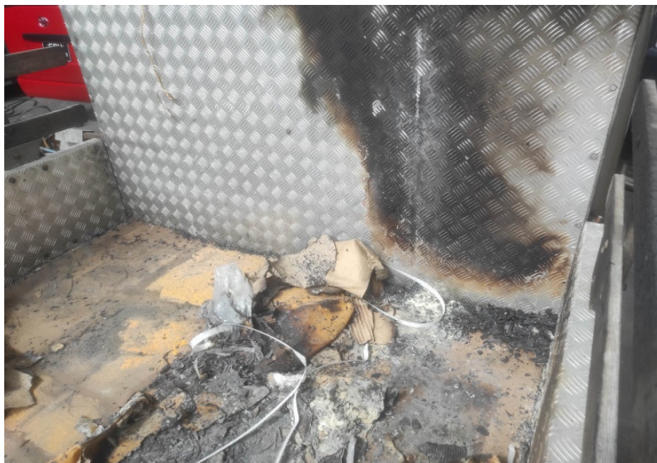
Photo 3 shows a closer view of the partially burnt aluminium plates surrounding the right side front of the Insured Vehicle's rear deck.
