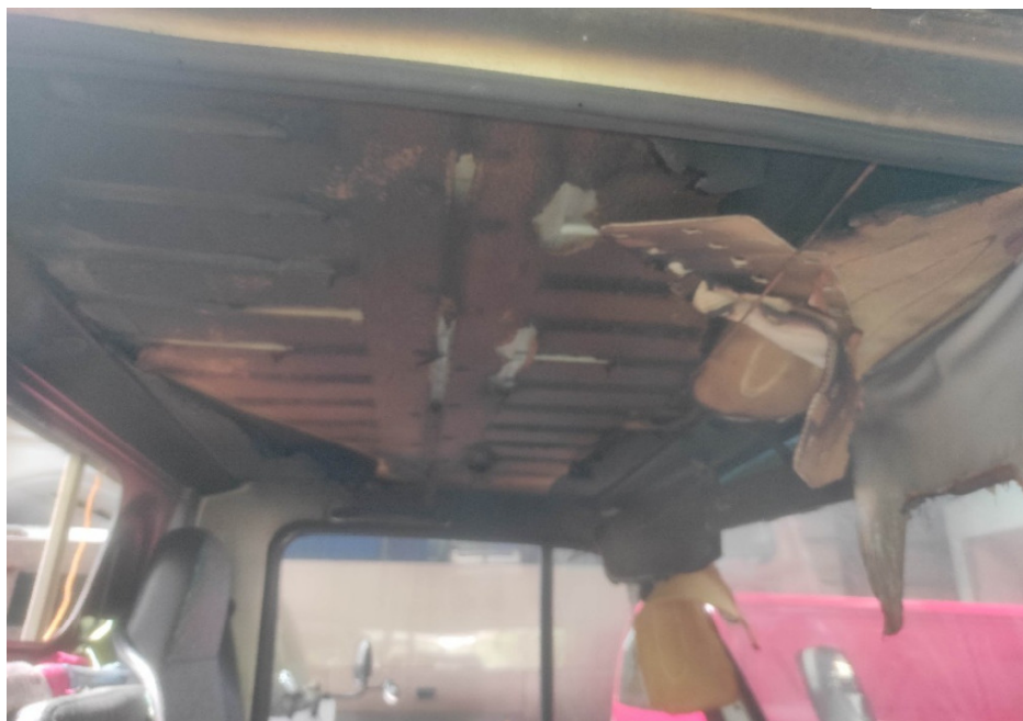
Photo 7 shows a closer view of the partially burnt roof upholstery in the interior compartment of the Insured Vehicle's front cabin. The driver's seat and roof upholstery amongst others in the interior compartment of the front cabin was affected by the fire.
