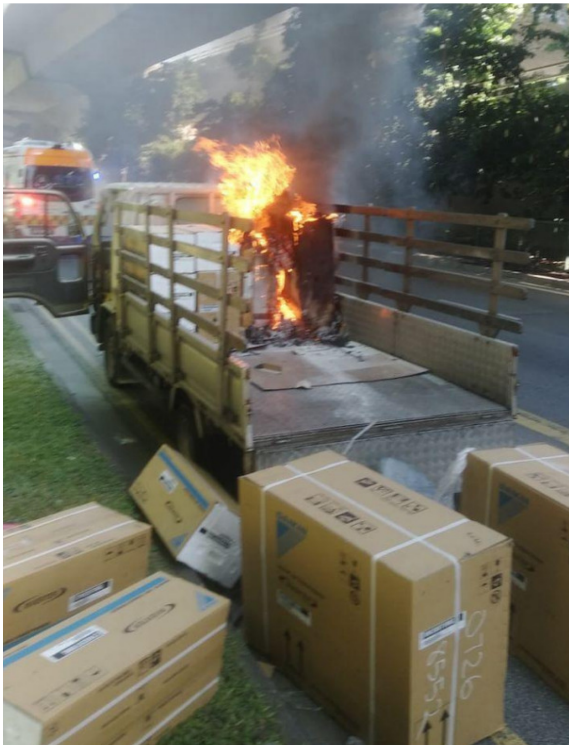
Photo 12 shows the Insured Vehicle at the incident scene (photograph extracted from Mr Leong's Singapore Accident Statement). Fire can be seen engulfing the same new air conditioning compressor that had emitted the white smoke that was seen in the video recordings (refer to photograph 10 above). This new air conditioning compressor was noted to be at the right side front of the Insured Vehicle's rear deck.
