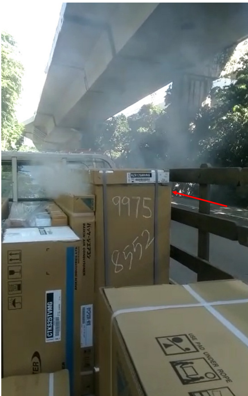
Photo 10 shows a screenshot extracted from one of the video recordings that were provided to me by Mr Leong. White smoke can be seen coming out from one of the new air conditioning compressors (arrowed) at the right side front of the Insured Vehicle's rear deck. Hissing sound was also heard in one of the video recordings.
