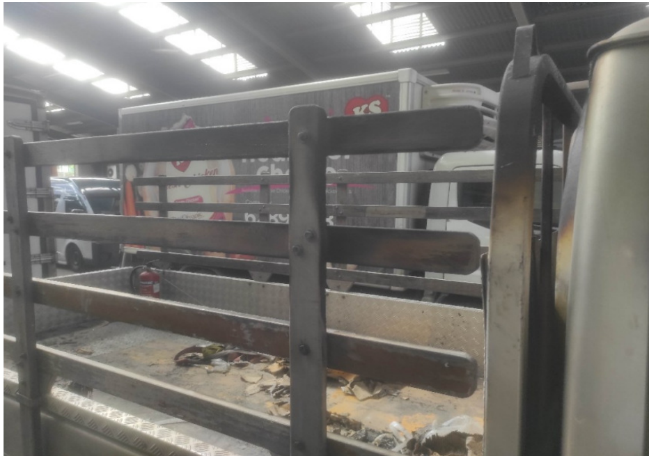
Photo 5 shows a closer view of the partially burnt vertical wooden side gate extension at the right side front of the Insured Vehicle.
