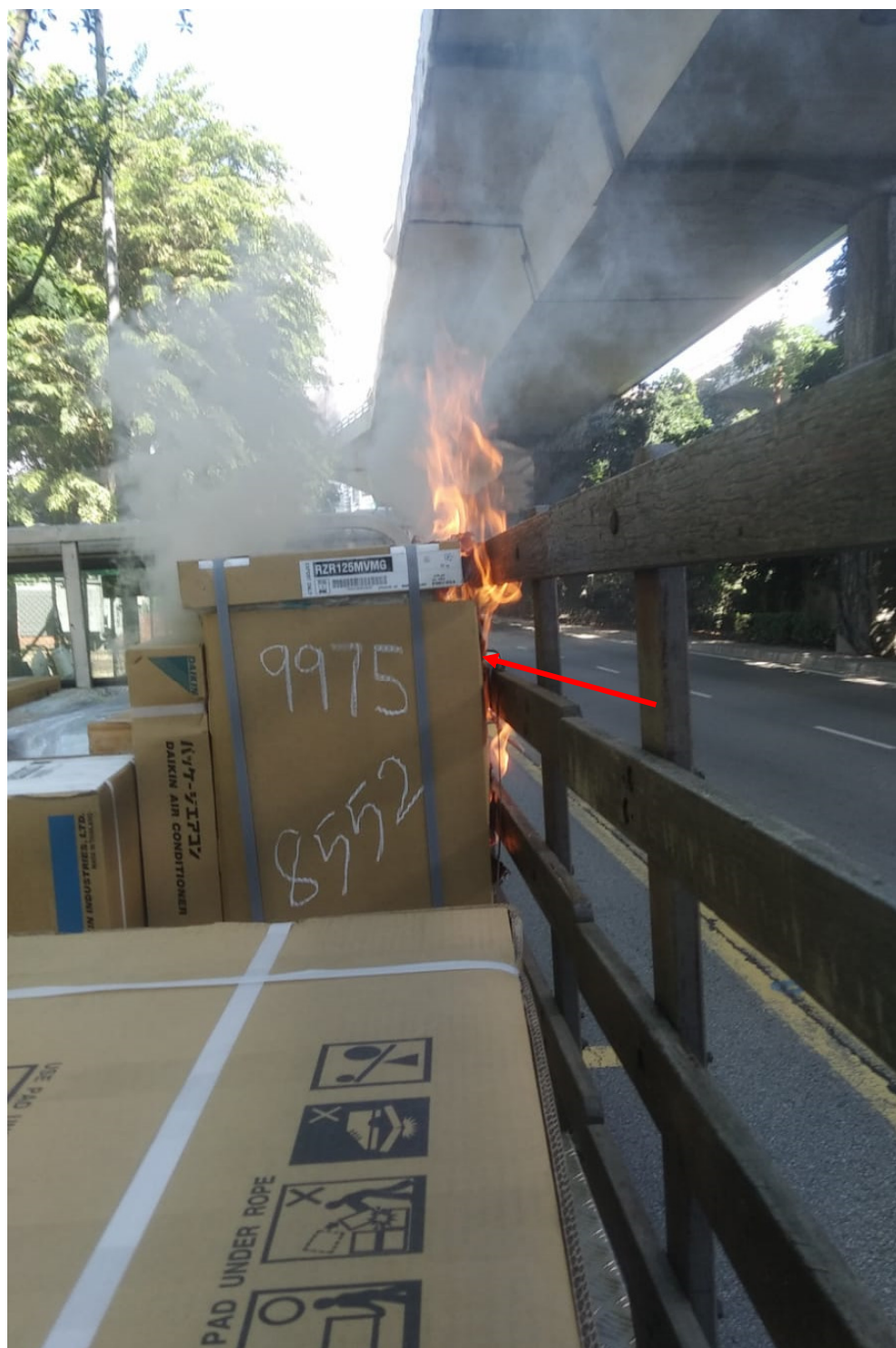
Photo 11 shows the Insured Vehicle at the incident scene (photograph extracted from Mr Leong's Singapore Accident Statement). Fire can be seen engulfing the same new air conditioning compressor (arrowed) that had emitted the white smoke that was seen in the video recordings (refer to photograph 10 above). The brand of the new air conditioning equipment(s) loaded on the rear deck of the Insured Vehicle was observed to be Daikin.
