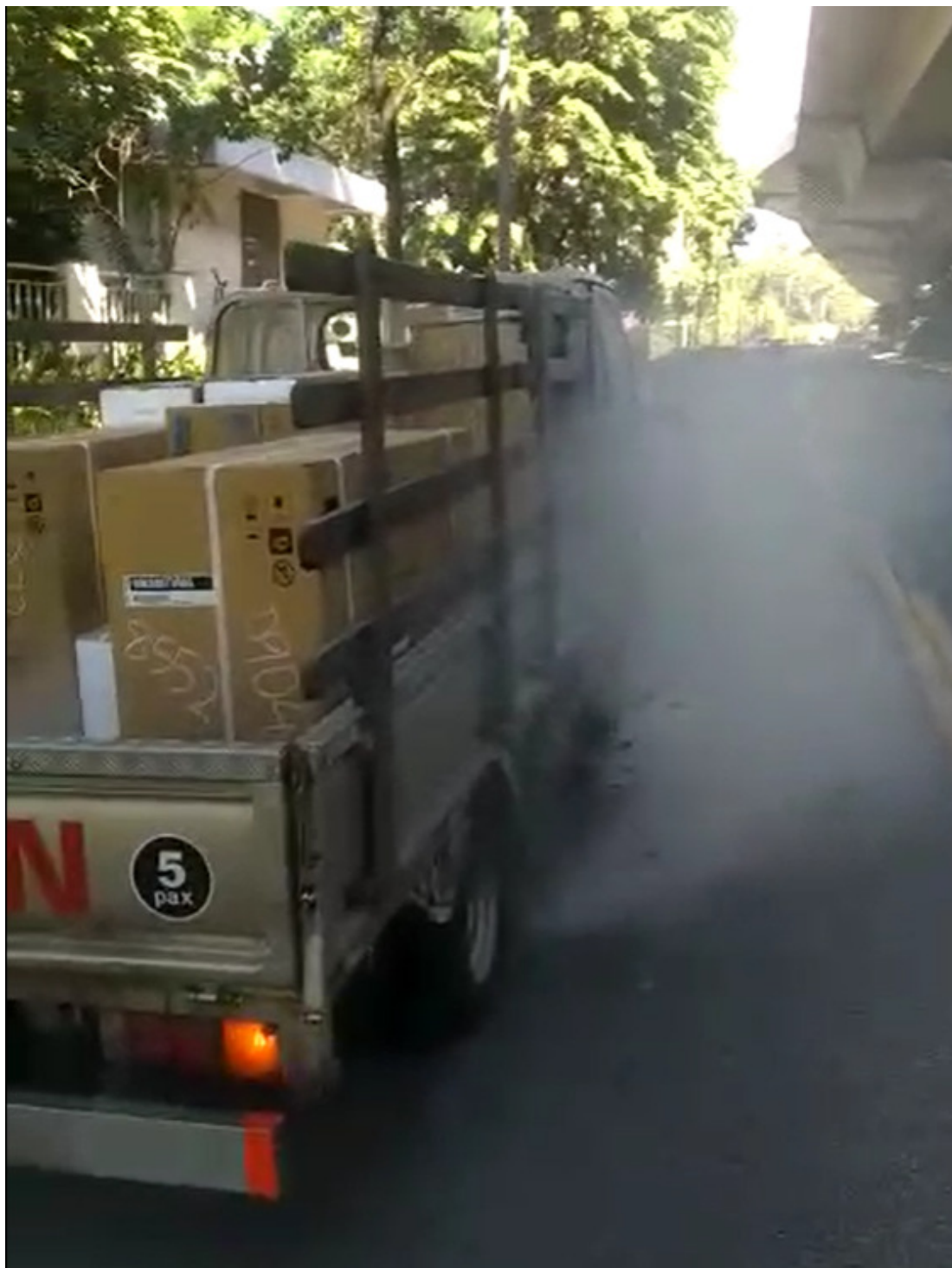
Photo 9 shows a screenshot extracted from one of the video recordings that were provided to me by Mr Leong. The Insured Vehicle can be seen stopped on the left lane with white smoke coming out from one of the new air conditioning compressors at the right side front of the Insured Vehicle's rear deck. Hissing sound was also heard in one of the video recordings.
