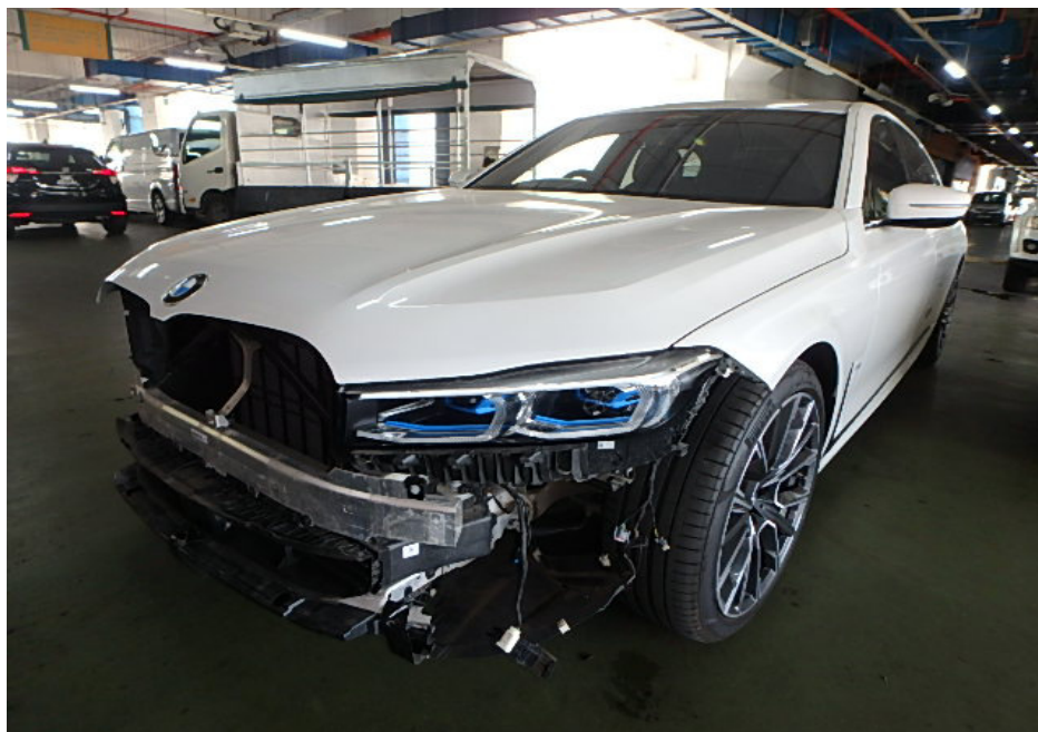
Photo 3 shows the front left body of the Motor Car (photograph provided to me). The front bumper and all its related parts and attachments like the front bumper centre lower grille, front bumper left and right lower grilles, front bumper left and right lower grille garnishes amongst others, front right headlamp and radiator grilles were damaged/missing/dislodged (refer to photograph 1 above).
