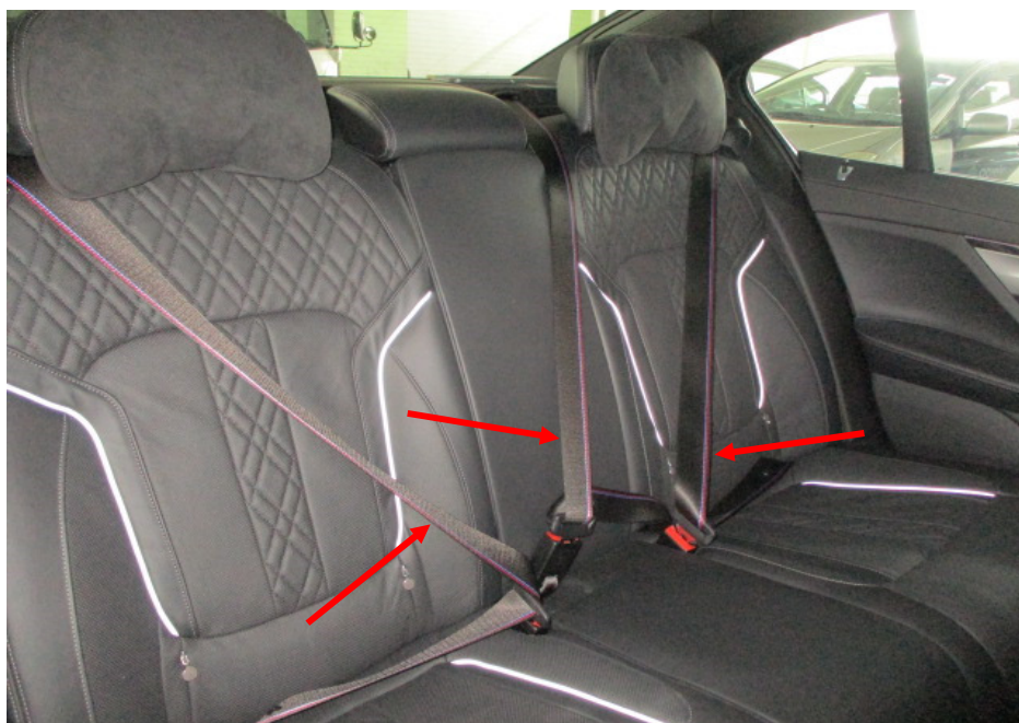
Photo 17 shows the rear seats of the Motor Car. All the seats of the Motor Car were secured via seat rails to the floorboard. They were also fitted with a retractable seat belt reel and a pre-tensioner. The seat belts (arrowed) were tested and were able to be fastened into the respective pre-tensions that were fitted on the side of each individual seat.
