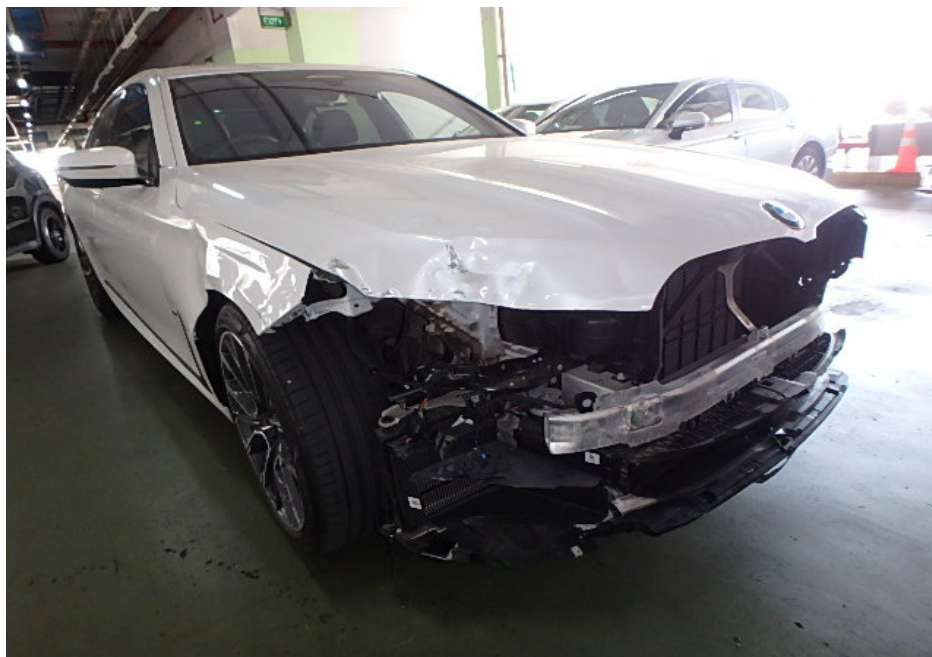
Photo 1 shows the front right body of the Motor Car (photograph provided to me). The Motor Car was observed to have sustained damage at its front right portion. The front bumper reinforcement, front bonnet and front right fender were amongst the body parts that were observed to be damaged. The front right headlamp, front bumper and all its related parts and attachments were observed to be damaged/missing/dislodged.
