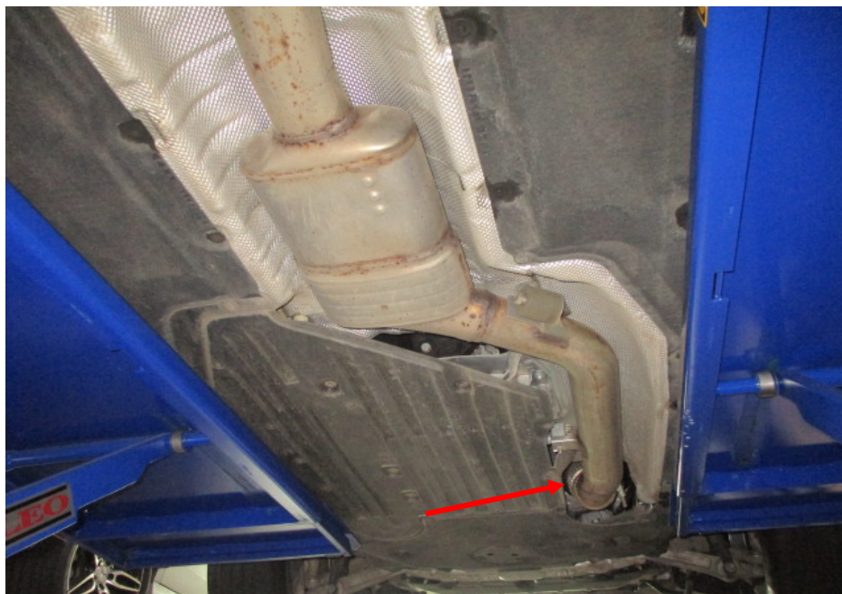
Photo 26 shows a general view of the front section of the Motor Car's exhaust system. My examination of the Motor Car's exhaust system revealed no sign(s) or indication(s) of any cut or weld marks along its exhaust pipes, on its centre resonator box, on its catalytic converter (arrowed) and on its rear muffler.
