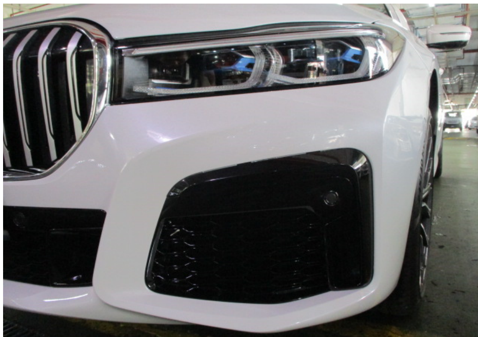
Photo 10 shows a closer view of the Motor Car's front bumper, front bumper left lower grille, front bumper left lower grille garnish and front left headlamp at the time of my inspection. The body parts at the frontal portion of the Motor Car were visually examined, and it was observed that the repair/restoration works carried out to the damaged area of the Motor Car (refer to photograph 3 above) were reasonably adequate and in order.
