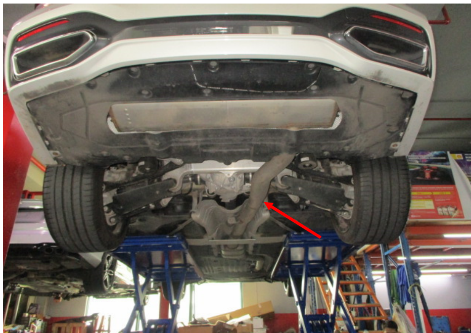
Photo 25 shows a general view of the rear section of the Motor Car's exhaust system. My examination of the Motor Car's exhaust system revealed no sign(s) or indication(s) of any cut or weld marks along its exhaust pipes (arrowed), on its centre resonator box, on its catalytic converter and on its rear muffler.
