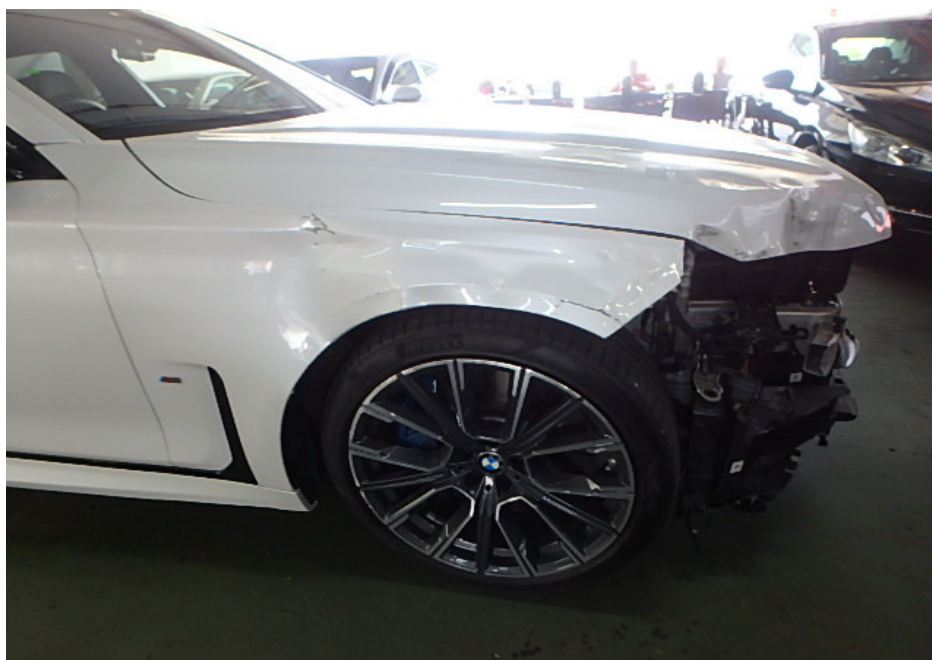
Photo 2 shows another view of the front right body of the Motor Car (photograph provided to me). The front bonnet and front right fender were amongst the body parts that were observed to be damaged.
