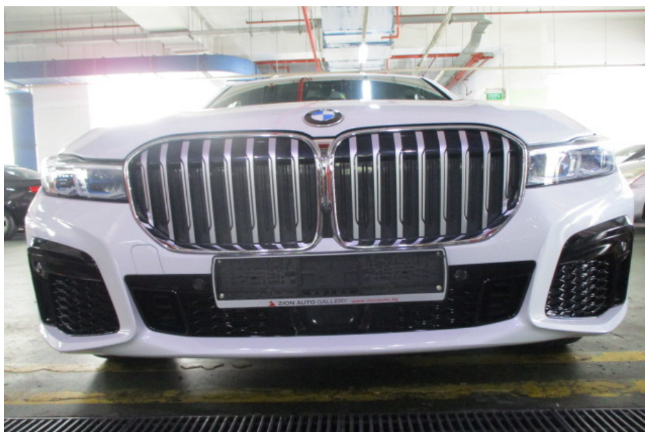
Photo 11 shows a closer view of the Motor Car's front bumper, front bumper centre lower grille, radiator grilles and front headlamps at the time of my inspection. The body parts at the frontal portion of the Motor Car were visually examined, and it was observed that the repair/restoration works carried out to the damaged area of the Motor Car (refer to photograph 1 & 3 above) were reasonably adequate and in order.
