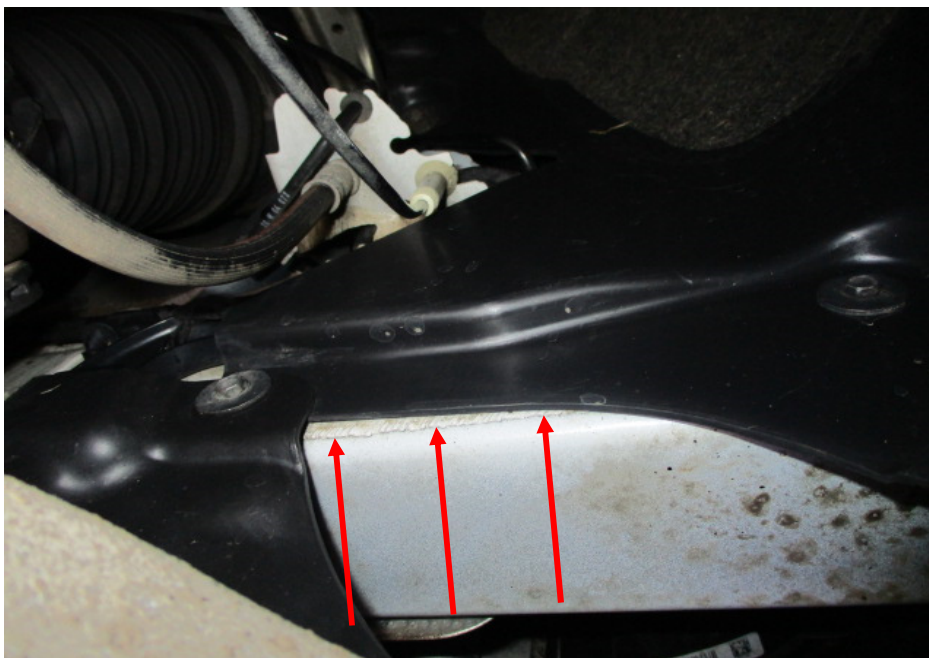
Photo 27 shows the chassis/structural body at the underside front right of the Motor Car. I did not find any weld marks other than original spot weld marks on the chassis/structural body of the Motor Car. The original factory sealant (arrowed) at the joints along the chassis/structural body was untouched, indicating no work was done on the chassis/structural body of the Motor Car and that the chassis/structural body was originally fitted.
