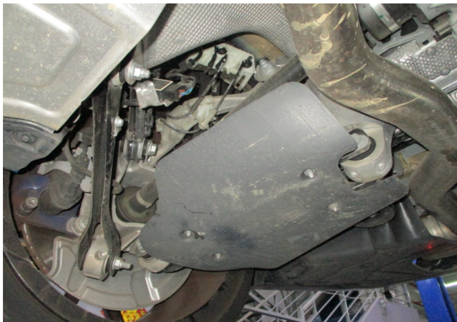
Photo 22 shows the various undercarriage components at the rear right wheel of the Motor Car. The various mechanical components, control arms and linkages were all found to be intact and secured in an appropriate manner.
