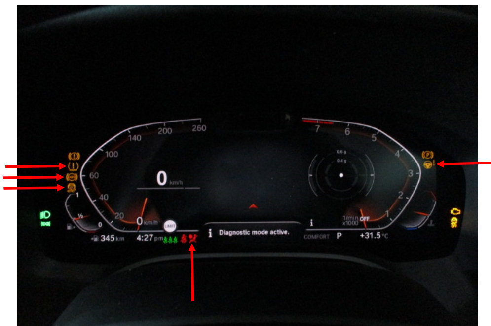
Photo 18 shows the warning lights for the various electronic safety features appearing on the instrument panel of the Motor Car during its self-test when the engine is cranked, in particular the ABS, SRS, IAS, TPM and DSC lights (arrowed).
