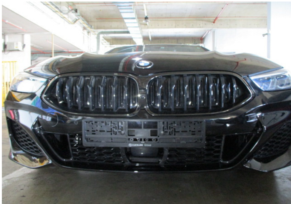
Photo 11 shows a closer view of the Motor Car's front bumper, front bumper front bumper centre lower grille and front radar unit. The body parts at the frontal portion of the Motor Car were visually examined and it was observed that the repair/restoration works carried out to the damaged area of the Motor Car (refer to photograph 1 & 2) were reasonably adequate and in order.
