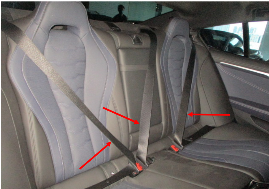
Photo 17 shows the rear seats of the Motor Car. All the seats of the Motor Car were secured via seat rails to the floorboard. They were also fitted with a retractable seat belt reel and a pre-tensioner. The seat belts (arrowed) of the Motor Car were tested and were able to be fastened into the respective pre-tensions that were fitted on the side of each individual seat.
