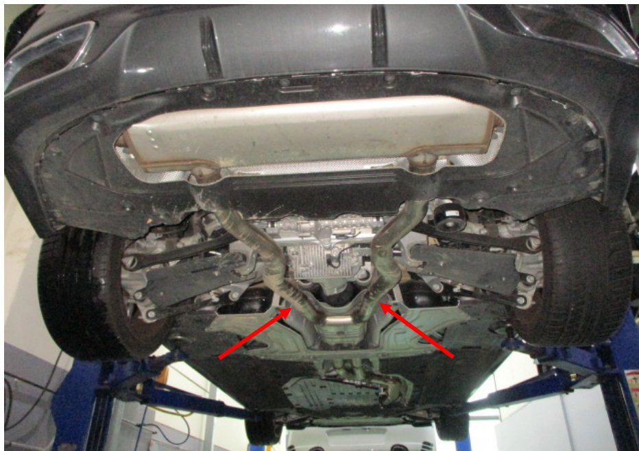
Photo 25 shows a general view of the rear section of the Motor Car's exhaust system. My examination of the Motor Car's exhaust system revealed no sign(s) or indication(s) of any cut or weld marks along its exhaust pipes (arrowed), on its catalytic converter, on its centre resonator box and on its rear muffler.
