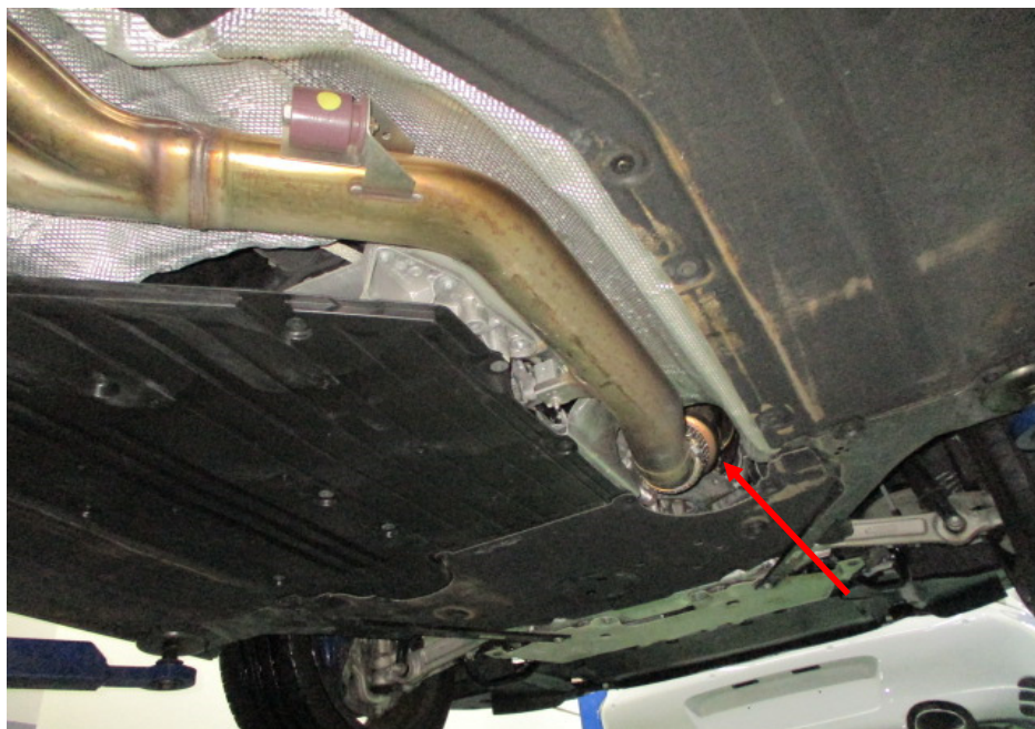
Photo 26 shows a general view of the front section of the Motor Car's exhaust system. My examination of the Motor Car's exhaust system revealed no sign(s) or indication(s) of any cut or weld marks along its exhaust pipes, on its catalytic converter (arrowed), on its centre resonator box and on its rear muffler.
