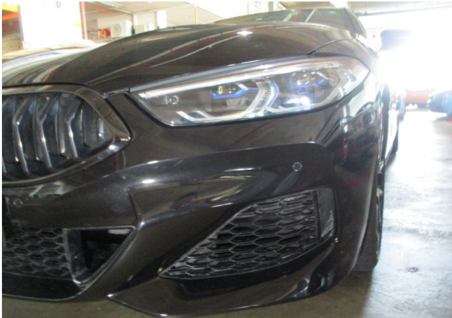
Photo 6 shows a closer view of the Motor Car's front bumper, front bumper left lower grille, front sensors and front left headlamp. The body parts at the frontal portion of the Motor Car were visually examined and it was observed that the repair/restoration works carried out to the damaged area of the Motor Car (refer to photograph 1 & 2) were reasonably adequate and in order.
