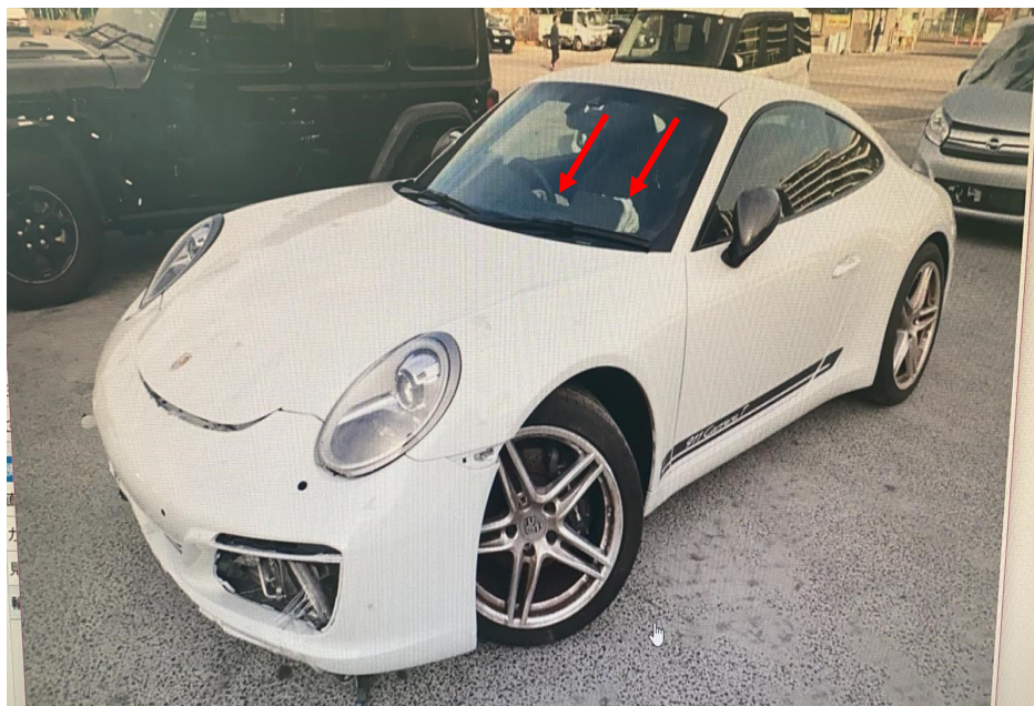
Photo 2 shows the front left body of the Motor Car (photograph provided to me). The Motor Car was observed to have sustained damage at its frontal portion. The front bumper, front bumper lower lip, front bumper left lower grille, front left day light and front left signal lamp were amongst the body parts that were observed to have been damaged. As seen from the photograph, the driver's airbag and front left passenger airbag were activated (arrowed).
