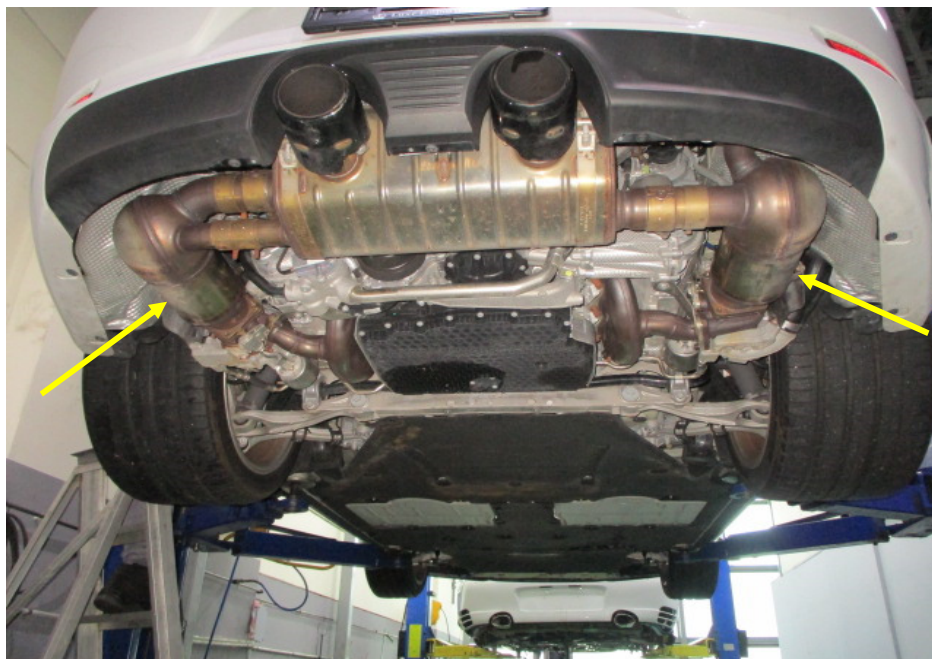
Photo 23 shows the Motor Car's exhaust system. My examination of the Motor Car's exhaust system revealed no sign(s) or indication(s) of any cut or weld marks along its exhaust pipes, on its exhaust manifolds, on its catalytic converters (arrowed) and on its rear muffler.
