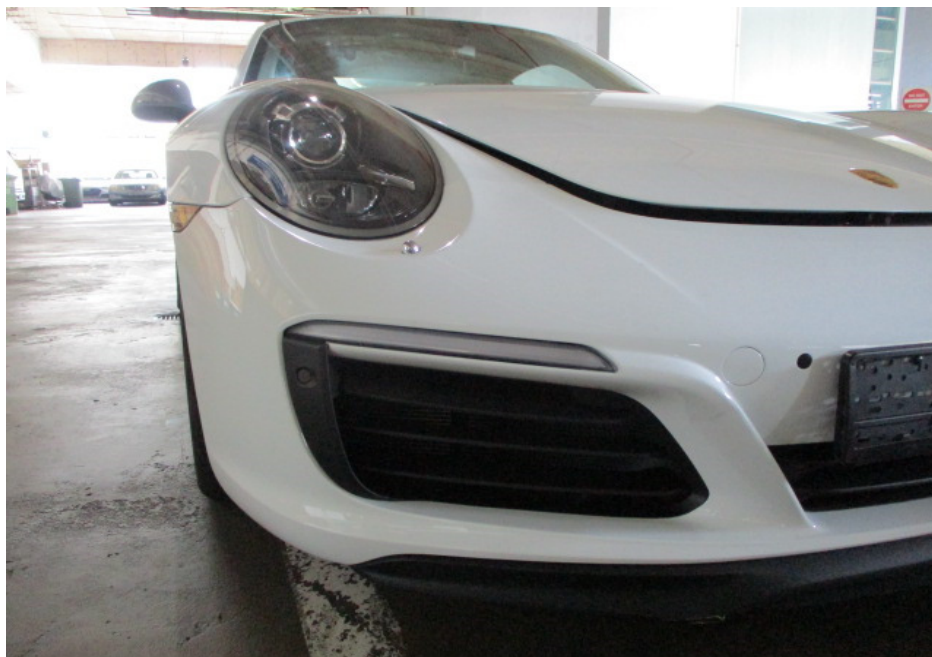
Photo 6 shows a closer view of the Motor Car's front bumper, front bumper lower lip, front bumper right lower grille and front right day light. The body parts at the frontal portion of the Motor Car were visually examined and it was observed that the repair/restoration works carried out to the damaged area of the Motor Car (refer to photograph 1 above) were reasonably adequate and in order.
