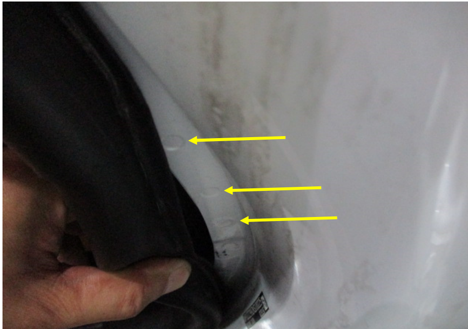
Photo 30 shows the front right "A" pillar of the Motor Car. I did not find any weld marks other than original spot weld marks (arrowed) on front right "A" pillar of the Motor Car, which indicates that there was no re-welding works carried out. In general, I had found all the non-detachable body panels of the Motor Car to be originally fitted at the time of my inspection.
