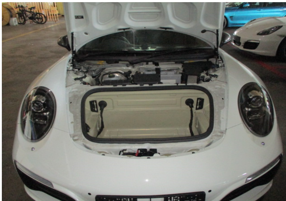
Photo 10 shows a general of the Motor Car's front bonnet compartment at the time of my inspection. Original spot weld marks and original factory sealant were found on the non-detachable body panels at the frontal portion of the Motor Car. The non-detachable body panels at the frontal portion of the Motor Car were originally fitted.
