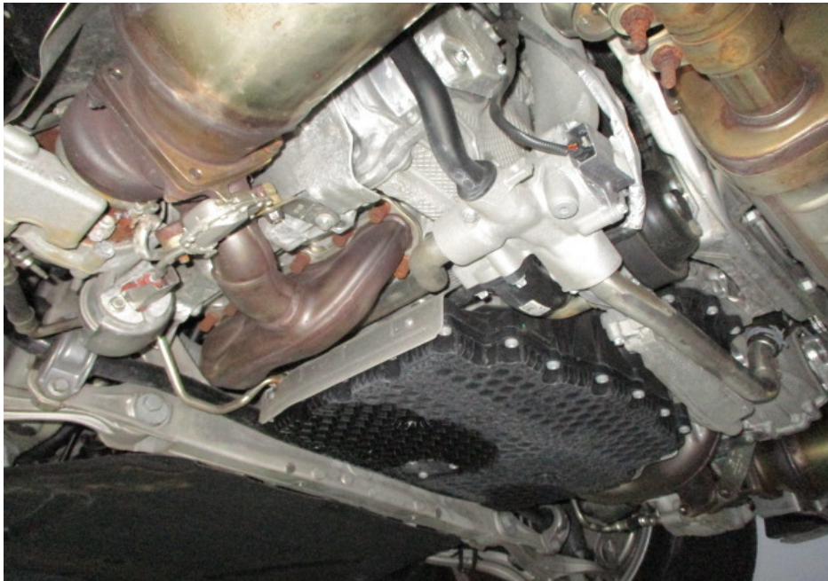
Photo 24 shows a general view of the Motor Car's engine compartment. The engine compartment was at the rear underside of the Motor Car. The various parts and components inside the engine compartment were all observed to be intact and properly fitted. There was also no sign(s) or indication(s) of fluid leak and/or fluid stain found inside the engine compartment.
