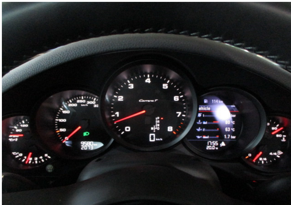
Photo 17 shows the respective warning lights no longer illuminated, indicating that there is no fault detected to the ABS, SRS and TCS systems of the Motor Car during the self-test. These electronic systems were hence in working condition at the time of my inspection.
