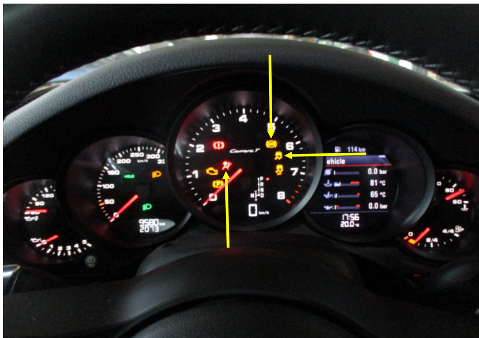
Photo 16 shows the warning lights for the various electronic safety features appearing on the instrument panel of the Motor Car during its self-test when the engine is cranked, in particular the ABS, SRS and TCS lights (arrowed).
