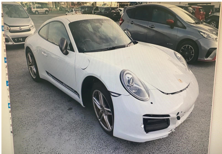
Photo 1 shows the front right body of the Motor Car (photograph provided to me). The Motor Car was observed to have sustained damage at its frontal portion. The front bumper, front bumper lower lip, front bumper right lower grille and front right day light were amongst the body parts that were observed to have been damaged. The front right wheel was seen to be tilted outwards, indicating damage to the front right undercarriage parts of the Motor Car.
