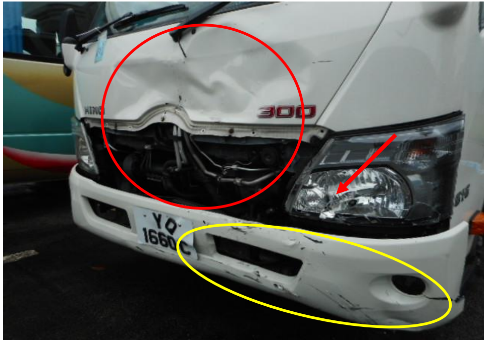
Photo 4 shows a close up view of the Motor Lorry's front portion at the time of my inspection. Its front bumper (yellow circle) and front body panel (red circle) and front left headlamp (arrowed) was damage at the time of my inspection as a result of the accident.
