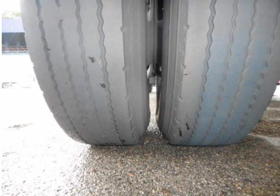
Photo 10 shows the condition of the rear left tyres of the Motor Lorry, which was observed to be in serviceable condition with remaining tread depth of approximately 2.4mm. The tyres, which were wrapped around standard steel wheel rim, were also observed to be sufficiently inflated for vehicular operation. There was also no damage found on all 6 steel wheel rims of the Motor Lorry.
