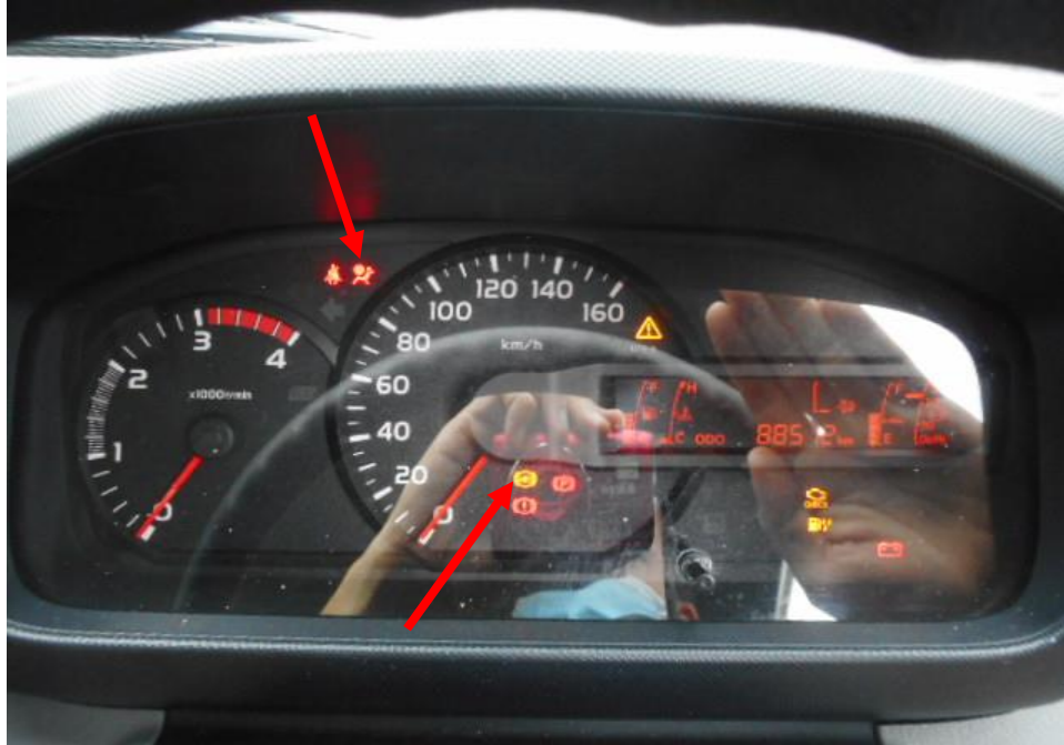
Photo 25 shows the warning light for Anti-Lock Brake System (ABS), and Supplemental Restraint System (SRS) (arrowed) appearing on the instrument panel of the Motor Car during the self-test of its various electronic operating systems when its engine was cranked.
