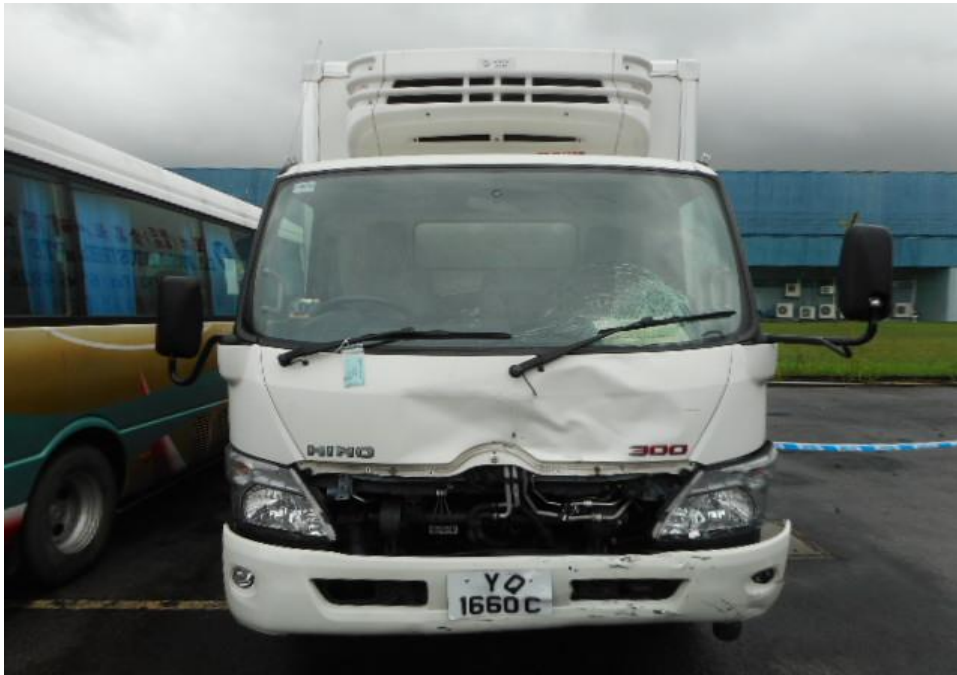
Photo 2 shows a general view of the Motor Lorry's frontal portion at the time of my inspection. It appeared to have sustained damage at its front portion. Its front windscreen, front body panel, front left headlamp and front bumper were damage at the time of my inspection as a result of the accident.
