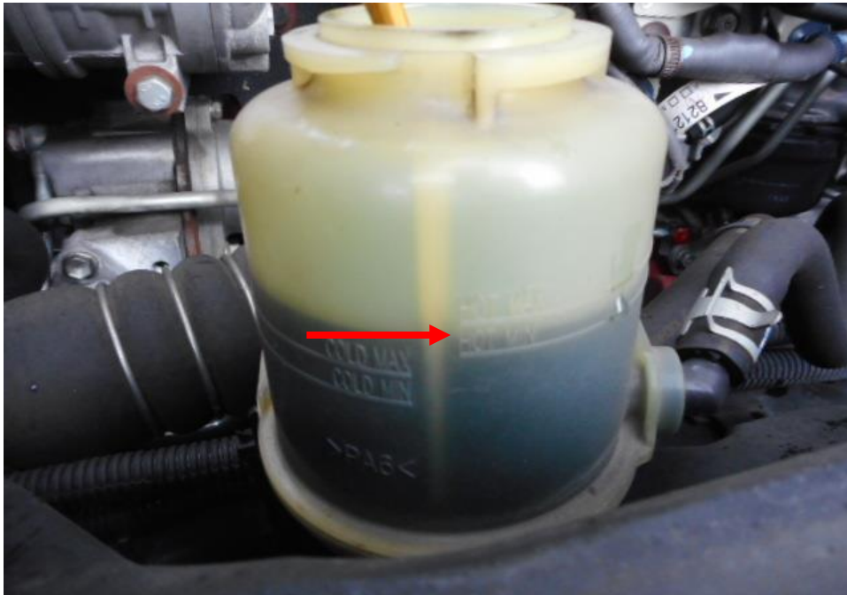
Photo 16 shows the power steering fluid reservoir of the Motor Lorry at the time of my inspection. The power steering fluid was observed to be of sufficient level (arrowed) and without any visible contamination.
