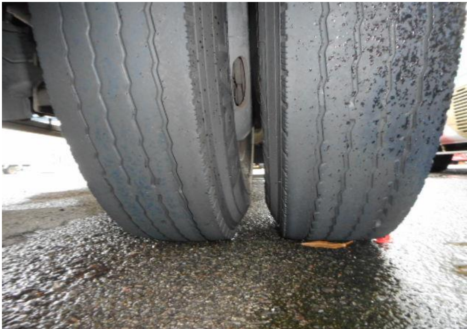
Photo 9 shows the condition of the rear right tyre of the Motor Lorry, which was observed to be in serviceable condition with remaining tread depth of approximately 1.9mm. The tyre, which was wrapped around standard steel wheel rim, it was observed to be sufficiently inflated for vehicular operation.
