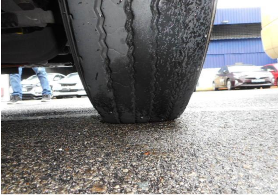
Photo 8 shows the condition of the front right tyre of the Motor Lorry, which was observed to be in serviceable condition with remaining tread depth of approximately 5.3mm. The tyre, which was wrapped around standard steel wheel rim, was also observed to be sufficiently inflated for vehicular operation. There was no tear, cut or burst mark(s) on the outer and the inner sidewalls as well as across the tread of the 6 tyres that were fitted on the Motor Lorry.
