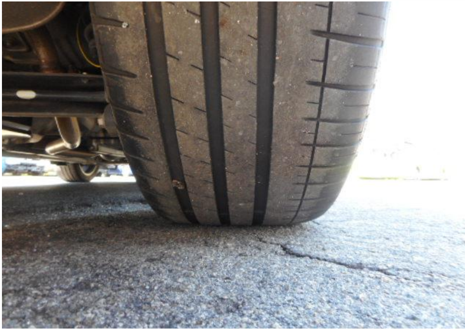
Photo 8 shows the condition of the rear right tyre of the Motor Car, which was observed to be in serviceable condition with remaining tread depth of approximately 3.6mm. The tyre was also observed to be sufficiently inflated for vehicular operation with no tear, cut or burst mark(s).
