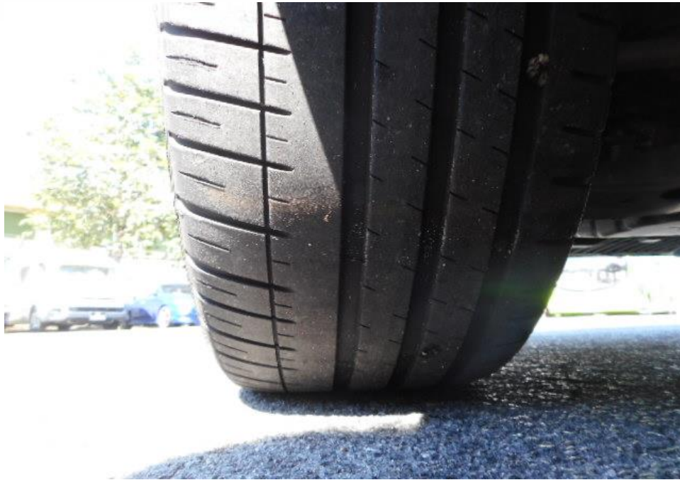
Photo 10 shows the condition of the front left tyre of the Motor Car, which was observed to be in serviceable condition with remaining tread depth of approximately 3mm. There was also no tear, cut or burst mark(s) on the outer and the inner sidewalls as well as across the tread of the Motor Car's 4 tyres.
