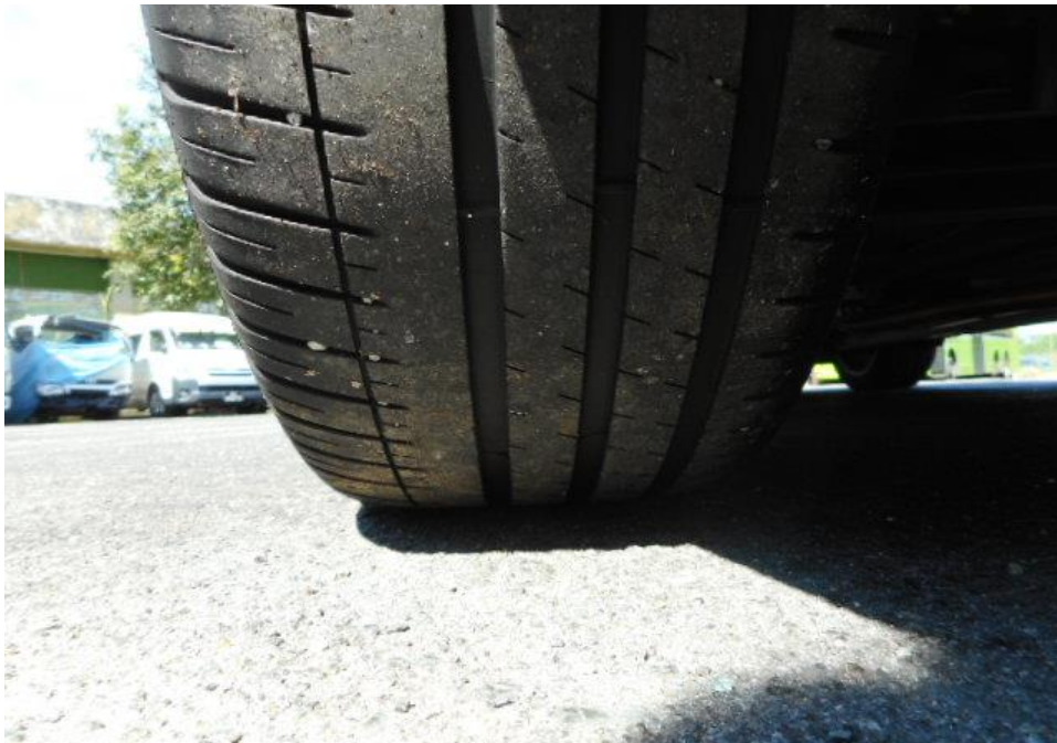
Photo 9 shows the condition of the rear left tyre of the Motor Car, which was observed to be in serviceable condition with remaining tread depth of approximately 3.6mm. The tyre, which was wrapped around steel wheel rim, was also observed to be sufficiently inflated for vehicular operation. The 4 tyres of the Motor Car were wrapped around standard steel wheel rims.
