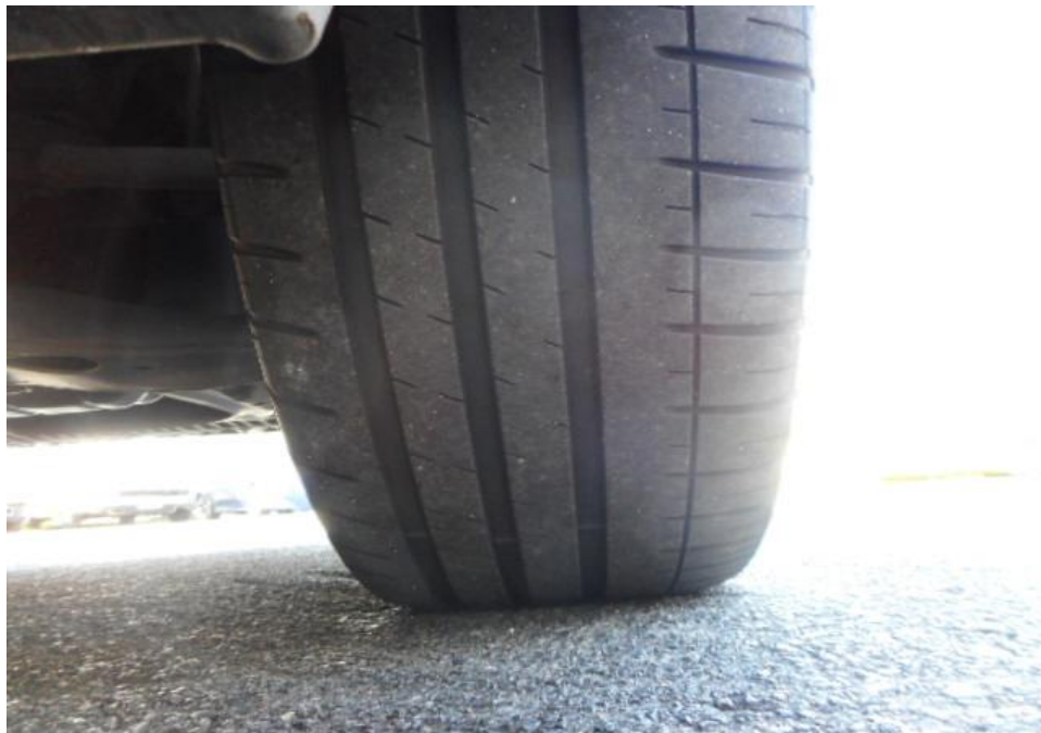
Photo 7 shows the condition of the front right tyre of the Motor Car, which was observed to be in serviceable condition with remaining tread depth of approximately 3.3mm. The tyre was sufficiently inflated for vehicular operation with no tear, cut or burst mark(s) on the outer and the inner sidewalls as well as across the tread. The 4 tyres of the Motor Car were wrapped around standard steel wheel rims without any damage.
