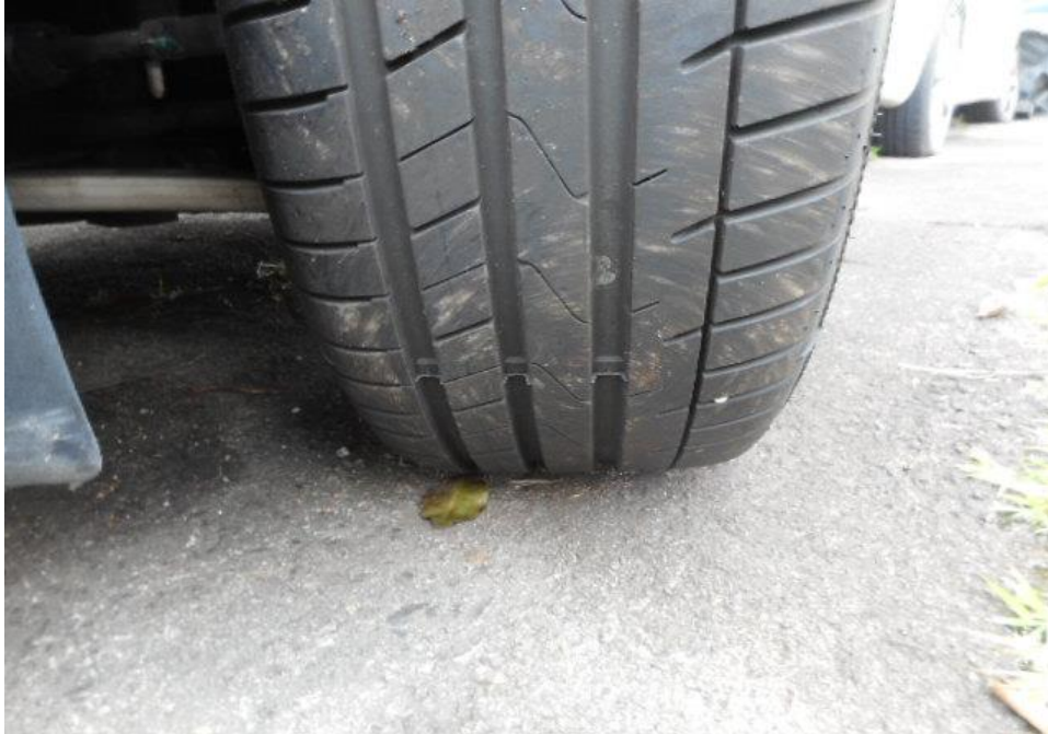
Photo 8 shows the condition of the front right tyre of the Motor Car, which was observed to be in serviceable condition with remaining tread depth of approximately 6.6mm. The tyre was sufficiently inflated for vehicular operation with no tear, cut or burst mark(s) on the outer and the inner sidewalls as well as across the tread. The 4 tyres of the Motor Car were wrapped around standard steel wheel rims without any damage.
