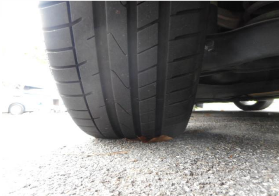
Photo 10 shows the condition of the rear left tyre of the Motor Car, which was observed to be in serviceable condition with remaining tread depth of approximately 6.2mm. The tyre, which was wrapped around steel wheel rim, was also observed to be sufficiently inflated for vehicular operation. The 4 tyres of the Motor Car were wrapped around standard steel wheel rims.
