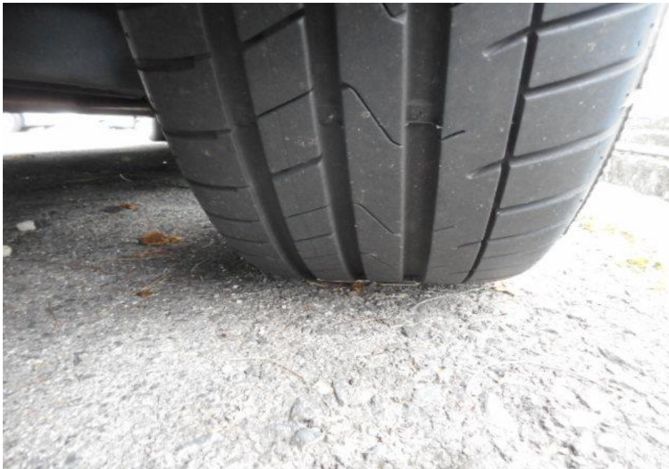
Photo 9 shows the condition of the rear right tyre of the Motor Car, which was observed to be in serviceable condition with remaining tread depth of approximately 6.2mm. The tyre was also observed to be sufficiently inflated for vehicular operation with no tear, cut or burst mark(s).
