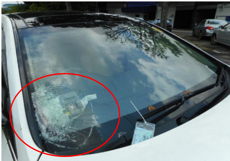
Photo 3 shows a close up view of the Motor Car's front body at the time of my inspection. The front portion of the Motor Car was observed to have sustained damage. Its front windscreen (circled) was the body part that were damaged as a result of the accident.
