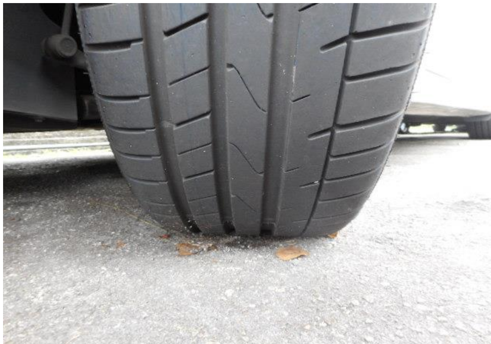
Photo 11 shows the condition of the front left tyre of the Motor Car, which was observed to be in serviceable condition with remaining tread depth of approximately 6.6mm. There was also no tear, cut or burst mark(s) on the outer and the inner sidewalls as well as across the tread of the Motor Car's 4 tyres.
