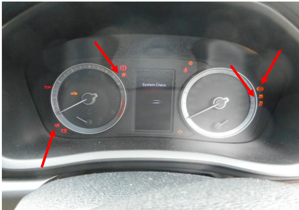
Photo 24 shows the warning light for Anti-Lock Brake System (ABS), Electric Power Steering System (EPS), Traction Control System (TCS) and Supplemental Restraint System (SRS) (arrowed) appearing on the instrument panel of the Motor Car during the self-test of its various electronic operating systems when its engine was cranked.
