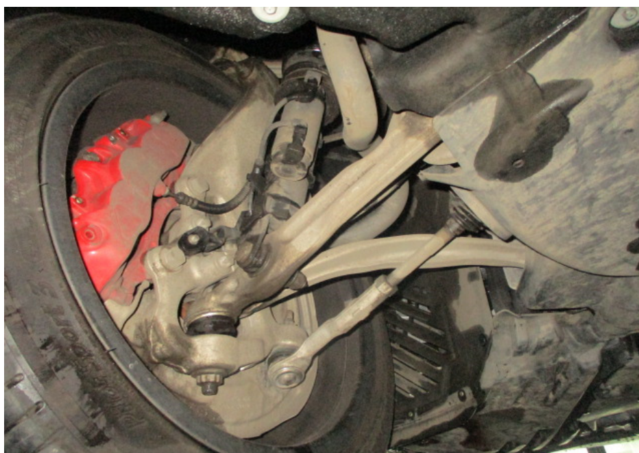
Photo 23 shows the various undercarriage components at the front left wheel of the Motor Car. The mechanical components, control arms and linkages were all found to be intact and secured in an appropriate manner.
