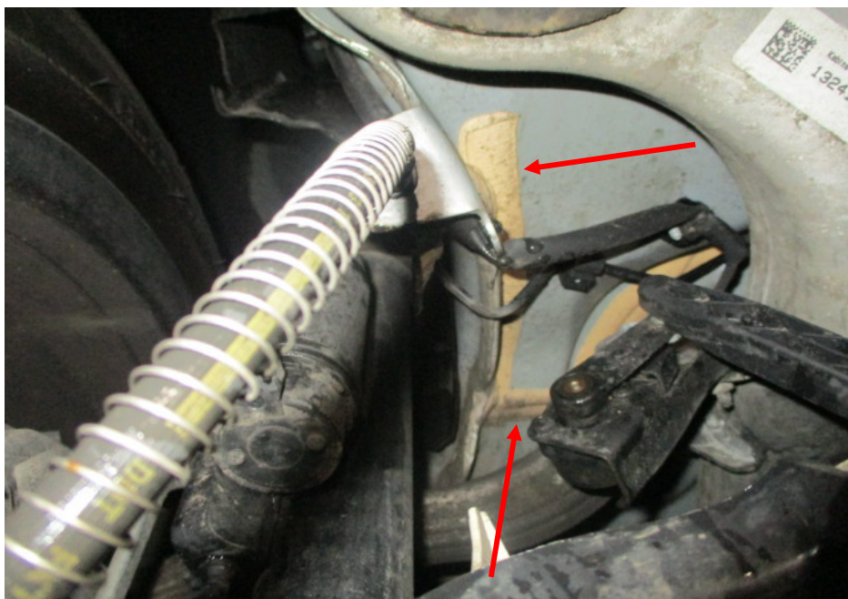
Photo 29 shows the chassis/structural body at the underside rear left of the Motor Car. I did not find any weld marks other than original spot weld marks on the chassis/structural body of the Motor Car. The original factory sealant (arrowed) at the joints along the chassis/structural body was untouched, indicating no work was done on the chassis/structural body of the Motor Car and that the chassis/structural body was originally fitted.
