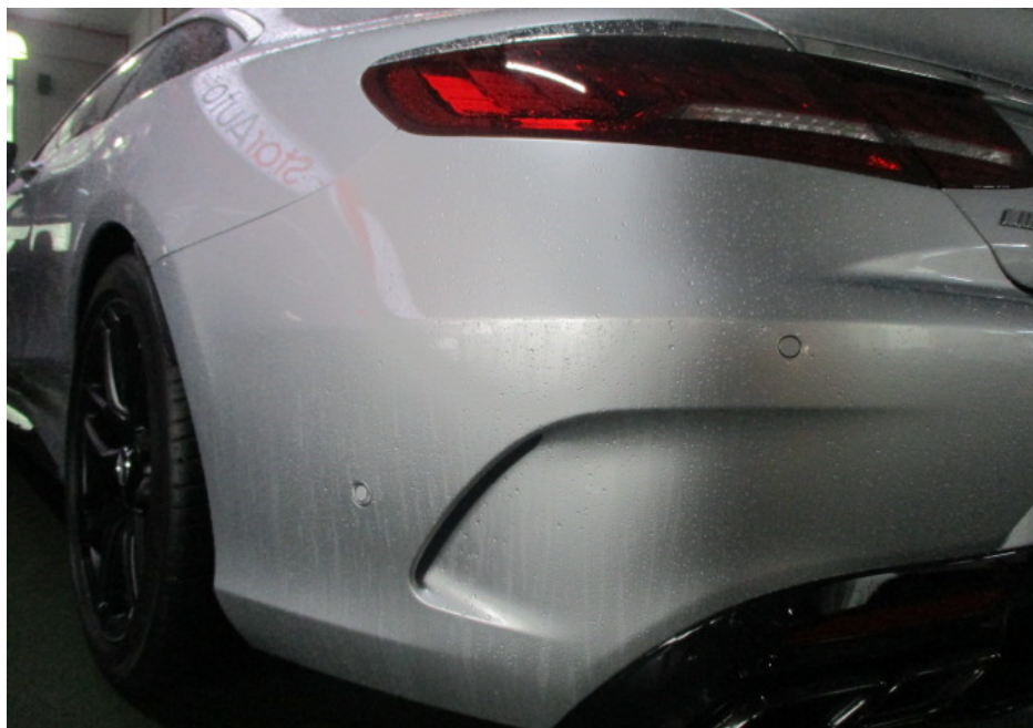
Photo 12 shows a closer view of the Motor Car's rear bumper, rear bumper left sensors and rear left taillamp at the time of my inspection. The body parts at the rear left portion of the Motor Car were visually examined, and it was observed that the repair/restoration works carried out to the damaged area of the Motor Car (refer to photograph 3 & 4 above) were reasonably adequate and in order.
