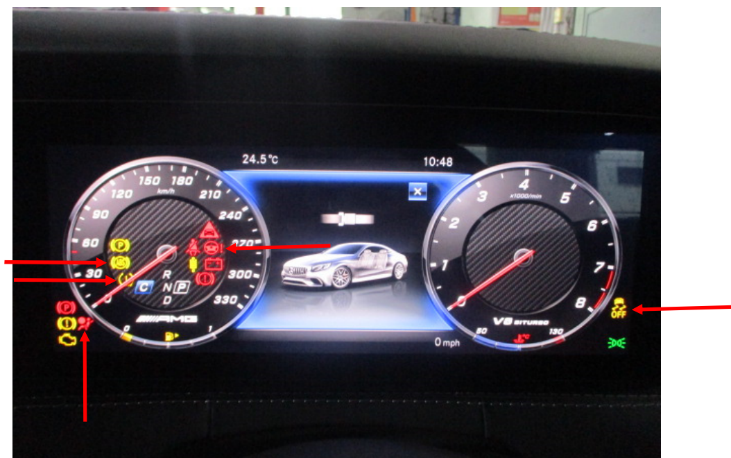
Photo 18 shows the warning lights for the various electronic safety features appearing on the instrument panel of the Motor Car during its self-test when the engine is cranked, in particular the ABS, SRS, EPS, TPM and TCS lights (arrowed).
