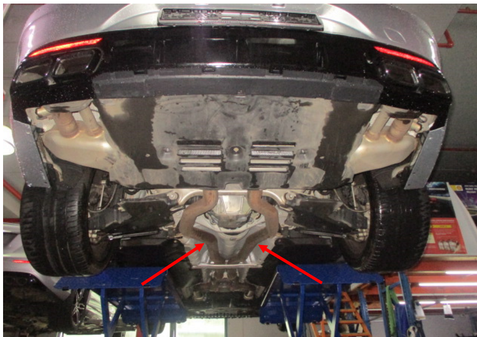
Photo 25 shows a general view of the rear section of the Motor Car's exhaust system. My examination of the Motor Car's exhaust system revealed no sign(s) or indication(s) of any cut or weld marks along its exhaust pipes (arrowed), on its catalytic converters and on its rear mufflers.
