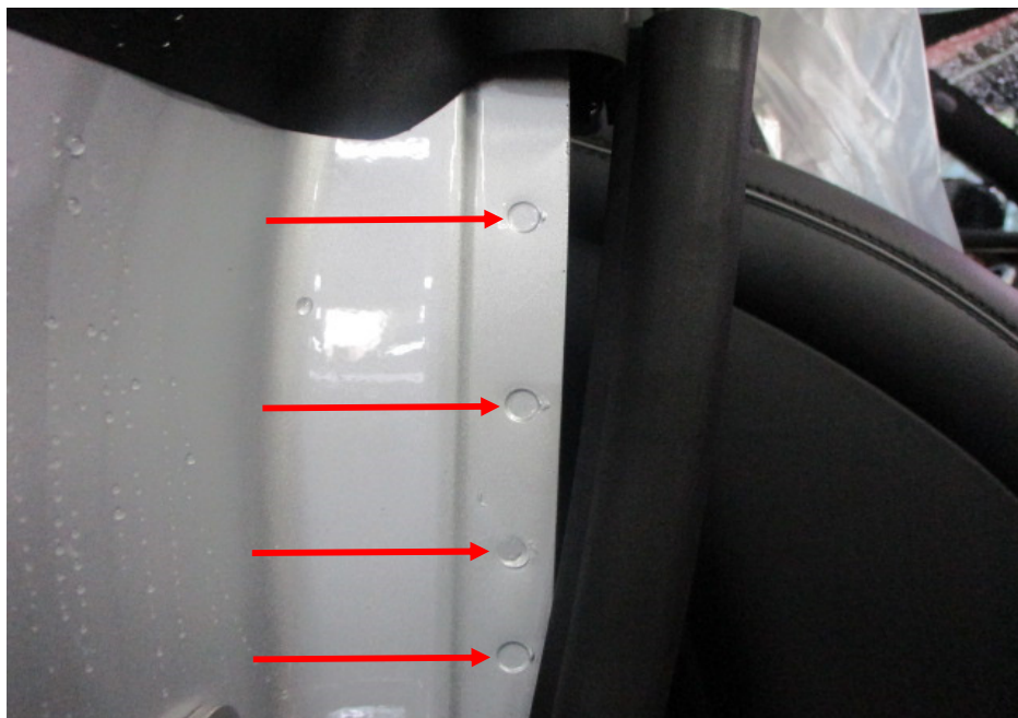
Photo 32 shows the right side rear body panel of the Motor Car. I did not find any weld marks other than original spot weld marks (arrowed) on the right side rear body panel of the Motor Car which, indicates that there was no re-welding works carried out. In general, I had found all the non-detachable body panels of the Motor Car to be originally fitted at the time of my inspection.
