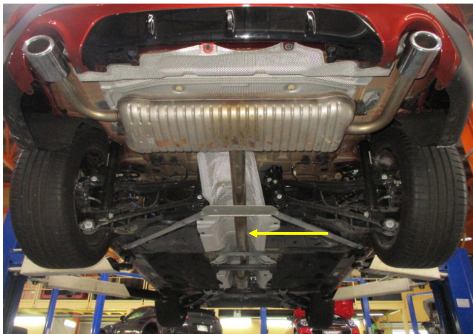
Photo 22 shows a general view of the rear section of the Motor Car's exhaust system. My examination of the Motor Car's exhaust system revealed no sign(s) or indication(s) of any cut or weld marks along its exhaust pipes (arrowed), on its catalytic converter, on its centre resonator box and on its rear muffler.
