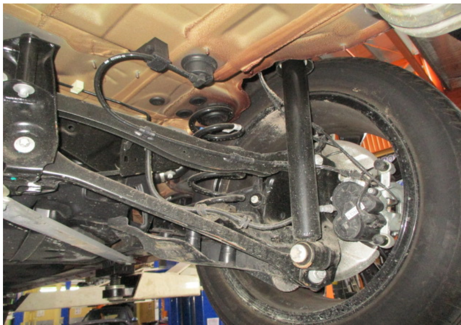
Photo 18 shows a general view of the control arms and linkages at the rear right wheel of the Motor Car. I did not observe any fluid leak and/or fluid stain on the underside of the Motor Car. All of the Motor Car's undercarriage components were observed to be intact and secured in an appropriate manner.
