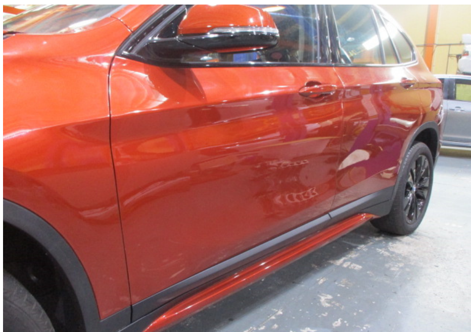
Photo 7 shows a closer view of the Motor Car's left side wing mirror, left side rocker panel garnish, front left door, front left door lower garnish, rear left door and rear left door lower garnish. The body parts along the left side portion of the Motor Car were visually examined and it was observed that the repair/restoration works carried out to the damaged area of the Motor Car (refer to photograph 1 & 2 above) were reasonably adequate and in order.
