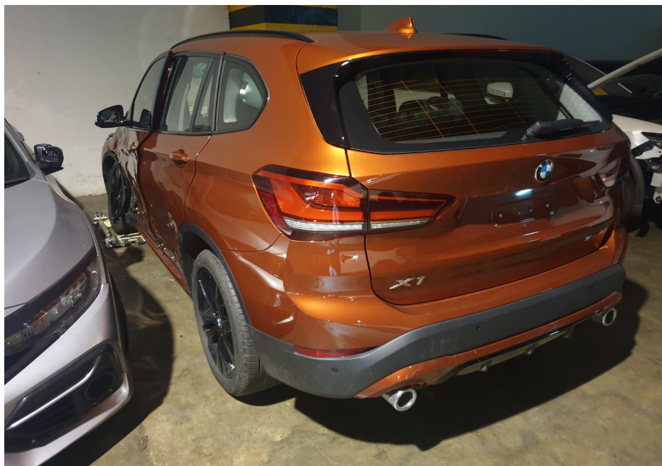
Photo 2 shows the rear left body of the Motor Car (photograph provided to me). Close examination of this photograph had showed damage to the Motor Car's rear left fender wheel arc garnish, rear left door and left side rocker panel garnish amongst others. The front left wheel was also seen to be tilted inwards on a vertical axis, indicating damage to the Motor Car's front left undercarriage parts.
