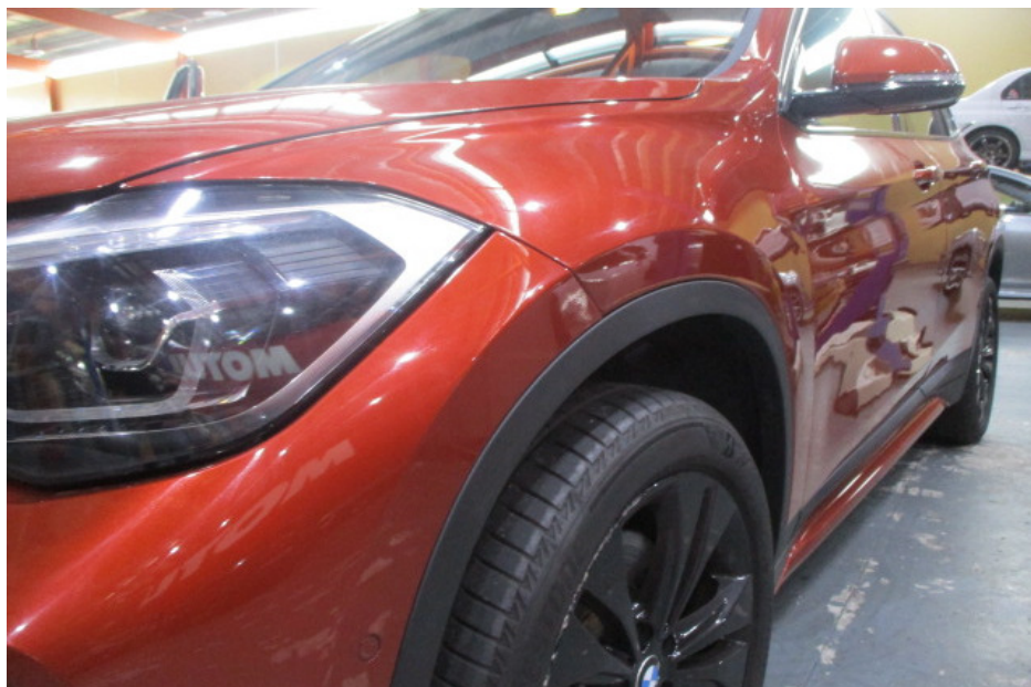
Photo 6 shows a closer view of the front bumper, front left headlamp, front bonnet, front left fender and front left fender wheel arc garnish of the Motor Car at the time of my inspection. The body parts along the left side portion of the Motor Car were visually examined and it was observed that the repair/restoration works carried out to the damaged area of the Motor Car (refer to photograph 1 above) were reasonably adequate and in order.
