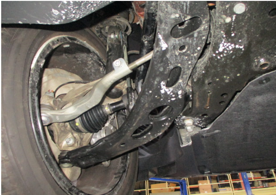
Photo 20 shows the various undercarriage components at the front left wheel of the Motor Car. The mechanical components, control arms and linkages were all found to be intact and secured in an appropriate manner.
